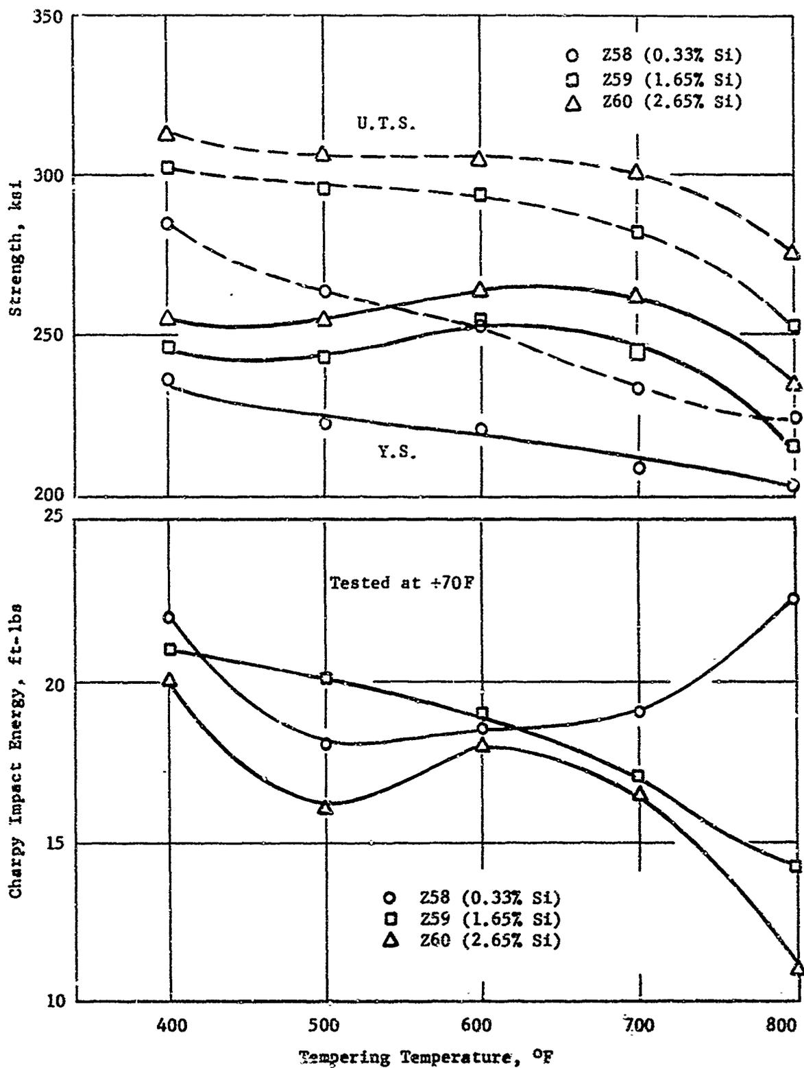
Figure 19. The Influence of Tempering Temperature on Strength and Toughness Properties of Alloys Z58, Z59, and Z60
