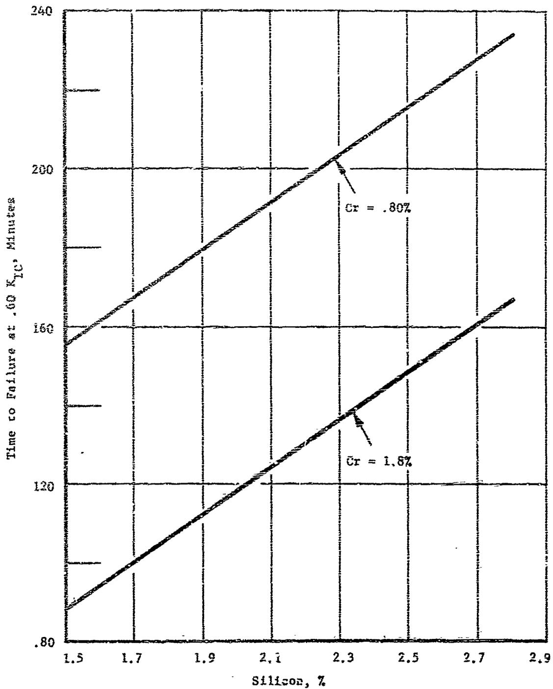
Figure 5'. The Influence of Si Content on Time to Failure at  $K_{II} = 0.60 K_{Ic}$  for Ni-Cr-Mo-Si-V Martensitic Steels
