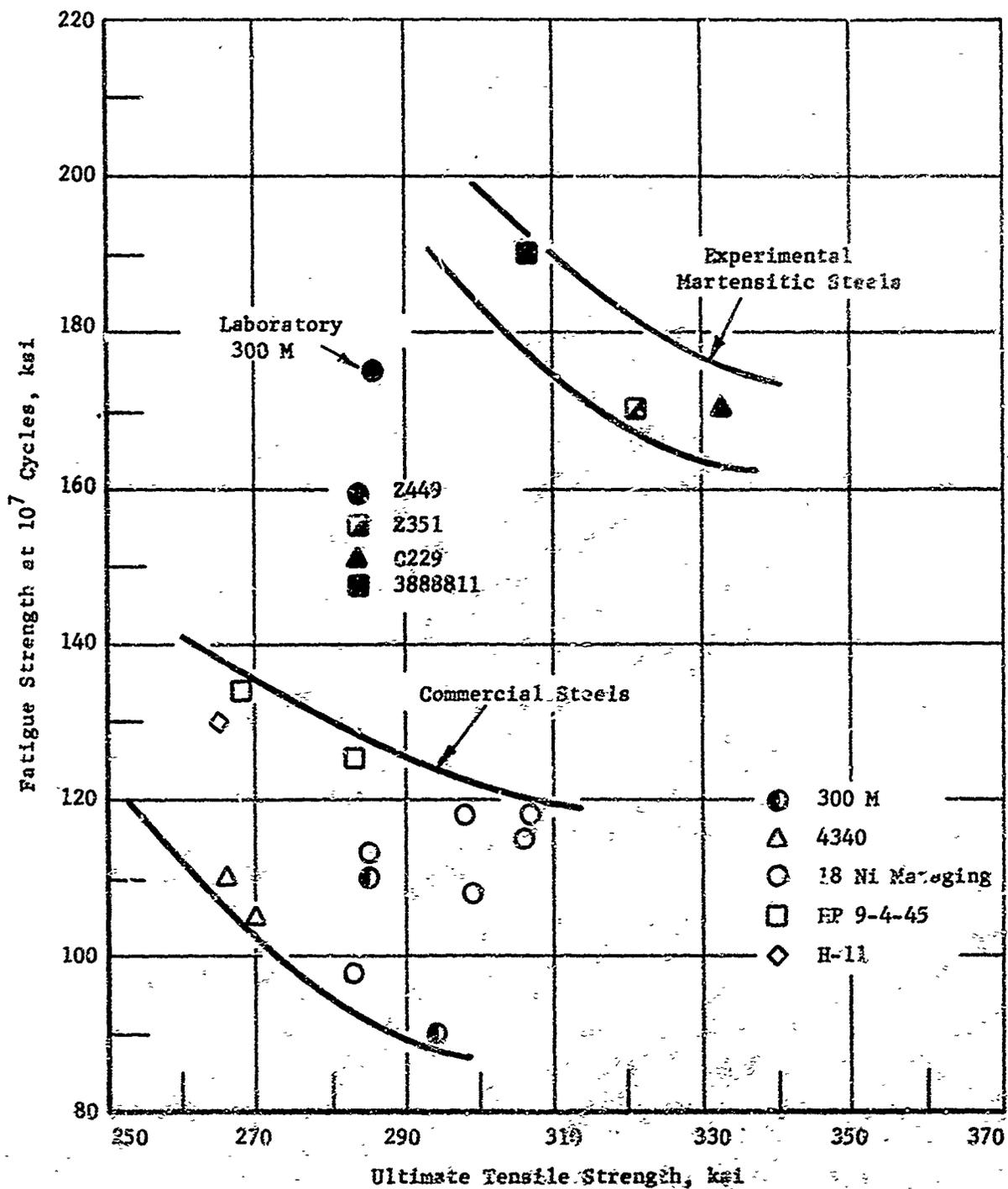
Figure 91. Comparison of the Unnotch 10<sup>7</sup> Cycle Fatigue Strengths of Experimental Martensitic Steels with Commercial High Strength Steels for R Values of +0.06 or +0.10
