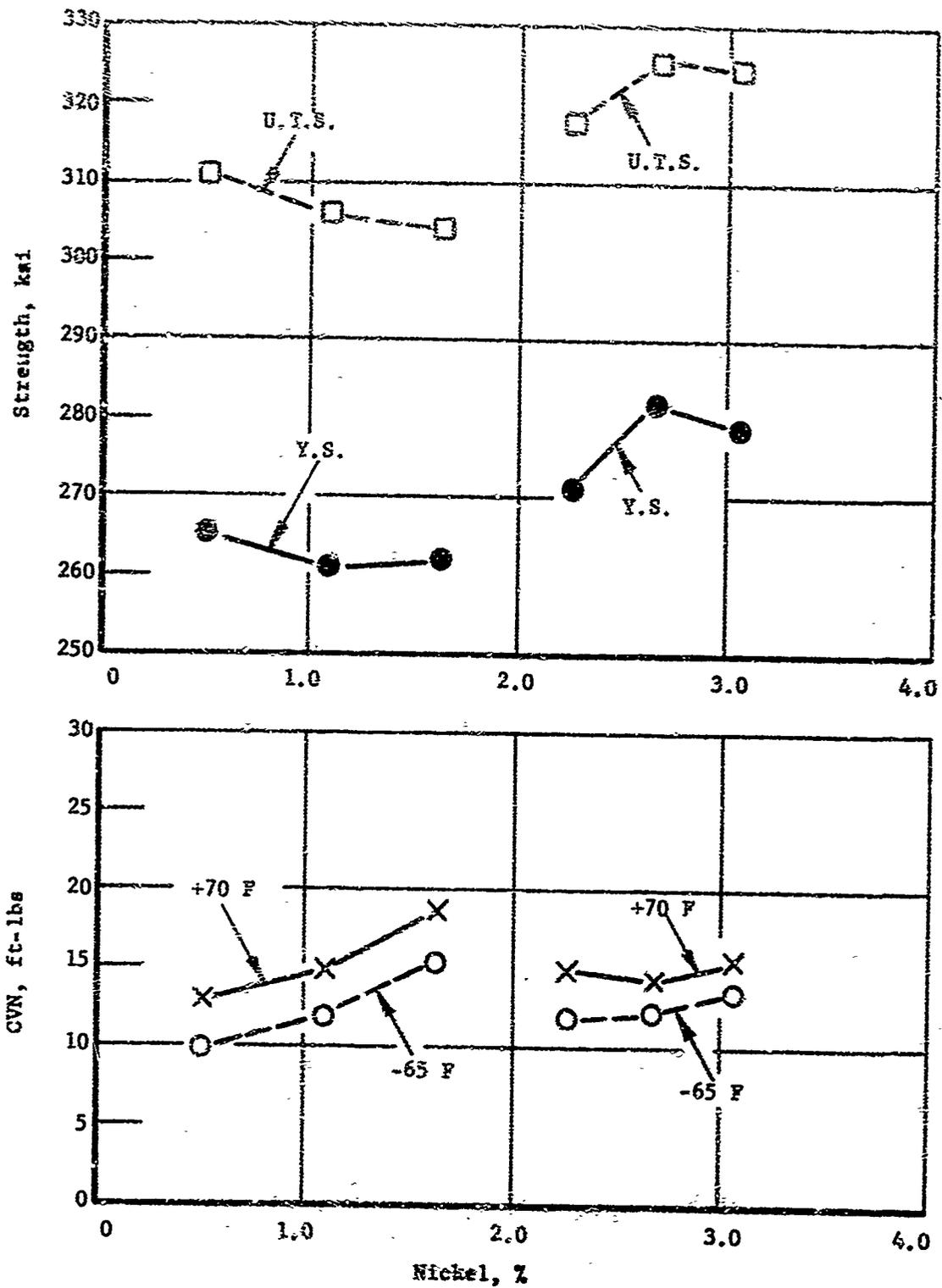
Figure 25. The Influence of Ni on Strength and Toughness in a Ni-Cr-Mn-Si-V Martensitic Steels
