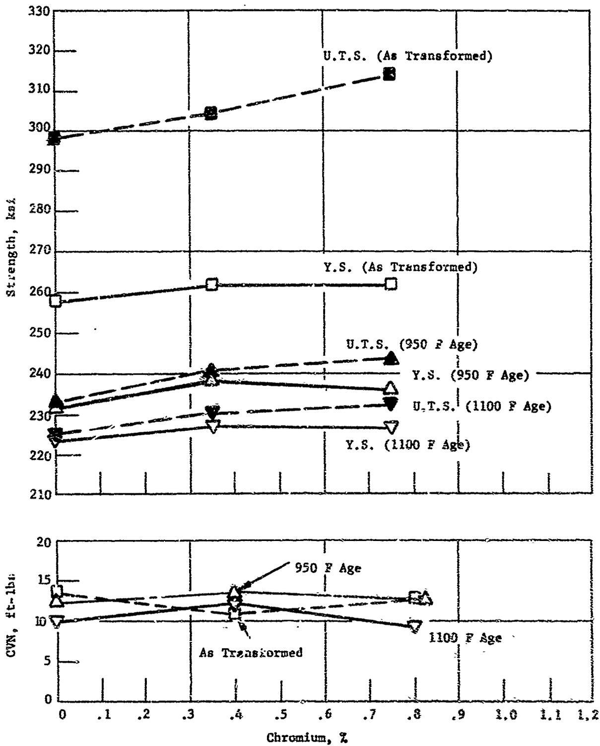
Figure 5. The Effect of Chromium on Strength and Toughness in Low Alloy Bainiting Steels
