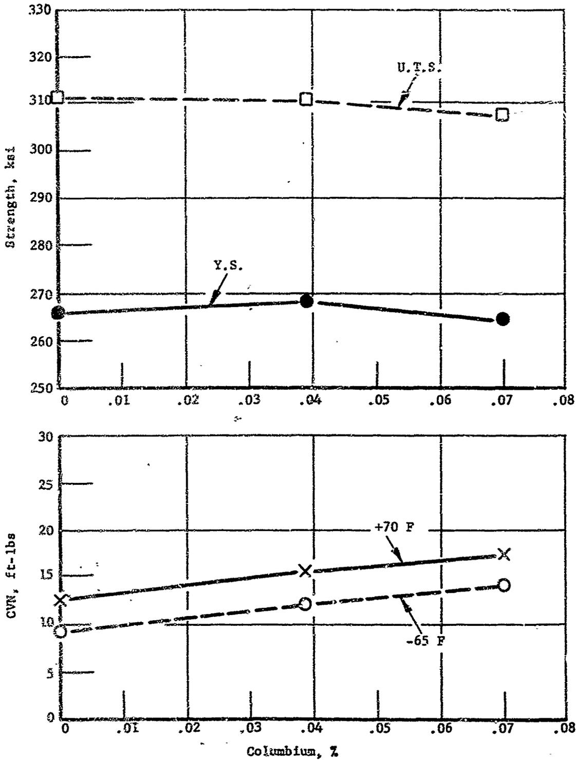
Figure 28. The Influence of Cb on Strength and Toughness in a Ni-Cr-Mo-Si Martensitic Steel
