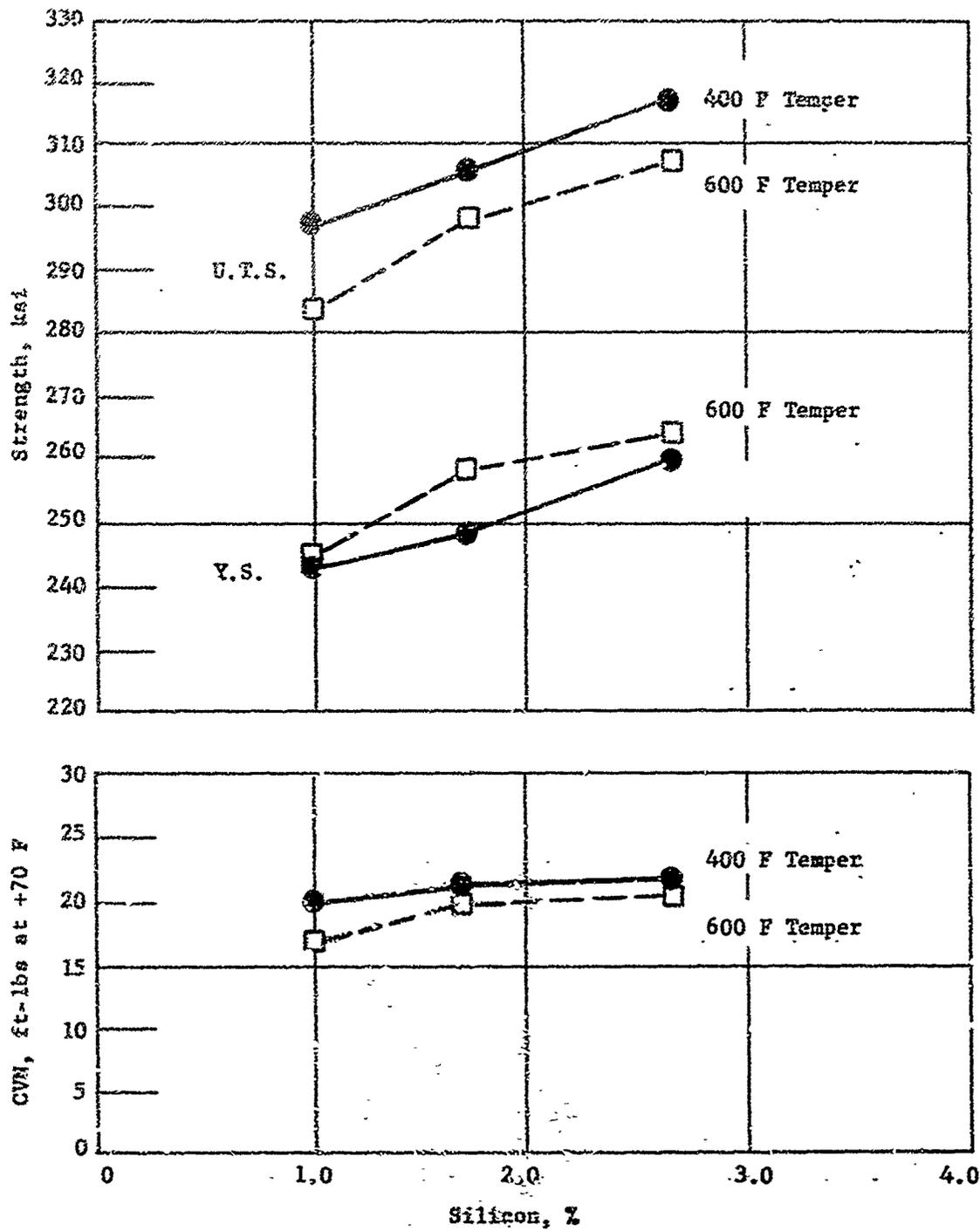
Figure 13. The Effect of Silicon on Strength and Toughness in Ni-Cr-Mn-Si-V Martensitic Alloys (Z43, Z44, Z45)
