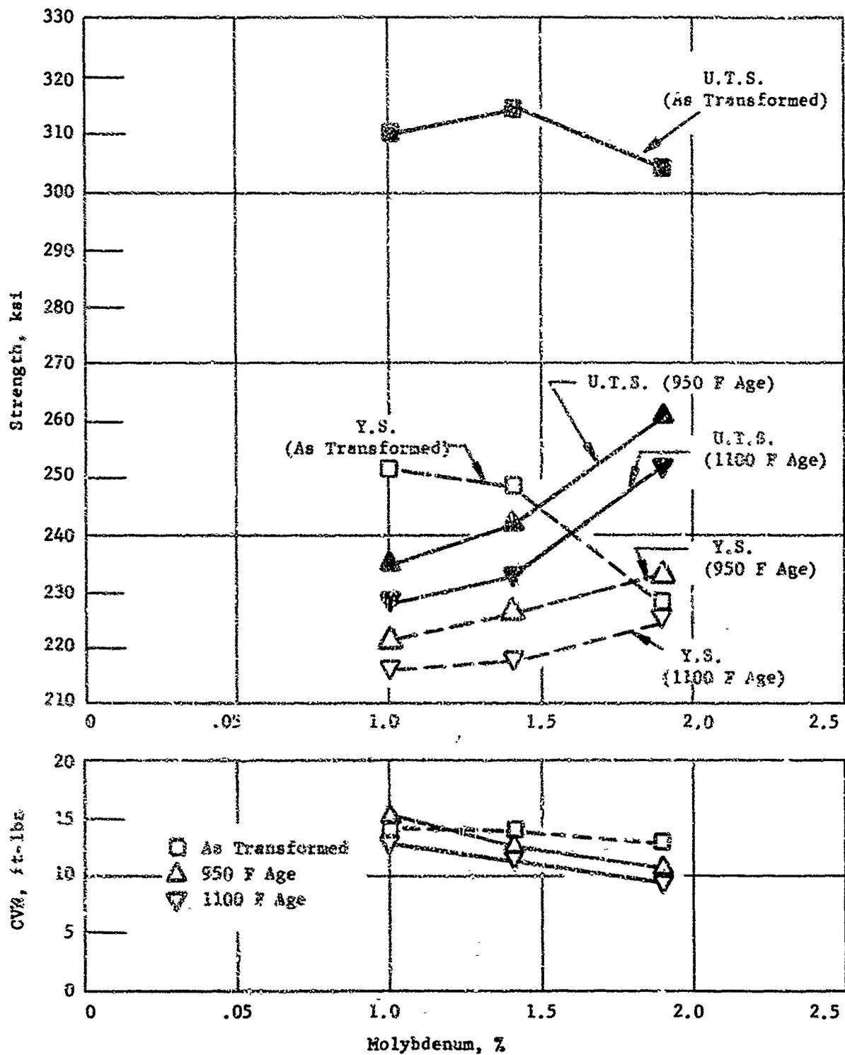
Figure 6. The Effect of Molybdenum on Strength and Toughness in Low Alloy Bainiting Steels
