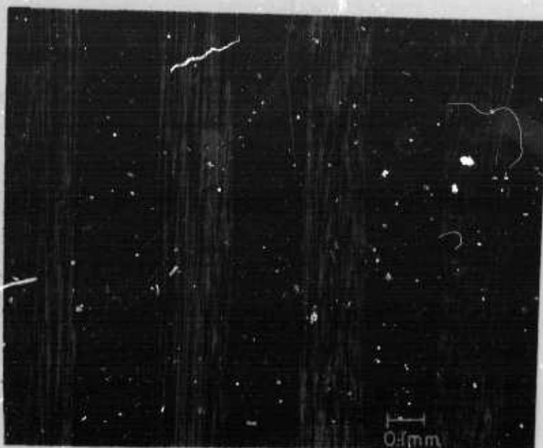
Figure 42. Cracks in Plate No. 4 Due to One Cycle Stress of 93 Percent UTS.
