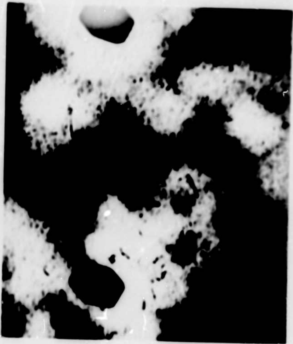
Figure 4. Transmission Electron Micrograph of M-W Composite Showing Transverse Cross Section of Several W Fibers. X about 25,000.
