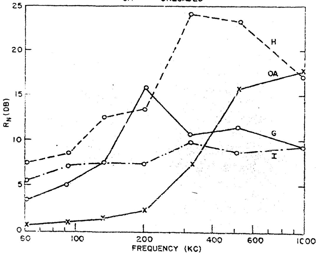
lead powder, i.e., 500 parts of butyl rubber. The first two materials were selected on the basis of the high sustained values of absorption over the frequency range from 60 to 1000 cps. The heavily-loaded lead material was selected in order to study the effect of extreme loading.
