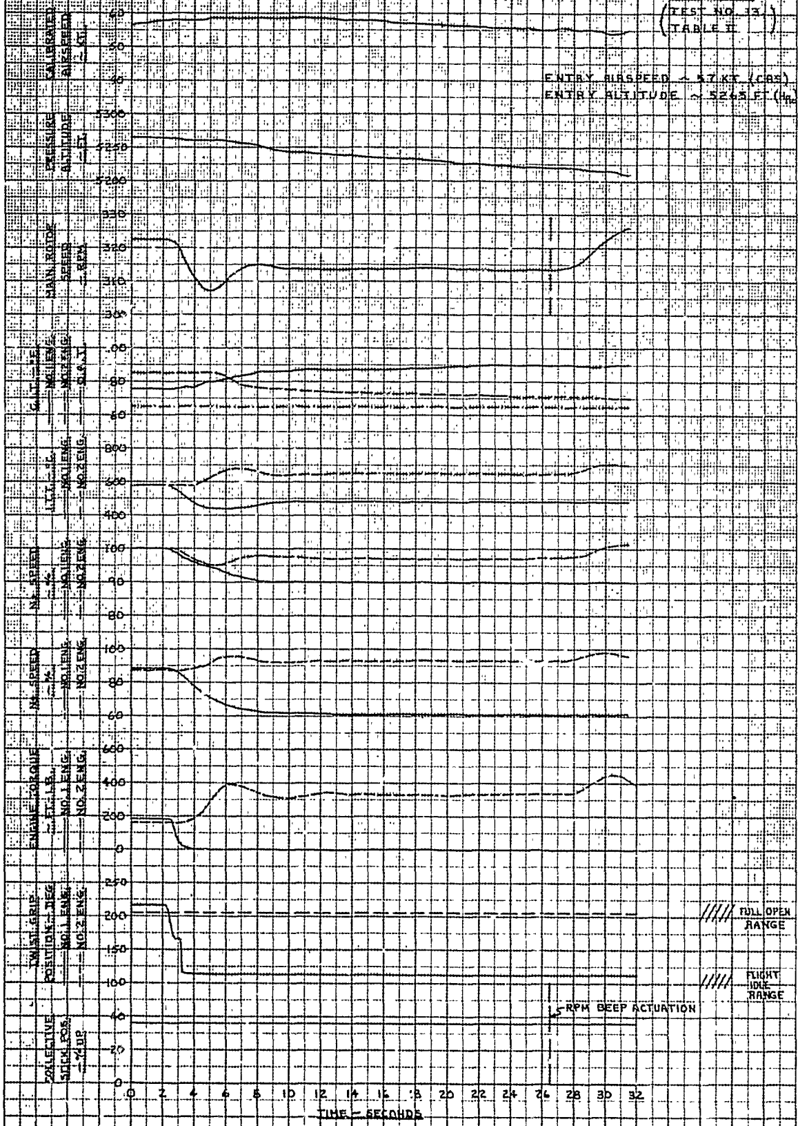
Fig. 24 TIME HISTORY OF POWER TRANSIENT - SINGLE ENGINE THROTTLE CHOP
