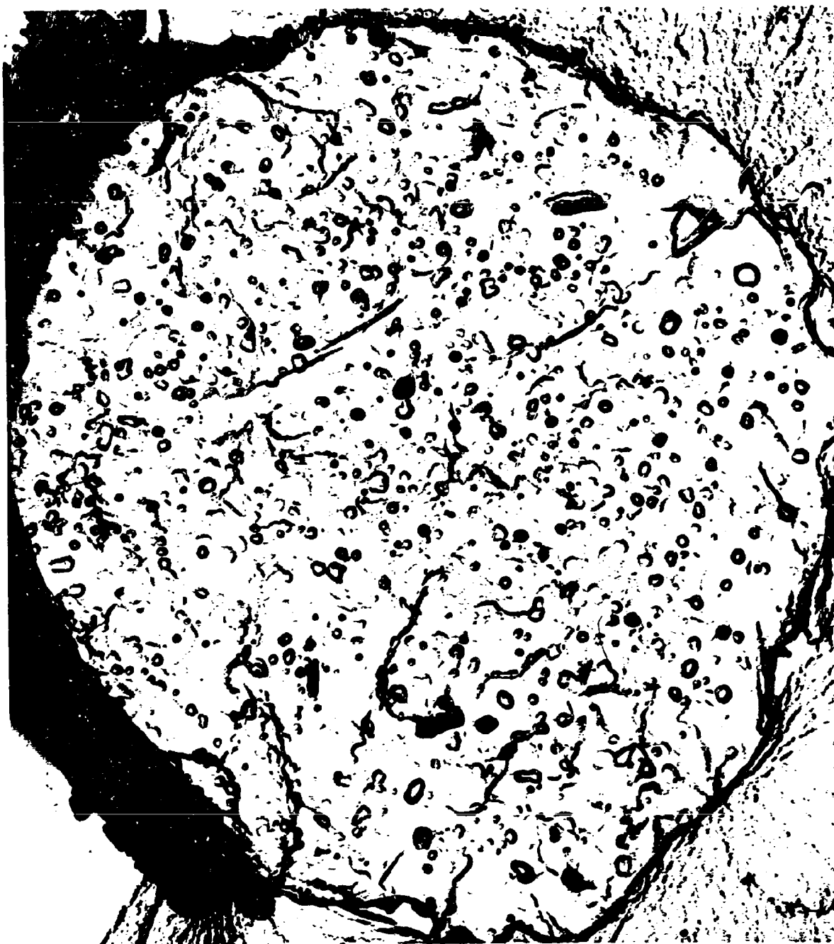
FIGURE 27. SAMPLE NO. M-103-4 CHEMISTRY: 73% \text{Al}_2\text{O}_3 , 27% \text{SiO}_2 CRYSTAL: Major, Mullite FIRING TEMPERATURE: 2300 F TENSILE STRENGTH: 112,000 psi - MODULUS: 20.7 \times 10^6 psi
