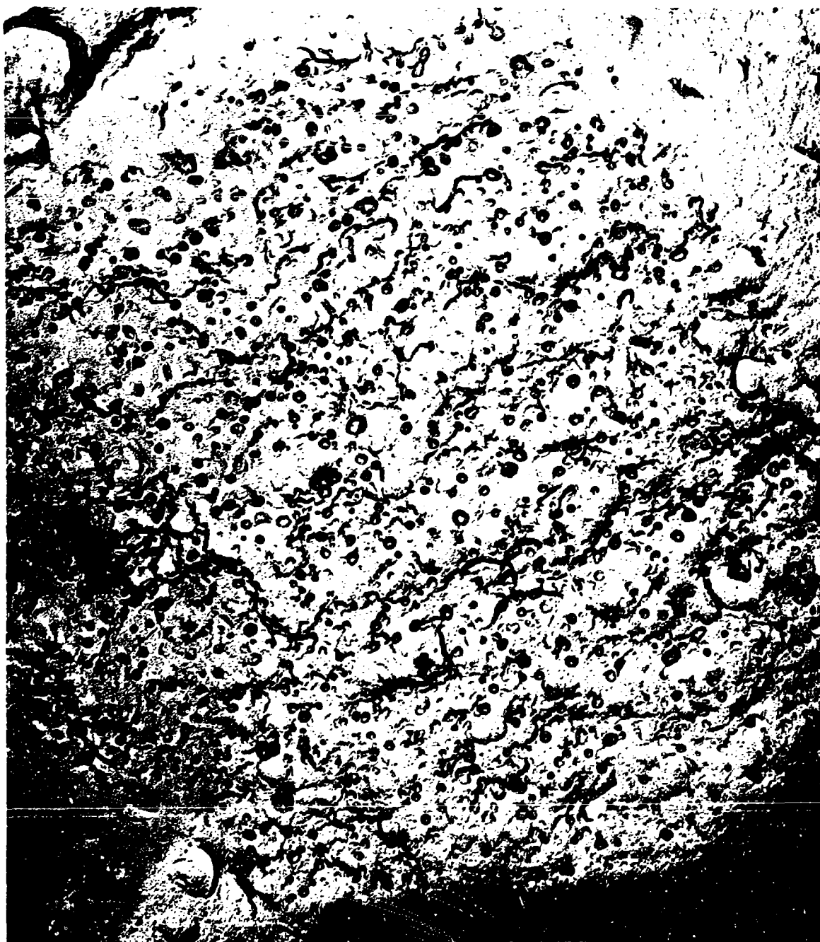
FIGURE 21. SAMPLE NO. B-313-25 X30,000 CHEMISTRY: 75% \text{Al}_2\text{O}_3 , 20% \text{SiO}_2 , 5% \text{B}_2\text{O}_3 CRYSTAL: Major, Millite FIRING TEMPERATURE: 2400 F TENSILE STRENGTH: 140,000 psi - MODULUS: 24.4 \times 10^6 psi
