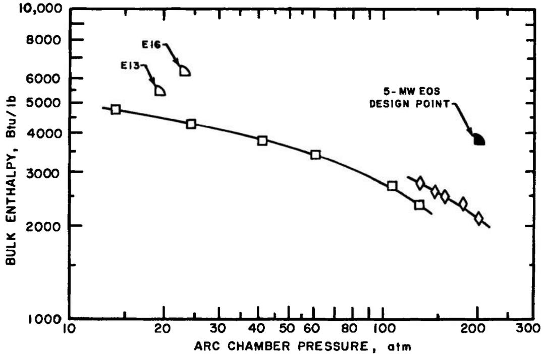
Fig. 17 Performance Comparison of 5-MW EOS and Linde N4000 Heaters
