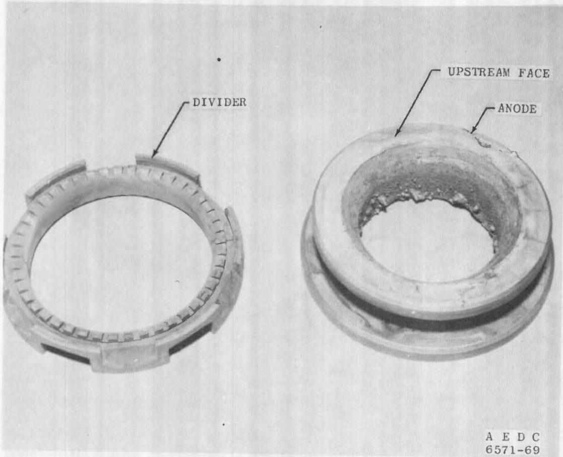
d. Anode and Its Cooling Flow Divider
