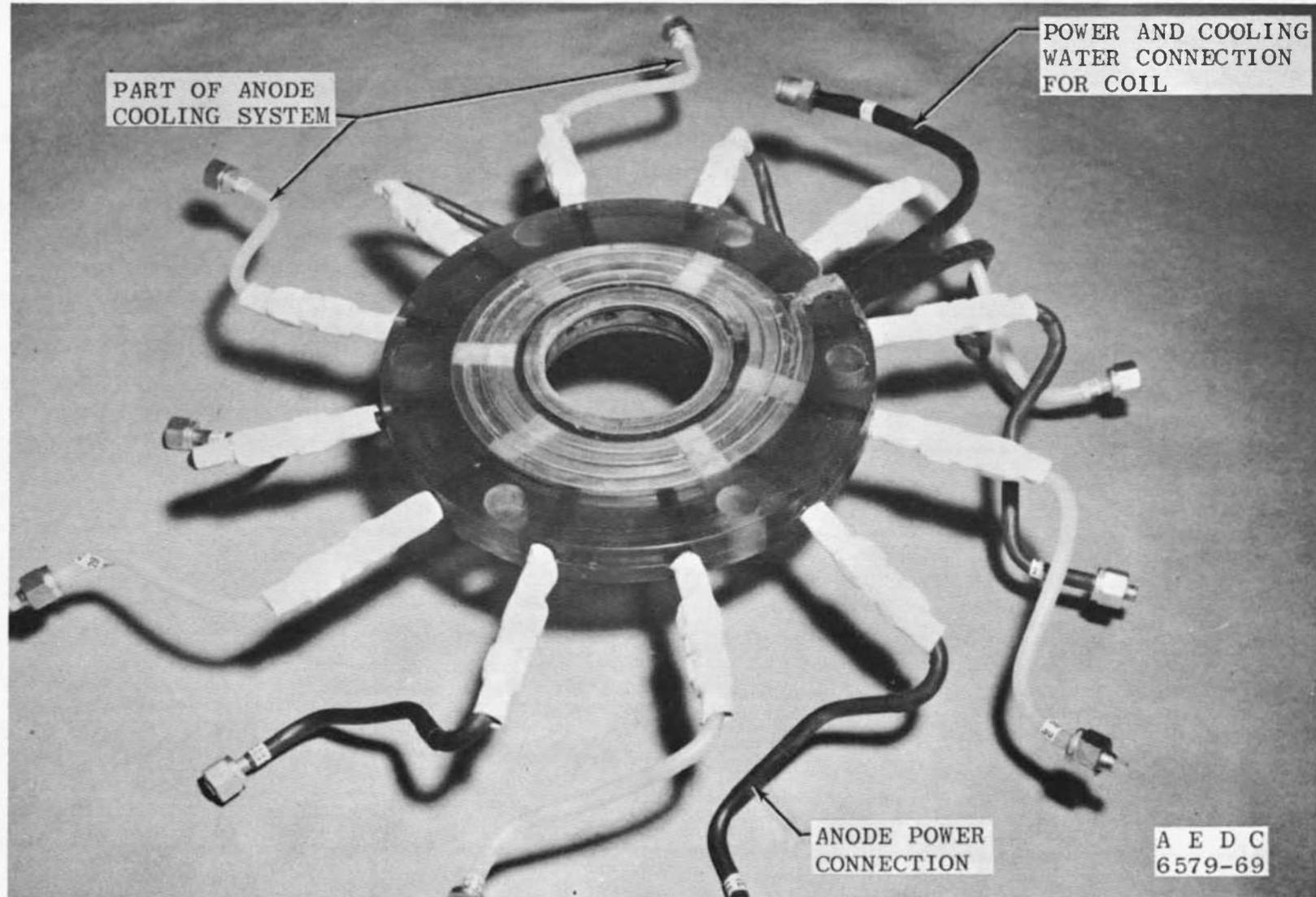
Fig. 4 Spin Coil Used on 1-MW Heaters
