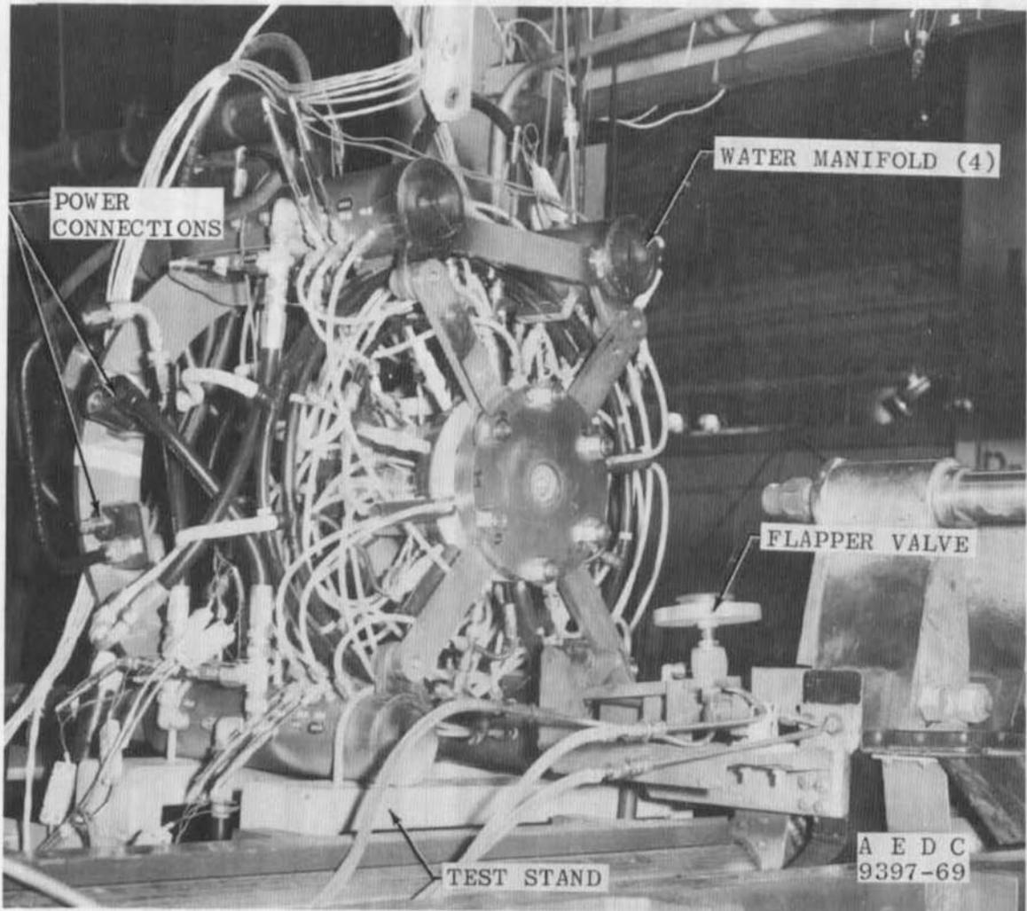
Fig. 5 1-MW Air Heater Mounted on Test Stand
