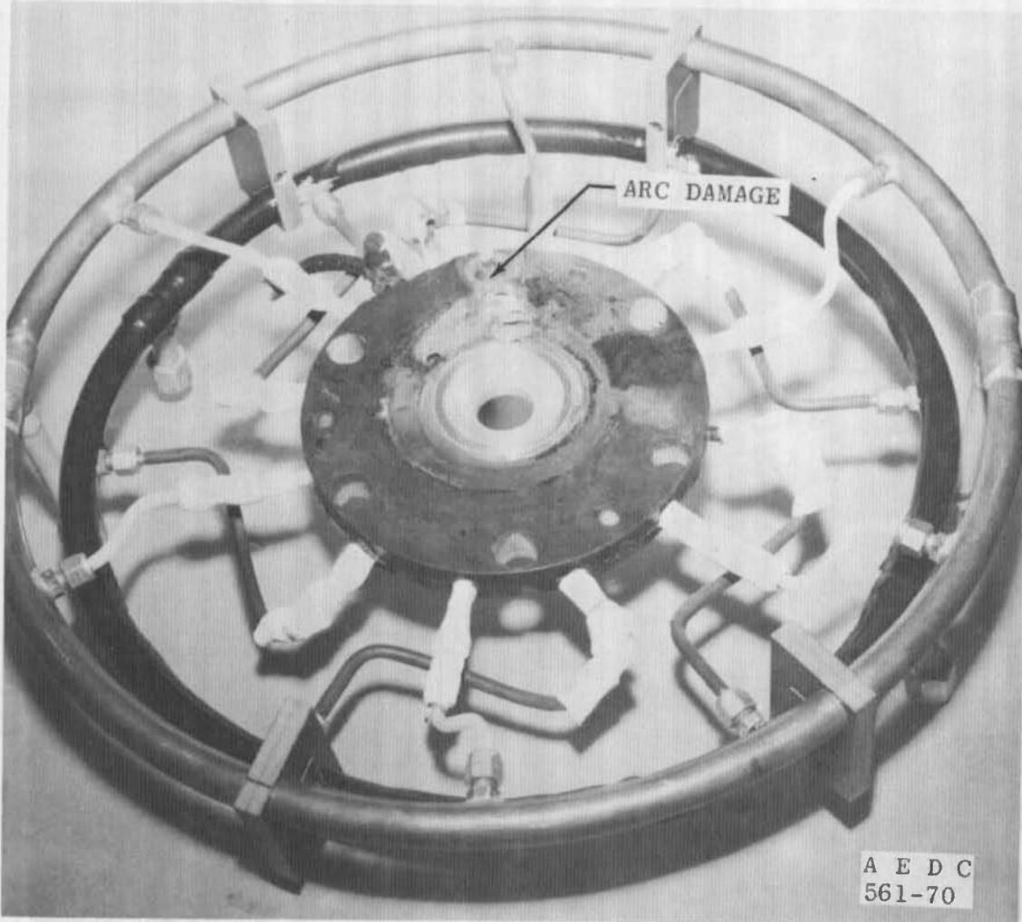
c. Downstream Face, Anode Spin Coil
