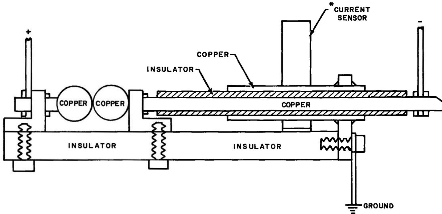
SYSTEM DESIGN CAPACITY = 750 amps FOR 0.5 sec DURATION
