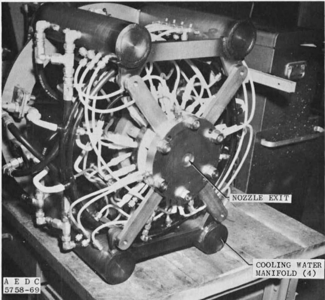
b. Assembled Heater, Discharge End View
