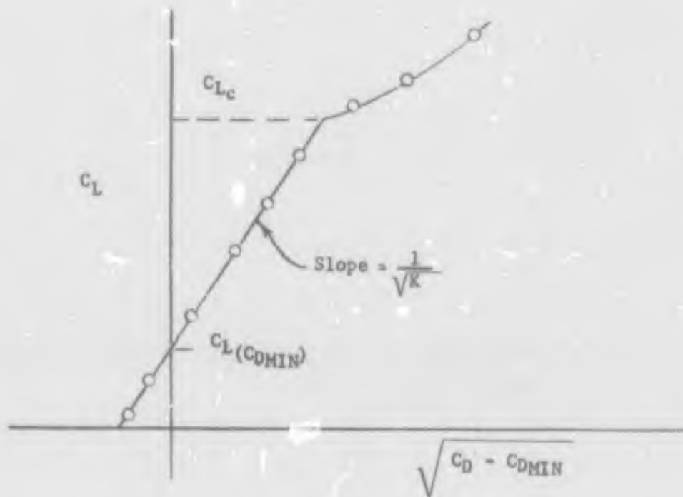
Figure 37 SQUARE ROOT PLOT FOR DRAG-DUE-TO-LIFT ANALYSIS OF CAMBERED CONFIGURATIONS
