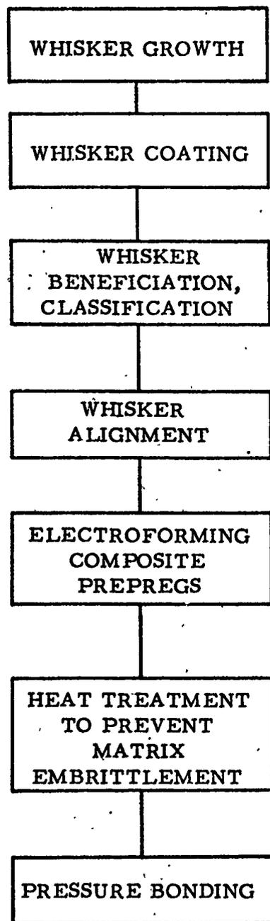
Figure 3. Process steps in the preparation of Ni-Al<sub>2</sub>O<sub>3</sub> whisker composites by EP/PB technique
