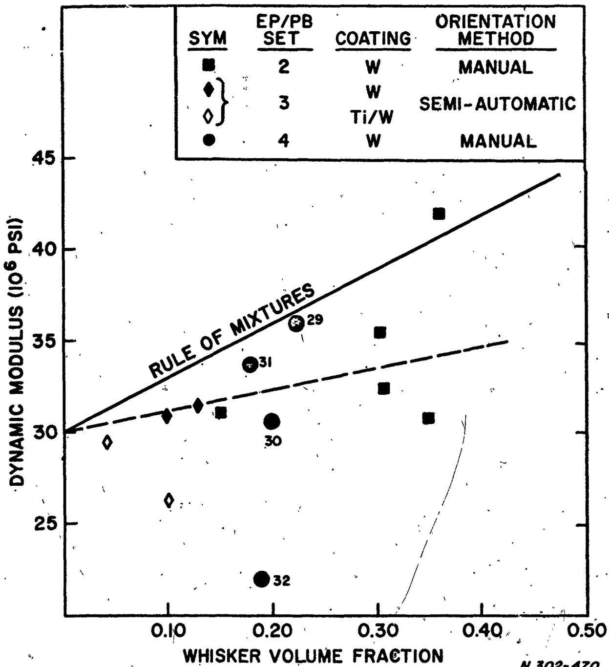
Figure 10. Relation between dynamic modulus and fiber volume fraction
