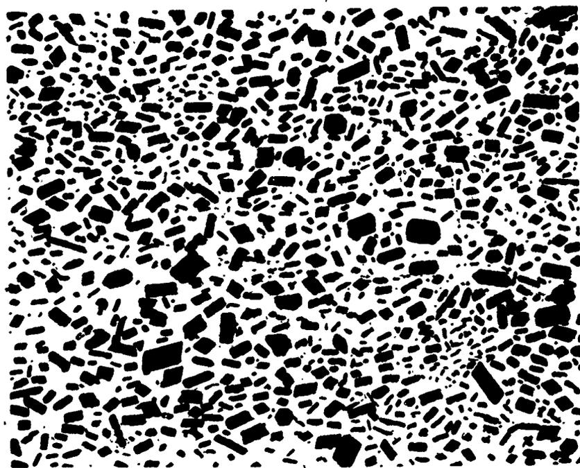
Figure 8. Microstructure of transverse cross-section of Ni - 23 v/o%  $\text{Al}_2\text{O}_3$  whisker composite (#29) prepared by the EP/PB process.
