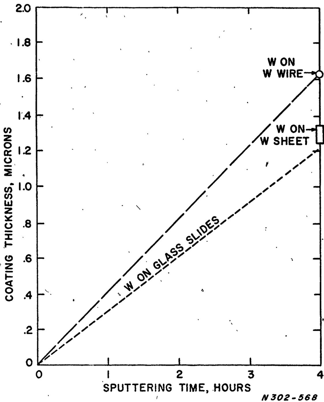
Figure 1. Coating thickness determination as a function of sputtering time.
