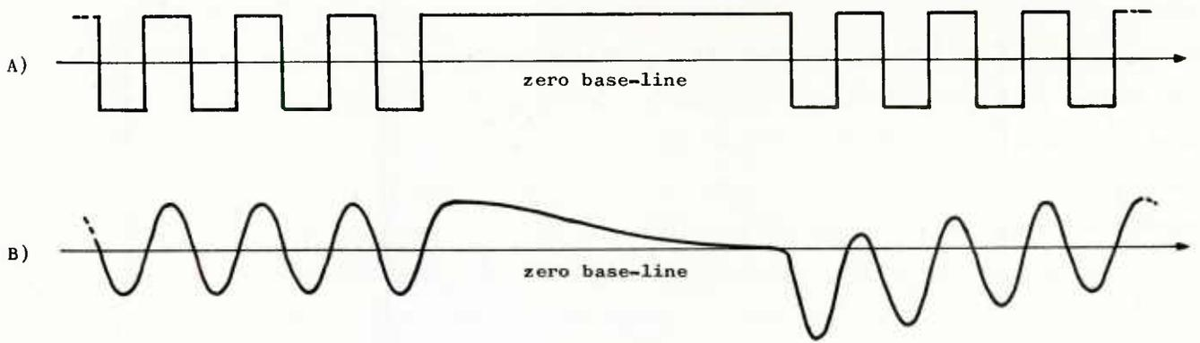
TRACE A - NRZ-coded recording signal
