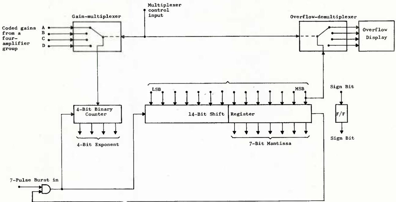
FIG. 4 FLOATING-POINT CONVERTER
