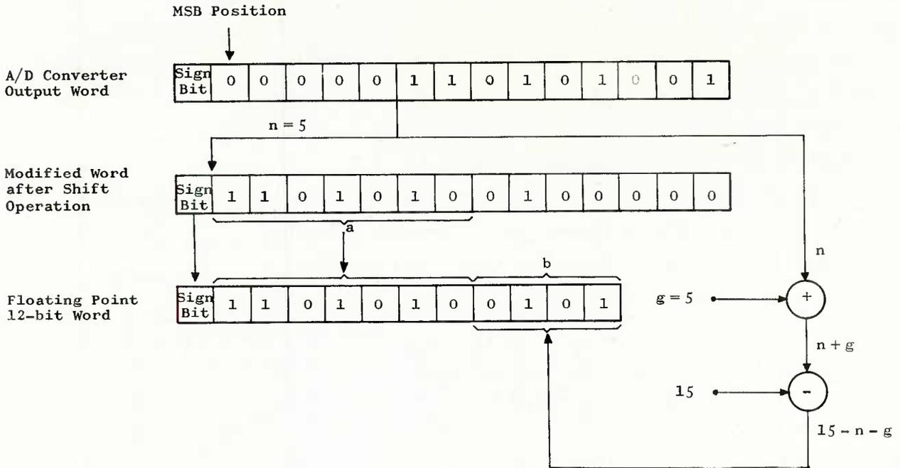
FIG. 3 EXAMPLE OF FLOATING-POINT CONVERSION (GAIN: 30 dB)
