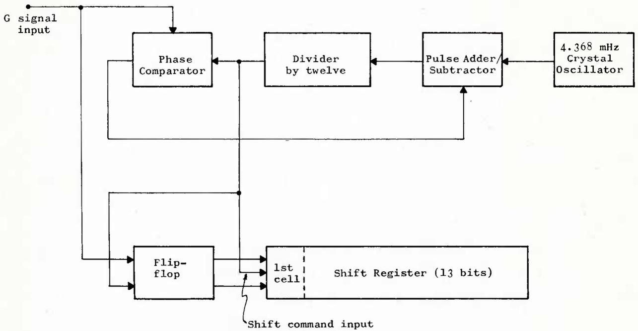
FIG. 17 SIMPLIFIED BLOCK DIAGRAM OF BIT SYNCHRONIZER
