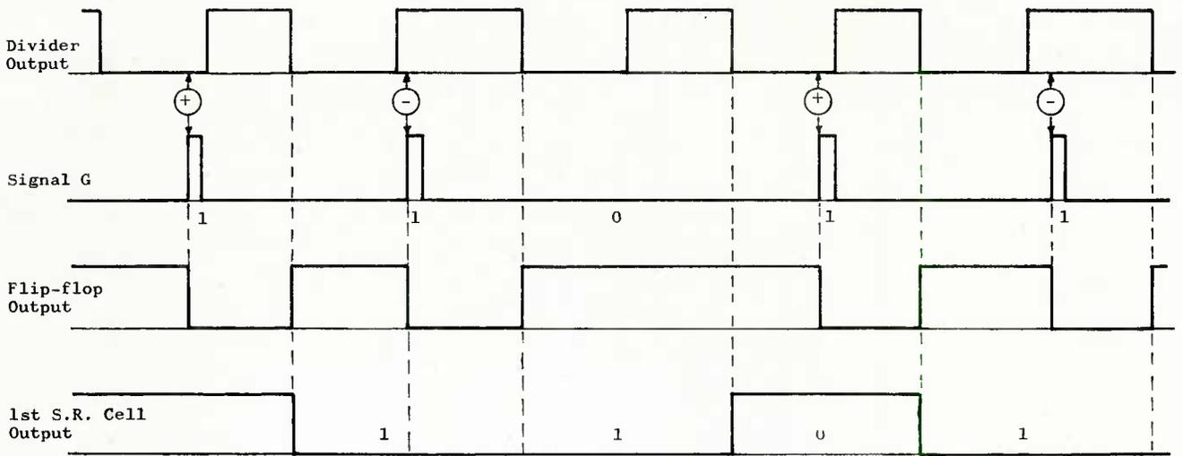
Rate fluctuations have been exaggerated for clarity:  $\oplus$  indicates that one pulse is added at the divider input;  $\ominus$  indicates that one pulse is subtracted from it.
