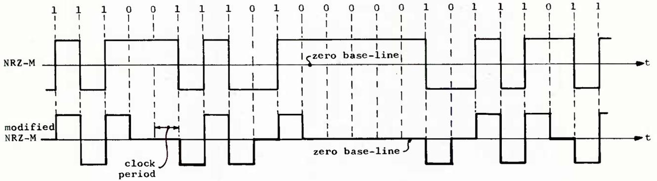
FIG. 11 EXAMPLE OF MODIFIED NRZ-M ENCODING FORMAT
