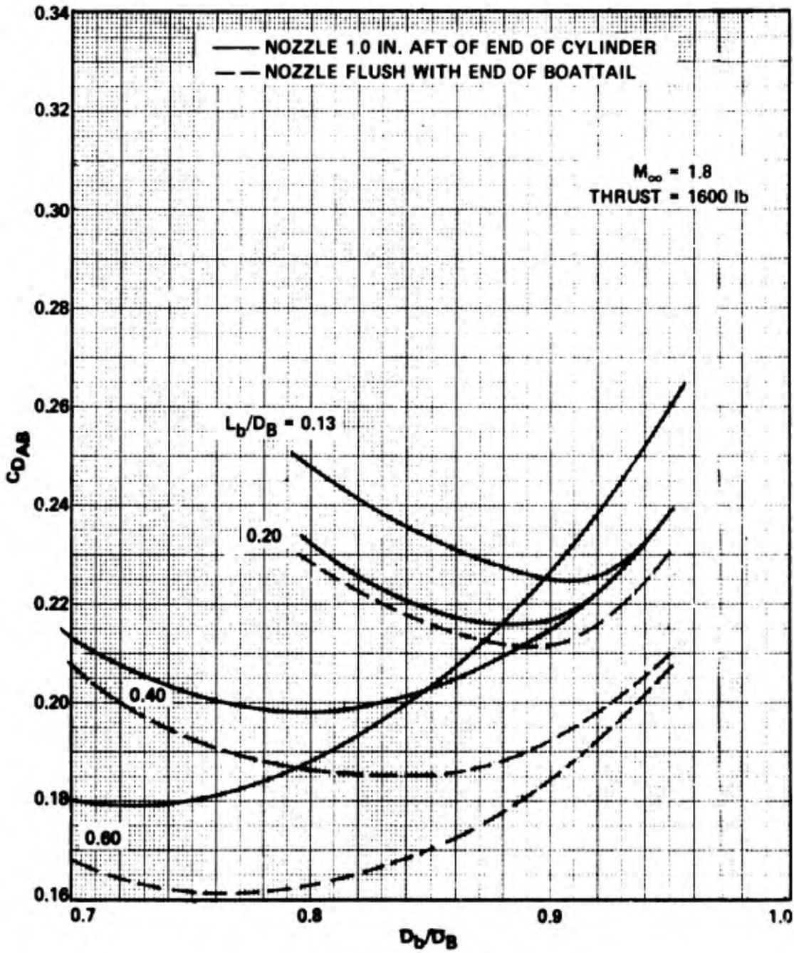
Fig. 11. Afterbody Drag for Parametric Variations
