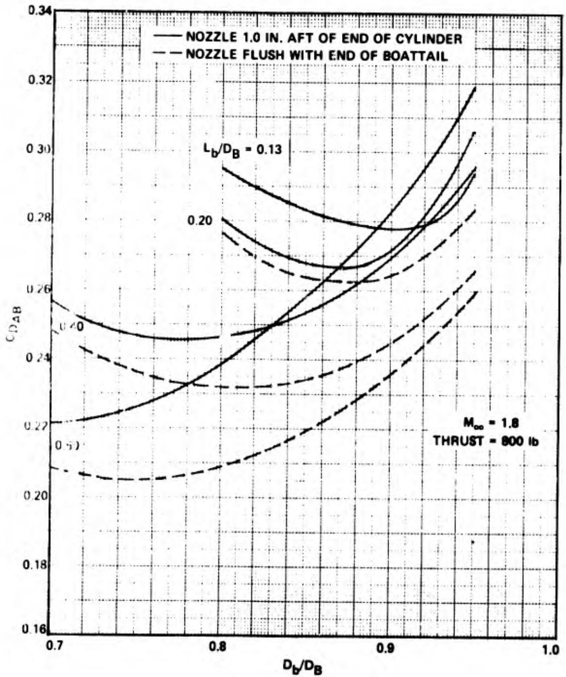
Fig. 10. Afterbody Drag for Parametric Variations
