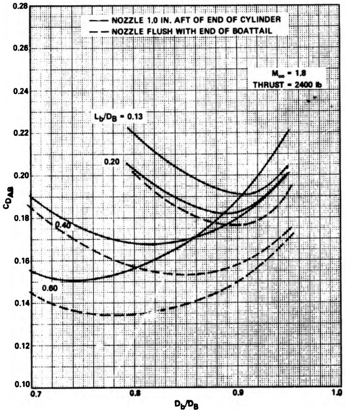
Fig. 12. Afterbody Drag for Parametric Variations
