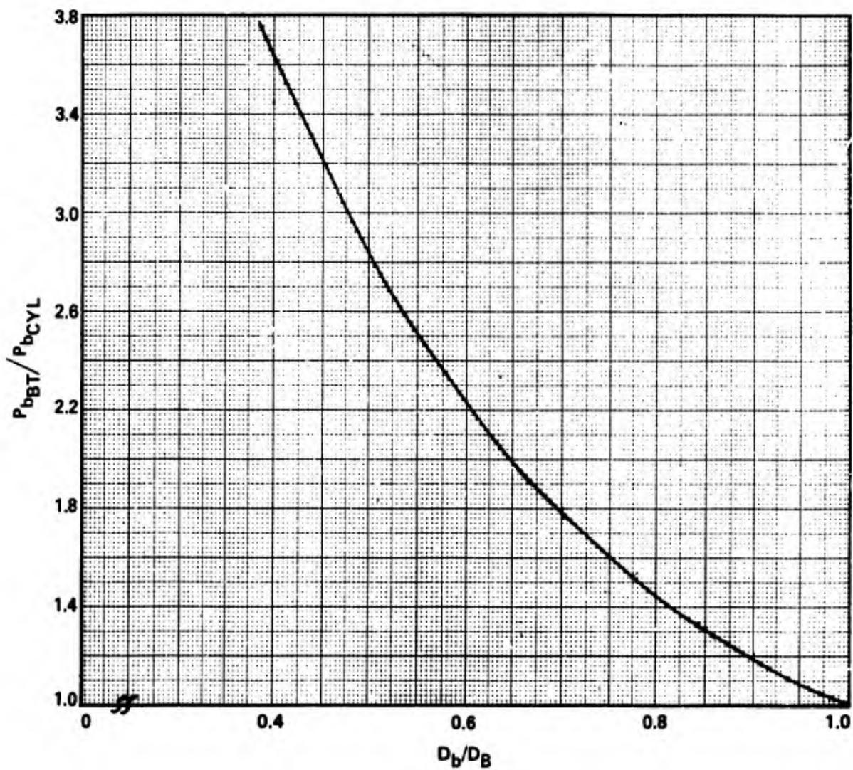
Fig. 3. Ratio of Base Pressure on a Boattail to Base Pressure on a Cylinder
