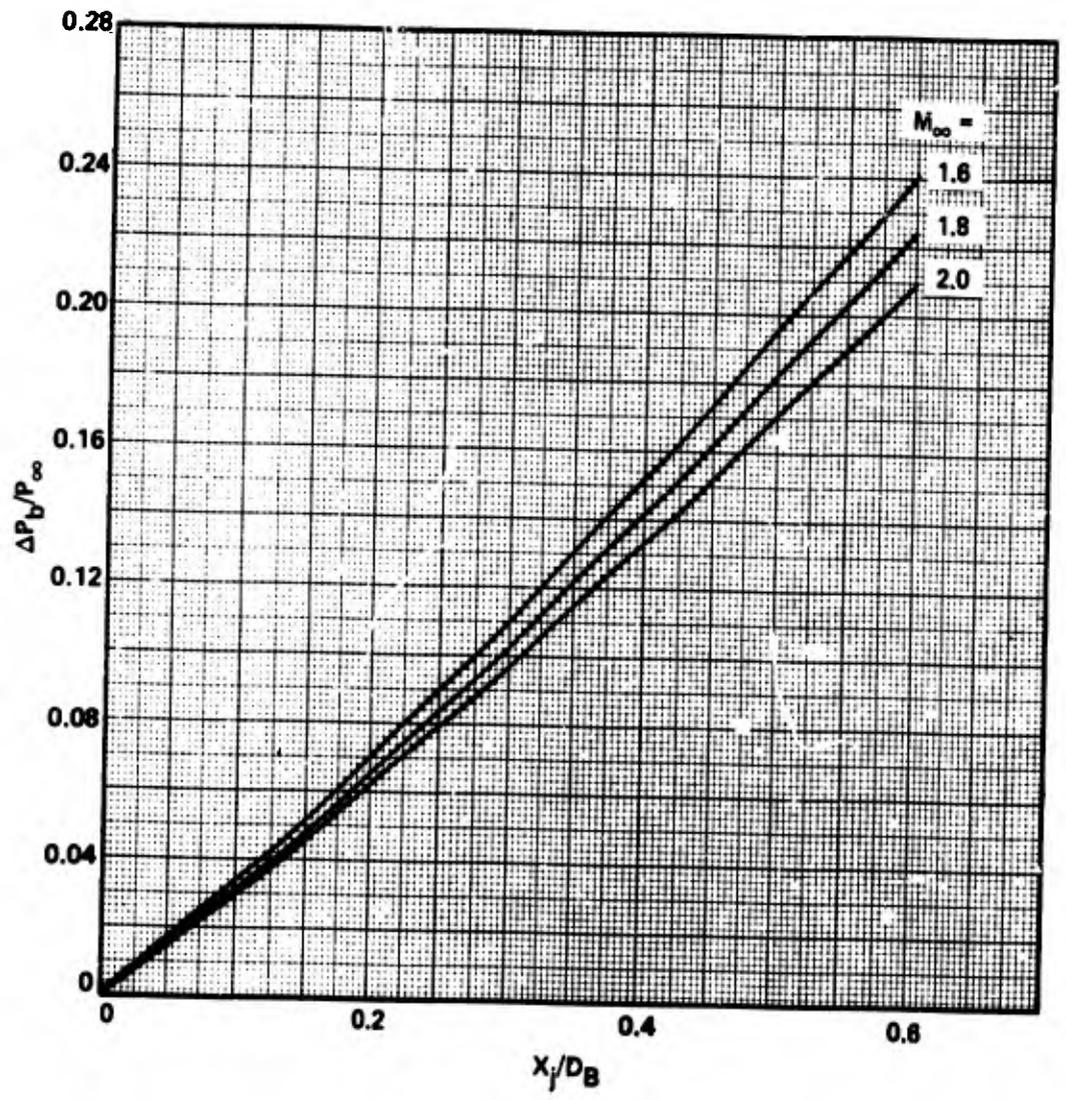
Fig. 4. Incremental Change in Base Pressure Due to Nozzle Aft of Base
