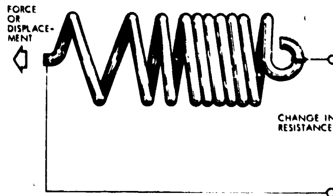
Figure 5.15.5.3. Variable Pitch Spring Linear Displacement Transducer
