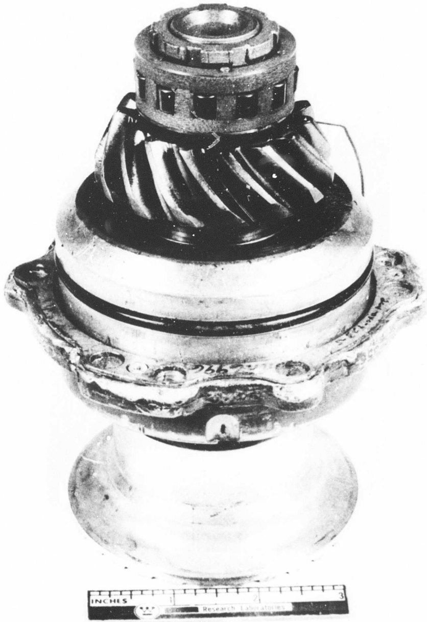
Figure 20. Pinion Assembly After Polyimide Retainer and Coated Idler Gear Operation, Series 4.
