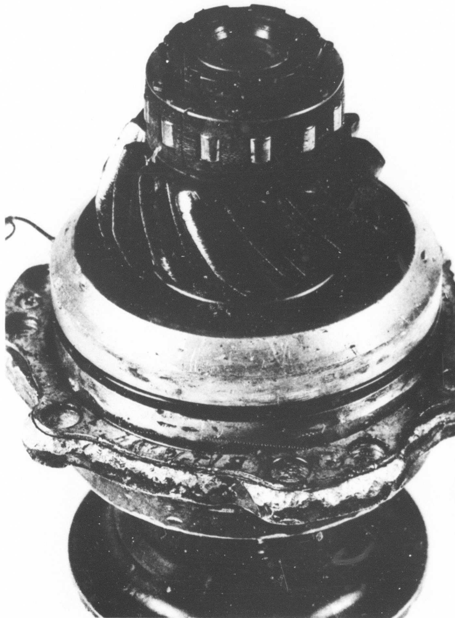
Figure 33. Pinion Assembly After Filled Polyimide "A" Retainer and Idler Gear Test, Series 1A.
