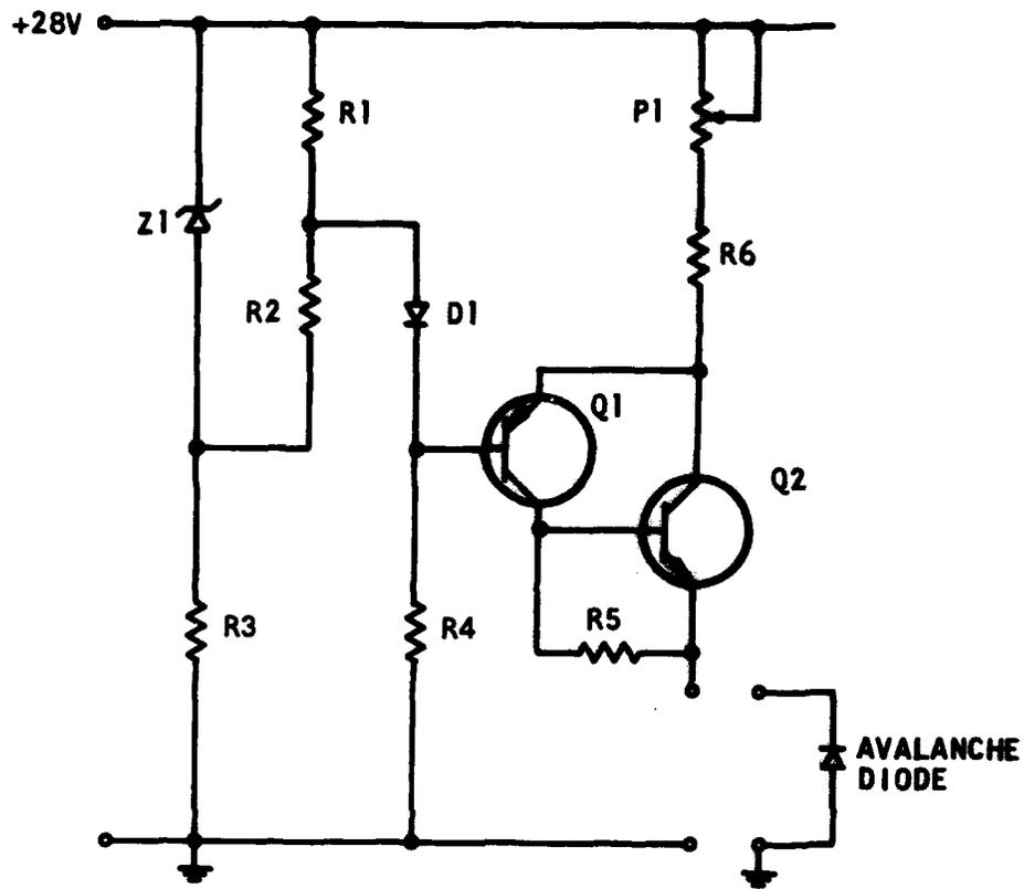
FIGURE 2 CONSTANT CURRENT REGULATOR TYPE II
