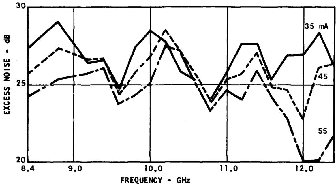
FIGURE 12 NOISE POWER VS FREQUENCY SOURCE NO. 4
