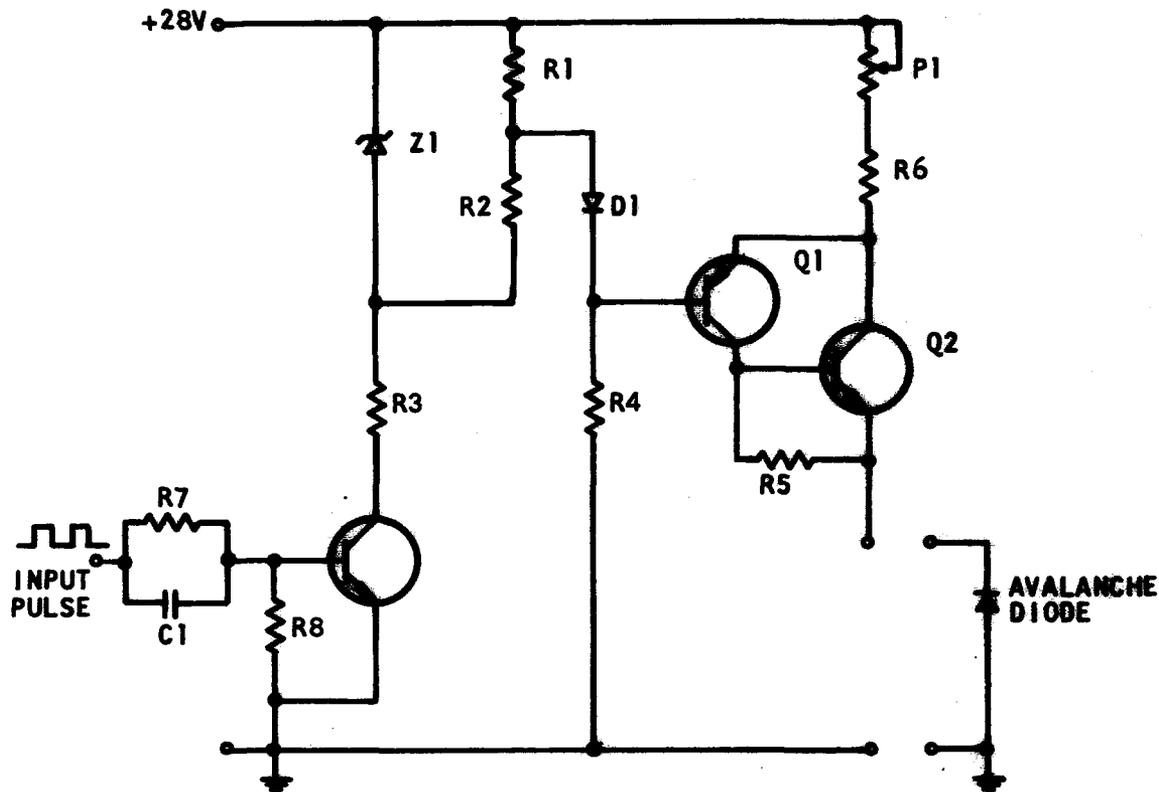
FIGURE 4 CONSTANT CURRENT REGULATOR TYPE II WITH PULSING CIRCUIT
