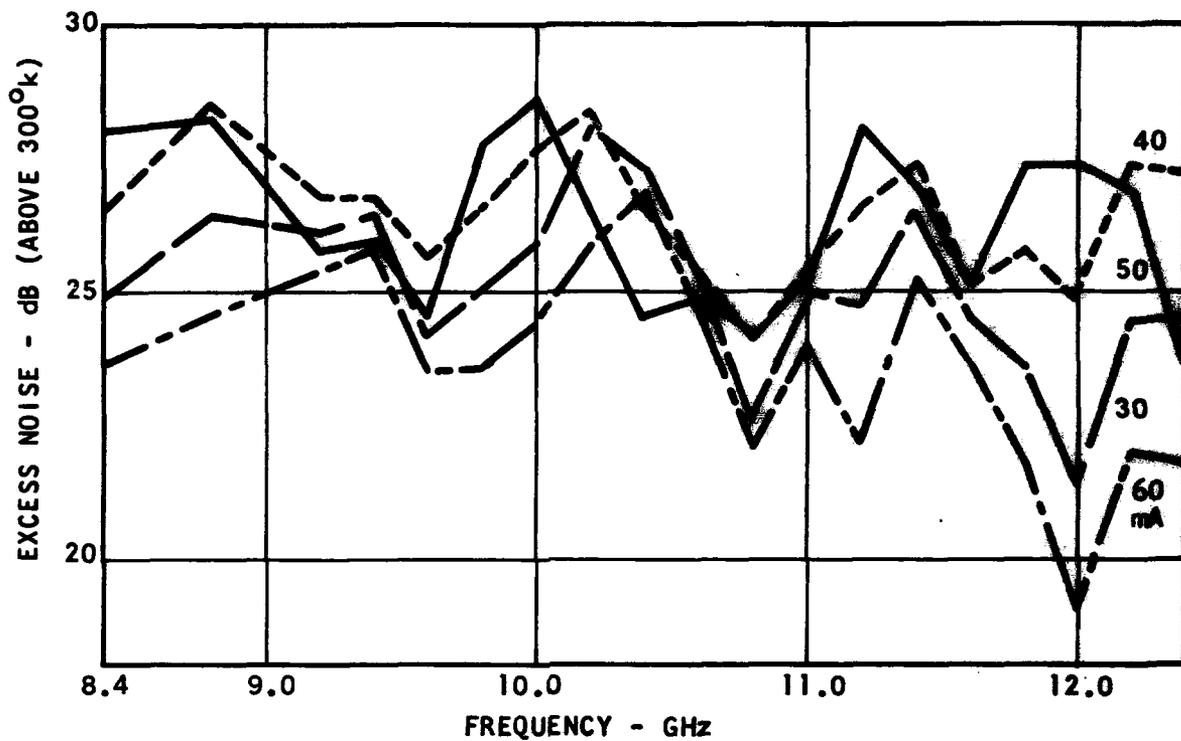
FIGURE 11 NOISE POWER VS FREQUENCY SOURCE NO. 4
