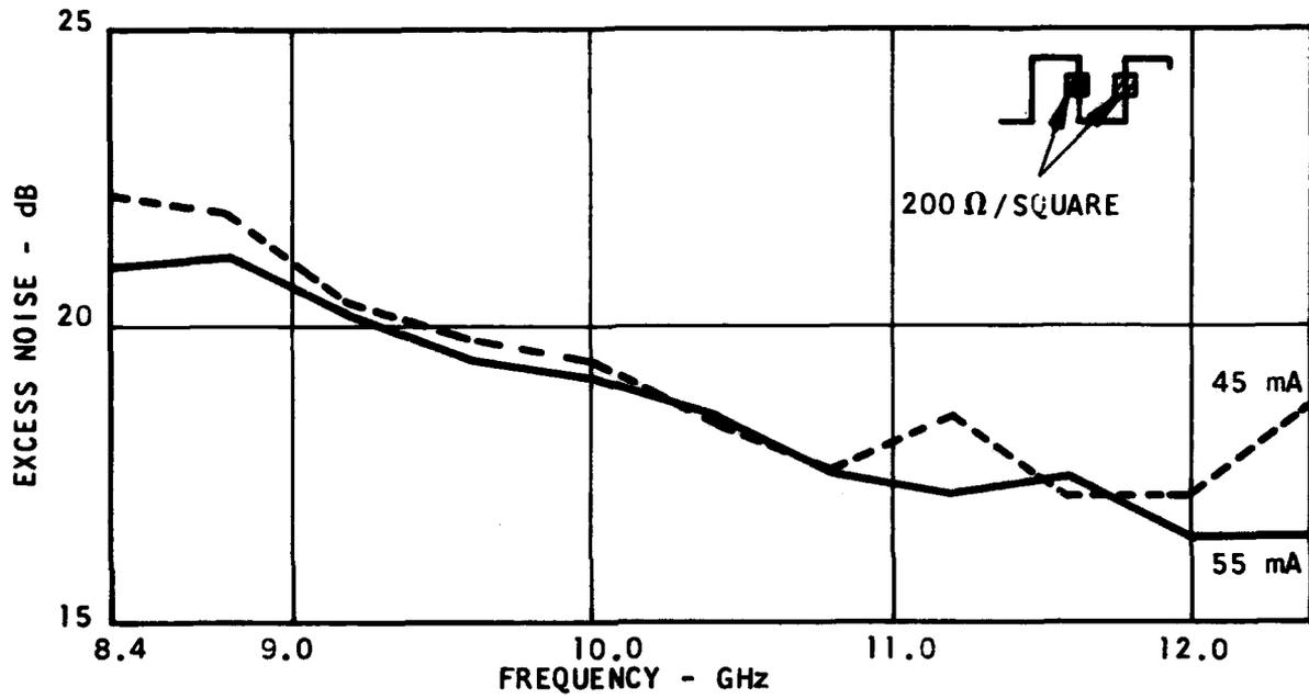
FIGURE 18 NOISE POWER VS FREQUENCY EFFECT OF TWO 200  $\Omega$  / SQUARE LOADS
