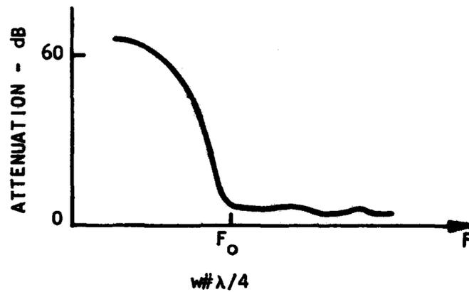
FIGURE 20 FILTERING EFFECT BY AN OVERSIZED CERAMIC SUBSTRATE
