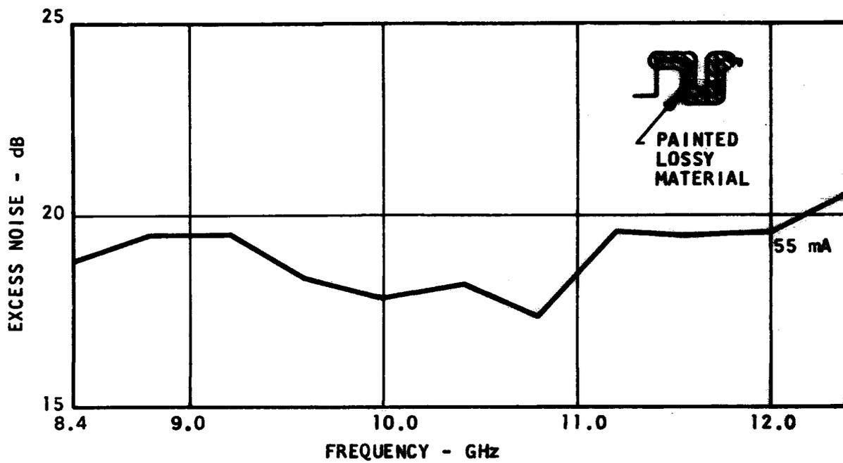
FIGURE 19 NOISE POWER VS FREQUENCY EFFECT OF A PAINTED LOSSY MATERIAL
