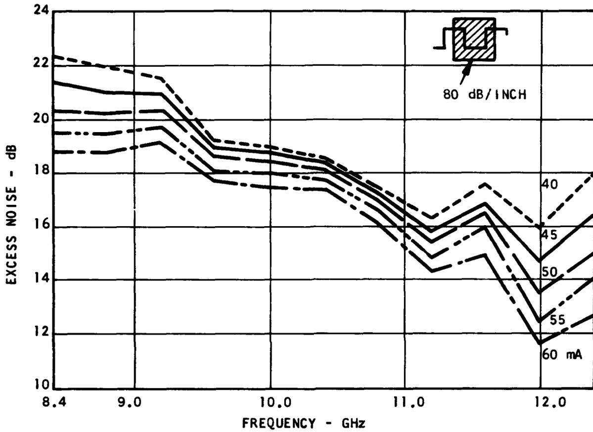
FIGURE 16 NOISE POWER VS FREQUENCY EFFECT OF AN 80 dB/INCH LOAD
