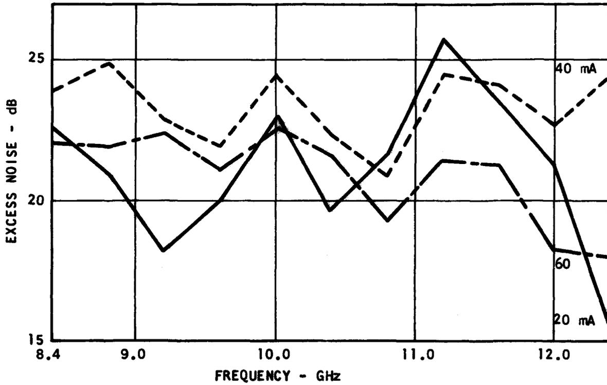
FIGURE 14 NOISE POWER VS FREQUENCY SOURCE NO. 1
