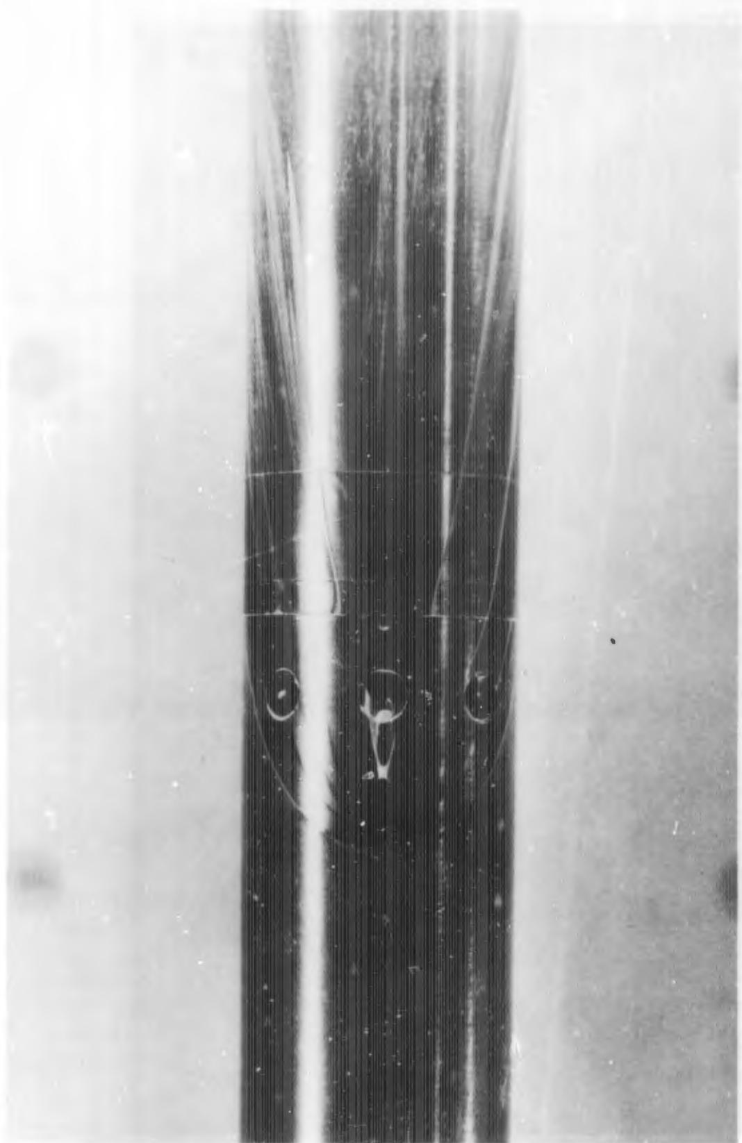
FIGURE C-4f. REACTION JET FOR  $B_1C_1X_3$  WITH  $\alpha = -5$  DEGREES;  $P_{01}/P_\infty = 40$
