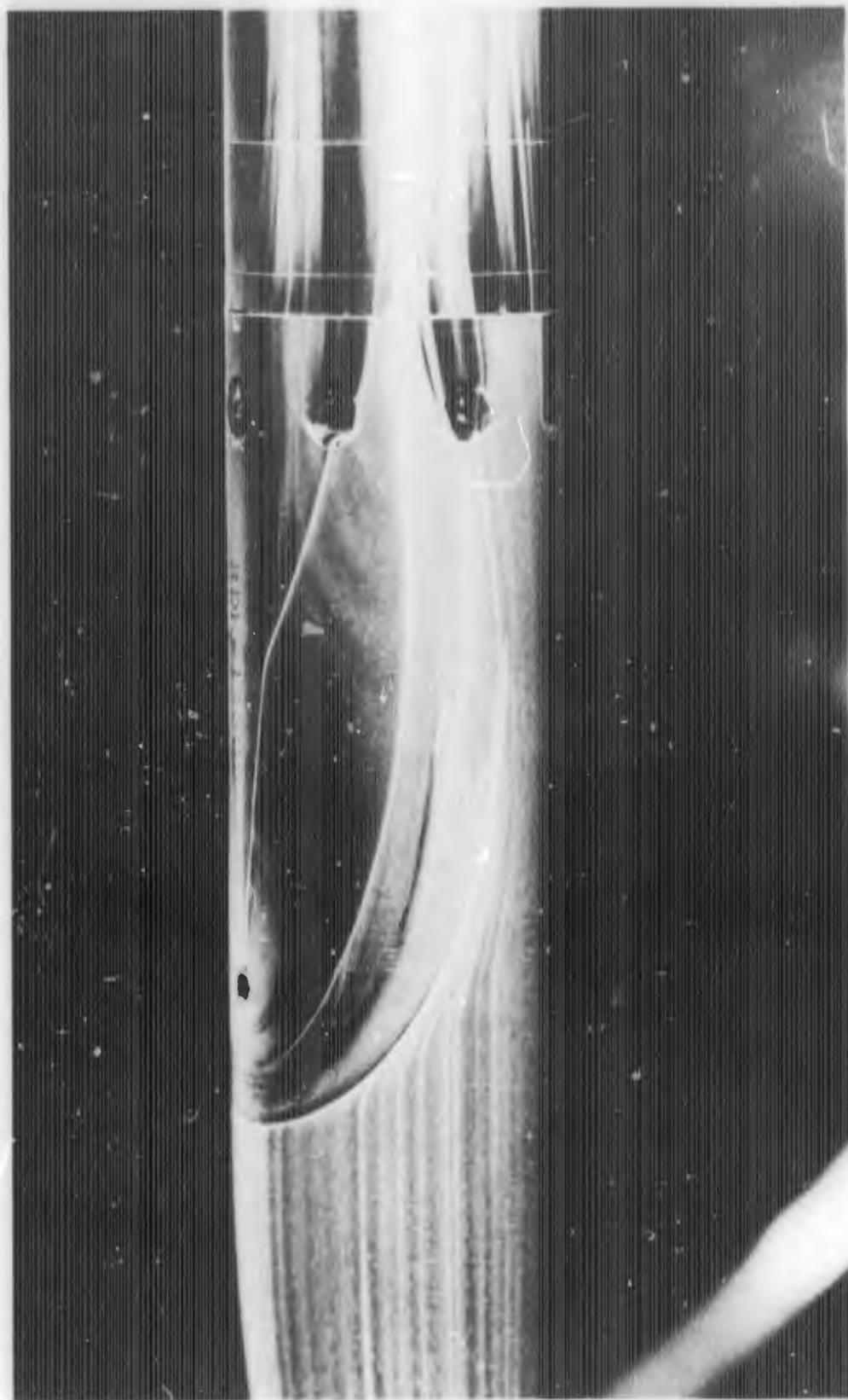
FIGURE B-1f. REACTION JET FOR  $B_1C_1X_2$  WITH  $\alpha = 0$  DEGREES;  $P_{0j}/P_\infty = 100$
