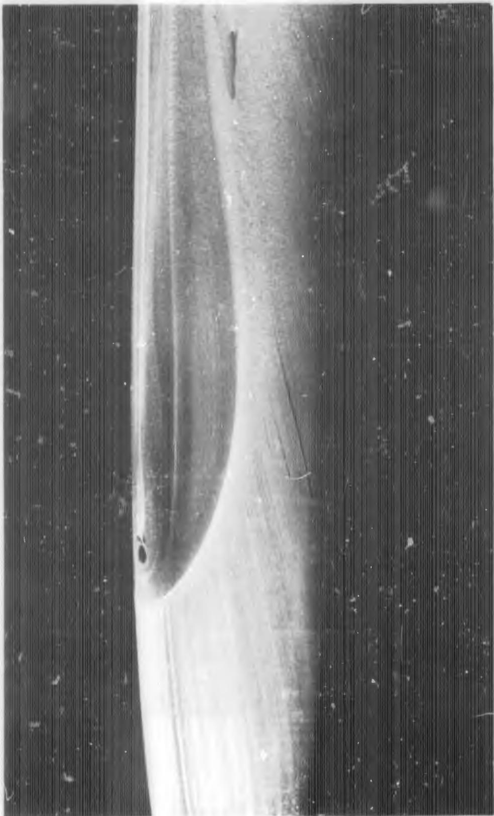
FIGURE E-5b. REACTION JET FOR  $B_1C_1X_1$  WITH  $\alpha = 5$  DEGREES;  $P_{0j}/P_\infty = 100$
