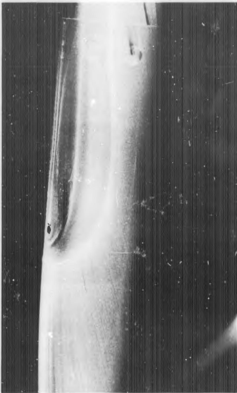
FIGURE E-10a. REACTION JET FOR  $B_1C_1X_2$  WITH  $\alpha = 5$  DEGREES;  $P_{0j}/P_\infty = 40$
