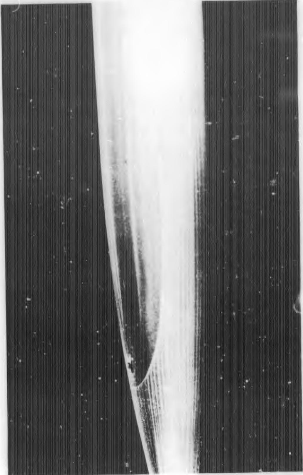
FIGURE E-1d. REACTION JET FOR  $B_1C_1X_0$  WITH  $\alpha = 0$  DEGREES;  $P_{0j}/P_\infty = 40$
