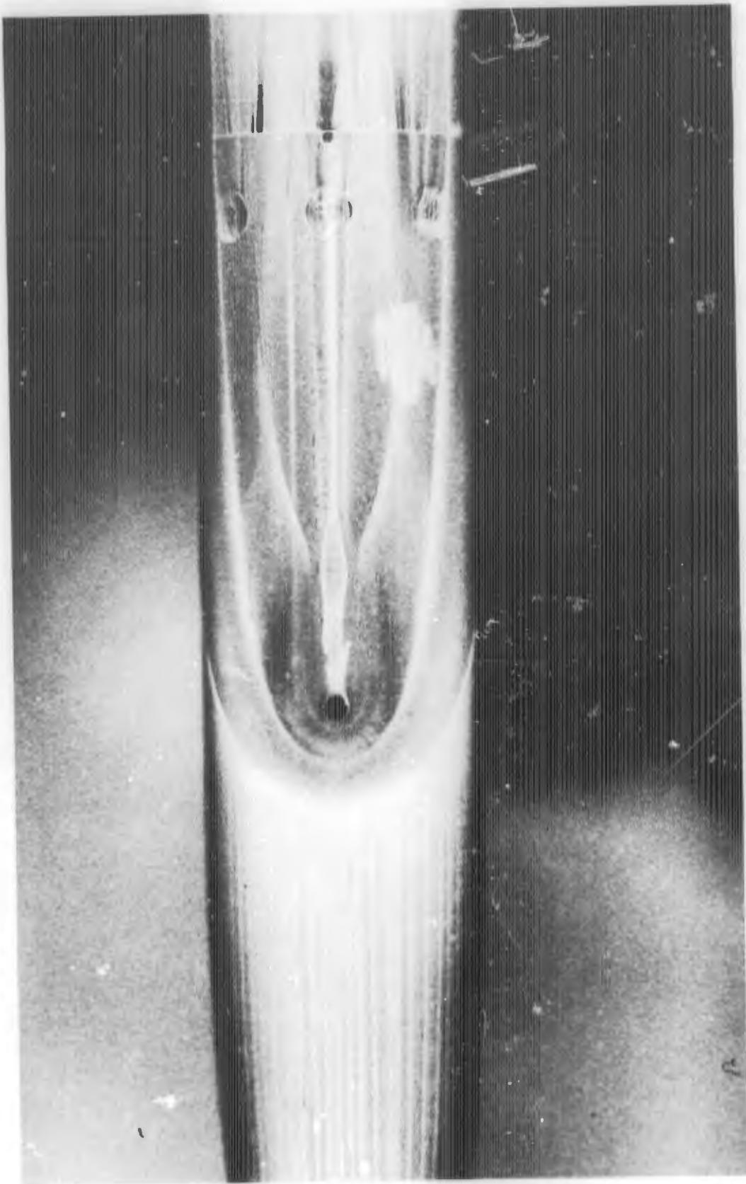
FIGURE E-9j. REACTION JET FOR  $B_1 C X_2$  WITH  $\alpha = 0$  DEGREES;  $P_{obj}/P_\infty = 100$
