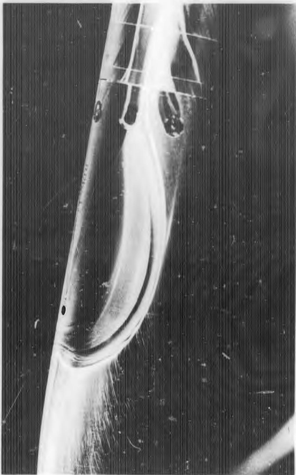
FIGURE B-3c. REACTION JET FOR  $B_1C_1X_2$  WITH  $\alpha = 10$  DEGREES;  $P_{obj}/P_\infty = 100$
