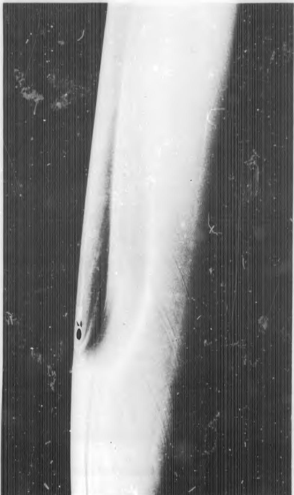
FIGURE E-6b. REACTION JET FOR  $B_1C_1X_1$  WITH  $\alpha = 10$  DEGREES;  $P_{obj}/P_\infty = 100$
