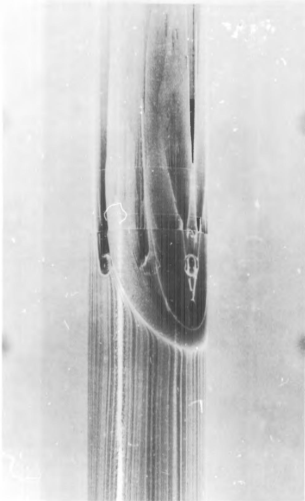
FIGURE D-6f. REACTION JET FOR  $B_1C_1X_3$  WITH  $\alpha = 0$  DEGREES;  $P_{0j}/P_\infty = 100$
