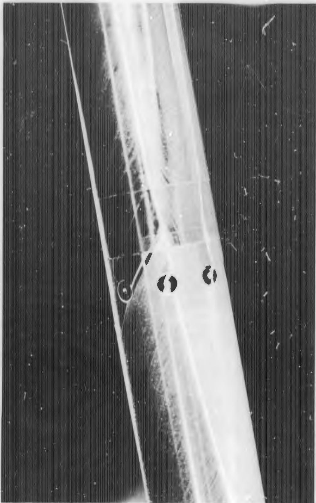
FIGURE C-5d. REACTION JET FOR  $B_1C_1X_3$  WITH  $\alpha = -10$  DEGREES;  $P_{0j}/P_\infty = 10$
