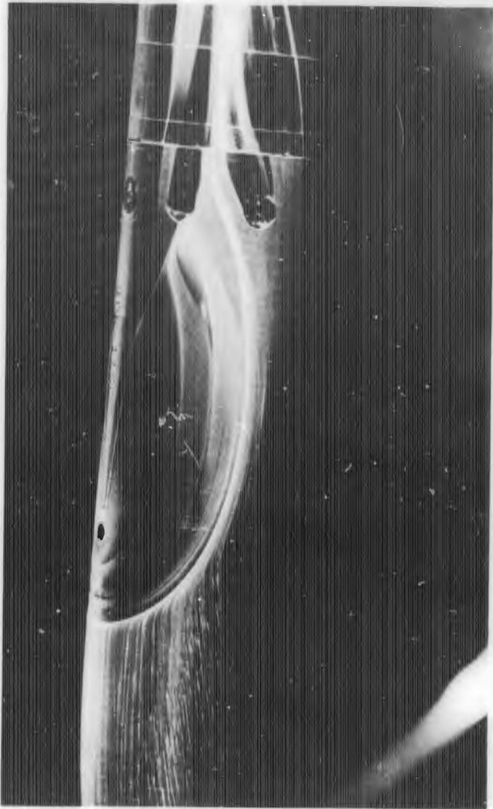
FIGURE B-2c. REACTION JET FOR  $B_1 C_1 X_2$  WITH  $\alpha = 5$  DEGREES;  $P_{0j}/P_\infty = 100$
