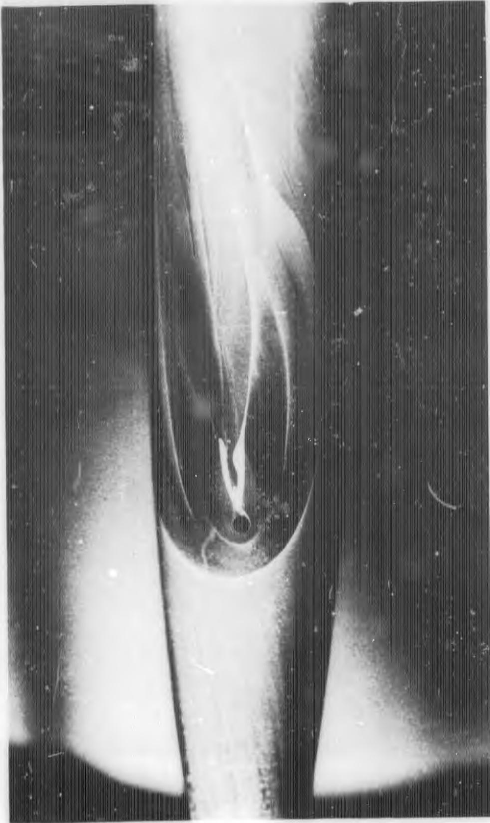
FIGURE E-5c. REACTION JET FOR  $B_1C_1X_1$  WITH  $\alpha = 5$  DEGREES;  $P_{obj}/P_\infty = 40$
