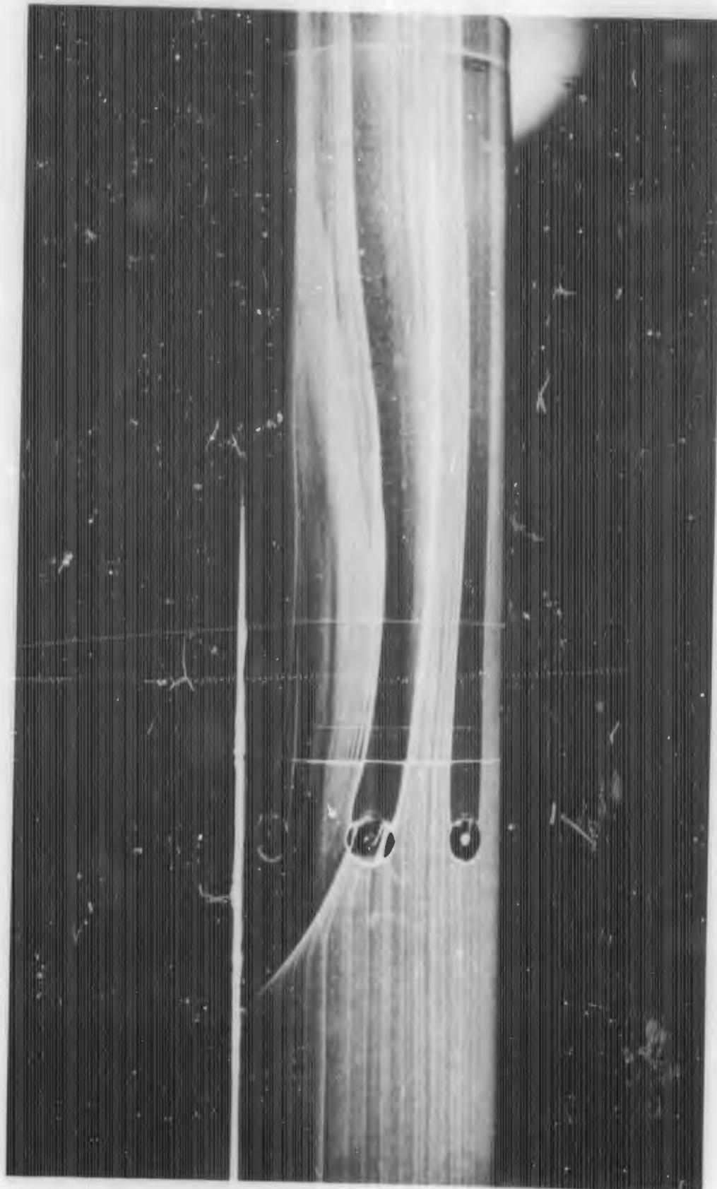
FIGURE C-1g. REACTION JET FOR B<sub>1</sub>C<sub>1</sub>X<sub>3</sub> WITH  $\alpha = 0$  DEGREES;  $P_{0j}/P_{\infty} = 100$
