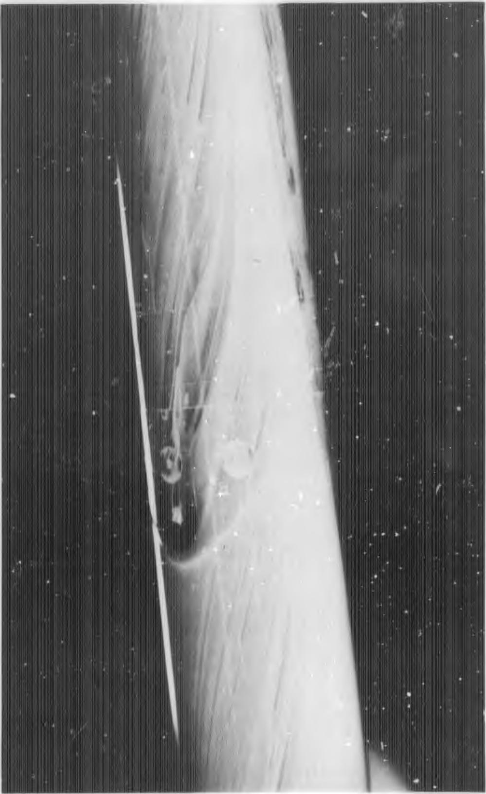
FIGURE D-9d. REACTION JET FOR B<sub>1</sub>C<sub>1</sub>X<sub>3</sub> WITH  $\alpha = -5$  DEGREES;  $P_{0j}/P_{\infty} = 10$
