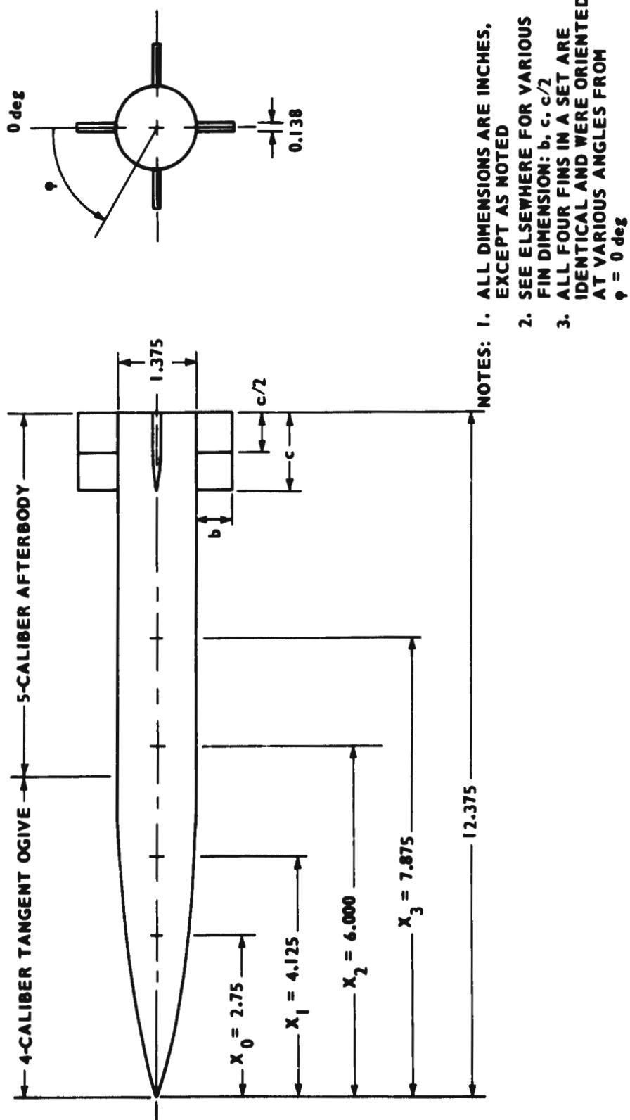
FIGURE 3. SCHEMATIC OF THE SUPPORTING RESEARCH REACTION JET TEST MODEL
