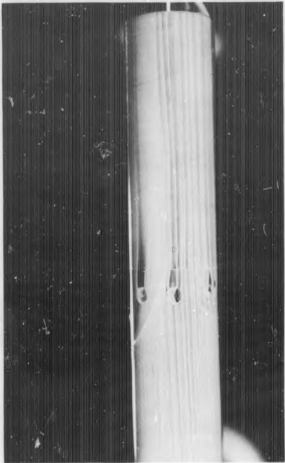
FIGURE D-1f. REACTION JET FOR B<sub>1</sub>C<sub>1</sub>X<sub>3</sub> WITH  $\alpha = 0$  DEGREES;  $P_{obj}/P_{\infty} = 40$
