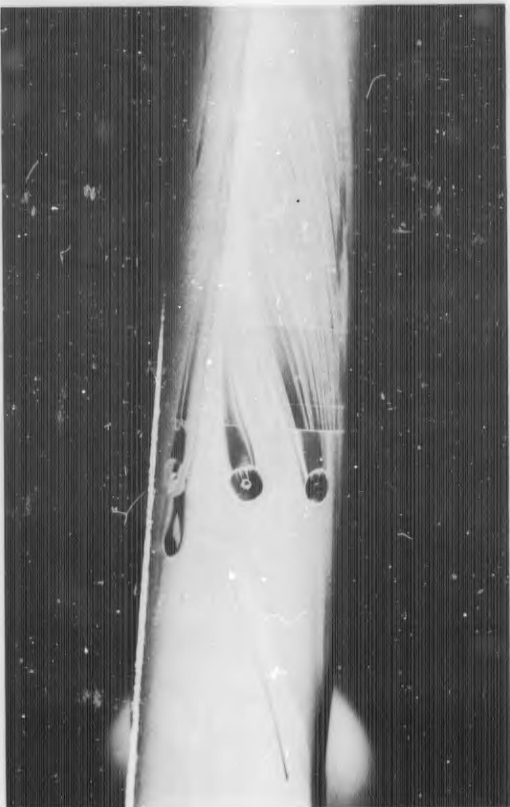
FIGURE D-7b. REACTION JET FOR  $B_1C_1X_3$  WITH  $\alpha = 5$  DEGREES;  $P_{0j}/P_\infty = 0$
