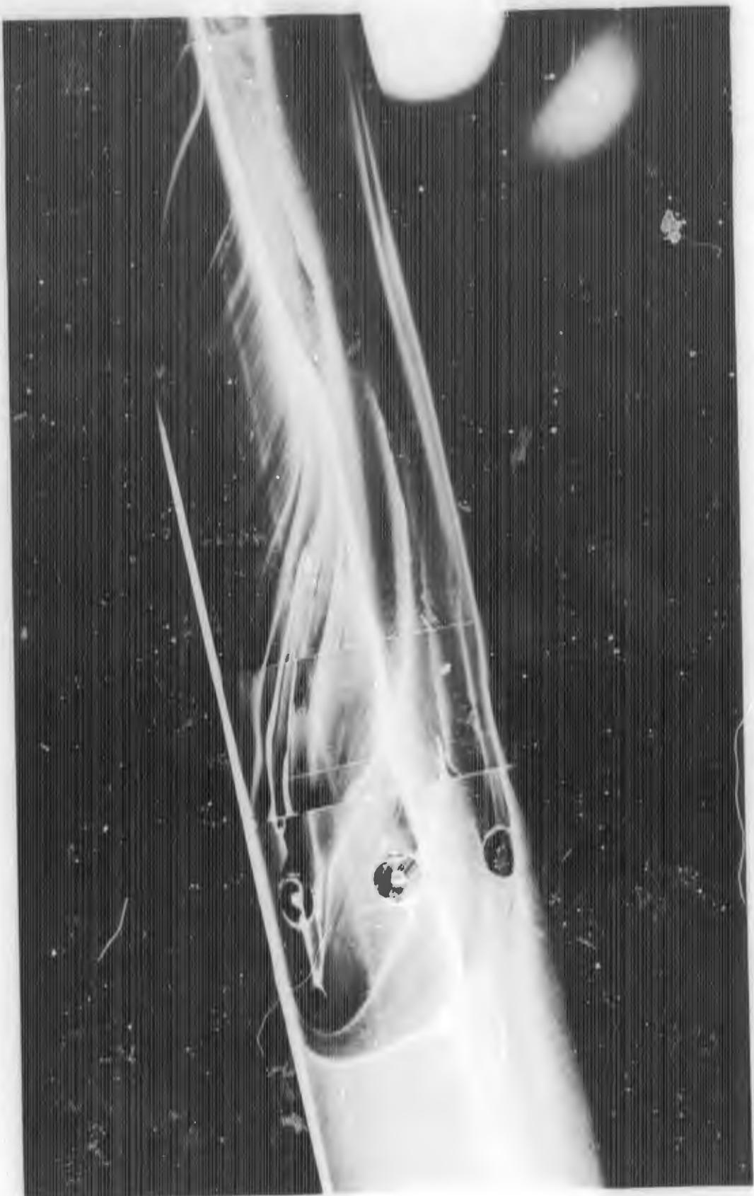
FIGURE C-10f. REACTION JET FOR B<sub>1</sub>C<sub>1</sub>X<sub>3</sub> WITH  $\alpha = -10$  DEGREES;  $P_{0j}/P_{\infty} = 40$
