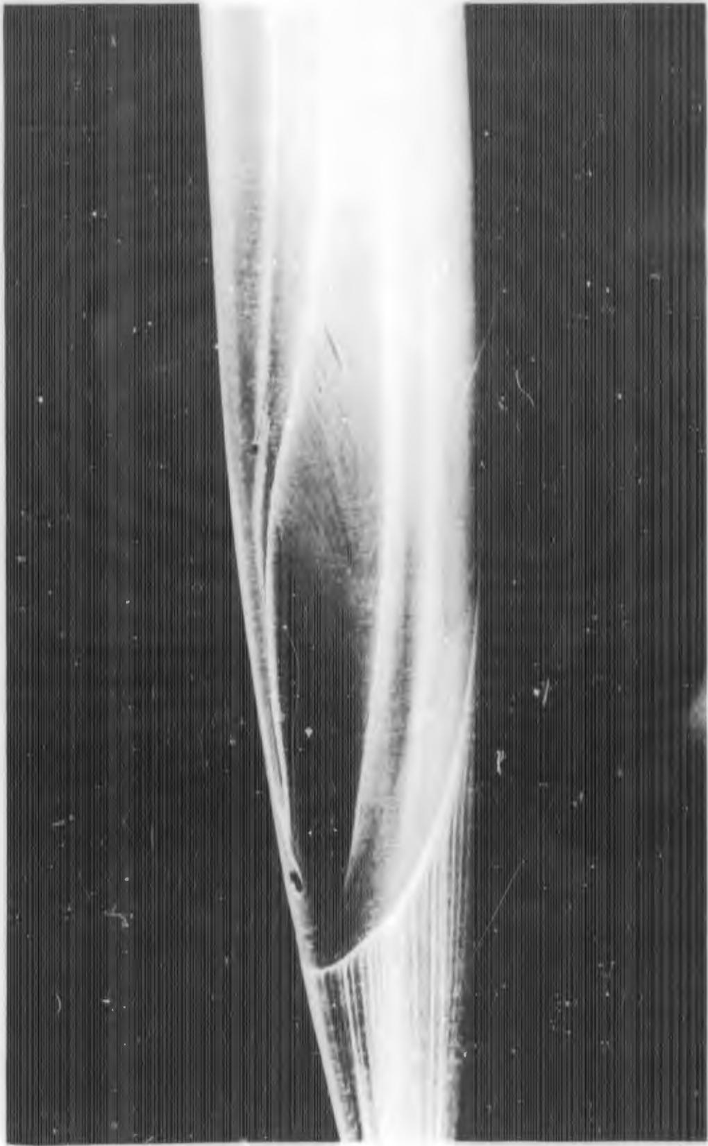
FIGURE E-1g. REACTION JET FOR  $B_1C_1X_0$  WITH  $\alpha = 0$  DEGREES;  $P_{obj}/P_\infty = \sim 550$
