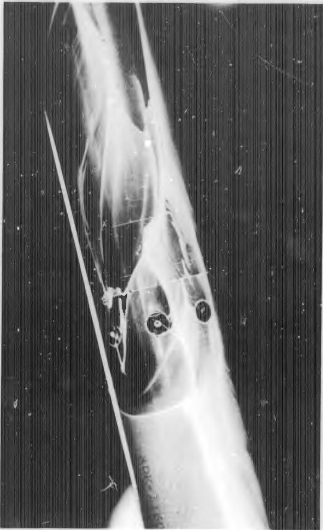
FIGURE C-10h. REACTION JET FOR  $B_1C_1X_3$  WITH  $\alpha = -10$  DEGREES;  $P_{0j}/P_\infty = 100$
