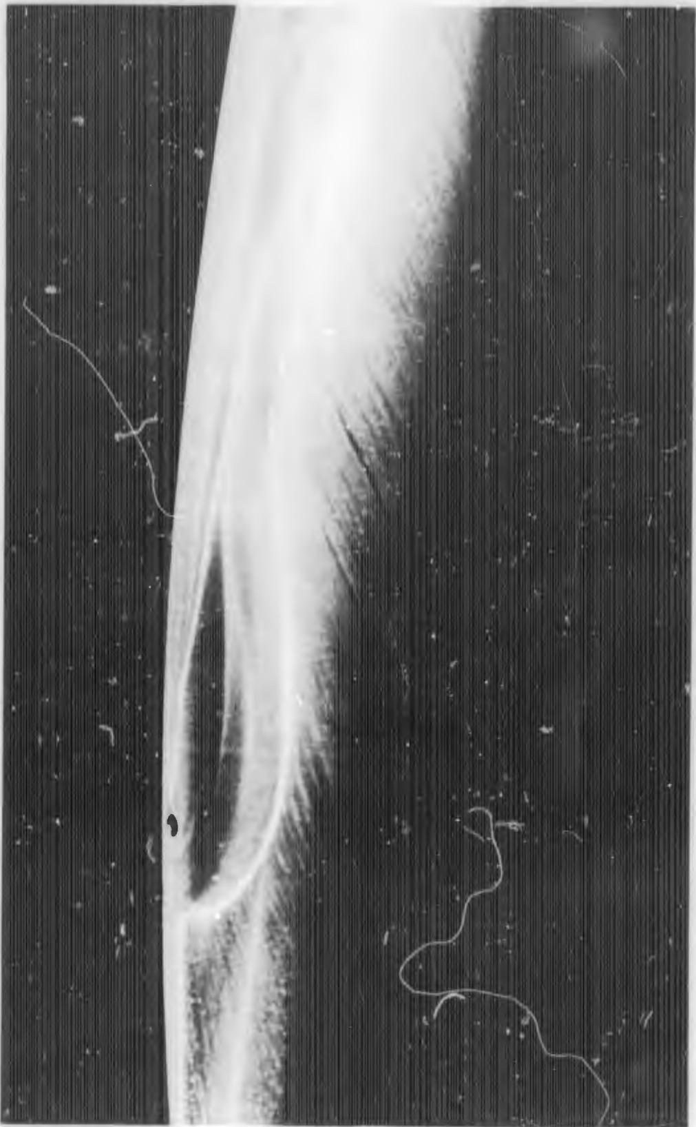
FIGURE E-2d. REACTION JET FOR  $B_1C_1X_0$  WITH  $\alpha = 10$  DEGREES;  $P_{0j}/P_\infty = 100$
