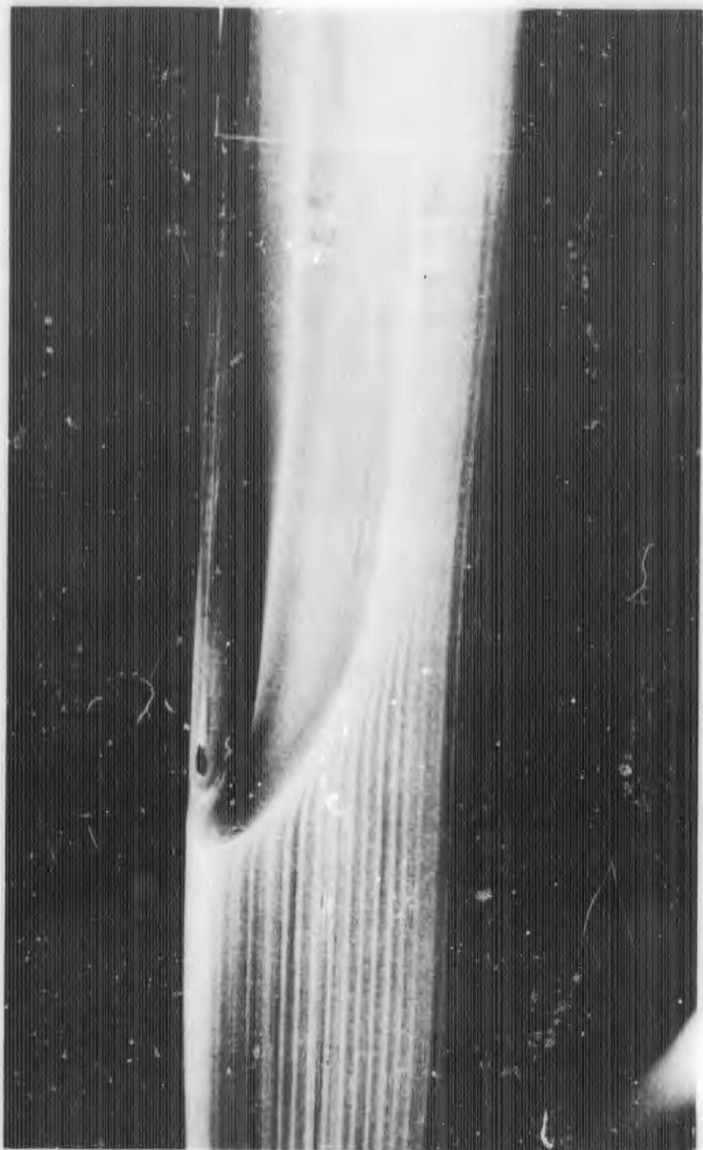
FIGURE E-9f. REACTION JET FOR  $B_1C_1X_2$  WITH  $\alpha = 0$  DEGREES;  $P_{0j}/P_\infty = 40$
