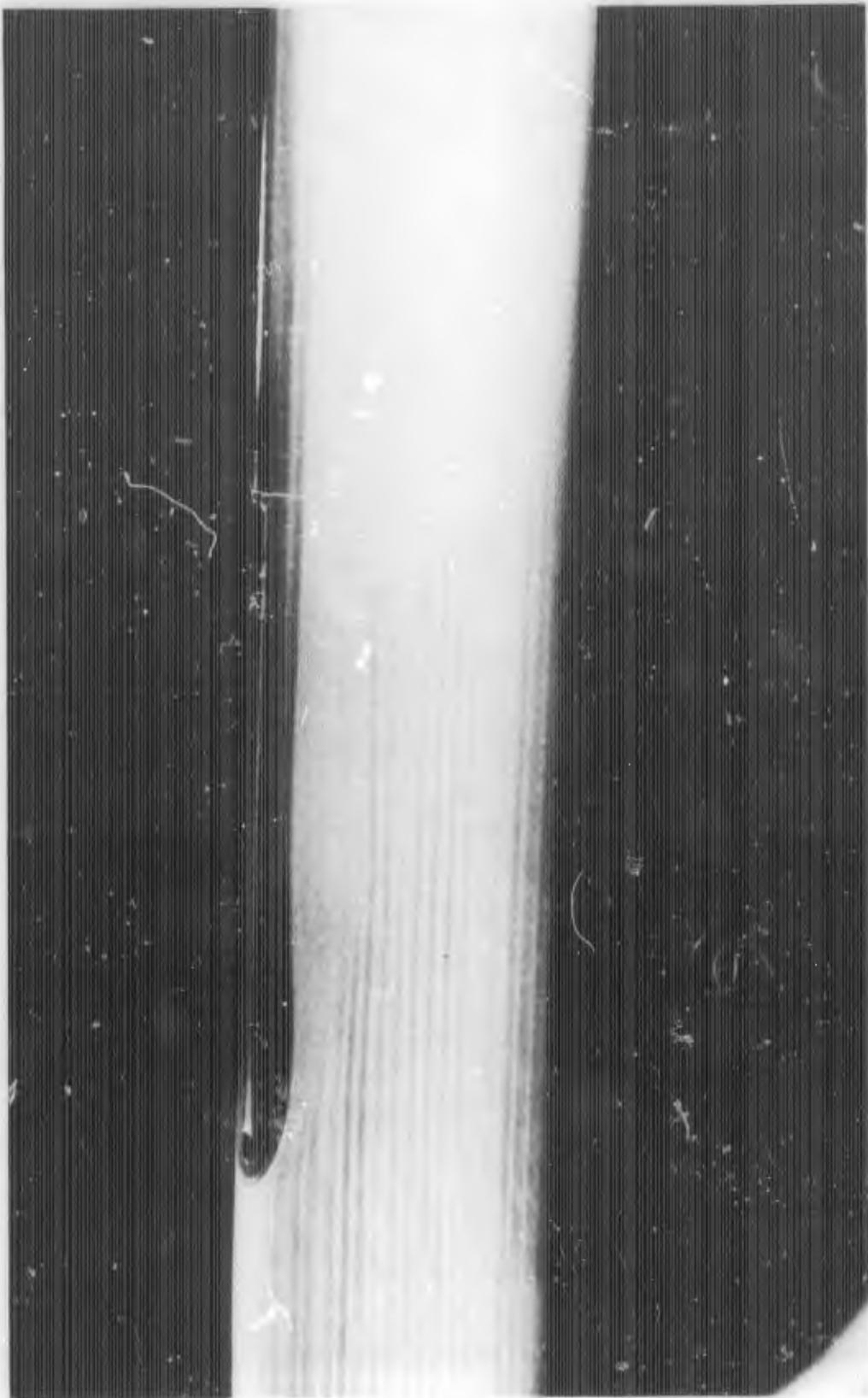
FIGURE E-9b. REACTION JET FOR  $B_1C_1X_2$  WITH  $\alpha = 0$  DEGREES;  $P_{0j}/P_\infty = 0$
