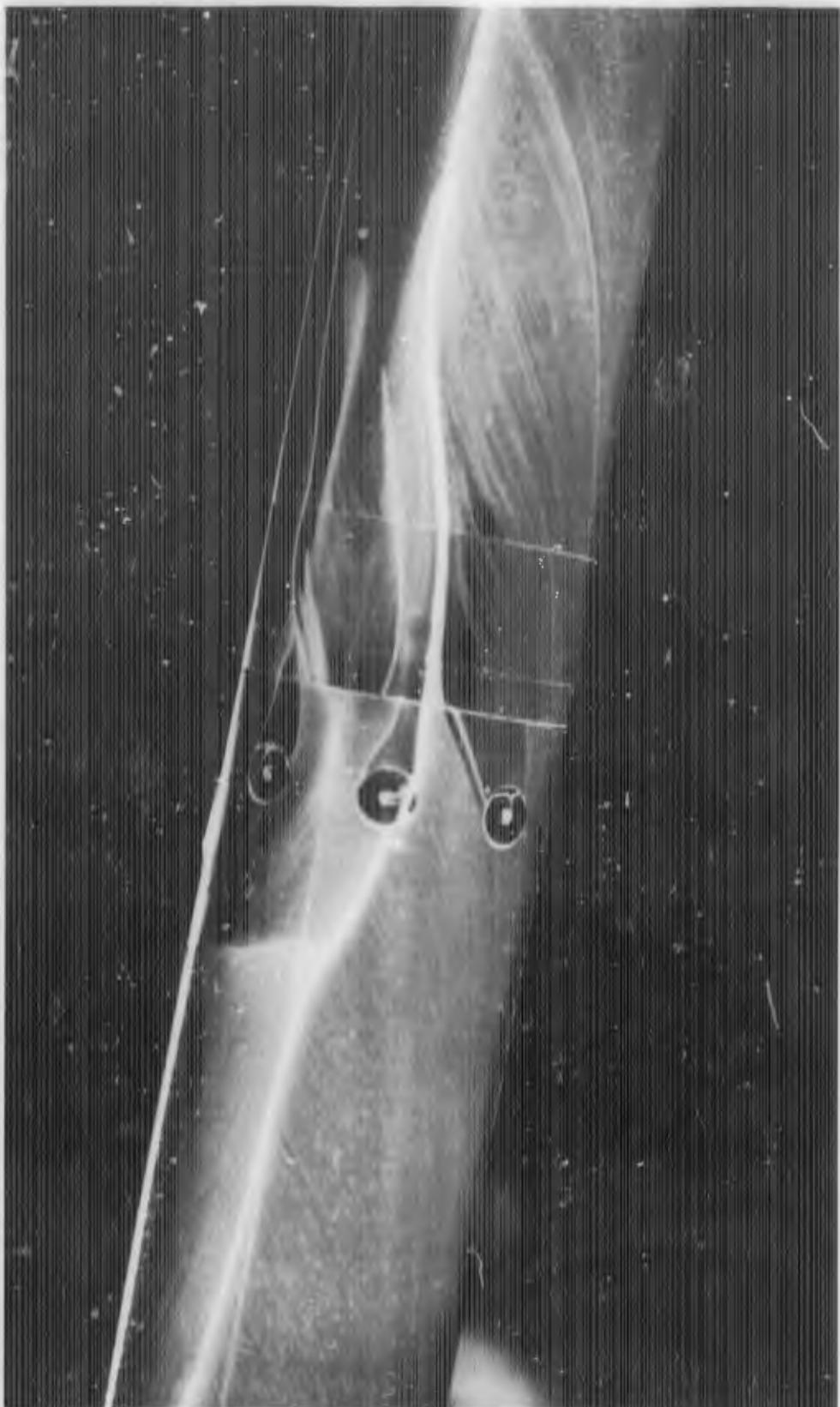
FIGURE C-3f. REACTION JET FOR  $B_1C_1X_3$  WITH  $\alpha = 10$  DEGREES;  $P_{0j}/P_\infty = 40$
