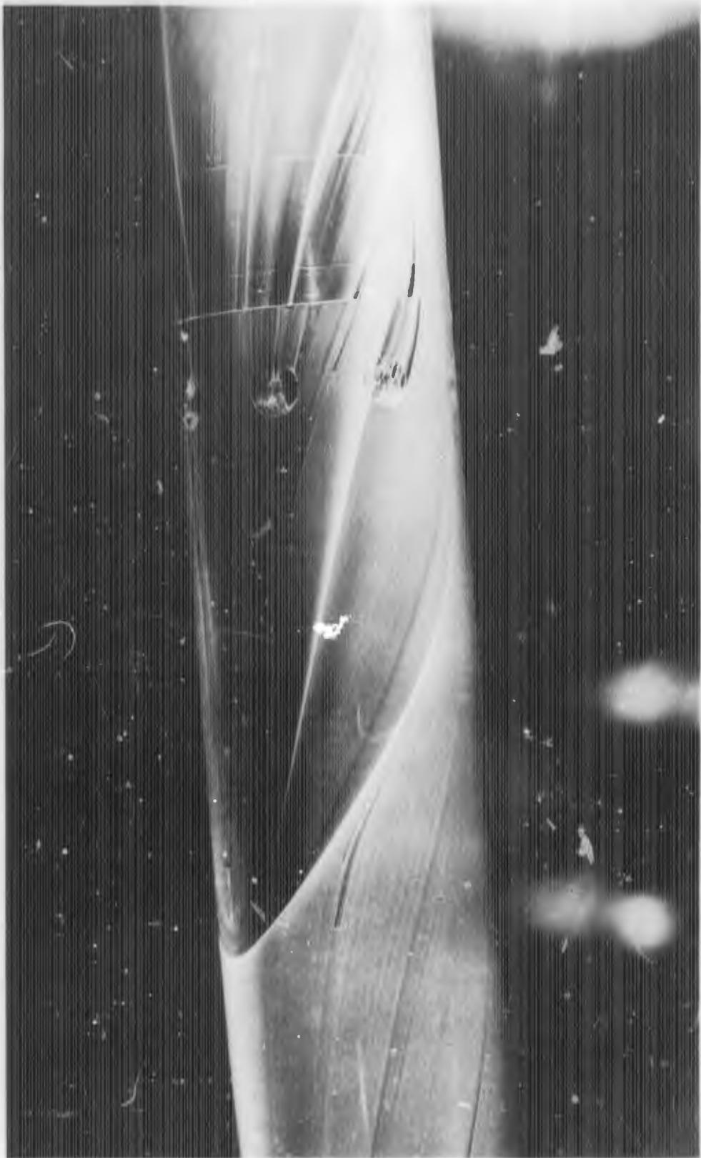
FIGURE E-18b. REACTION JET FOR  $B_1S_1LX_2$  WITH  $\alpha = -5$  DEGREES;  $P_{0j}/P_\infty = 100$
