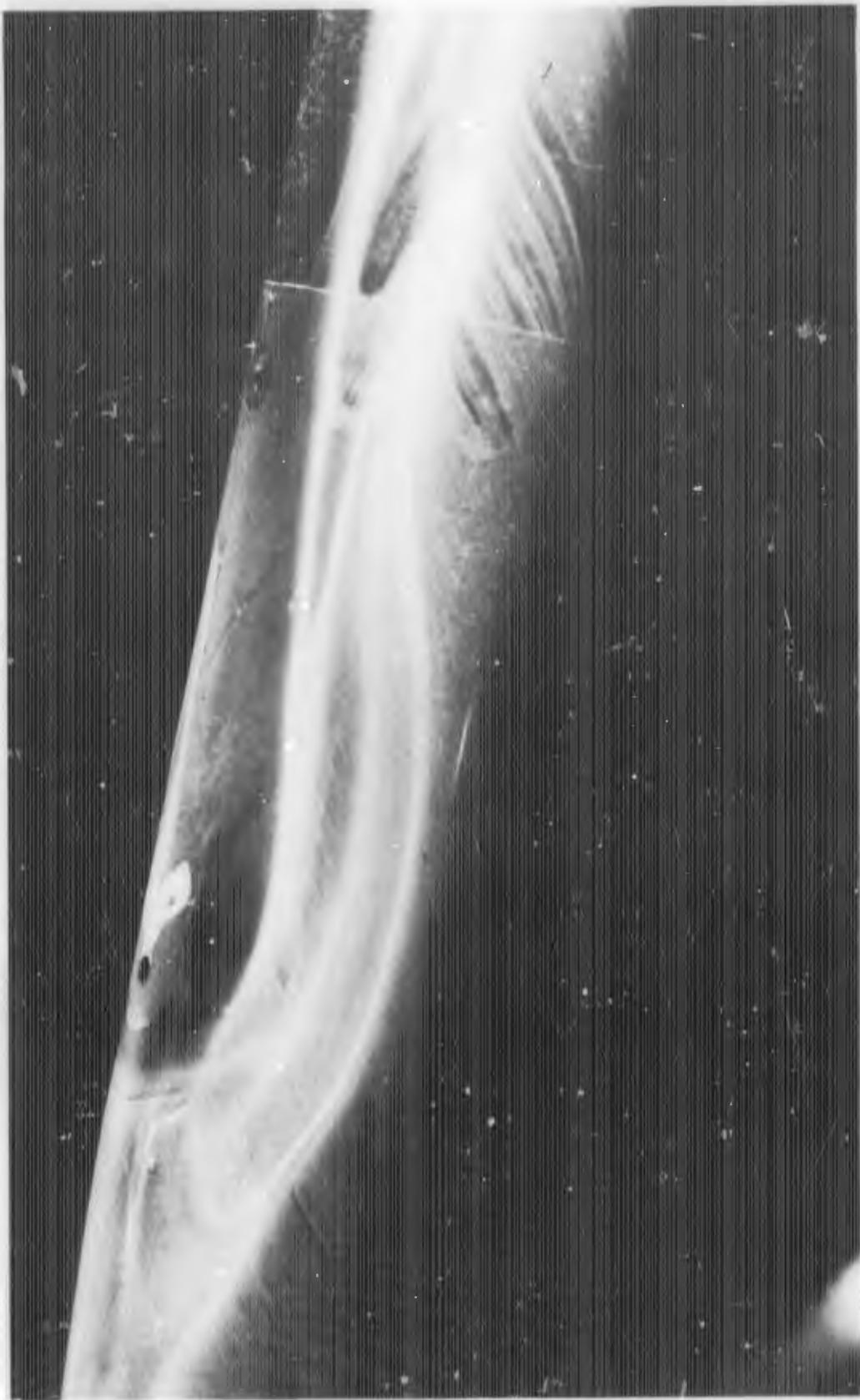
FIGURE E-11b. REACTION JET FOR  $B_1C_1X_2$  WITH  $\alpha = 10$  DEGREES;  $P_{0j}/P_\infty = 100$
