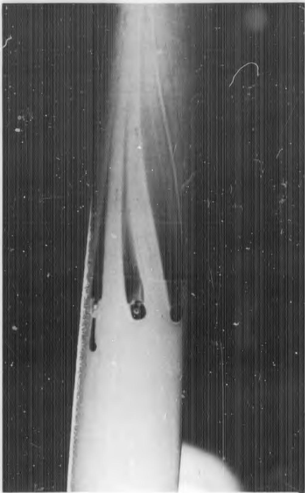
FIGURE C-7b. REACTION JET FOR  $B_1C_1X_3$  WITH  $\alpha = 5$  DEGREES;  $P_{0j}/P_\infty = 0$
