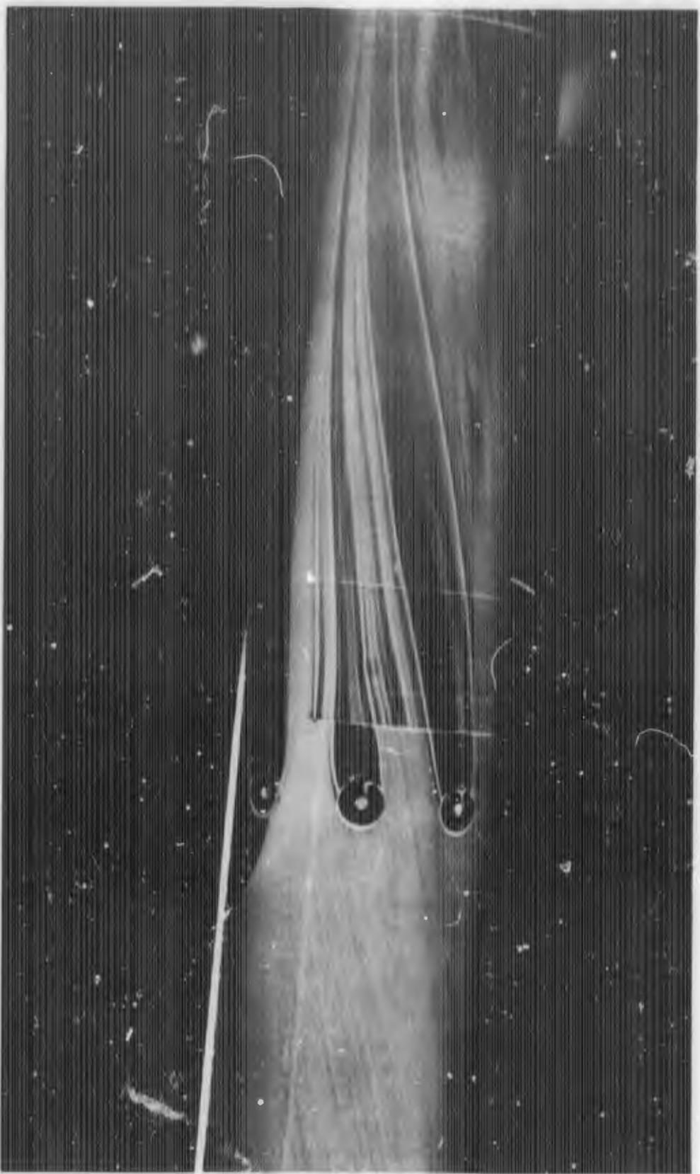
FIGURE C-2d. REACTION JET FOR B<sub>1</sub>C<sub>1</sub>X<sub>3</sub> WITH  $\alpha = 5$  DEGREES;  $P_{0j}/P_{\infty} = 10$
