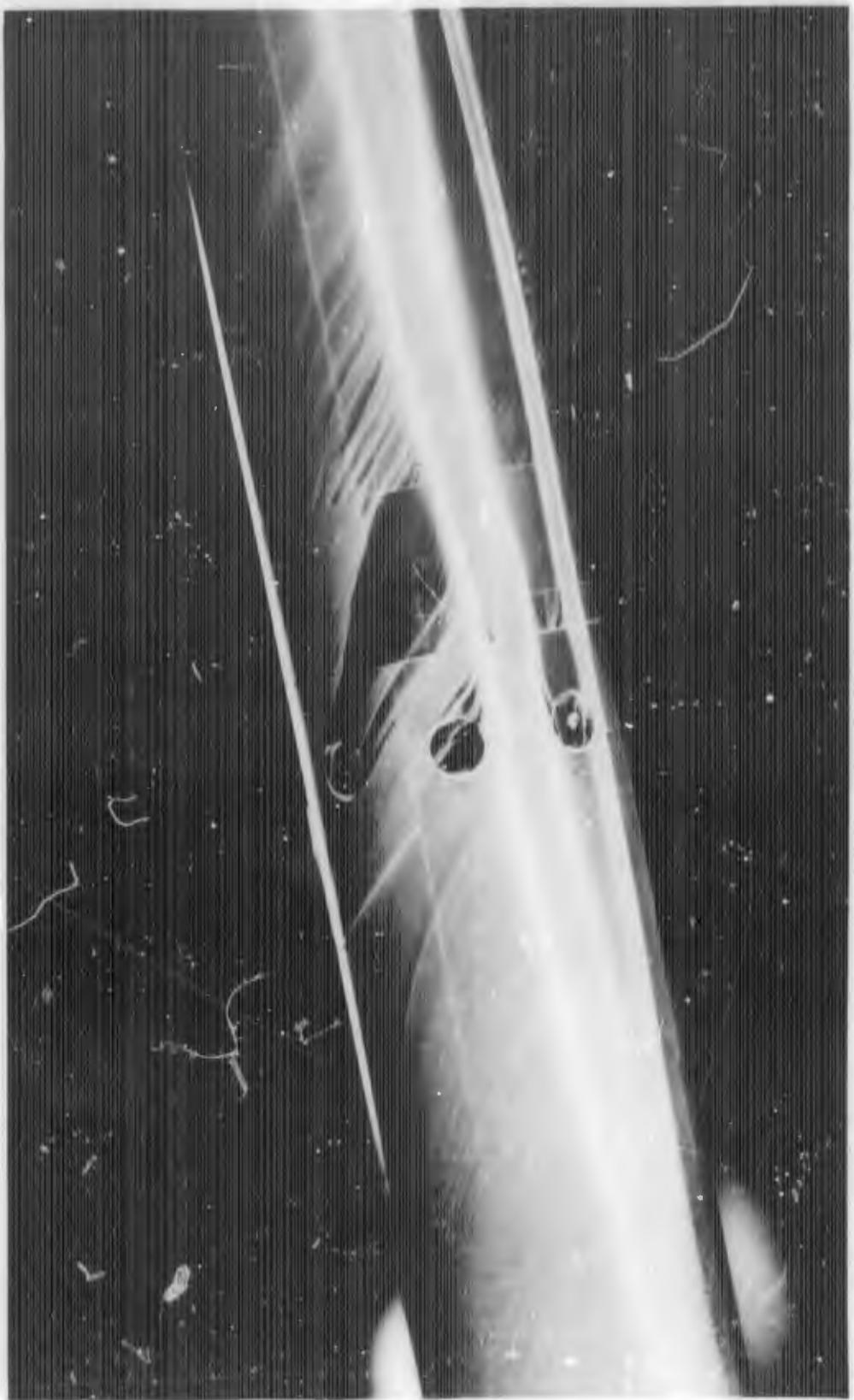
FIGURE D-5h. REACTION JET FOR  $B_1C_1X_3$  WITH  $\alpha = -10$  DEGREES;  $P_{obj}/P_\infty = 100$
