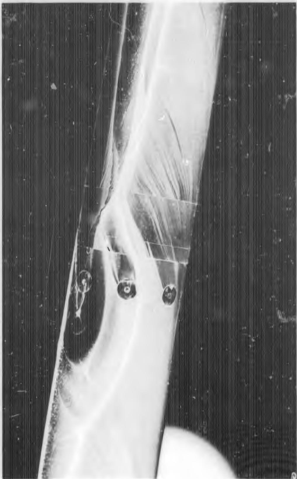
FIGURE C-8h. REACTION JET FOR  $B_1C_1X_3$  WITH  $\alpha = 10$  DEGREES;  $P_{0j}/P_\infty = 100$
