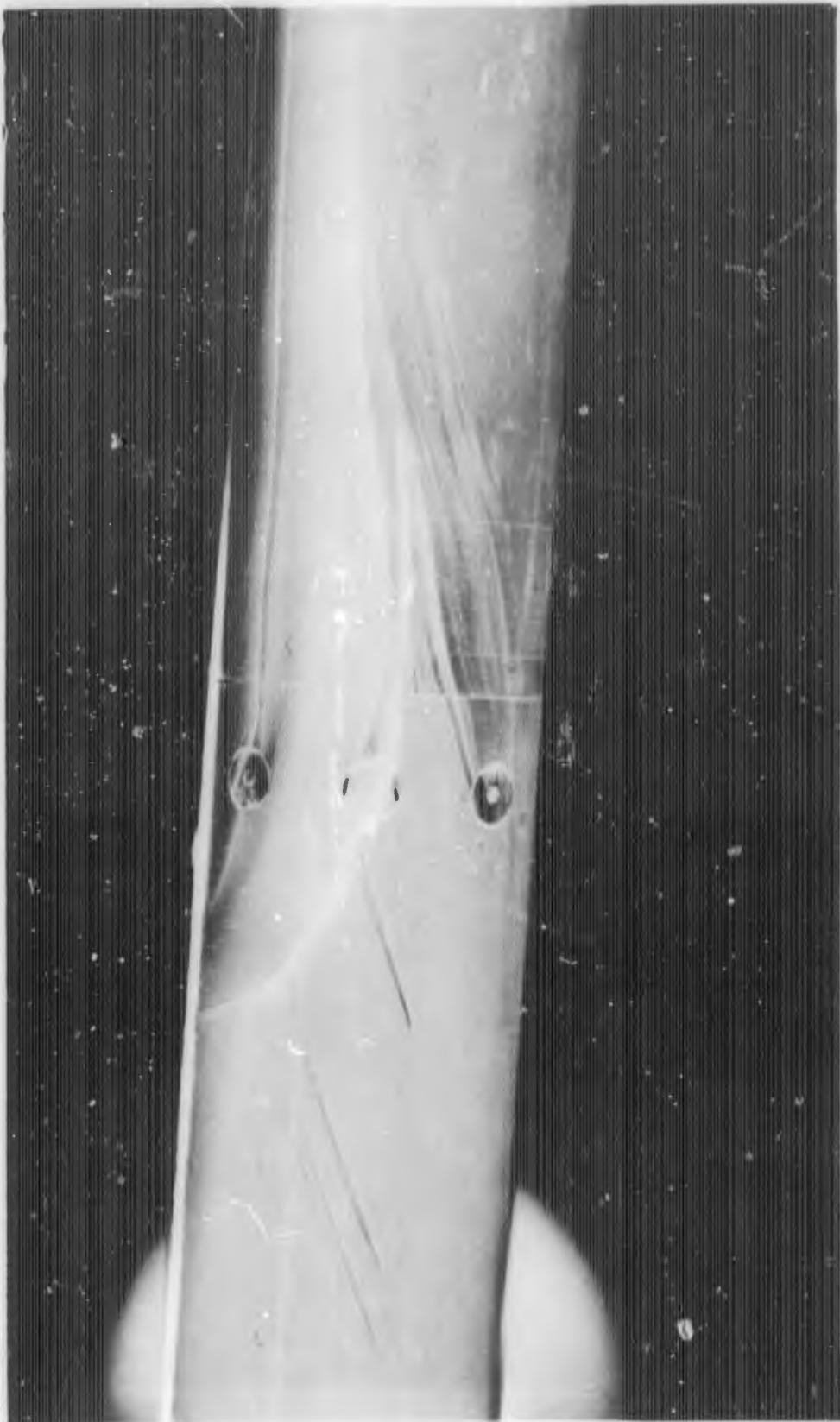
FIGURE D-2h. REACTION JET FOR  $B_1C_1X_3$  WITH  $\alpha = 5$  DEGREES;  $P_{0j}/P_\infty = 100$
