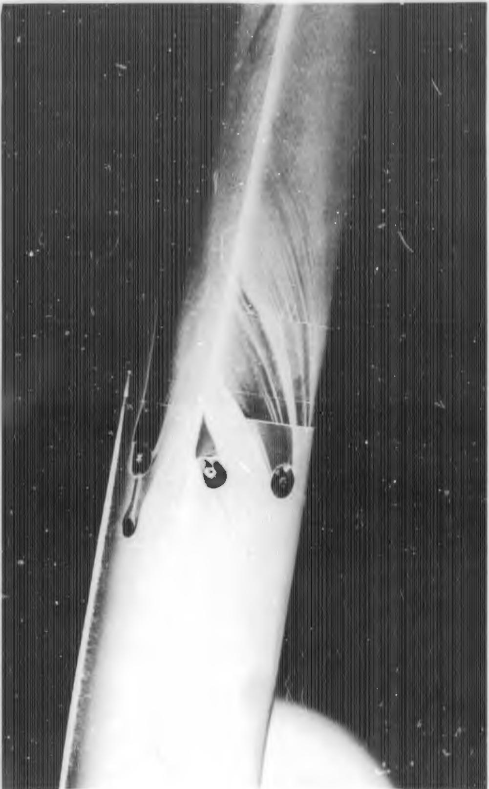
FIGURE C-8b. REACTION JET FOR  $B_1C_1N_3$  WITH  $\alpha = 10$  DEGREES;  $P_{0j}/P_\infty = 0$
