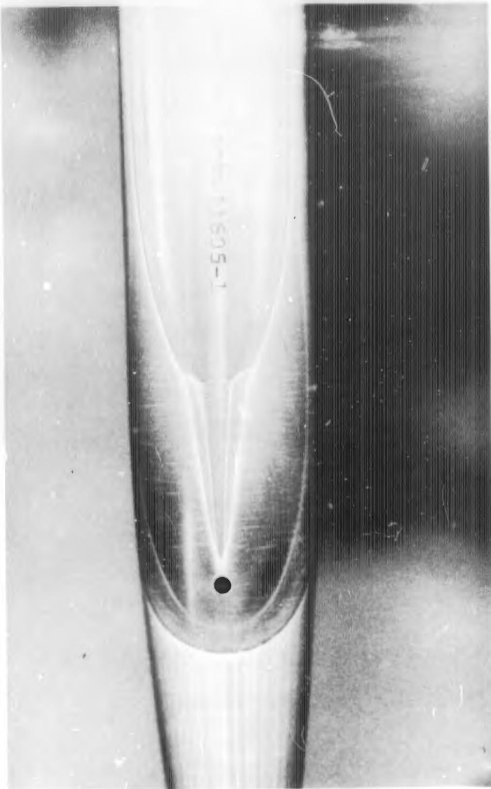
FIGURE B-6c. REACTION JET FOR  $B_1C_1X_1$  WITH  $\alpha = 0$  DEGREES;  $P_{0j}/P_\infty = 100$
