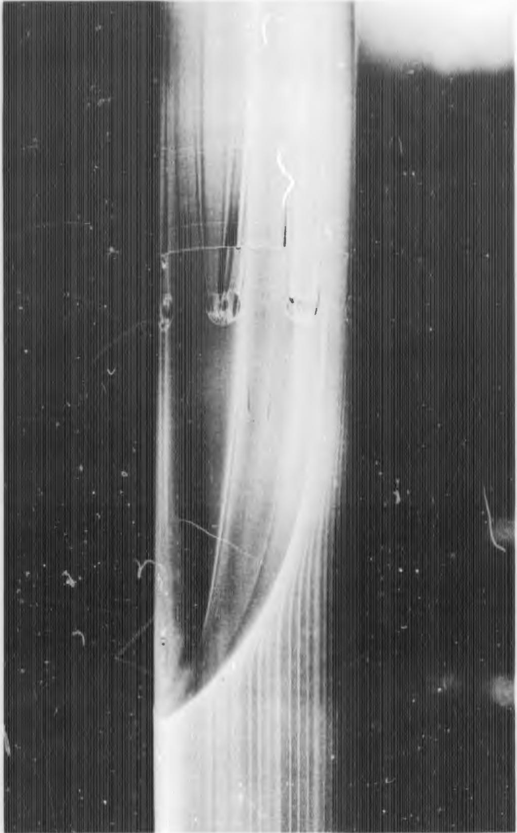
FIGURE E-15f. REACTION JET FOR  $B_1S_1L_2$  WITH  $\alpha = 0$  DEGREES;  $P_{0j}/P_\infty = 100$
