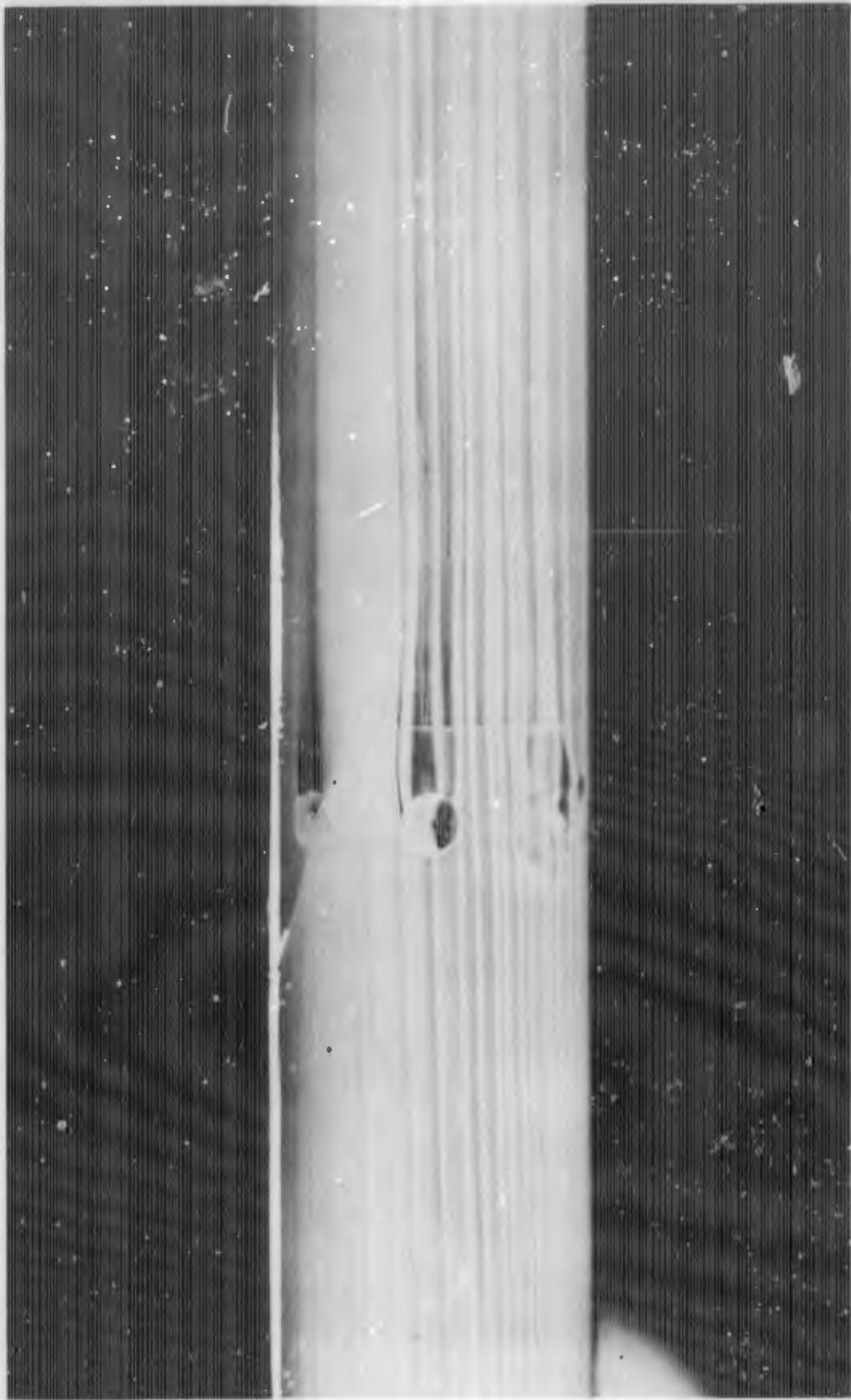
FIGURE D-1d. REACTION JET FOR  $B_1C_1X_3$  WITH  $\alpha = 0$  DEGREES;  $P_{obj}/P_\infty = 10$
