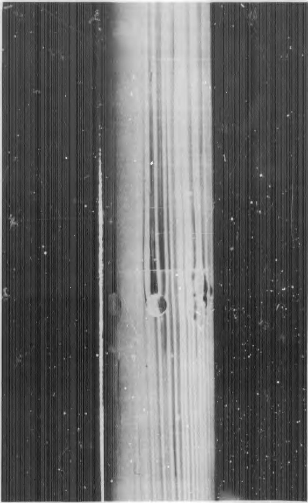
FIGURE D-1b. REACTION JET FOR  $B_1C_1X_3$  WITH  $\alpha = 0$  DEGREES;  $P_{0j}/P_\infty = 0$
