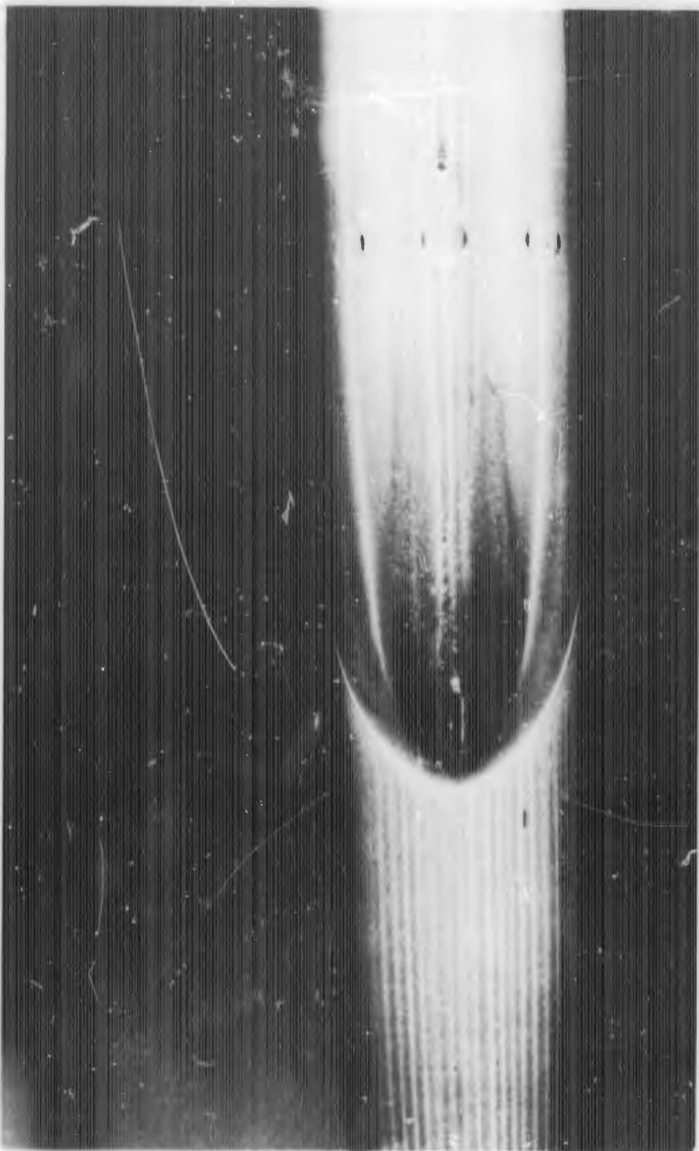
FIGURE E-15c. REACTION JET FOR  $B_1S_1L_2$  WITH  $\alpha = 0$  DEGREES;  $P_{0j}/P_\infty = 40$
