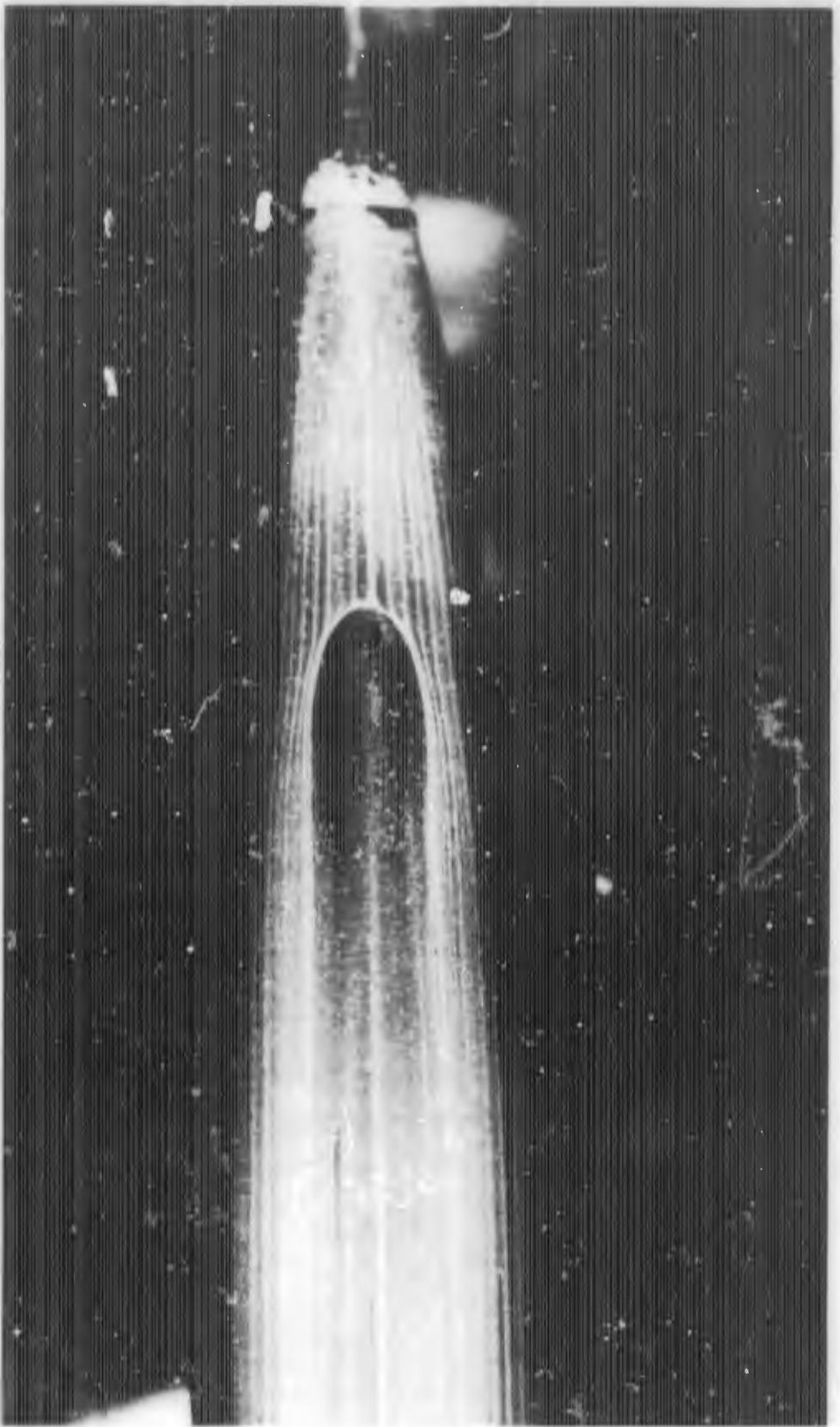
FIGURE E-1a. REACTION JET FOR  $B_1C_1X_0$  WITH  $\alpha = 0$  DEGREES;  $P_{0j}/P_\infty = 0$
