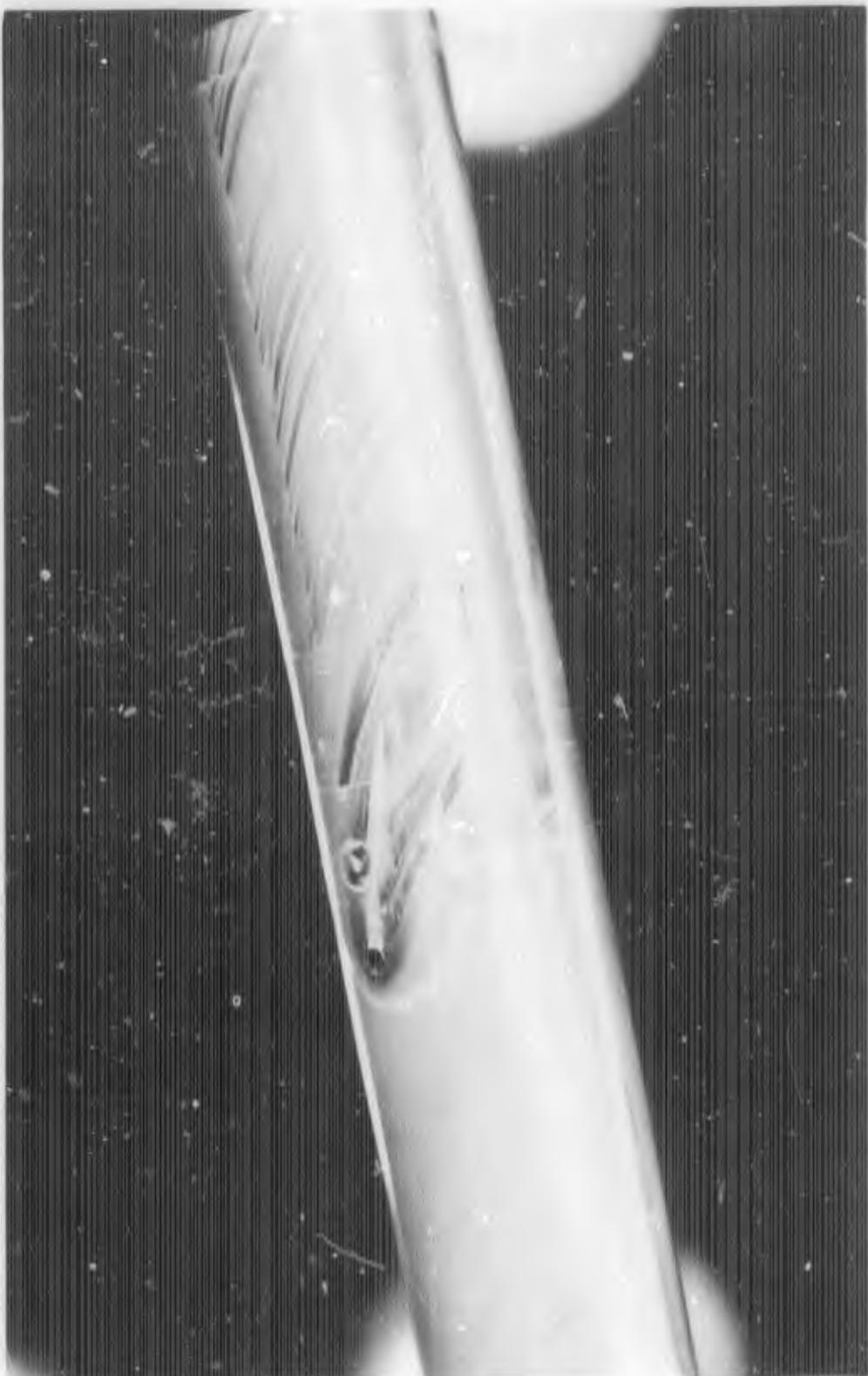
FIGURE D-10d. REACTION JET FOR  $B_1C_1X_3$  WITH  $\alpha = -10$  DEGREES;  $P_{oj}/P_\infty = 10$
