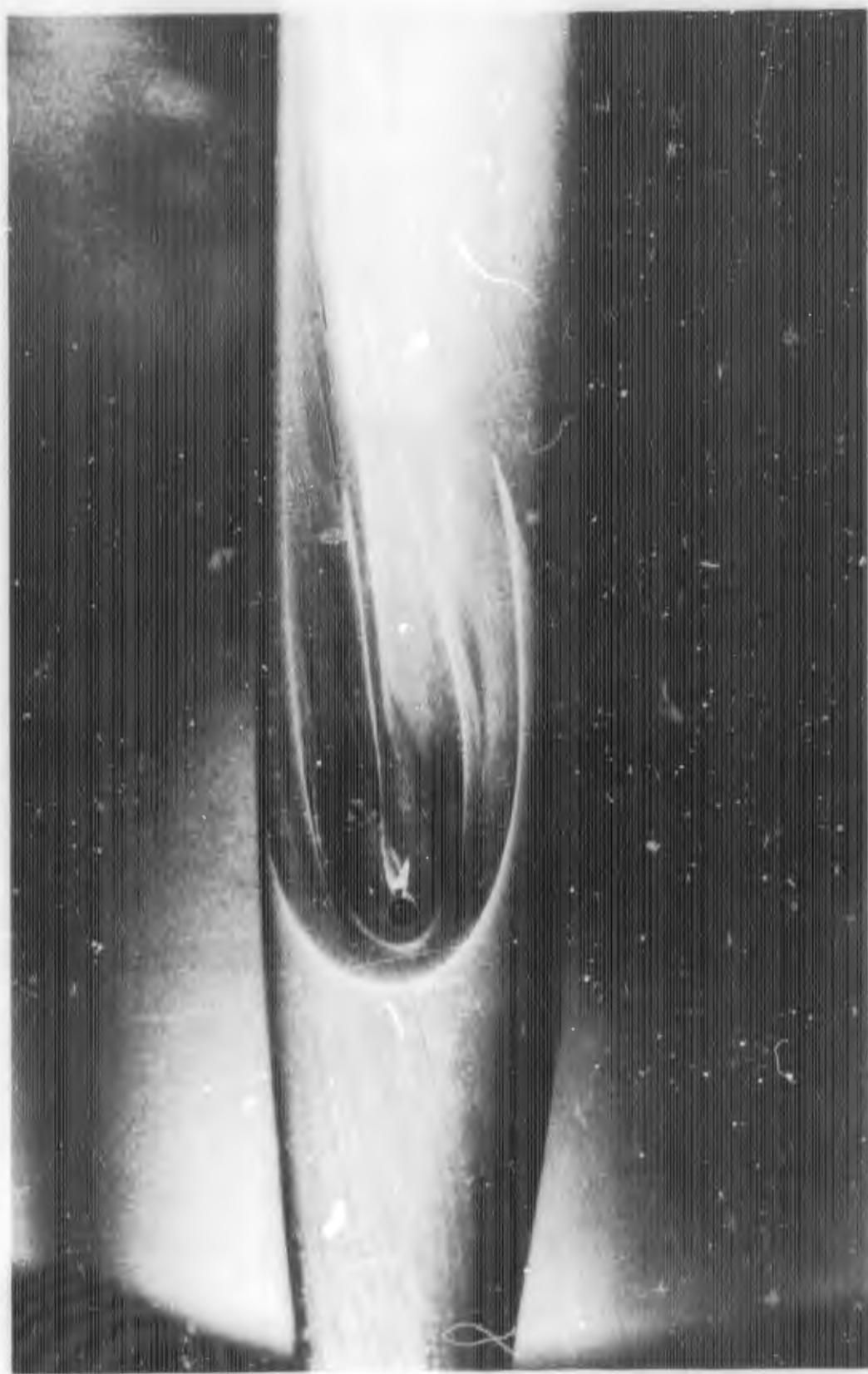
FIGURE I-5a. REACTION JET FOR B<sub>1</sub>C<sub>1</sub>N<sub>1</sub> WITH  $\alpha \approx 5$  DEGREES;  $P_{0j}/P_\infty = 40$
