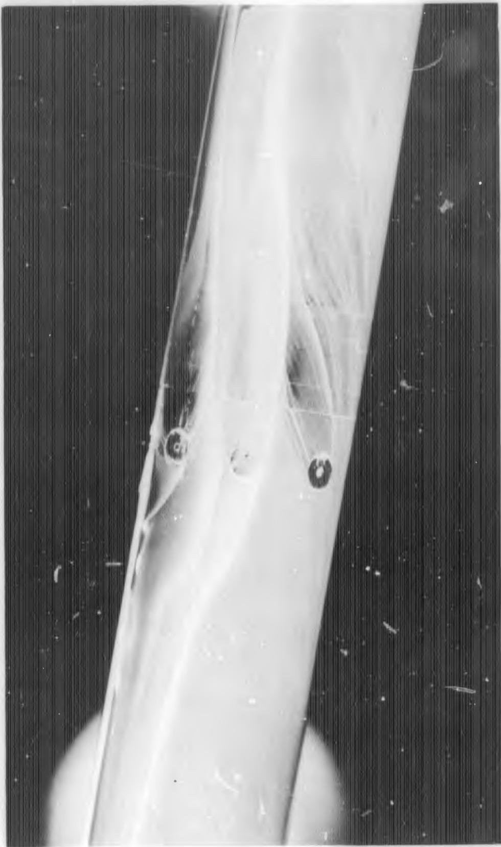
FIGURE D-3h. REACTION JET FOR  $B_1C_1X_3$  WITH  $\alpha = 10$  DEGREES;  $P_{obj}/P_\infty = 100$
