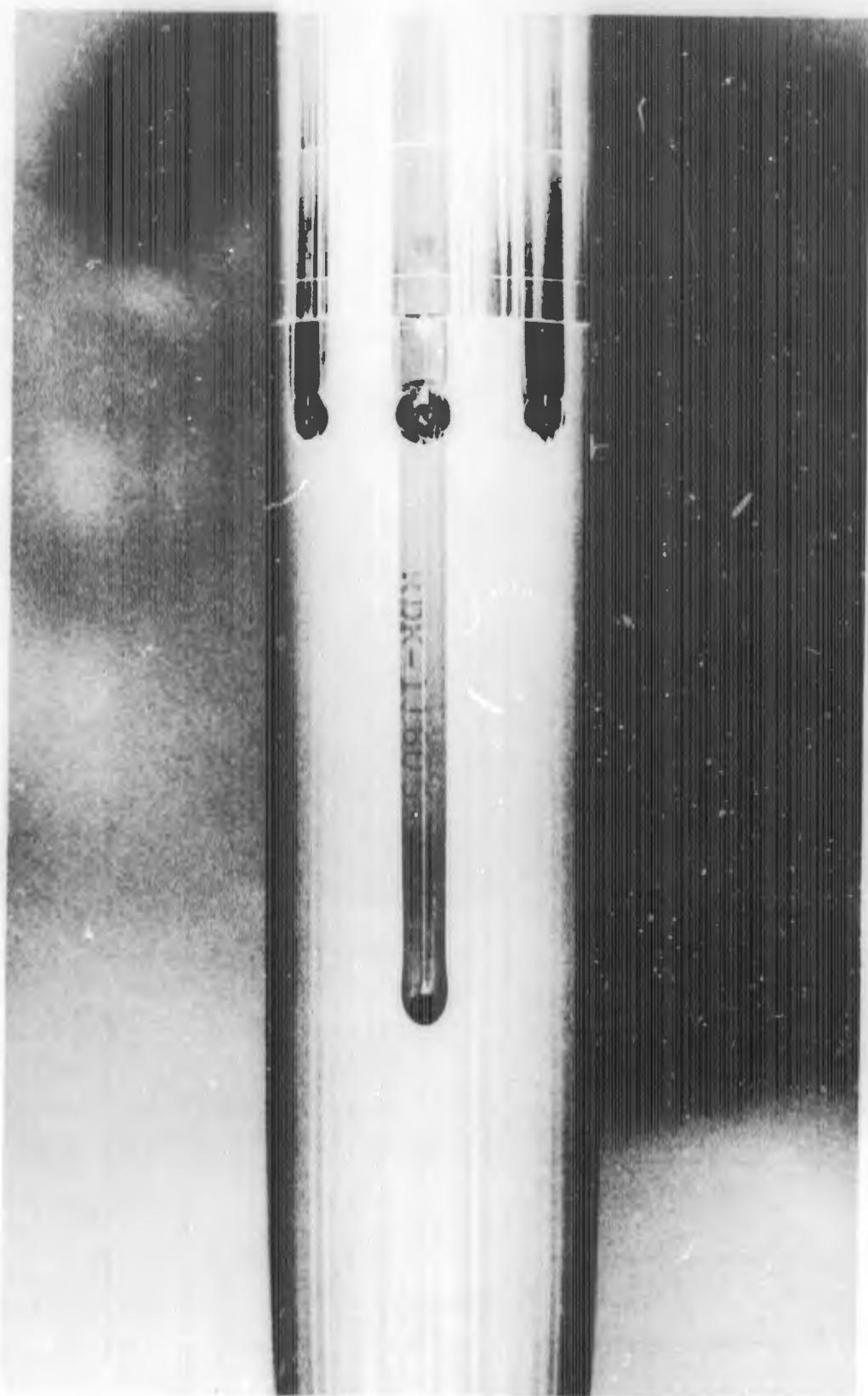
FIGURE B-1a. REACTION JET FOR  $B_1C_1X_2$  WITH  $\alpha = 0$  DEGREES;  $P_{0j}/P_\infty = 0$
