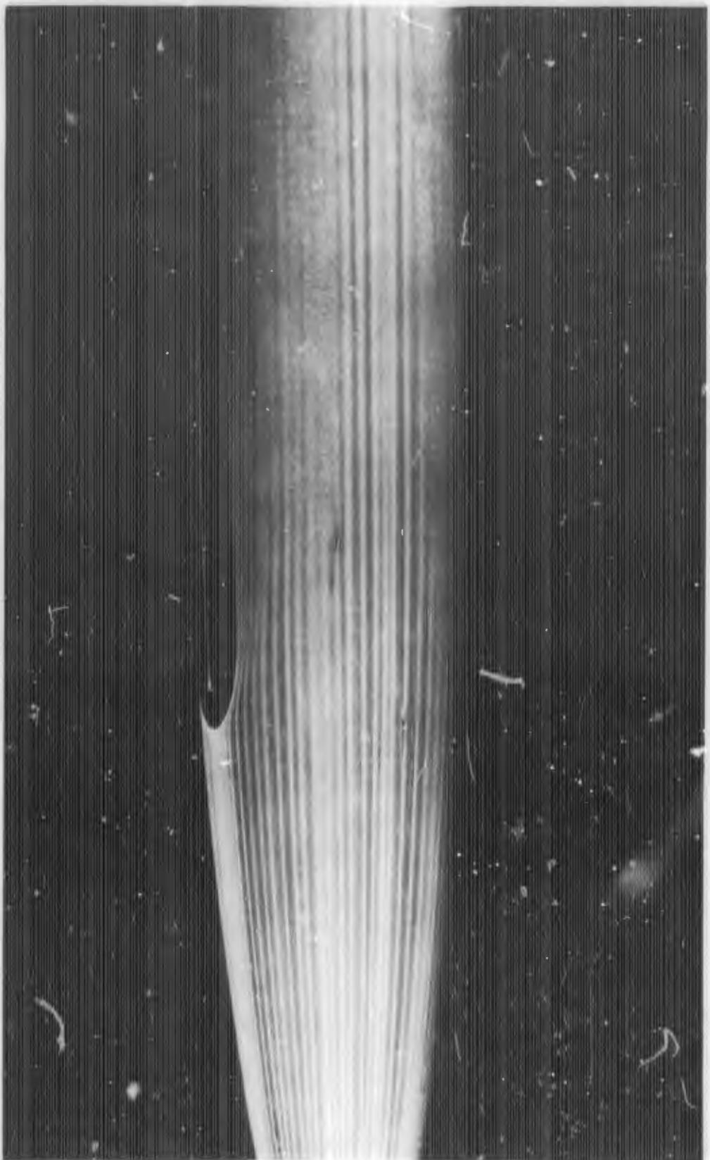
FIGURE E-4b. REACTION JET FOR  $B_1C_1X_1$  WITH  $\alpha = 0$  DEGREES;  $P_{0j}/P_\infty = 0$
