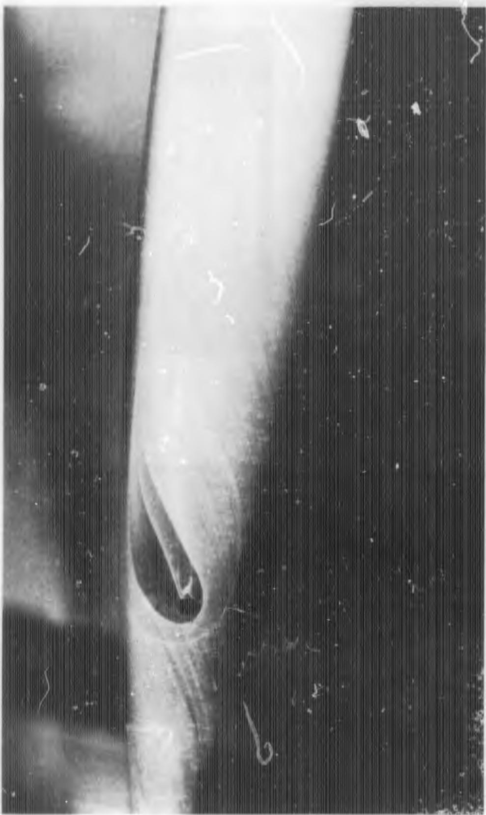
FIGURE E-2a. REACTION JET FOR  $B_1 C_1 X_0$  WITH  $\alpha = 10$  DEGREES;  $P_{0j}/P_\infty = 0$
