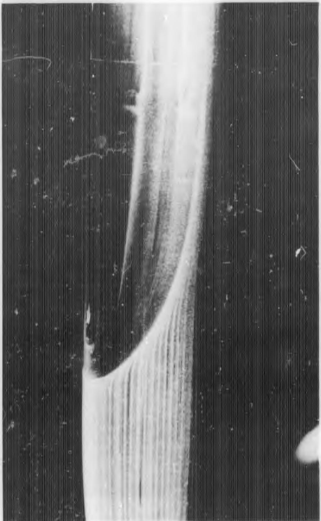
FIGURE E-9h. REACTION JET FOR  $B_1C_1X_2$  WITH  $\alpha = 0$  DEGREES;  $P_{0j}/P_\infty = 100$
