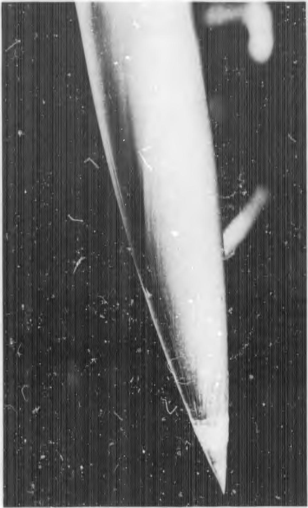
FIGURE E-3a. REACTION JET FOR  $B_1C_1X_0$  WITH  $\alpha = -10$  DEGREES;  $P_{obj}/P_\infty = 0$
