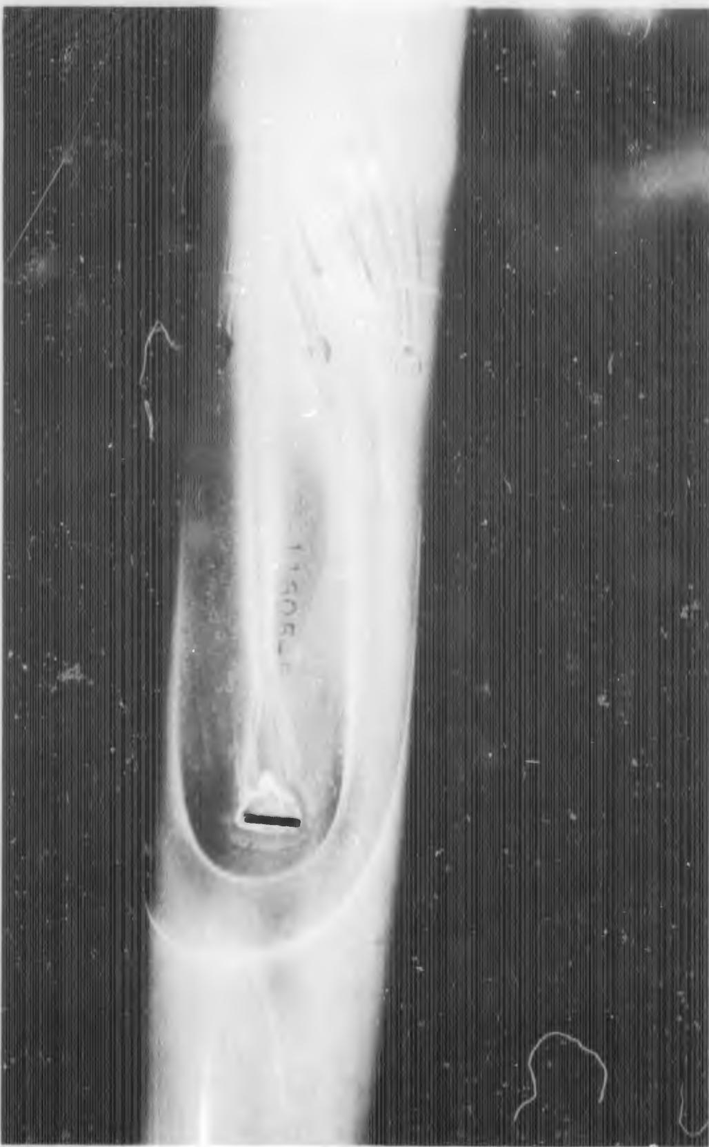
FIGURE E-21b. REACTION JET FOR  $B_1S_1T^X_2$  WITH  $\alpha = 5$  DEGREES;  $P_{0j}/P_\infty = 100$
