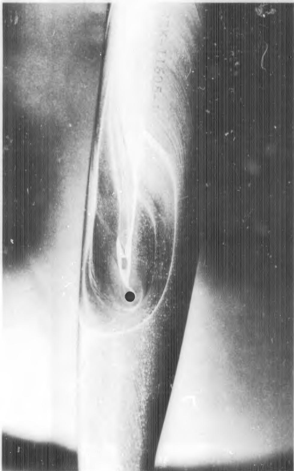
FIGURE E-6c. REACTION JET FOR  $B_1C_1N_1$  WITH  $\alpha = 10$  DEGREES;  $P_{obj}/P_\infty = 40$
