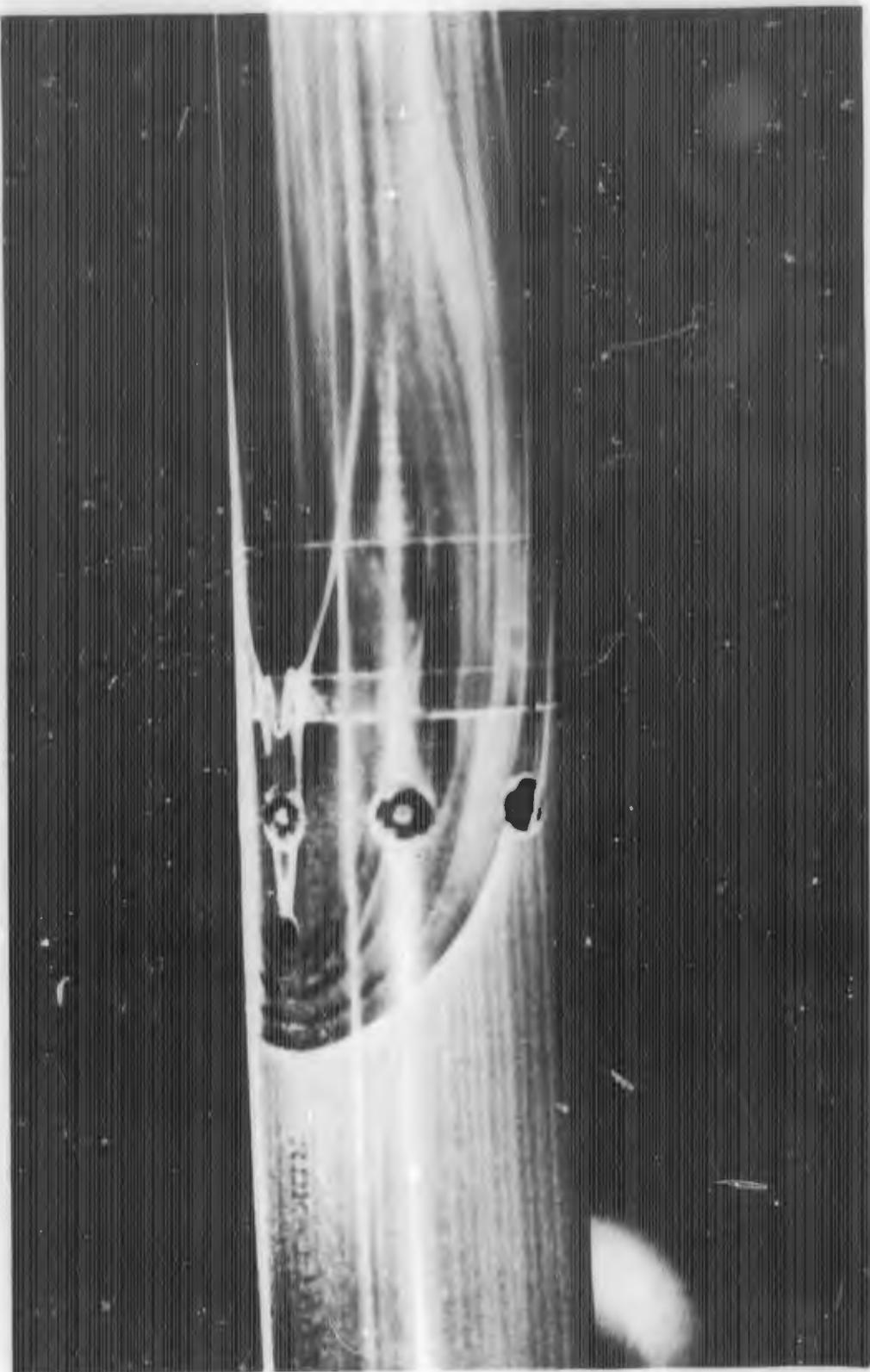
FIGURE C-6f. REACTION JET FOR  $B_1C_1X_3$  WITH  $\alpha = 0$  DEGREES;  $P_{0j}/P_\infty = 40$
