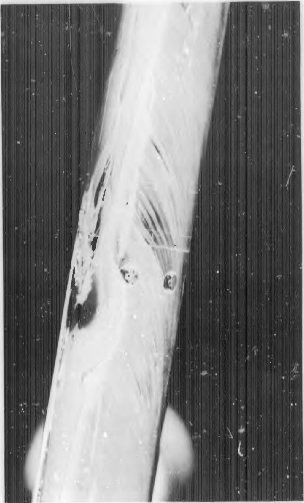
FIGURE D-8f. REACTION JET FOR B<sub>1</sub>C<sub>1</sub>X<sub>3</sub> WITH  $\alpha = 10$  DEGREES;  $P_{0j}/P_{\infty} = 40$
