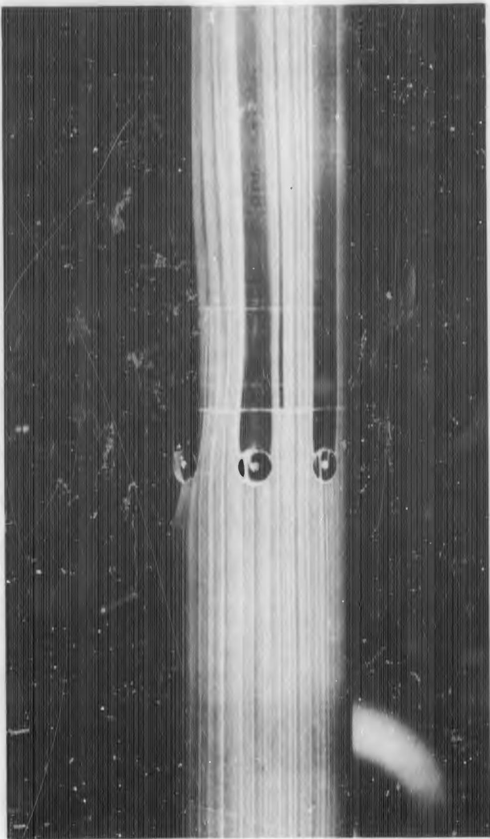
FIGURE C-1d. REACTION JET FOR BC<sub>1</sub>X<sub>3</sub> WITH  $\alpha = 0$  DEGREES;  $P_{0j}/P_{\infty} = 10$
