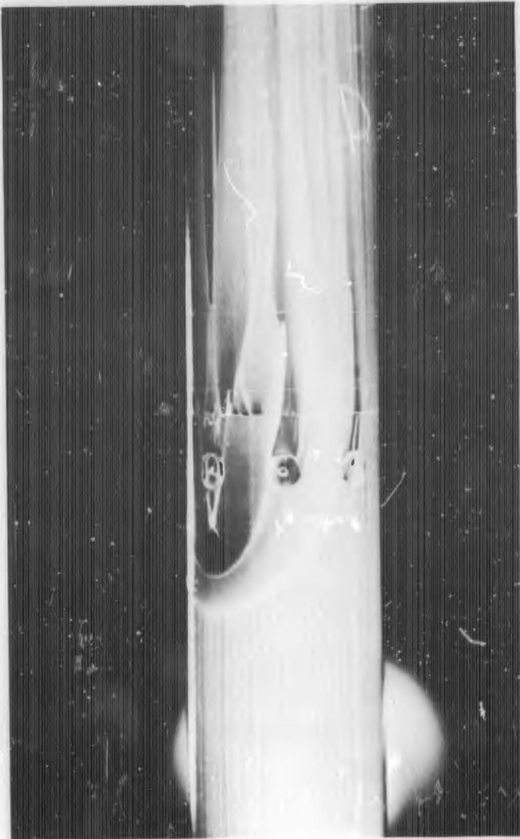
FIGURE D-6g. REACTION JET FOR  $B_1C_1X_3$  WITH  $\alpha = 0$  DEGREES;  $P_{0j}/P_\infty = 100$
