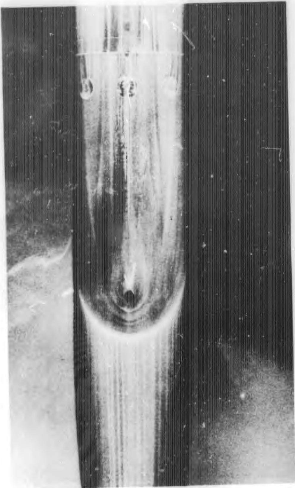
FIGURE E-9g. REACTION JET FOR  $B_1C_1X_2$  WITH  $\alpha = 0$  DEGREES;  $P_{oj}/P_\infty = 100$
