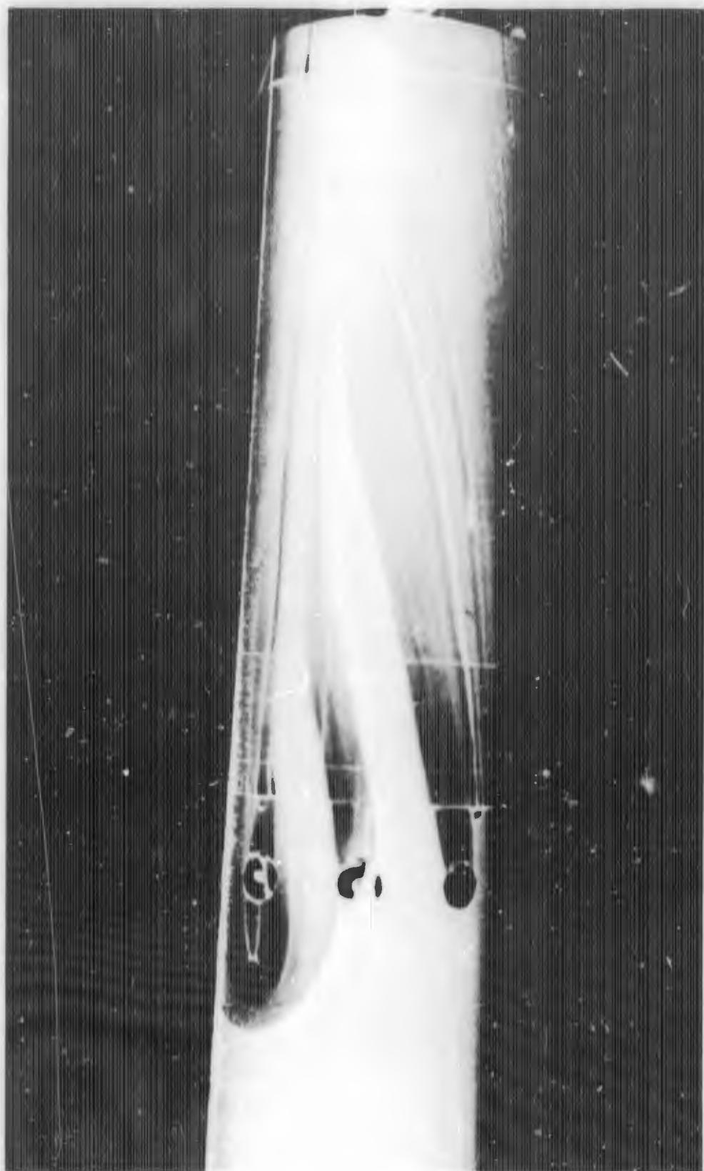
FIGURE C-7d. REACTION JET FOR  $B_1C_1X_3$  WITH  $\alpha = 5$  DEGREES;  $P_{0j}/P_\infty = 10$
