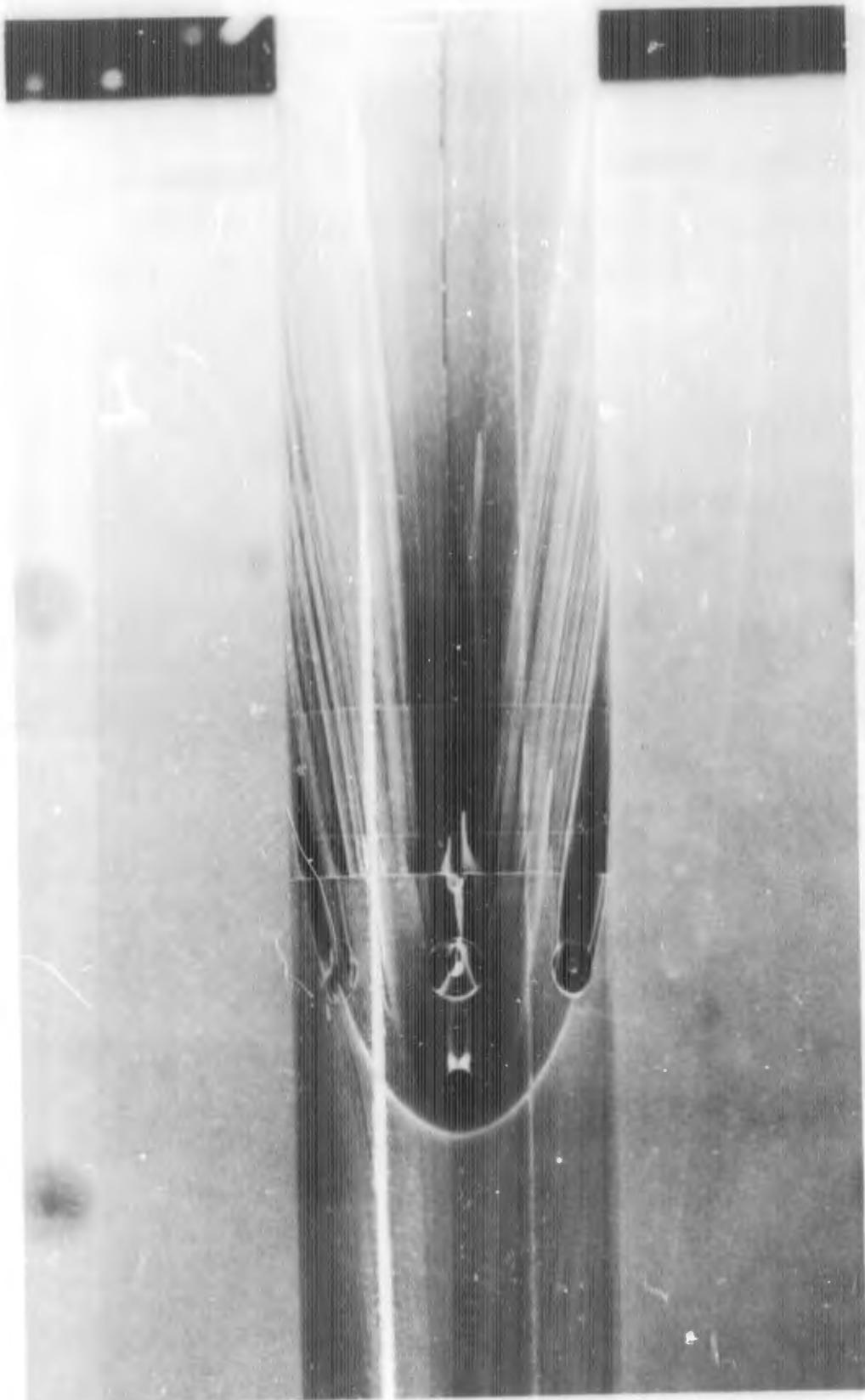
FIGURE D-4c. REACTION JET FOR  $B_1C_1X_3$  WITH  $\alpha = -5$  DEGREES;  $P_{0j}/P_\infty = 10$
