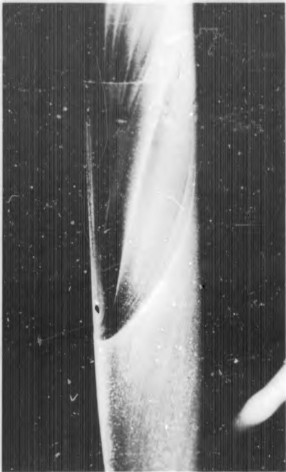
FIGURE E-12b. REACTION JET FOR  $B_1C_1X_2$  WITH  $\alpha = -5$  DEGREES;  $P_{0j}/P_\infty = 100$
