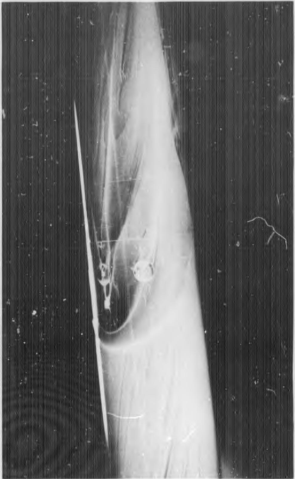
FIGURE D-9h. REACTION JET FOR  $B_1C_1X_3$  WITH  $\alpha = -5$  DEGREES;  $P_{obj}/P_\infty = 100$
