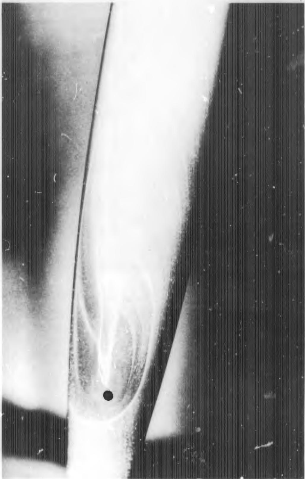
FIGURE E-2c. REACTION JET FOR  $B_1C_1X_0$  WITH  $\alpha = 10$  DEGREES;  $P_{0j}/P_\infty = 100$
