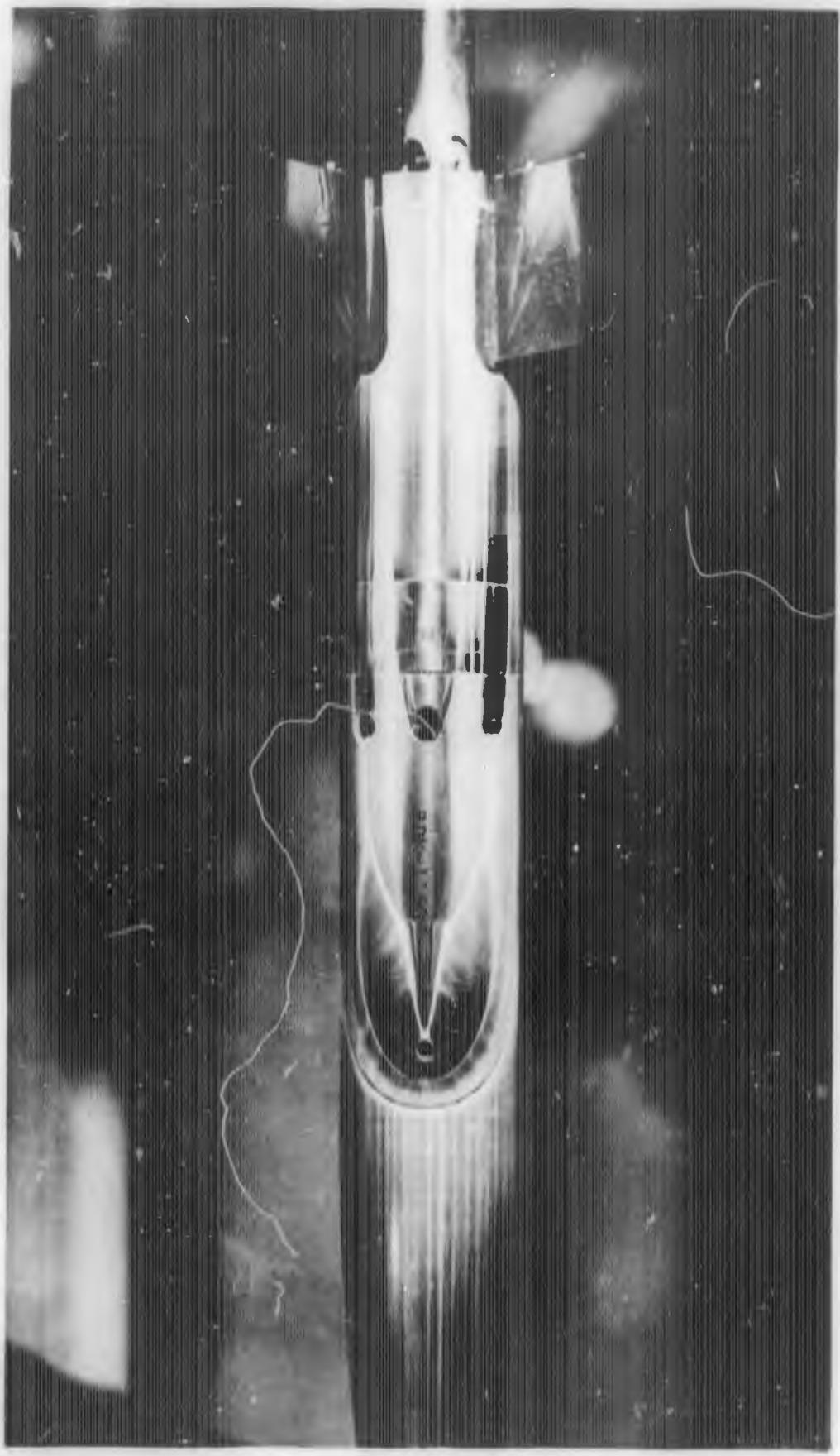
FIGURE A-1b. REACTION JET FOR  $B_1C_1X_2$  WITH  $\alpha = 0$  DEGREES;  $P_{0j}/P_\infty = 40$
