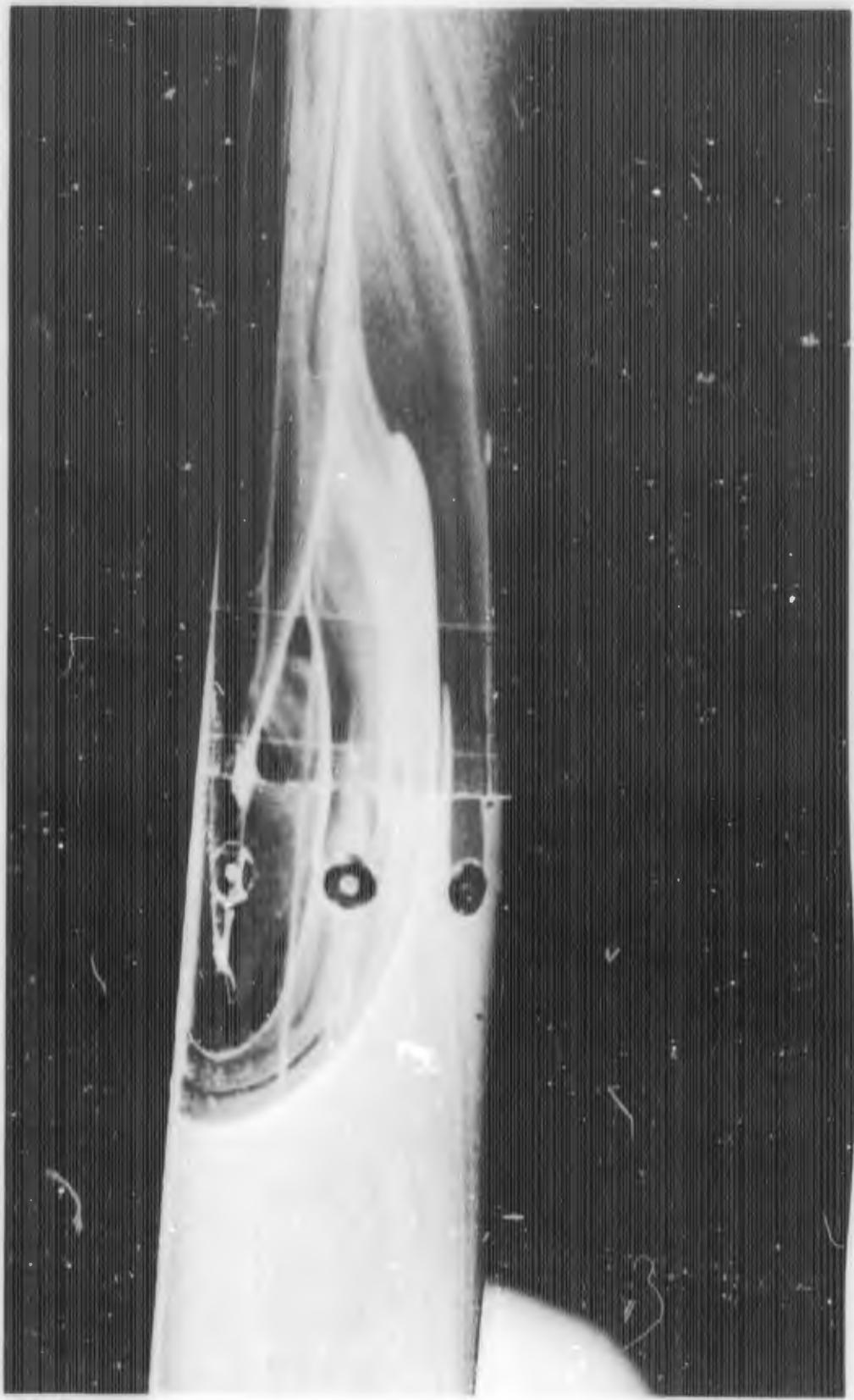
FIGURE C-7h. REACTION JET FOR  $BC_1X_3$  WITH  $\alpha = 5$  DEGREES;  $P_{0j}/P_\infty = 100$
