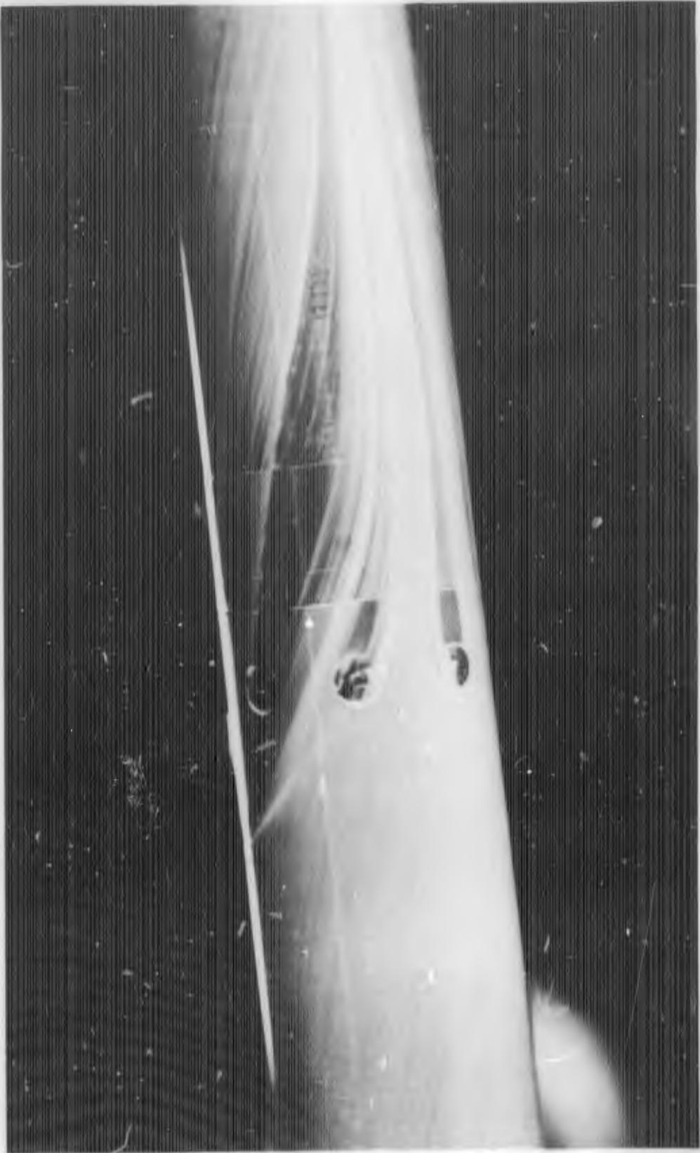
FIGURE D-4h. REACTION JET FOR  $B_1C_1X_3$  WITH  $\alpha = -5$  DEGREES;  $P_{0j}/P_{\infty} = 100$
