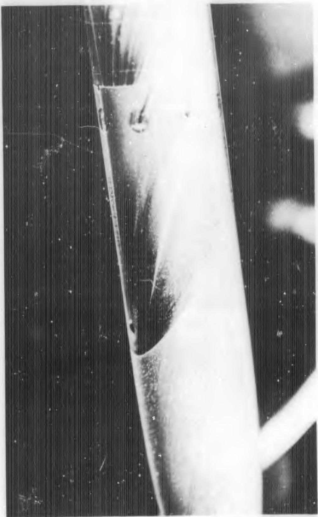
FIGURE E-13b. REACTION JET FOR B<sub>1</sub>C<sub>1</sub>X<sub>2</sub> WITH  $\alpha = -10$  DEGREES;  $P_{0j}/P_{\infty} = 100$
