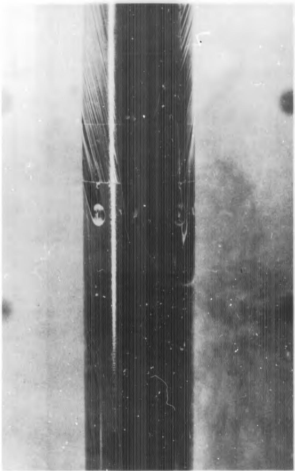
FIGURE D-10g. REACTION JET FOR  $B_1C_1X_3$  WITH  $\alpha = -10$  DEGREES;  $P_{obj}/P_\infty = 100$
