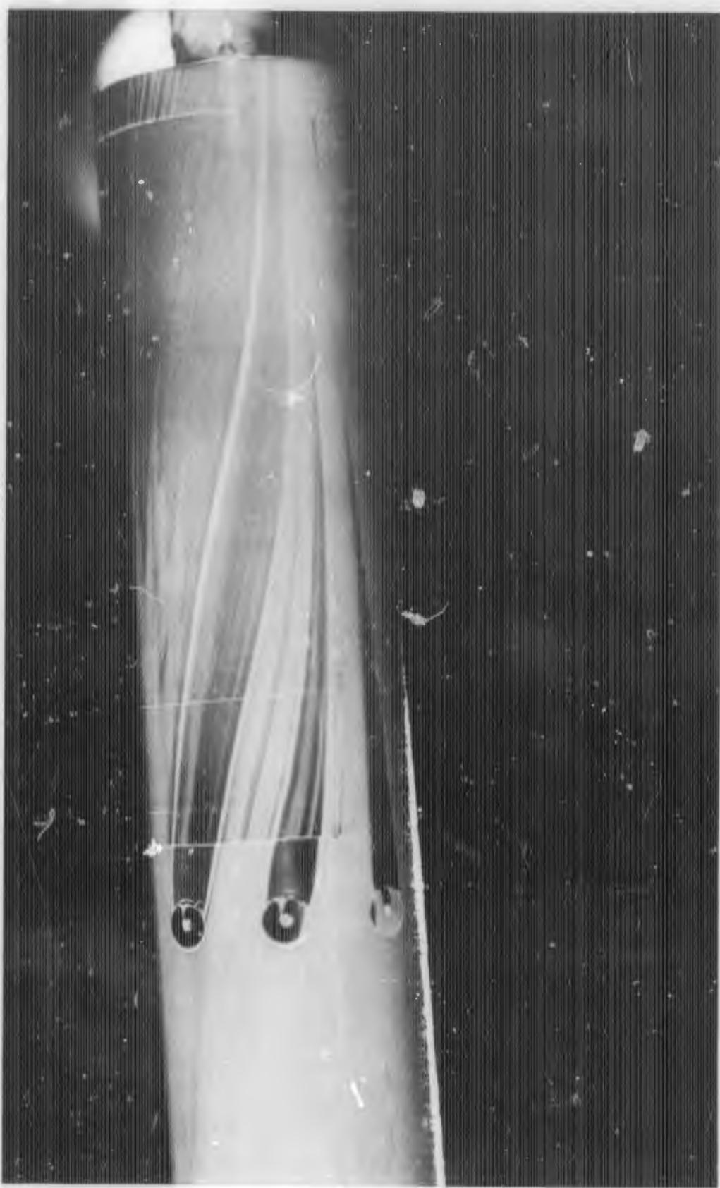
FIGURE C-2b. REACTION JET FOR B<sub>1</sub>C<sub>1</sub>X<sub>3</sub> WITH  $\alpha = 5$  DEGREES;  $P_{0j}/P_{\infty} = 0$
