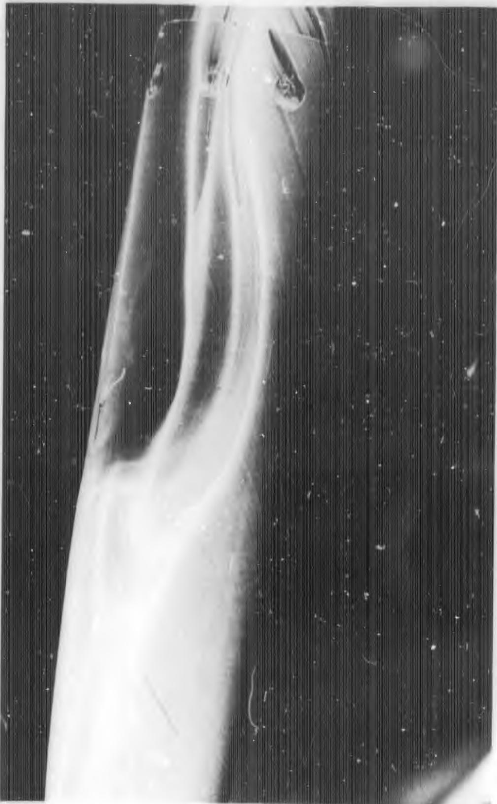
FIGURE E-17d. REACTION JET FOR  $B_1S_1LX_2$  WITH  $\alpha = 10$  DEGREES;  $P_{obj}/P_\infty = 100$
