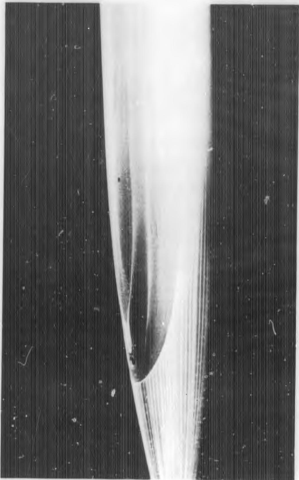
FIGURE E-1f. REACTION JET FOR  $B_1C_1X_0$  WITH  $\alpha = 0$  DEGREES;  $P_{obj}/P_\infty = 100$
