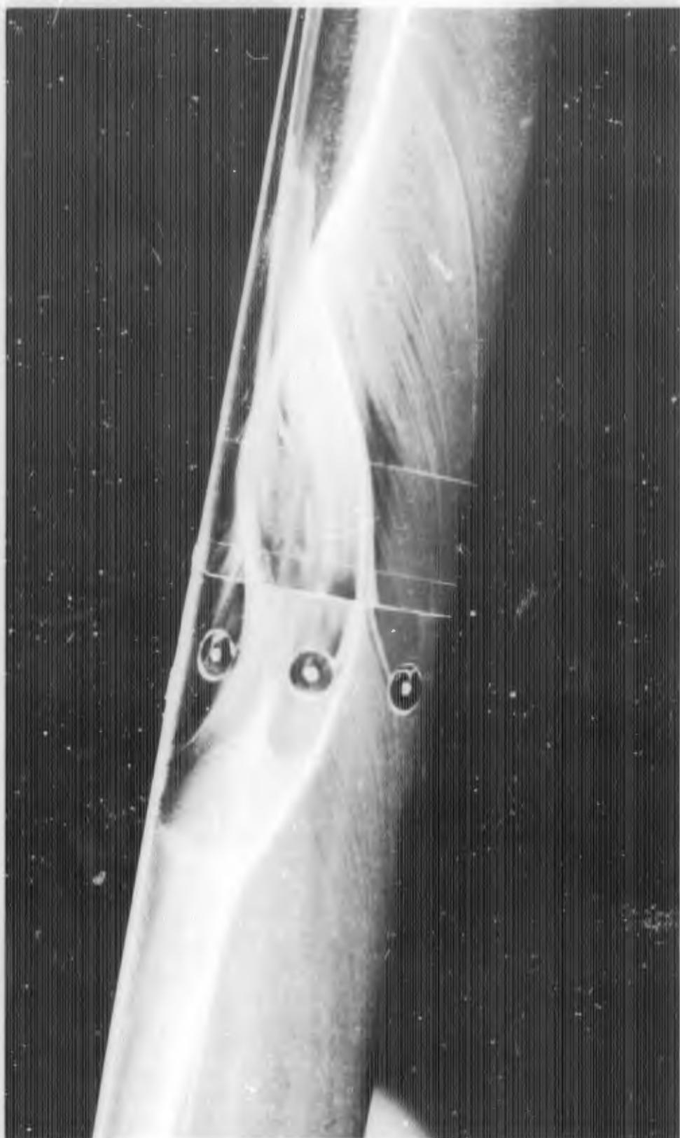
FIGURE C-3h. REACTION JET FOR  $B_1C_1X_3$  WITH  $\alpha = 10$  DEGREES;  $P_{0j}/P_\infty = 100$
