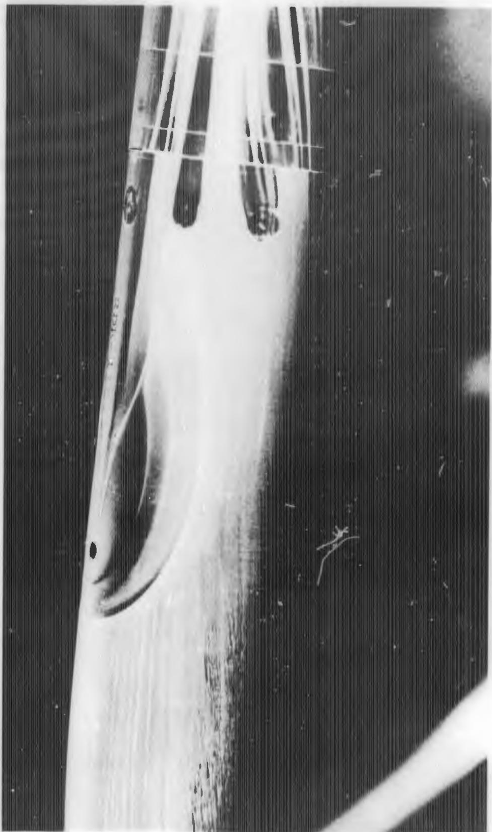
FIGURE B-2b. REACTION JET FOR  $B_1C_1X_2$  WITH  $\alpha = 5$  DEGREES;  $P_{obj}/P_\infty = 40$
