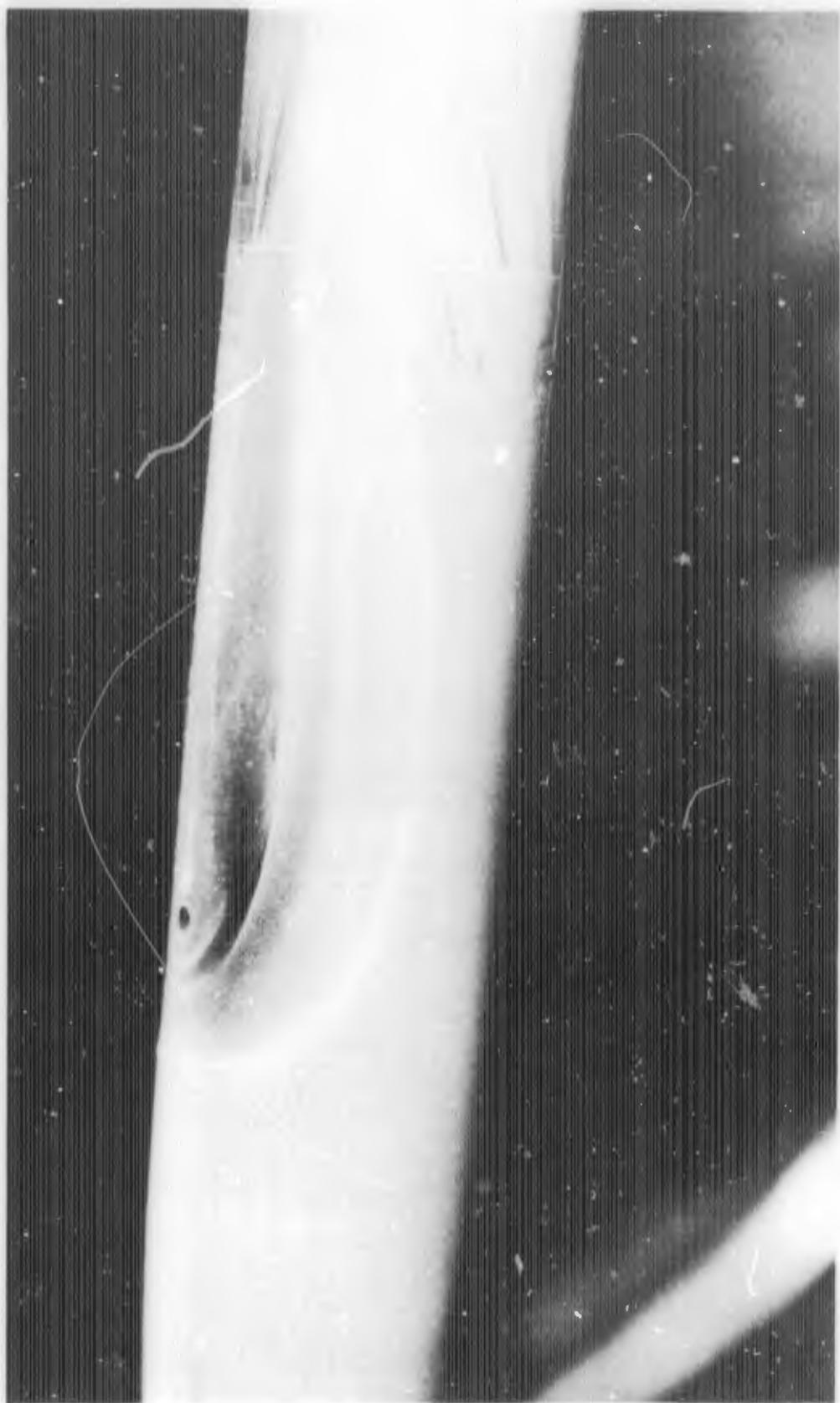
FIGURE E-10b. REACTION JET FOR  $B_1C_1X_2$  WITH  $\alpha = 5$  DEGREES;  $P_{0j}/P_\infty = 100$
