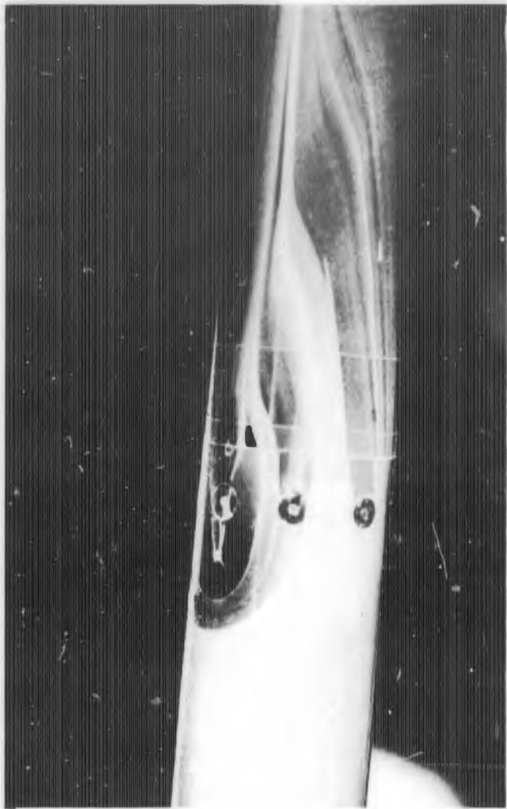
FIGURE C-7f. REACTION JET FOR  $\text{BC}_1\text{C}_1\text{N}_3$  WITH  $\alpha = 5$  DEGREES;  $P_{0j}/P_\infty = 40$
