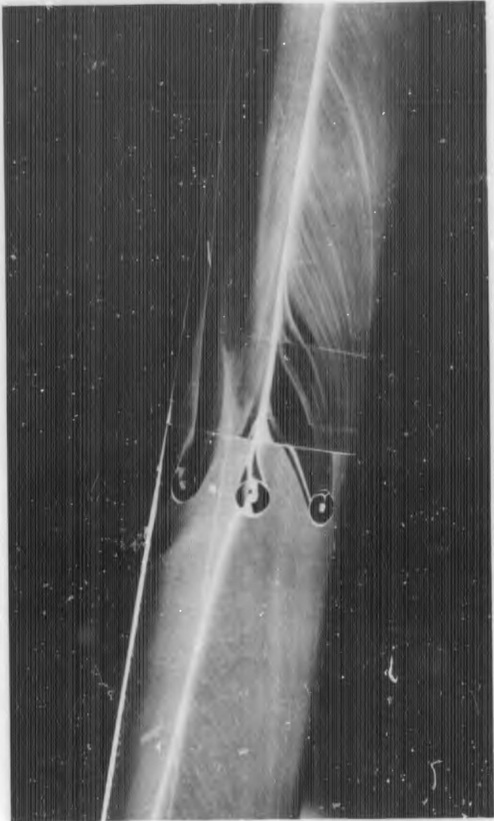
FIGURE C-3d. REACTION JET FOR  $B_1C_1X_3$  WITH  $\alpha = 10$  DEGREES;  $P_{0j}/P_\infty = 10$
