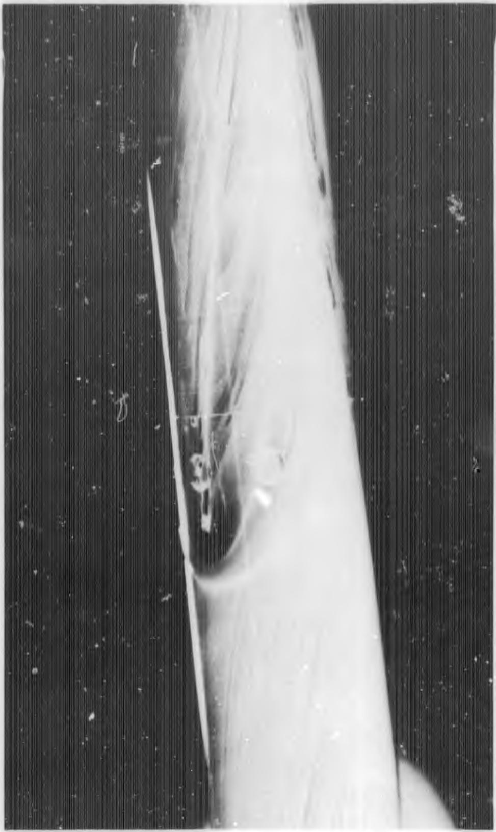
FIGURE D-9f. REACTION JET FOR B<sub>1</sub>C<sub>1</sub>X<sub>3</sub> WITH  $\alpha = -5$  DEGREES;  $P_{\text{obj}}/P_{\infty} = 40$
