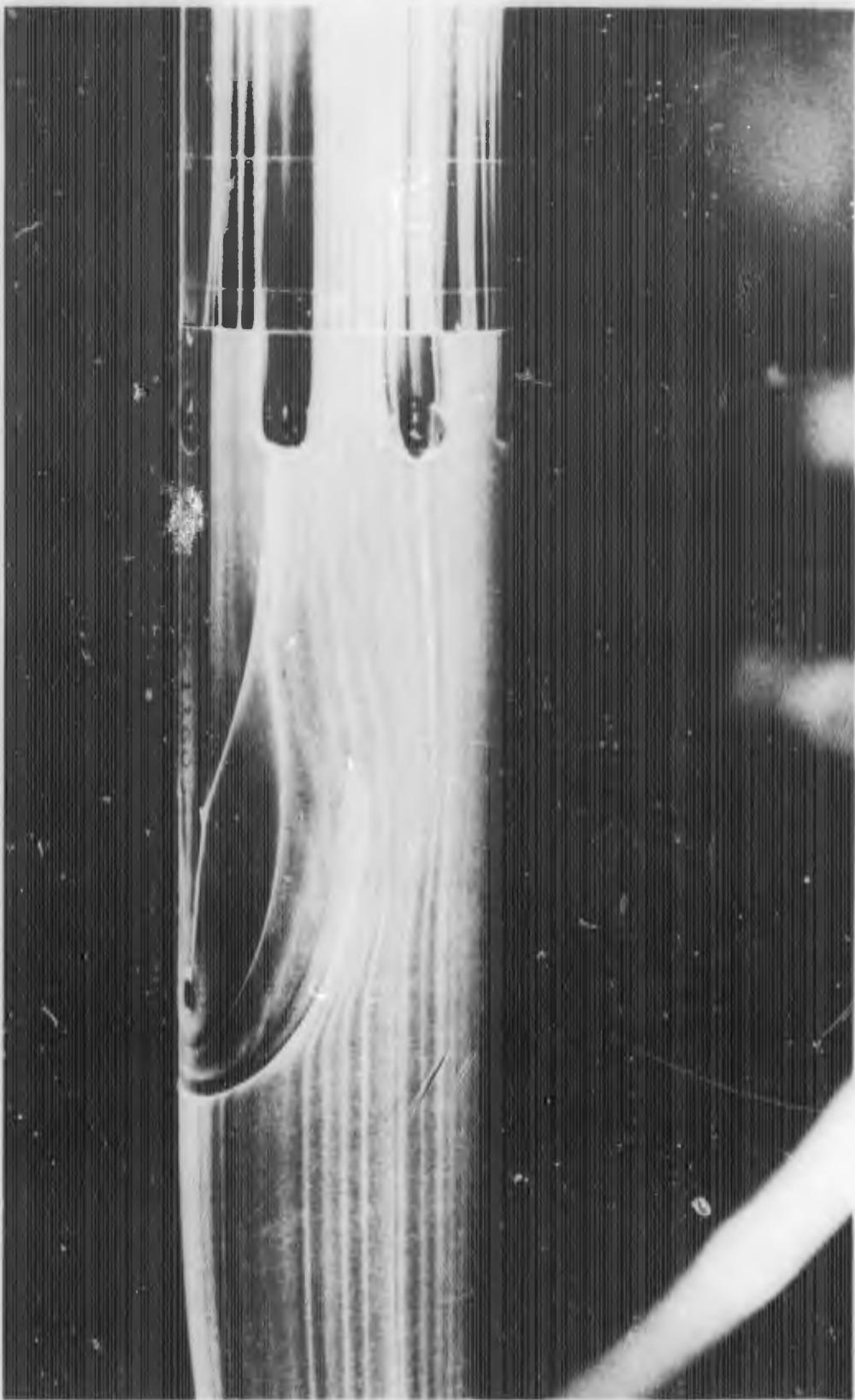
FIGURE B-1d. REACTION JET FOR B<sub>1</sub>C<sub>1</sub>X<sub>2</sub> WITH  $\alpha = 0$  DEGREES;  $P_{0j}/P_{\infty} = 40$
