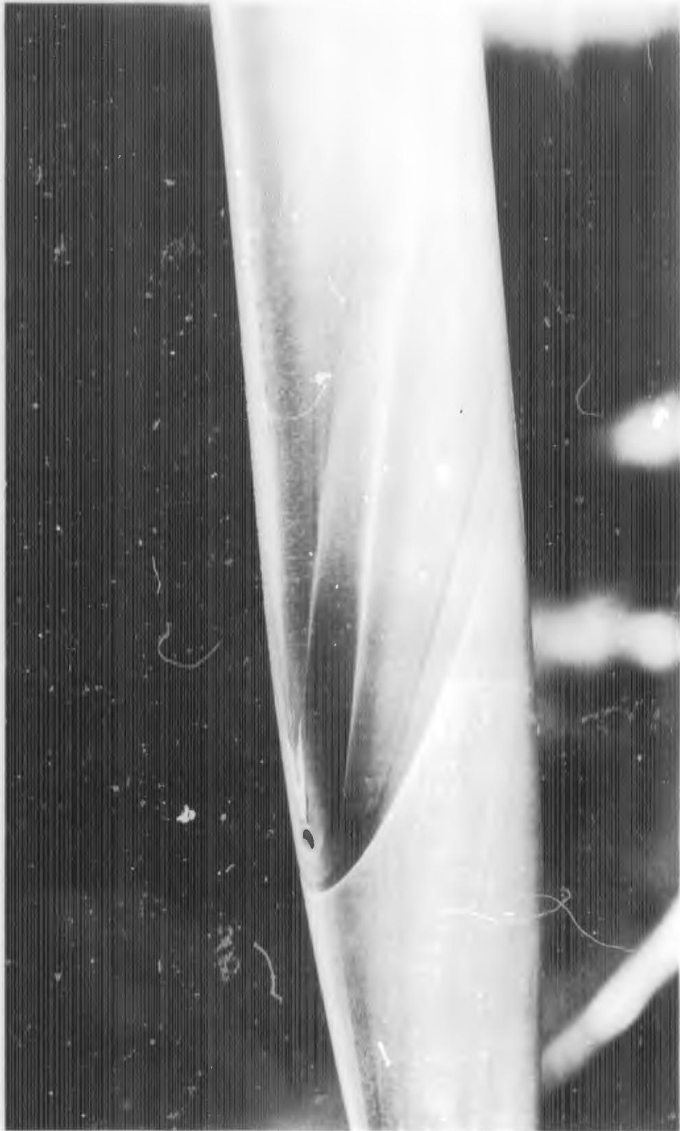
FIGURE E-7b. REACTION JET FOR  $B_1C_1X_1$  WITH  $\alpha = -5$  DEGREES;  $P_{obj}/P_\infty = 100$
