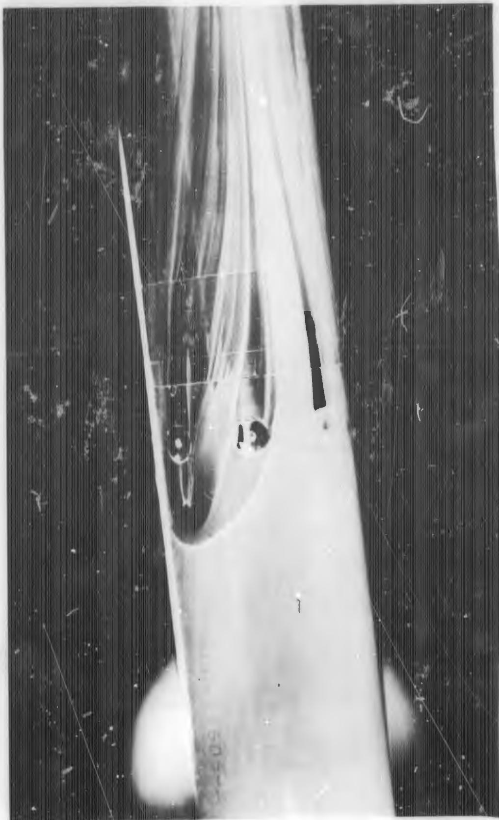
FIGURE C-9c. REACTION JET FOR  $B_1C_1N_3$  WITH  $\alpha = -5$  DEGREES;  $P_{0j}/P_\infty = 10$
