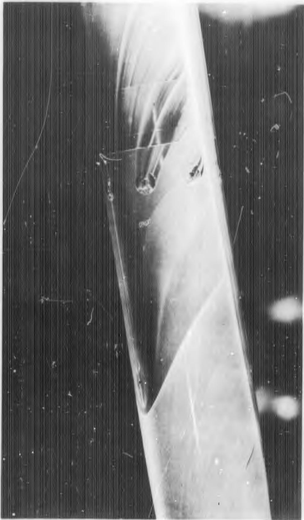
FIGURE E-19a. REACTION JET FOR B<sub>1</sub>S<sub>1</sub>LX<sub>2</sub> WITH  $\alpha = -10$  DEGREES;  $P_{oj}/P_{\infty} = 40$
