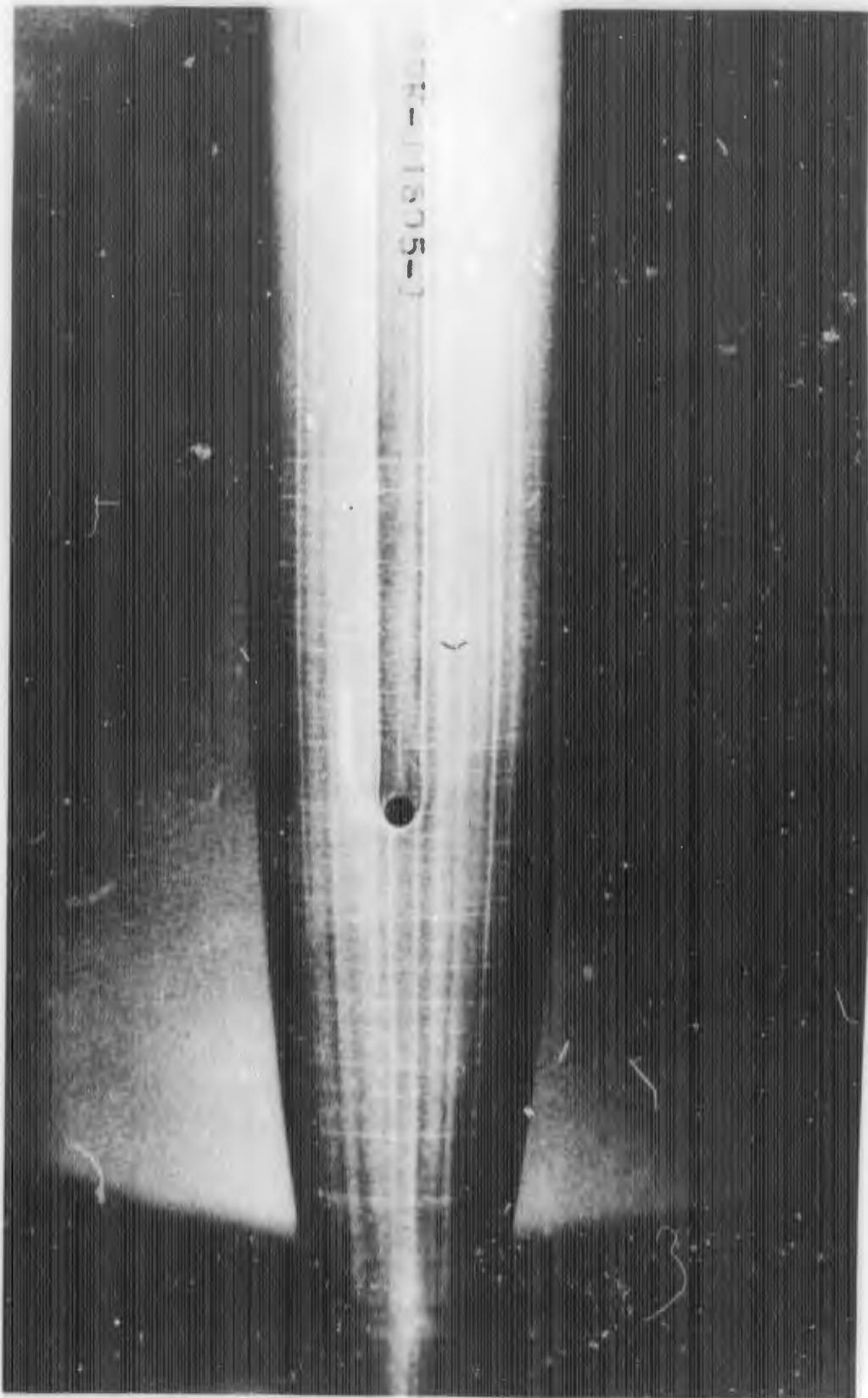
FIGURE B-6a. REACTION JET FOR  $B_1C_1X_1$  WITH  $\alpha = 0$  DEGREES;  $P_{0j}/P_\infty = 0$
