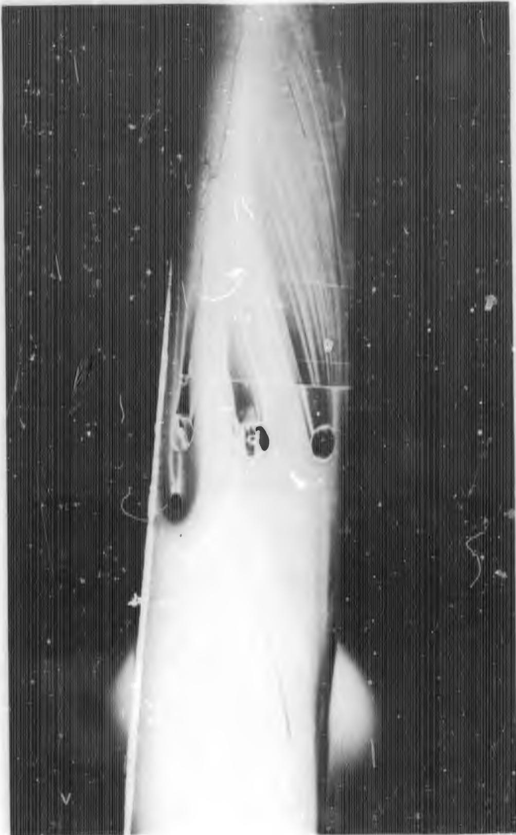
FIGURE D-7d. REACTION JET FOR  $B_1C_1X_3$  WITH  $\alpha = 5$  DEGREES;  $P_{0j}/P_\infty = 10$
