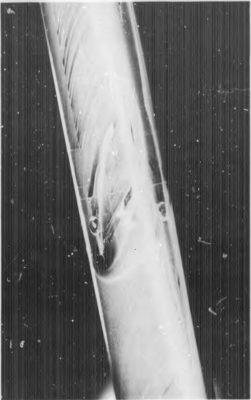
FIGURE D-10f. REACTION JET FOR B<sub>1</sub>C<sub>1</sub>X<sub>3</sub> WITH  $\alpha = -10$  DEGREES;  $P_{0j}/P_{\infty} = 40$
