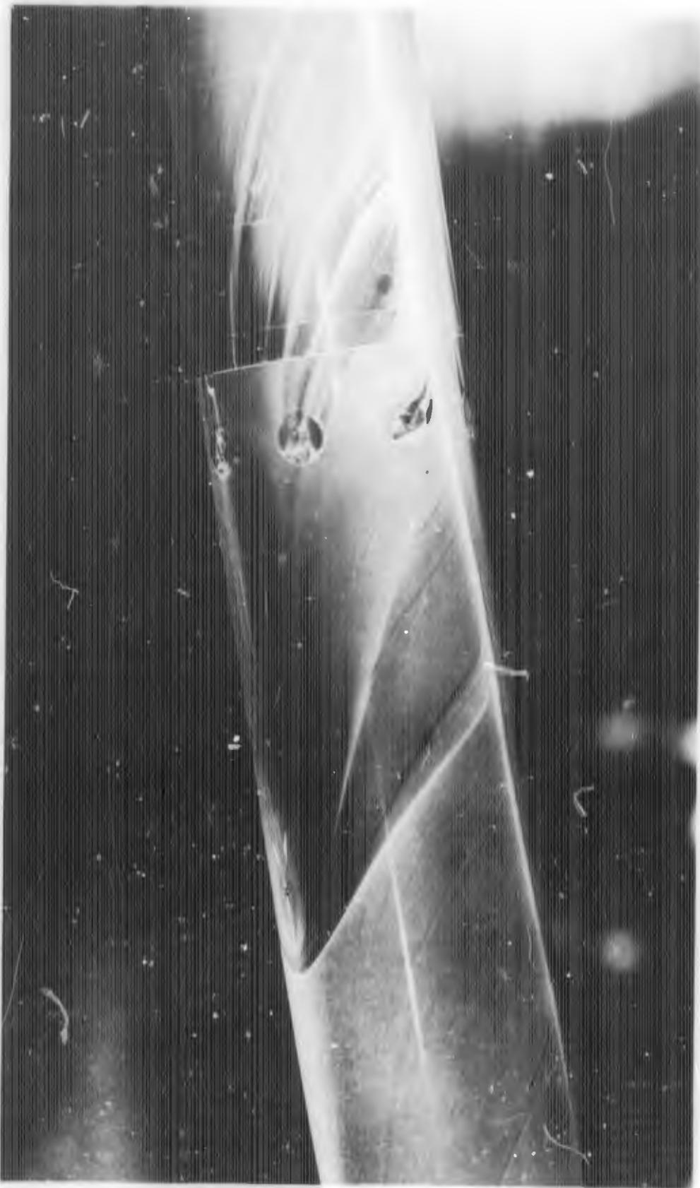
FIGURE E-19b. REACTION JET FOR  $B_1S_1LX_2$  WITH  $\alpha = -10$  DEGREES;  $P_{obj}/P_\infty = 100$
