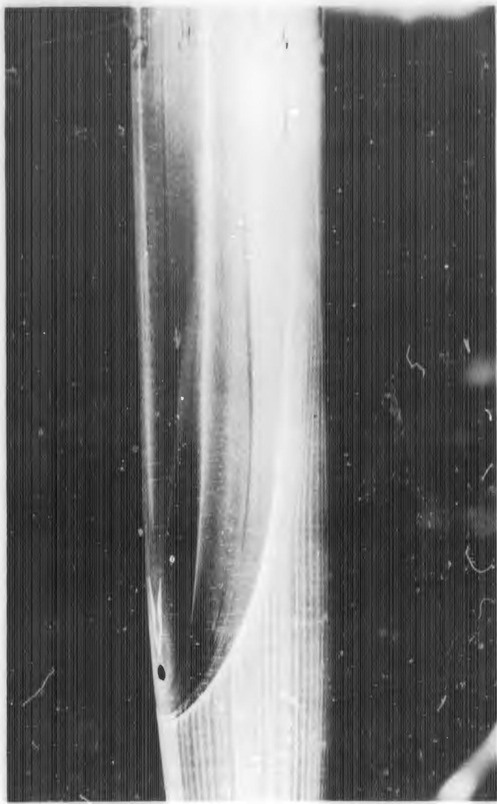
FIGURE E-4f. REACTION JET FOR  $B_1C_1X_1$  WITH  $\alpha = 0$  DEGREES;  $P_{\alpha}/P_{\infty} = 100$
