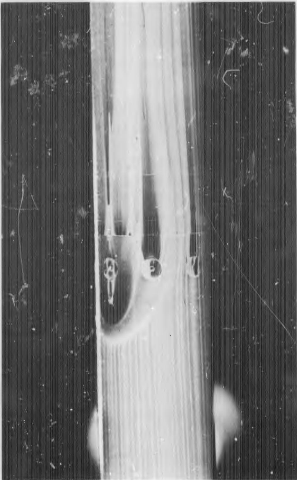
FIGURE D-6e. REACTION JET FOR  $B_1C_1X_3$  WITH  $\alpha = 0$  DEGREES;  $P_{0j}/P_\infty = 40$
