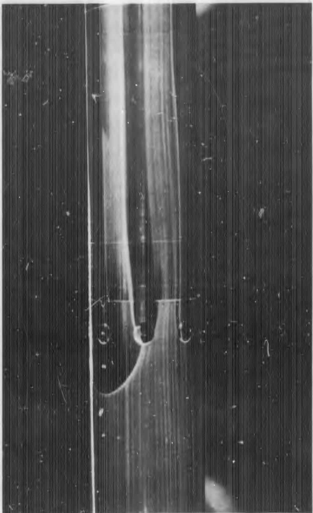
FIGURE C-6d. REACTION JET FOR  $B_1C_1X_3$  WITH  $\alpha = 0$  DEGREES;  $P_{0j}/P_\infty = 10$
