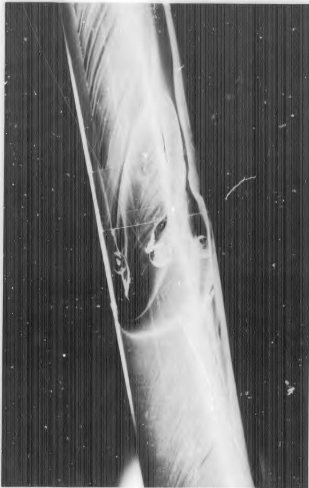
FIGURE D-10h. REACTION JET FOR  $B_1C_1X_3$  WITH  $\alpha = -10$  DEGREES;  $P_{obj}/P_\infty = 100$
