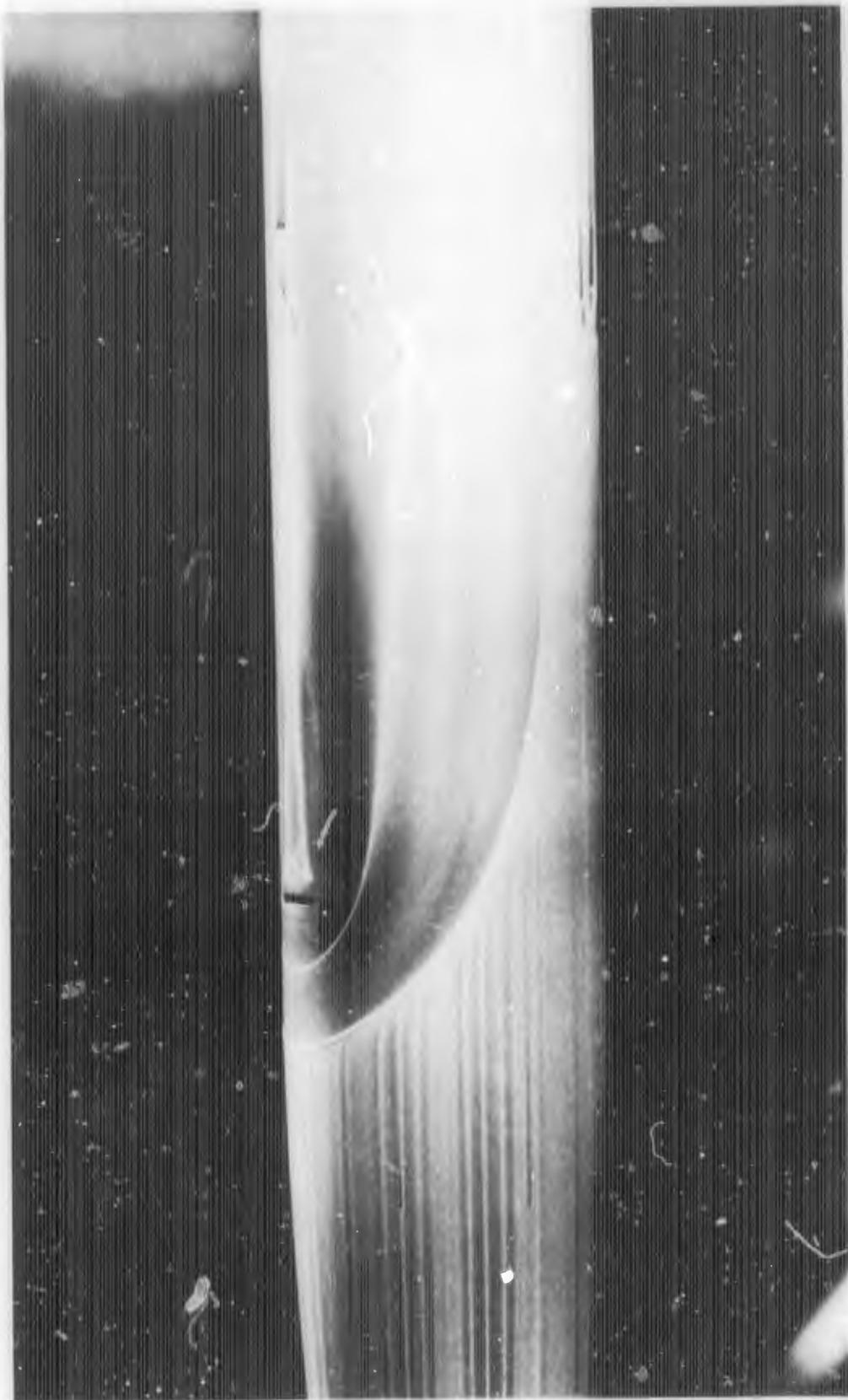
FIGURE E-20f. REACTION JET FOR  $E_1 S_1 T X_2$  WITH  $\alpha = 0$  DEGREES;  $P_{obj}/P_\infty = 100$
