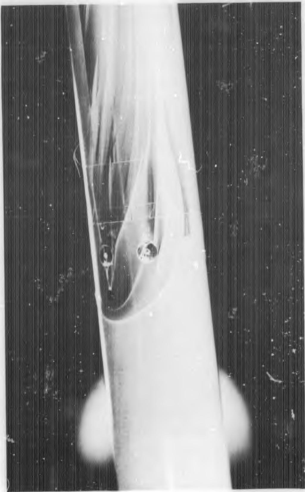
FIGURE C-9e. REACTION JET FOR  $B_1C_1X_3$  WITH  $\alpha = -5$  DEGREES;  $P_{obj}/P_\infty = 40$
