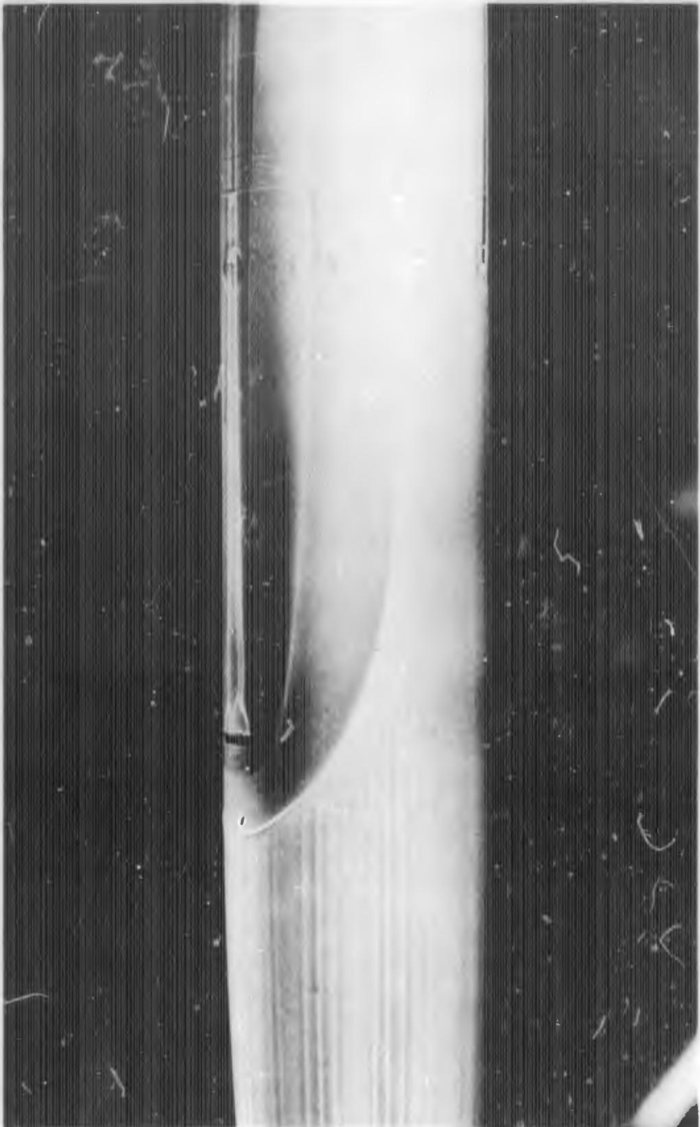
FIGURE E-20d. REACTION JET FOR  $B_1S_1T X_2$  WITH  $\alpha = 0$  DEGREES;  $P_{0j}/P_\infty = 40$
