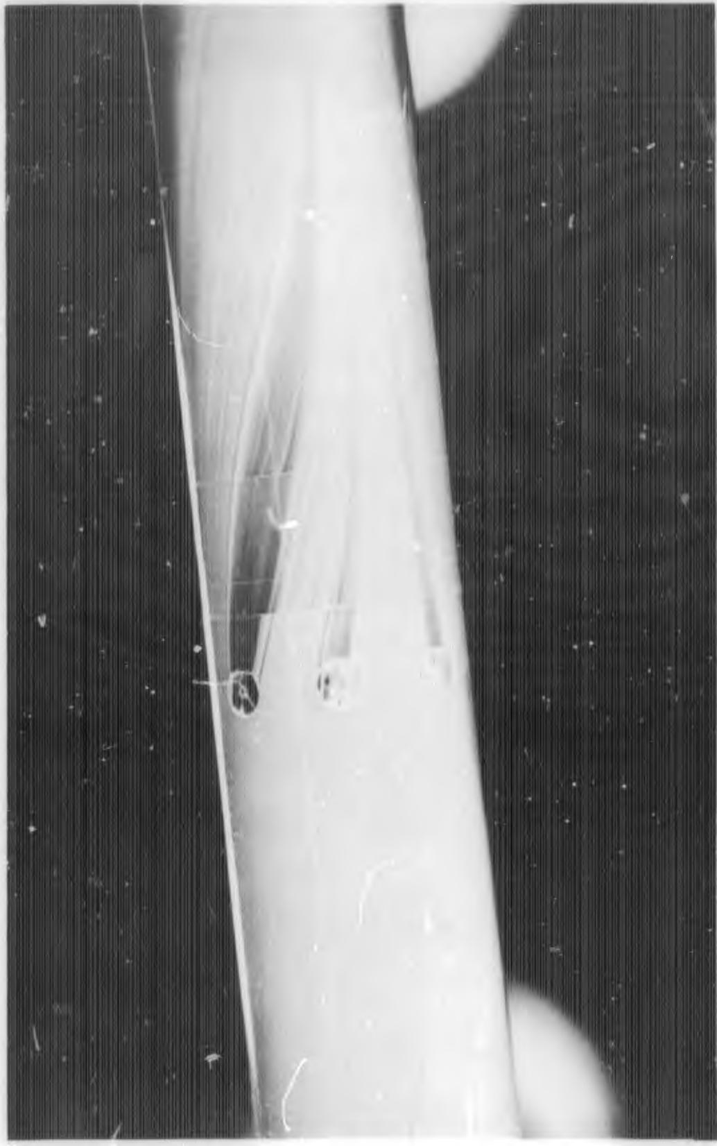
FIGURE D-4b. REACTION JET FOR  $B_1C_1X_3$  WITH  $\alpha = -5$  DEGREES;  $P_{\text{obj}}/P_{\infty} = 0$
