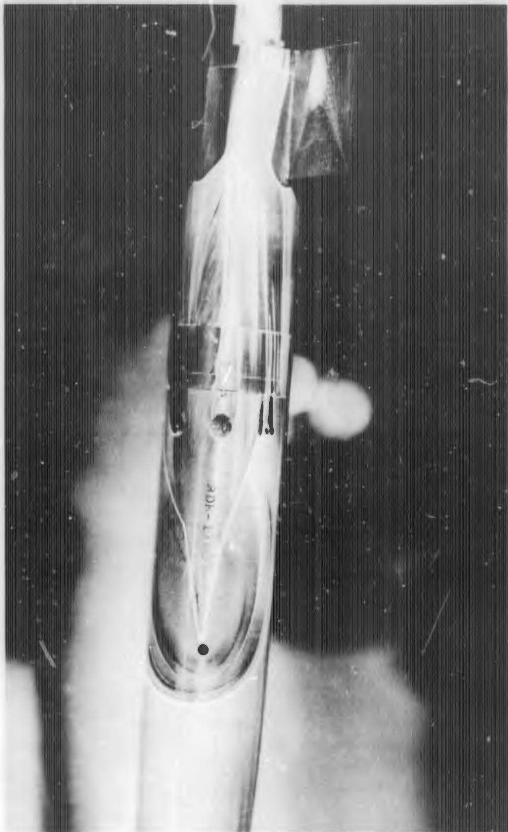
FIGURE A-2c. REACTION JET FOR  $B_1C_1X_2$  WITH  $\alpha = 5$  DEGREES;  $P_{0j}/P_\infty = 100$
