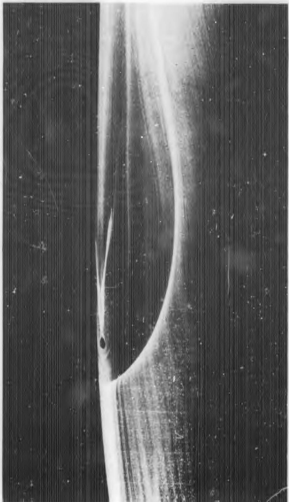
FIGURE E-5d. REACTION JET FOR  $B_1C_1X_1$  WITH  $\alpha = 5$  DEGREES;  $P_{0j}/P_\infty = 100$
