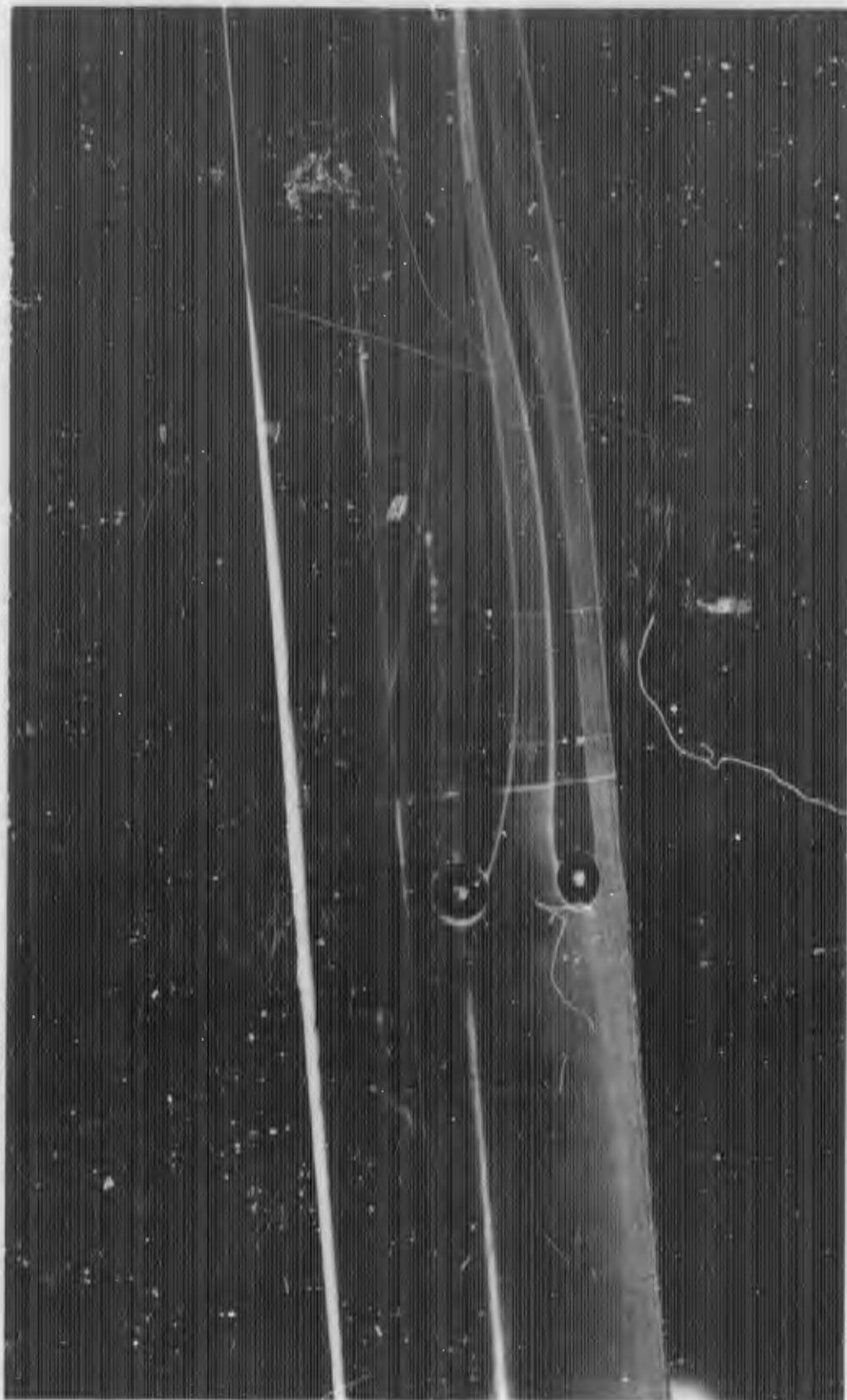
FIGURE C-4g. REACTION JET FOR  $B_1C_1X_3$  WITH  $\alpha = -5$  DEGREES;  $P_{0j}/P_\infty = 100$
