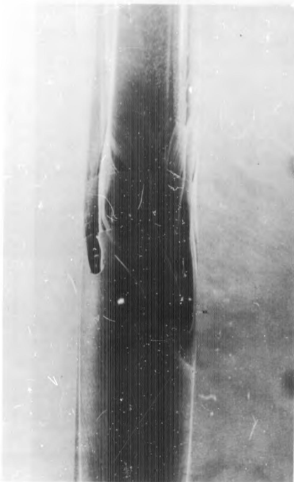
FIGURE C-8f. REACTION JET FOR  $B_1C_1N_3$  WITH  $\alpha = 10$  DEGREES;  $P_{obj}/P_\infty = 40$
