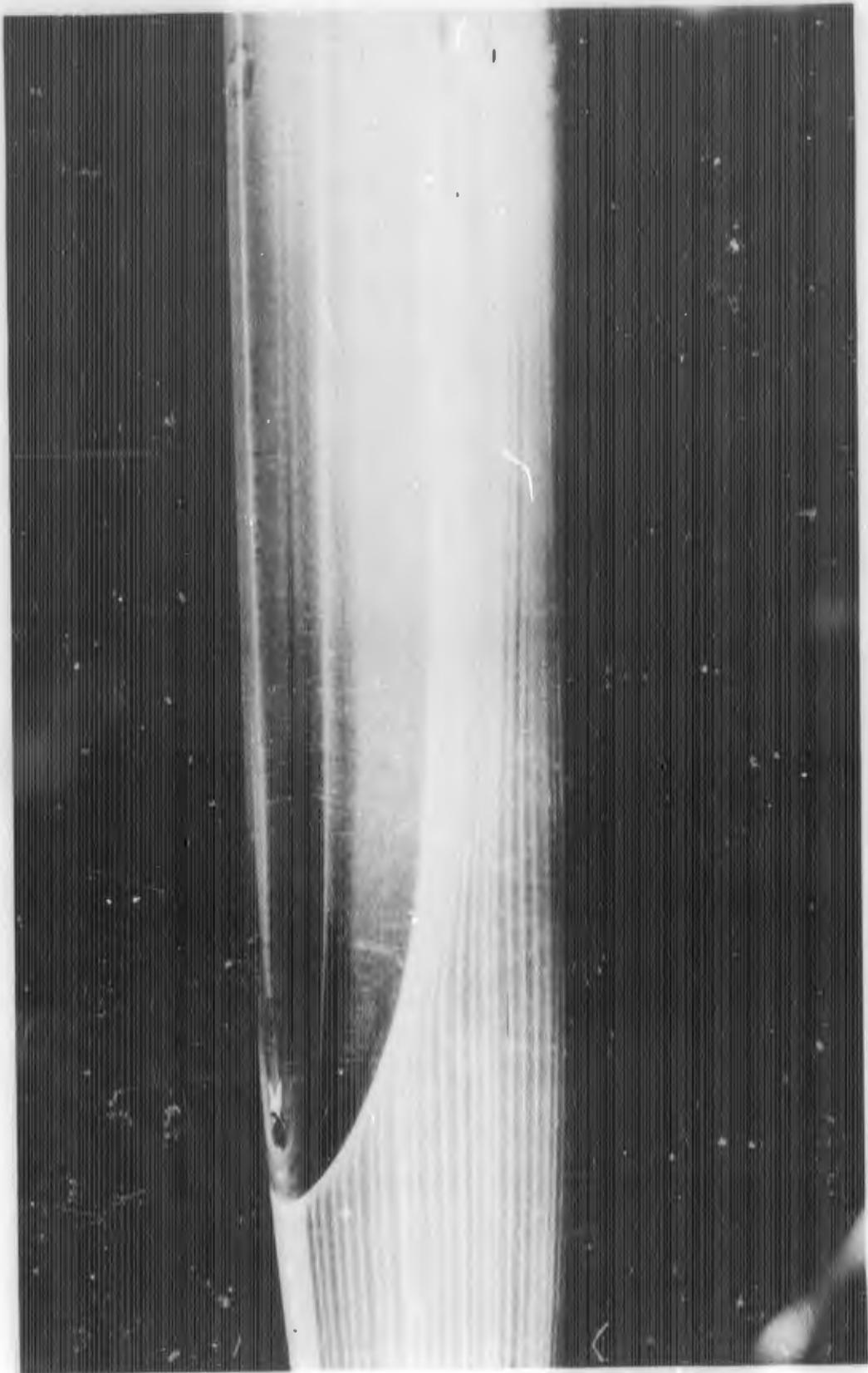
FIGURE E-4d. REACTION JET FOR  $B_1C_1X_1$  WITH  $\alpha = 0$  DEGREES;  $P_{0j}/P_\infty = 40$
