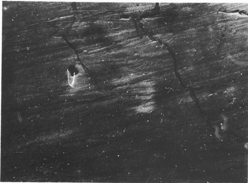
Figure 53. Surface of Sample A12, Slip in Vicinity of Crack, X9000.
