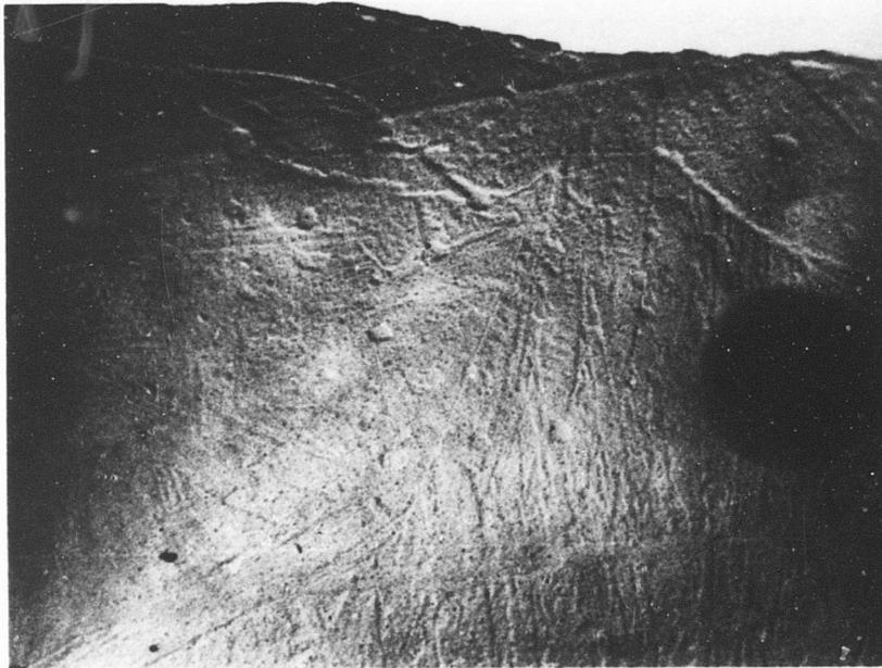
Figure 62. Sample S1, Edge of Crack at Top, No Slip Evident (Characteristic Observation for Steel Samples), X9000.
