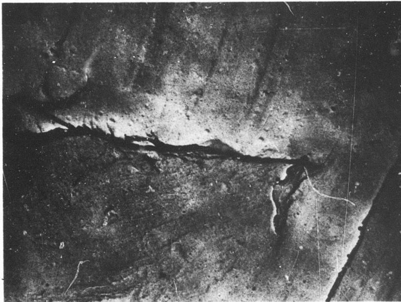
Figure 63. Sample S1, Tip of Primary Crack, No Evidence of Other Material Damage, X9000.
