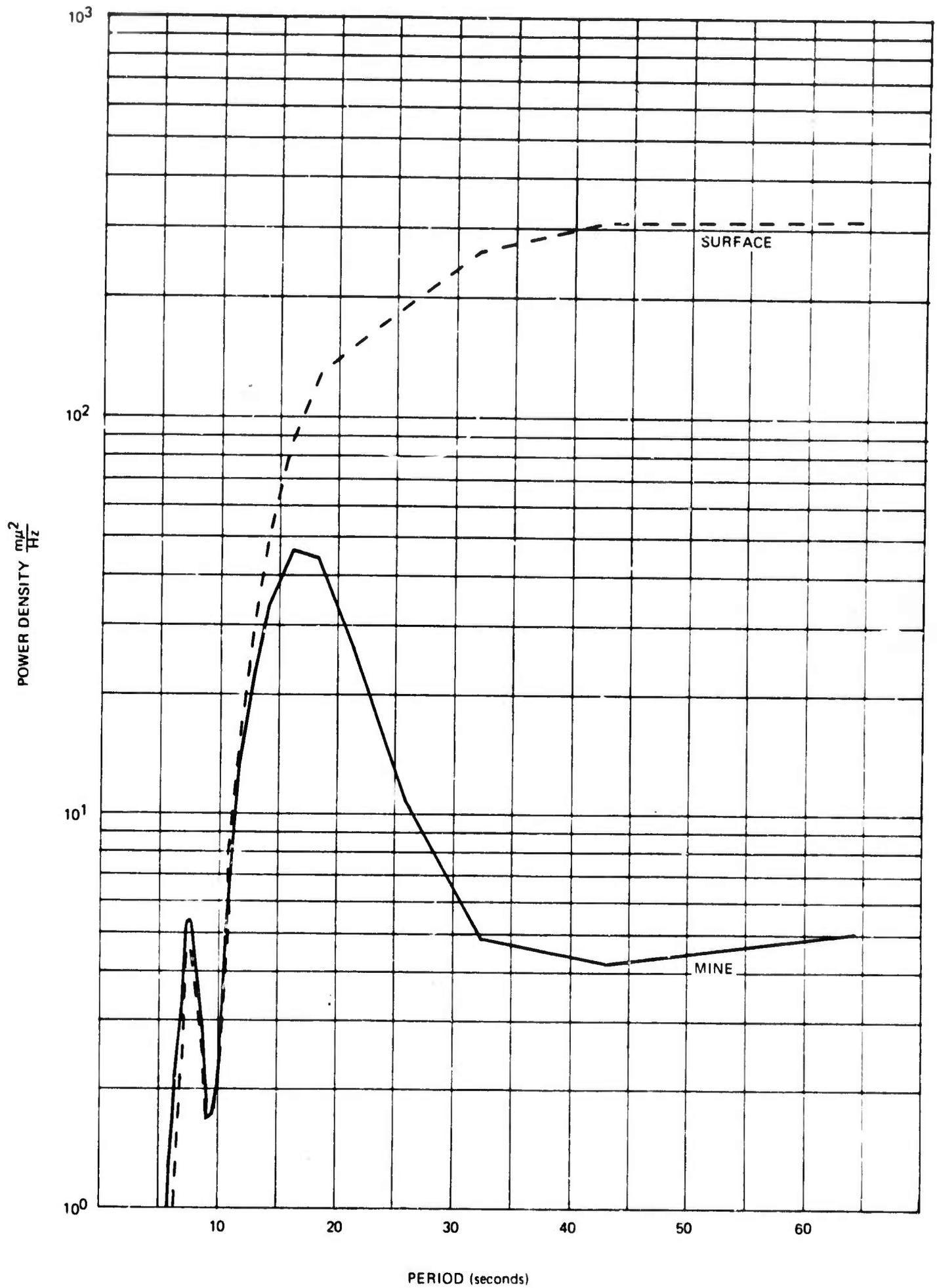
Figure 25. Example of long-period seismic noise spectra observed on vertical seismographs located at the surface and in the mine during a period of atmospheric turbulence
