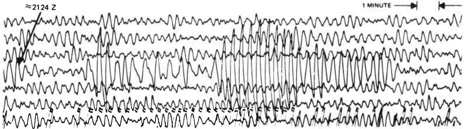
Figure 15. Reproduction of a portion of a Helicorder record showing data recorded by a long-period seismograph with a frequency response approximating the LRSM response. Magnification 167 K at 20 seconds. Recording made at Geotech facilities, Garland, Texas, 3 August 69.
