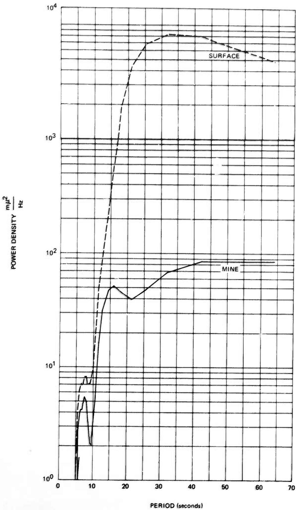
Figure 27. Example of long-period seismic noise spectra observed on horizontal seismographs located at the surface and in the mine during a period of atmospheric turbulence
