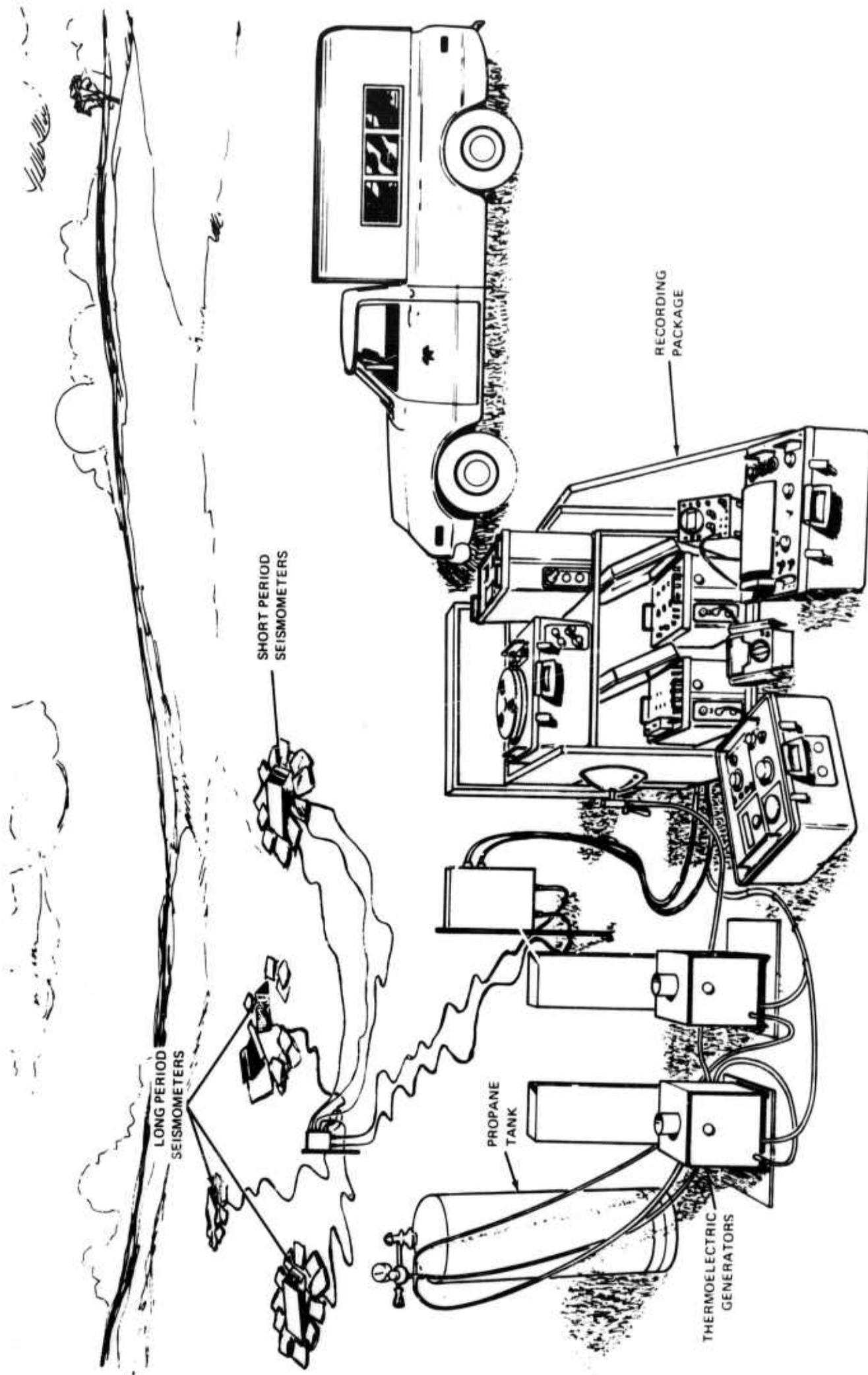
Figure 8. Portable systems site layout
