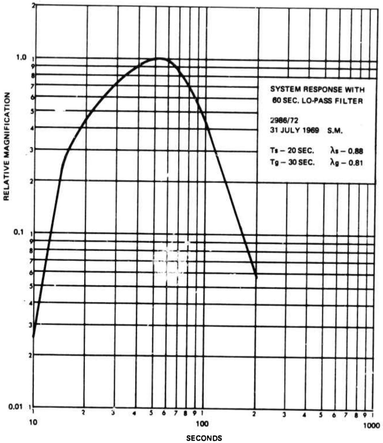
Figure 13 Extended range LP frequency response
