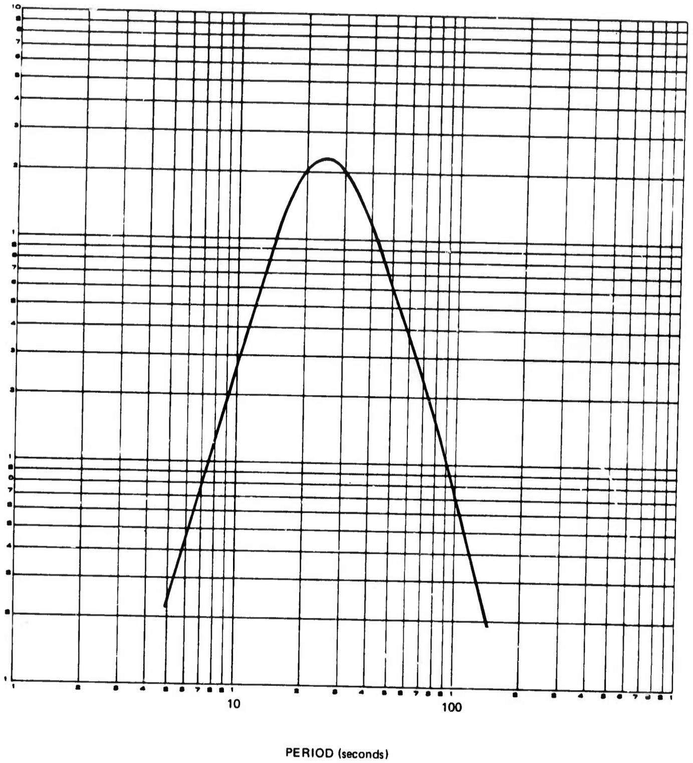
Figure 23. Frequency response of the long-period seismograph, Portable System Model 19282A
