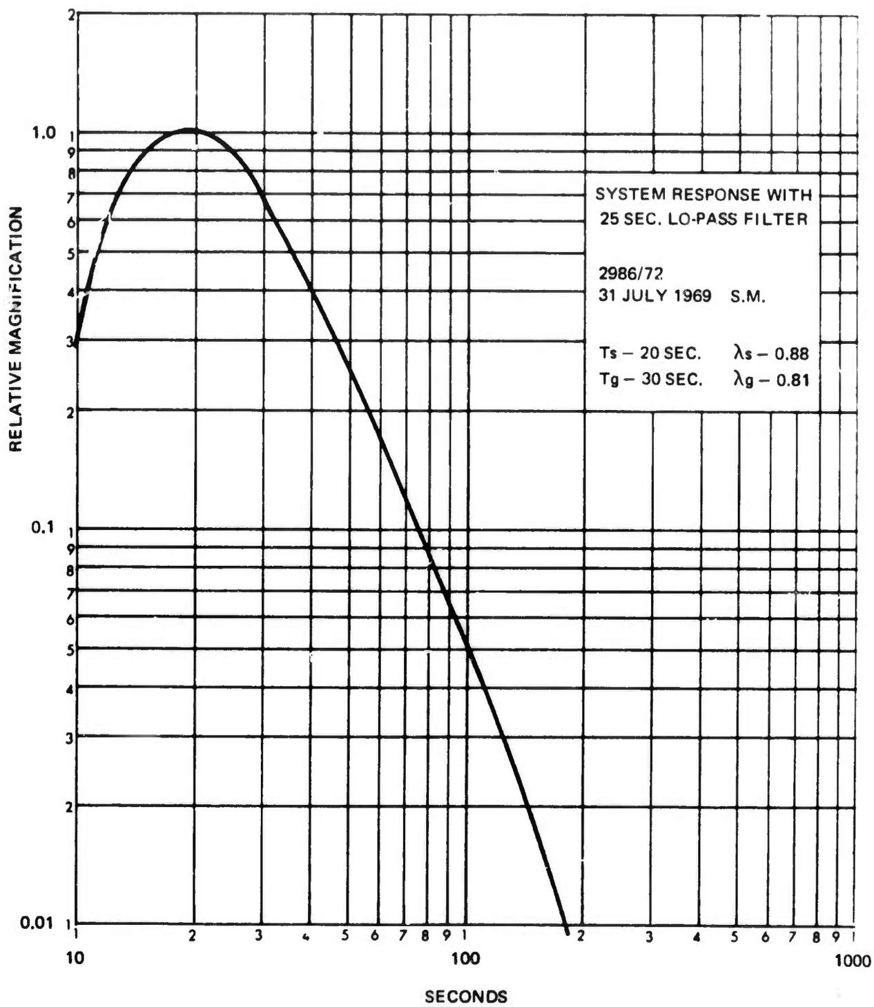
Figure 14. LP frequency response using a 25-second low-pass filter
