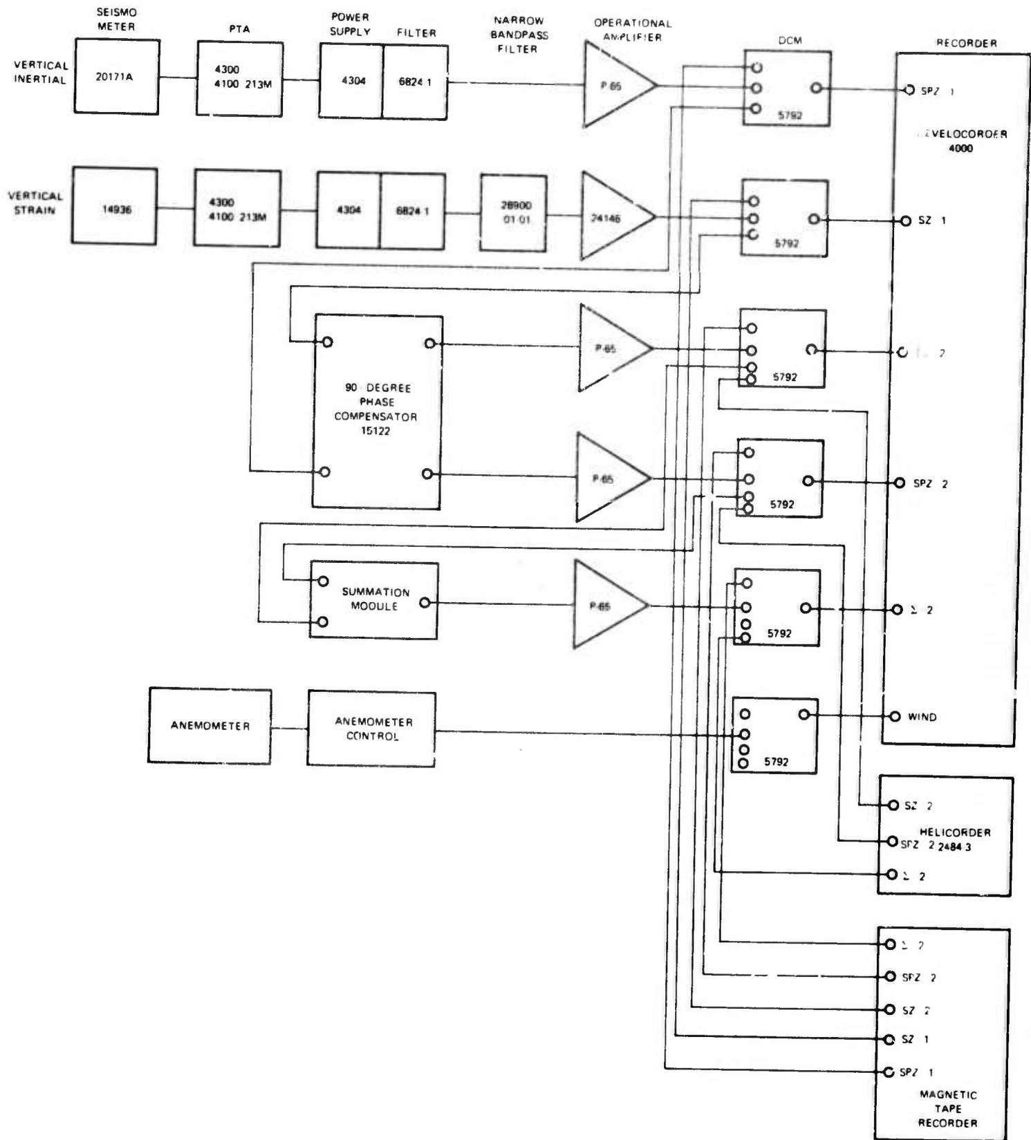
Figure 6. Block diagram of strain seismograph system at Houlton, Maine
