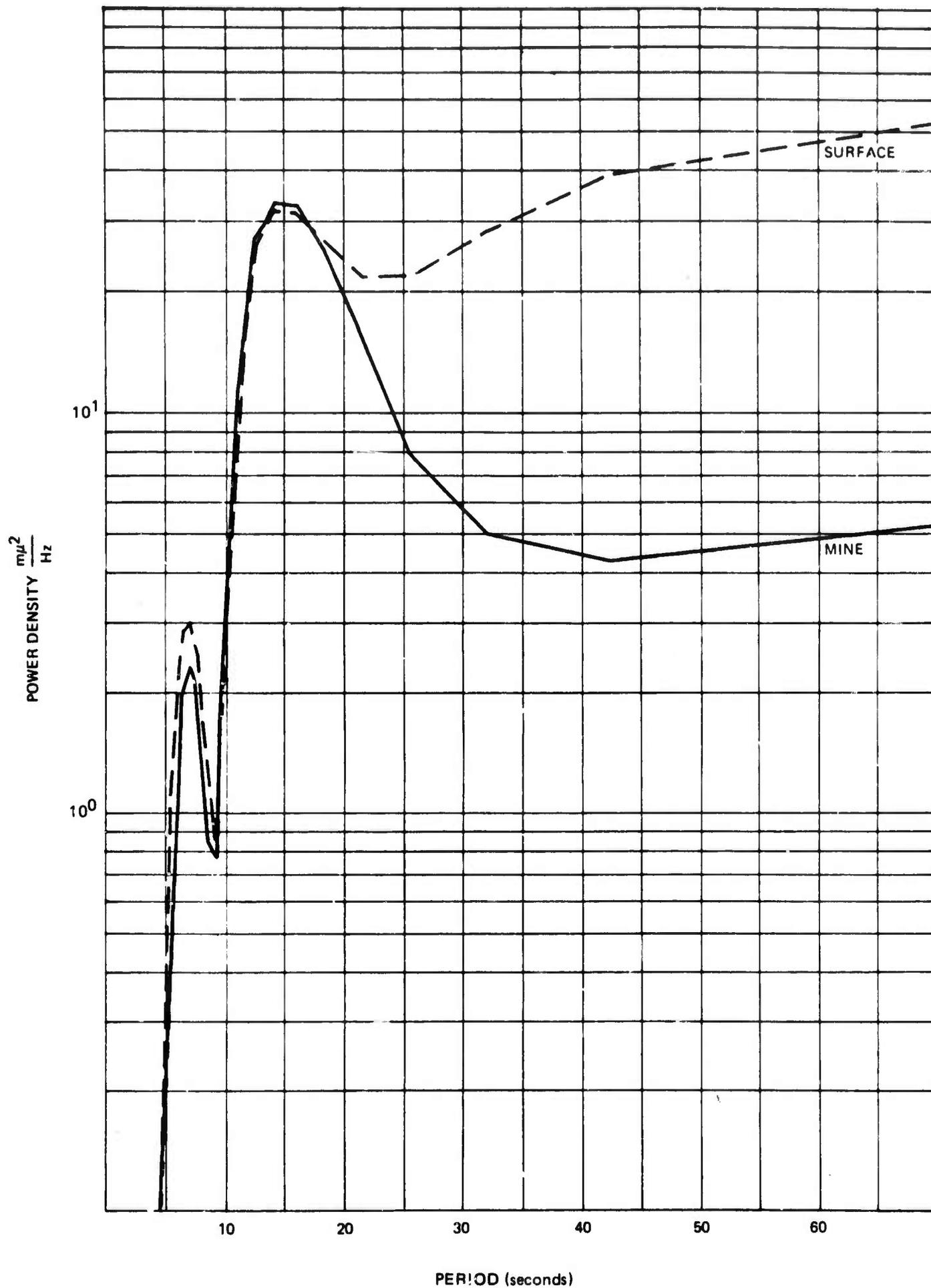
Figure 24. Example of long-period seismic noise spectra observed on vertical seismographs located at the surface and in the mine during a calm period G 5785
