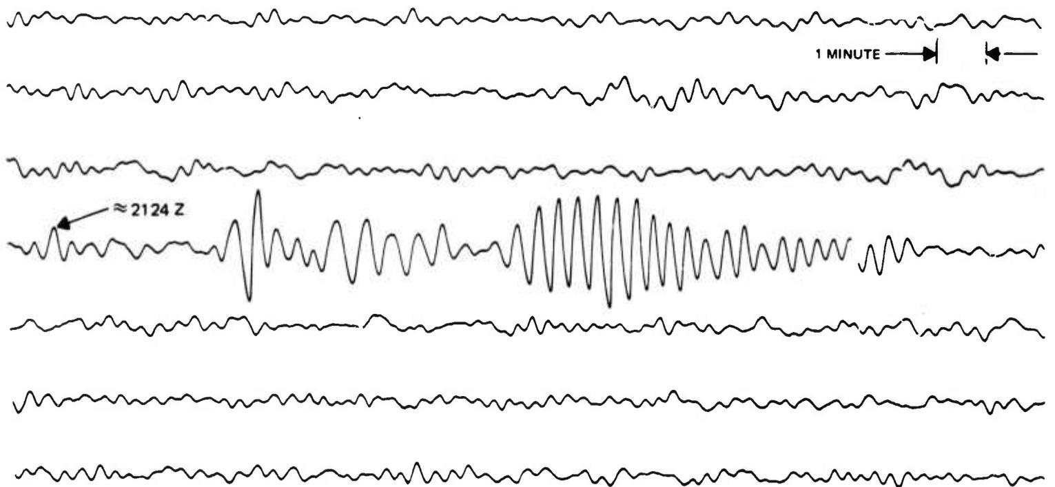
Figure 16. Reproduction of the same portion of a Helicorder record shown in figure 15, with data recorded by a long-period seismograph with a frequency response peaked at 50 seconds (magnification 100 K).
