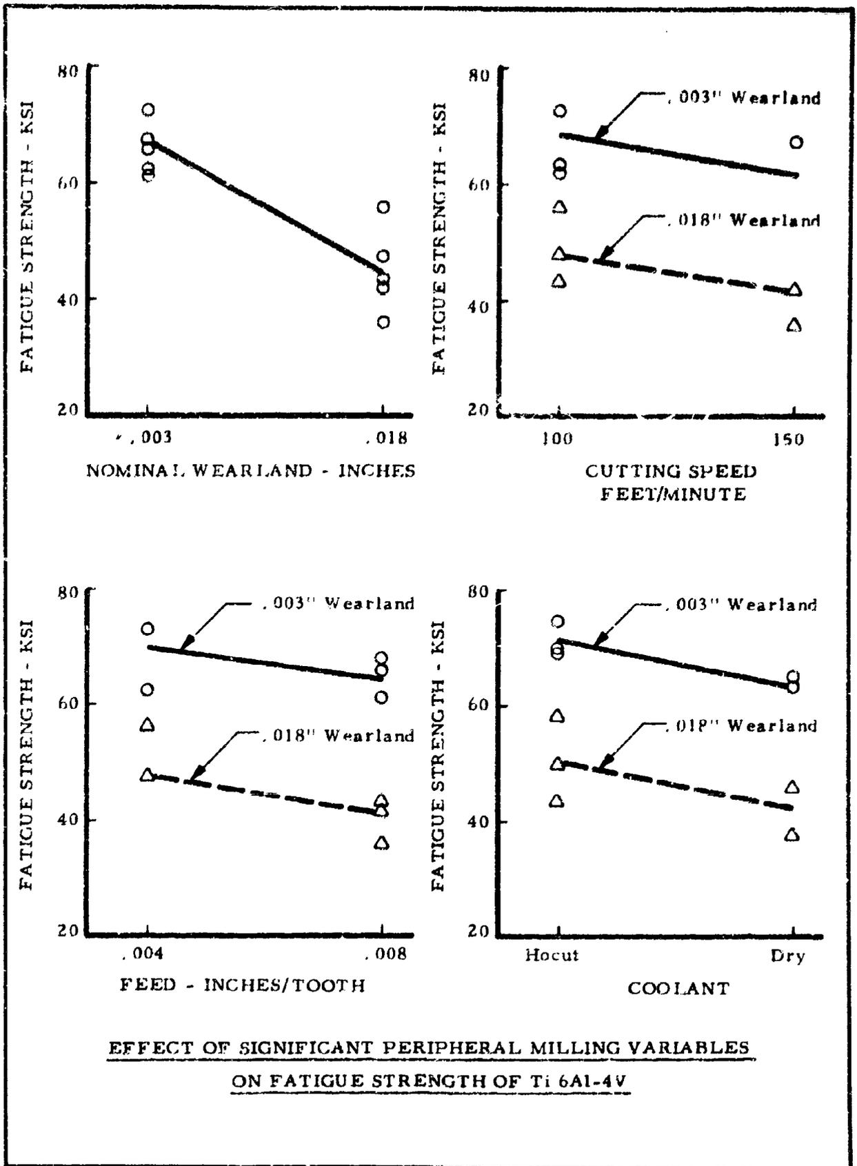
EFFECT OF SIGNIFICANT PERIPHERAL MILLING VARIABLES
