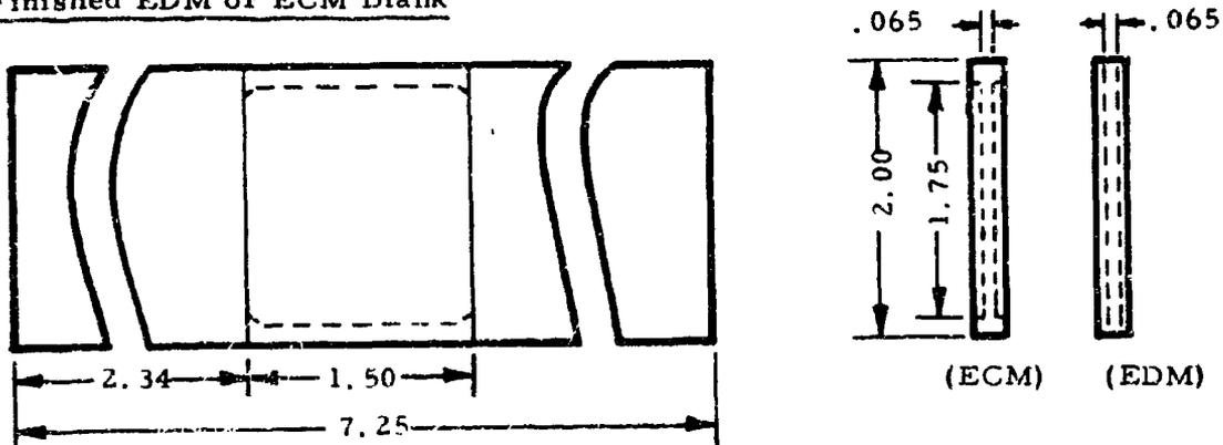
EDM cut is through-slot located as shown above.
