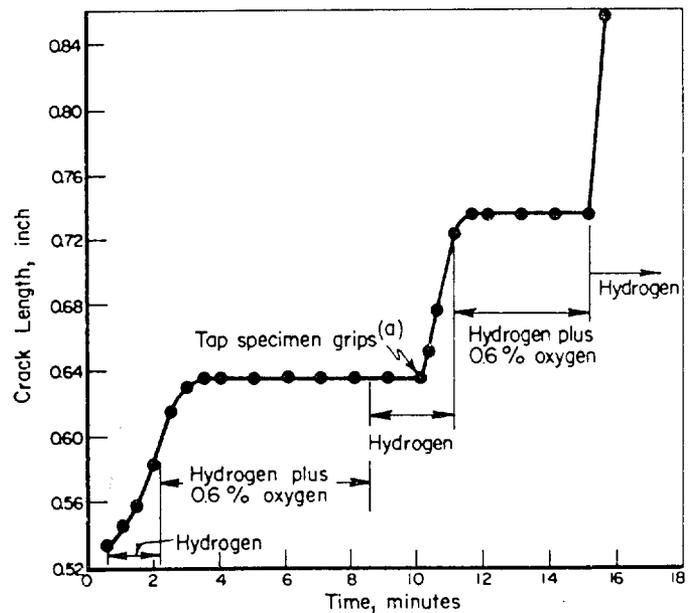
FIGURE 5. SUBCRITICAL CRACK GROWTH IN H-11 STEEL SPECIMENS IN ENVIRONMENTS OF PURE HYDROGEN AND A HYDROGEN-OXYGEN MIXTURE(12) (a) At this point, the specimen grips were tapped to initiate the reaction.
