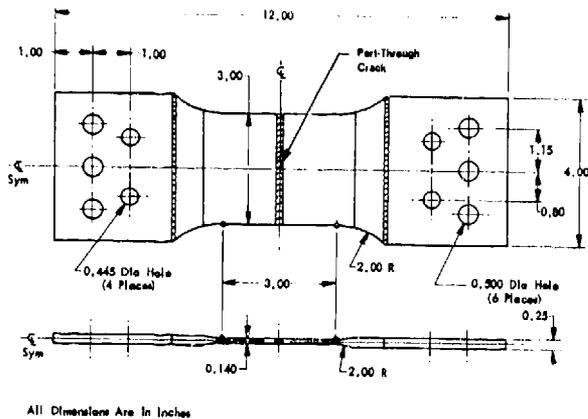
FIGURE 14. SPECIMEN DESIGN FOR PART-THROUGH-CRACKED WELDS IN SPECIMENS OF ALLOY 718(15)
