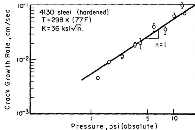
FIGURE 6. EFFECT OF HYDROGEN-GAS PRESSURE ON CRACK GROWTH RATE OF AISI 4130 STEEL<sup>(14)</sup>
