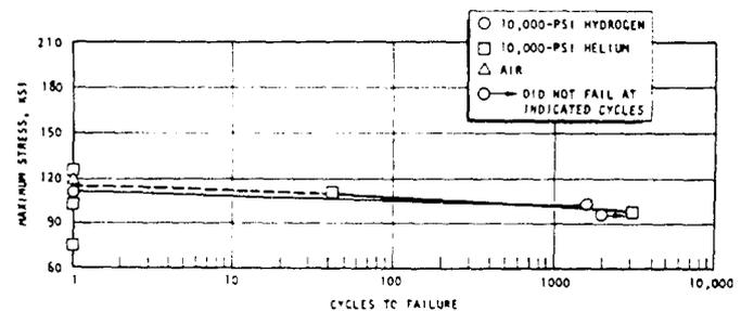
FIGURE 7. LOW-CYCLE FATIGUE CURVES FOR PRE-CRACKED SPECIMENS OF AISI TYPE 310 STAINLESS STEEL TESTED IN HELIUM OR HYDROGEN<sup>(6)</sup>
