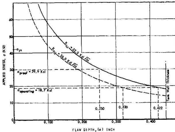
FIGURE 12. THRESHOLD FLAW DEPTH FOR WELDS IN 0.445 INCH THICK PLATE OF 2219-T6E46 ALUMINUM ALLOY IN HYDROGEN GAS AT 5200 PSI(15)
