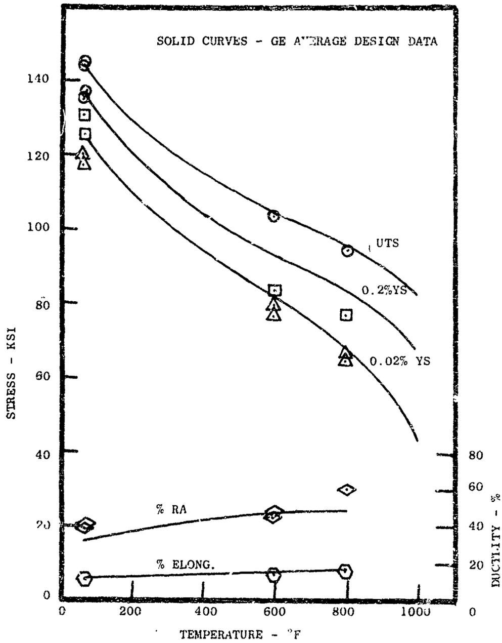
Figure 6 Tensile Properties - Inertia Welded Ti-6Al-4V
