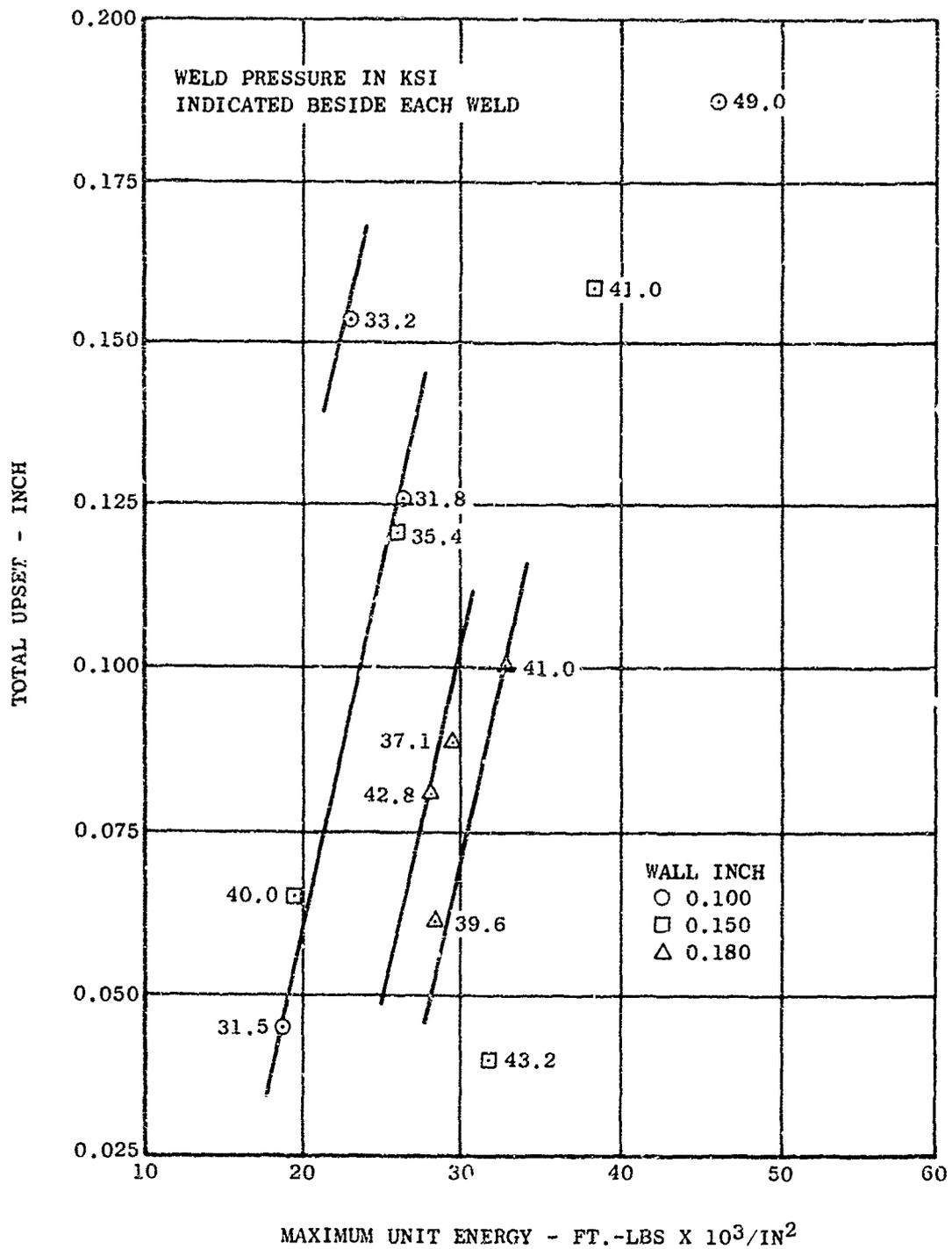
Figure 18 Total Upset vs. Energy - 24 Inch Diameter Inconel 718 Test Rings
