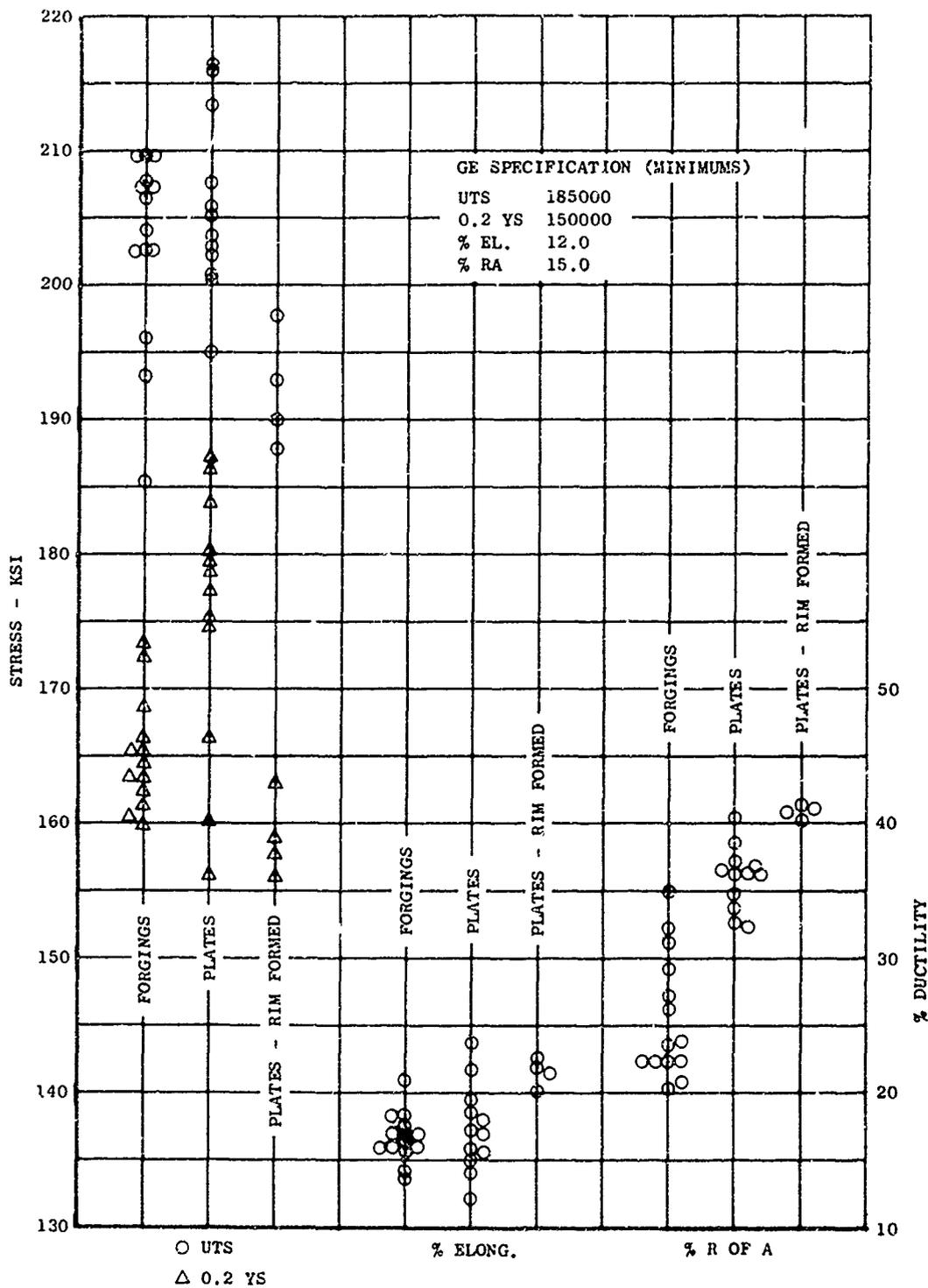
Figure 91. Room Temperature Tensile Properties of Inconel 718 Forgings, As Rolled Plates and Rim Formed Plates
