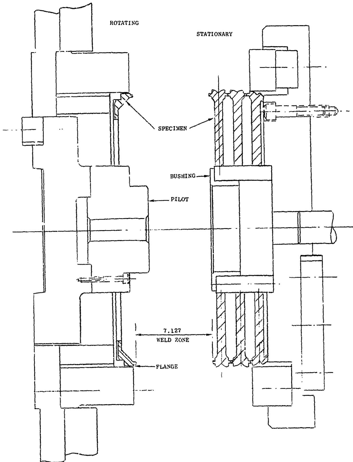
Figure 63 Assembly Layout for Rotor Weld No. 3
