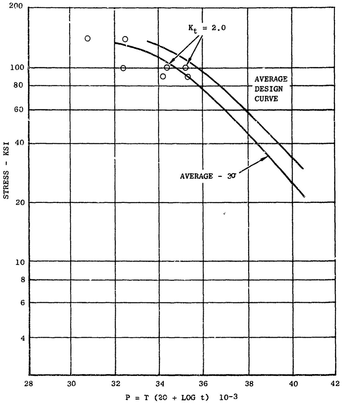
Figure 7 Stress Rupture Properties - Inertia Welded Inconel 718
