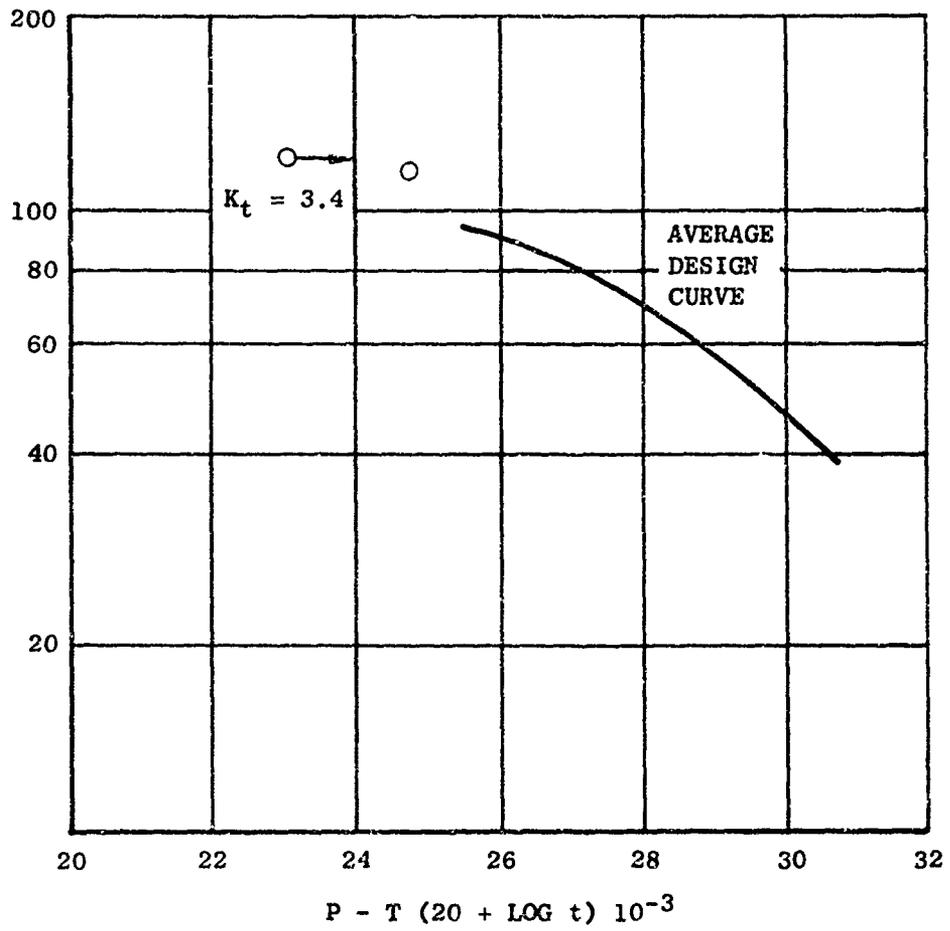
Figure 9 Stress Rupture Properties - Inertia Welded Ti 6Al-4V
