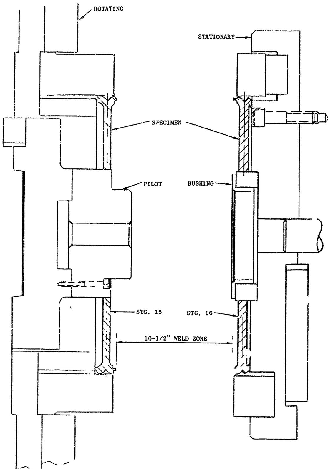
Figure 61 Assembly Layout for rotor Weld No. 1
