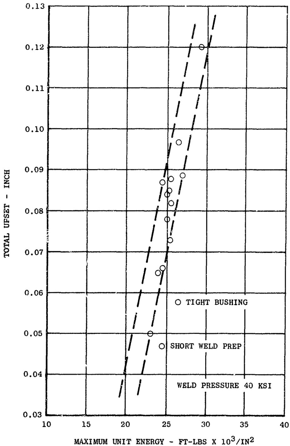
Figure 64 Upset vs. Unit Energy in Inertia Welding
