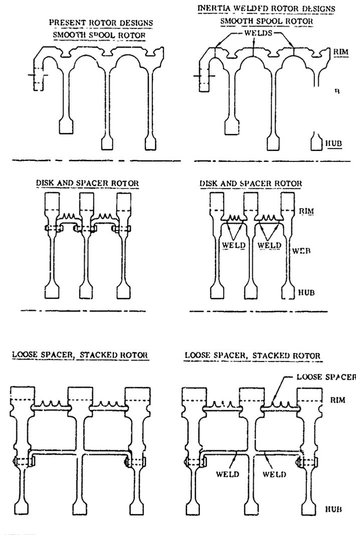
In general, spool type rotors consist of three or more stages machined from one piece forgings. Depending on the particular rotor design a number of such subassemblies are then bolted together to form the complete rotor. As shown in the sketch the rotor blades are mounted in circumferential dovetail slots or tracks.
