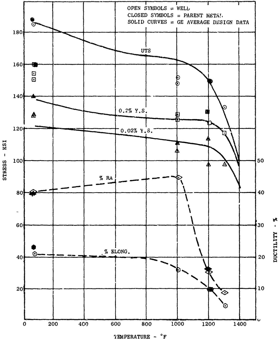
Figure 4 Tensile Properties - Inertia Welded Inconel 718 - Room Temperature
