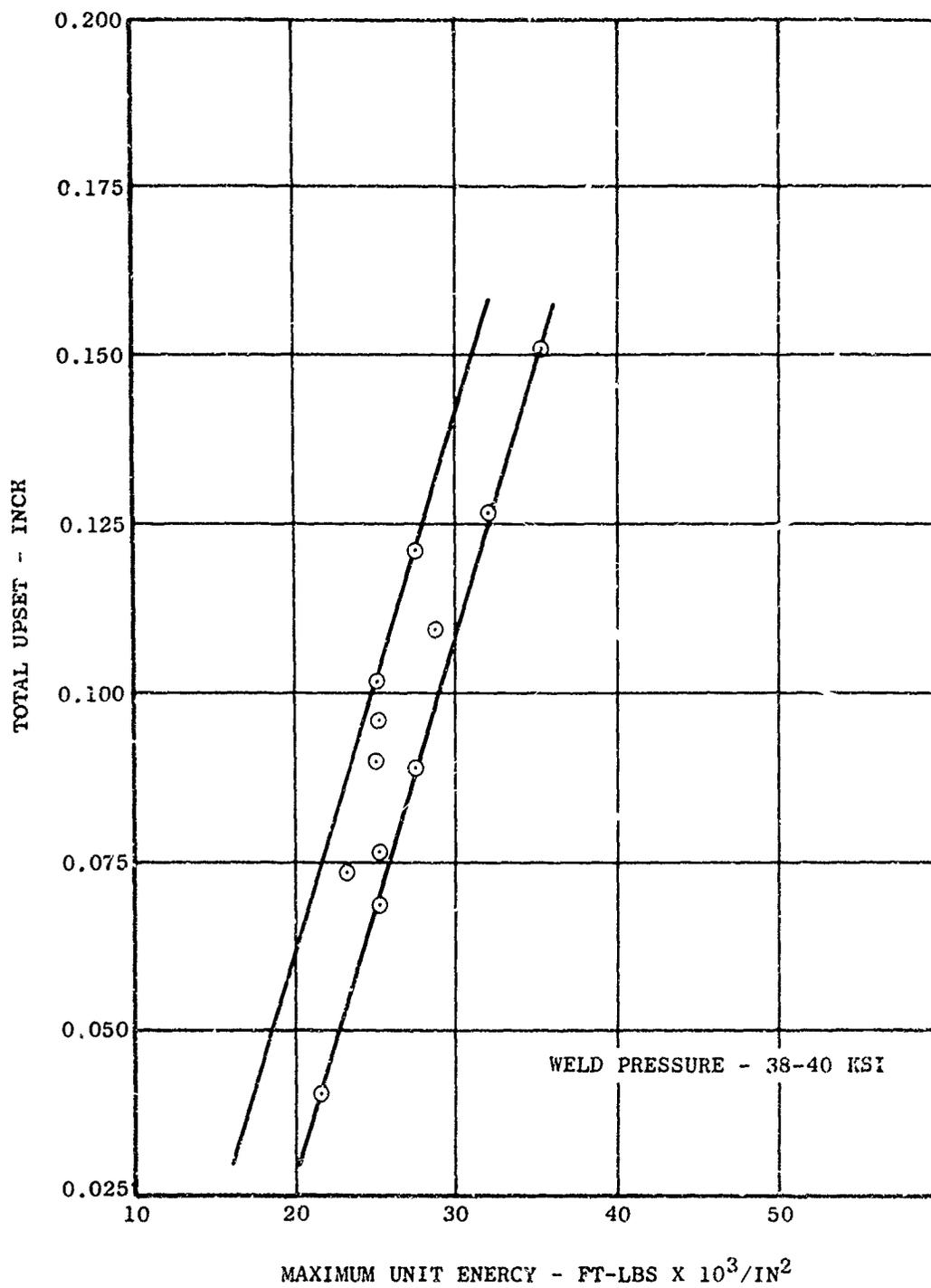
Figure 19 Total Upset vs Energy - 24 Inch Diameter Inconel 718 Test Rings with 0.180 Inch Walls.
