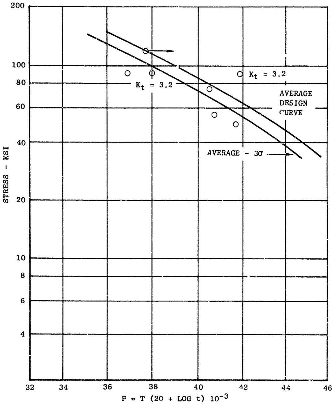
Figure 8 Stress Rupture Properties - Inertia Welded Udinet 700
