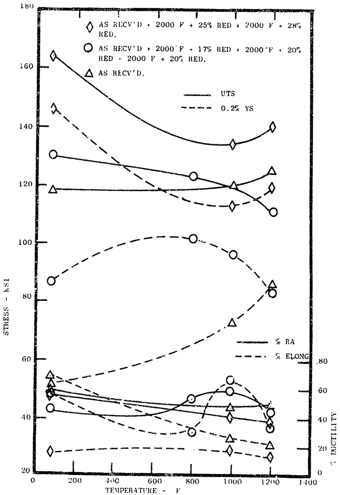
Figure 31 Tensile Properties of Cold Worked and Heat Treated Inconel 718 Cross Rolled Plate
