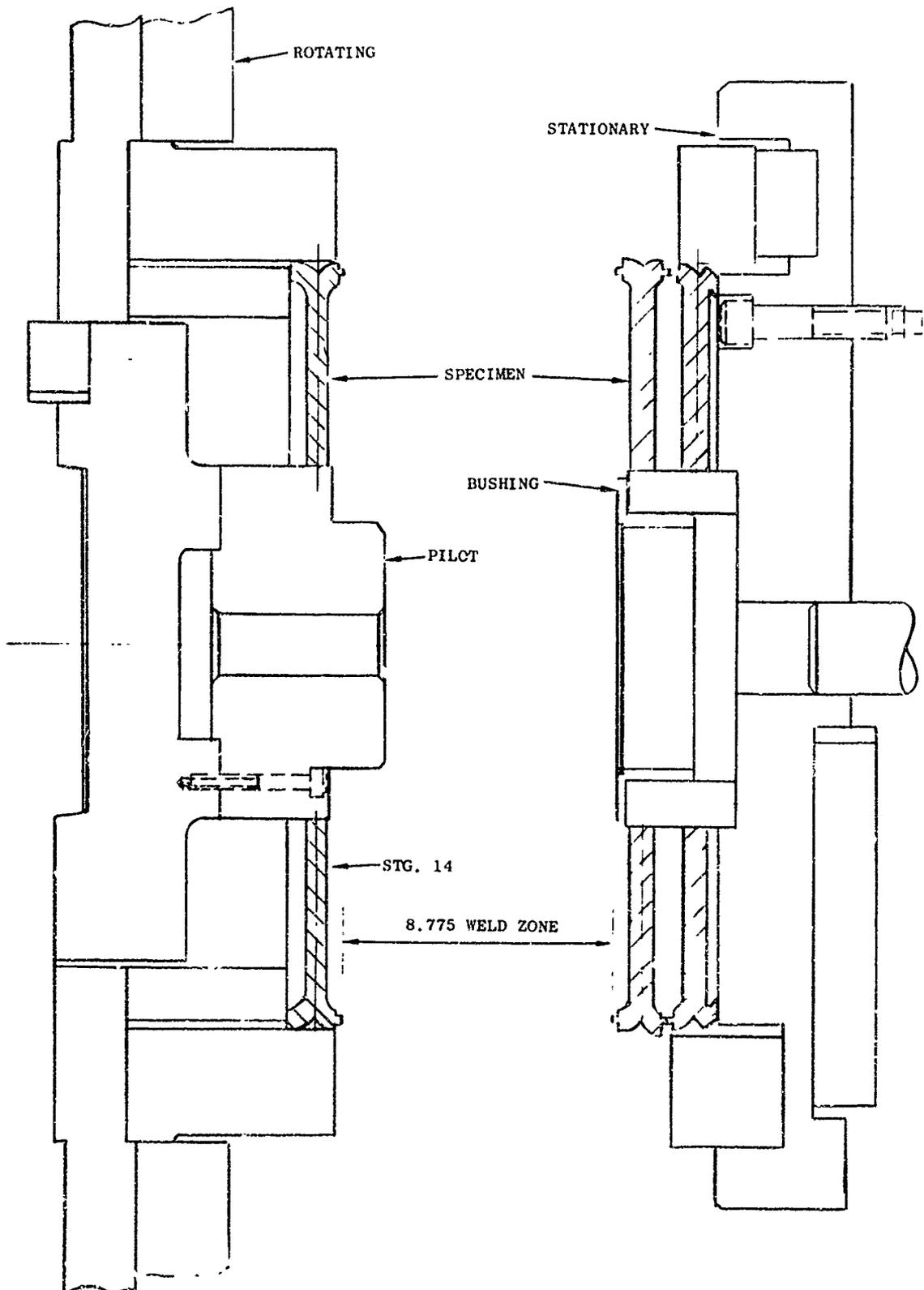
Figure 62 Assembly Layout for Rotor Weld No. 2
