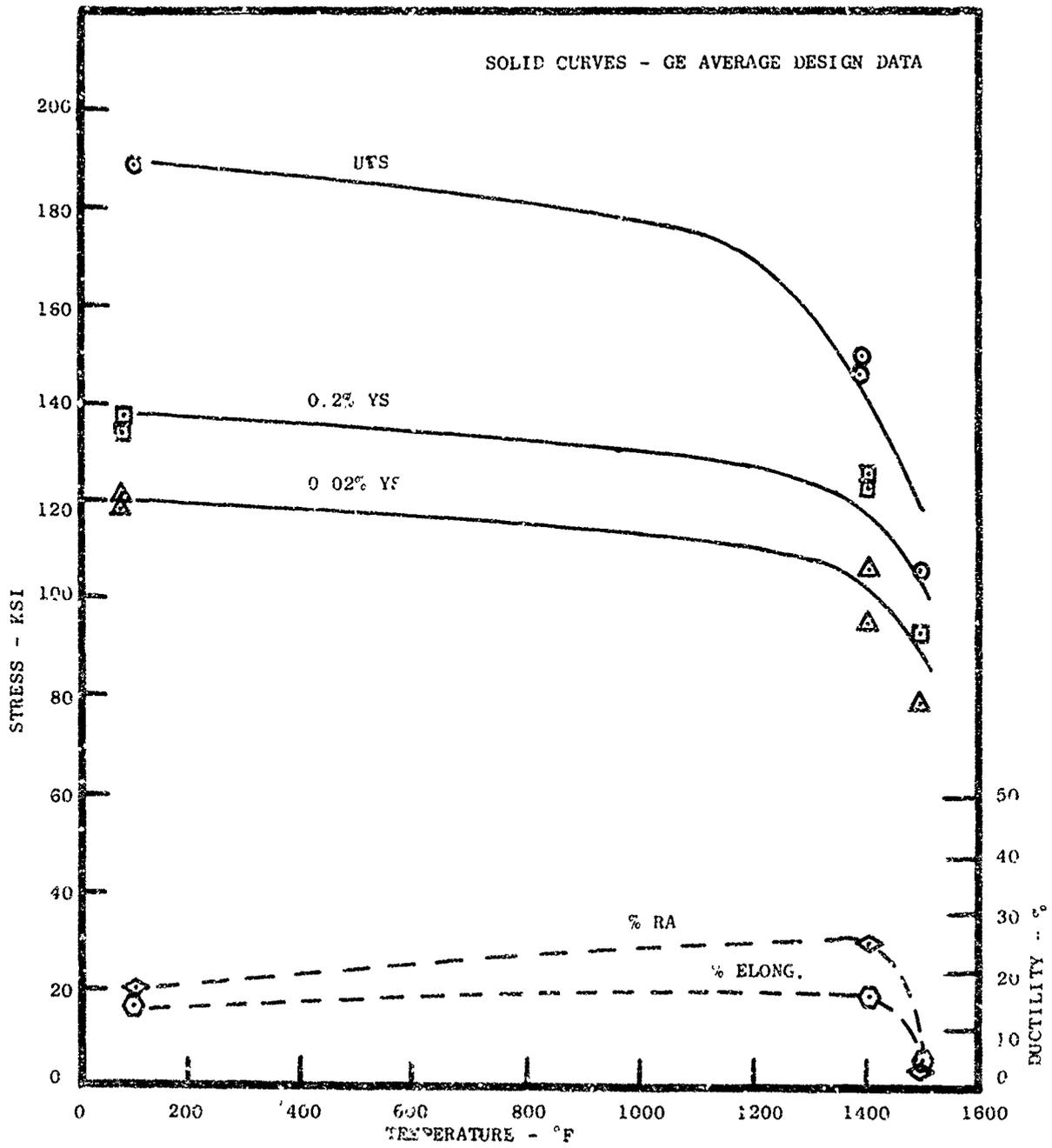
Figure 5 Tensile Properties - Inertia Welded Udimet 700
