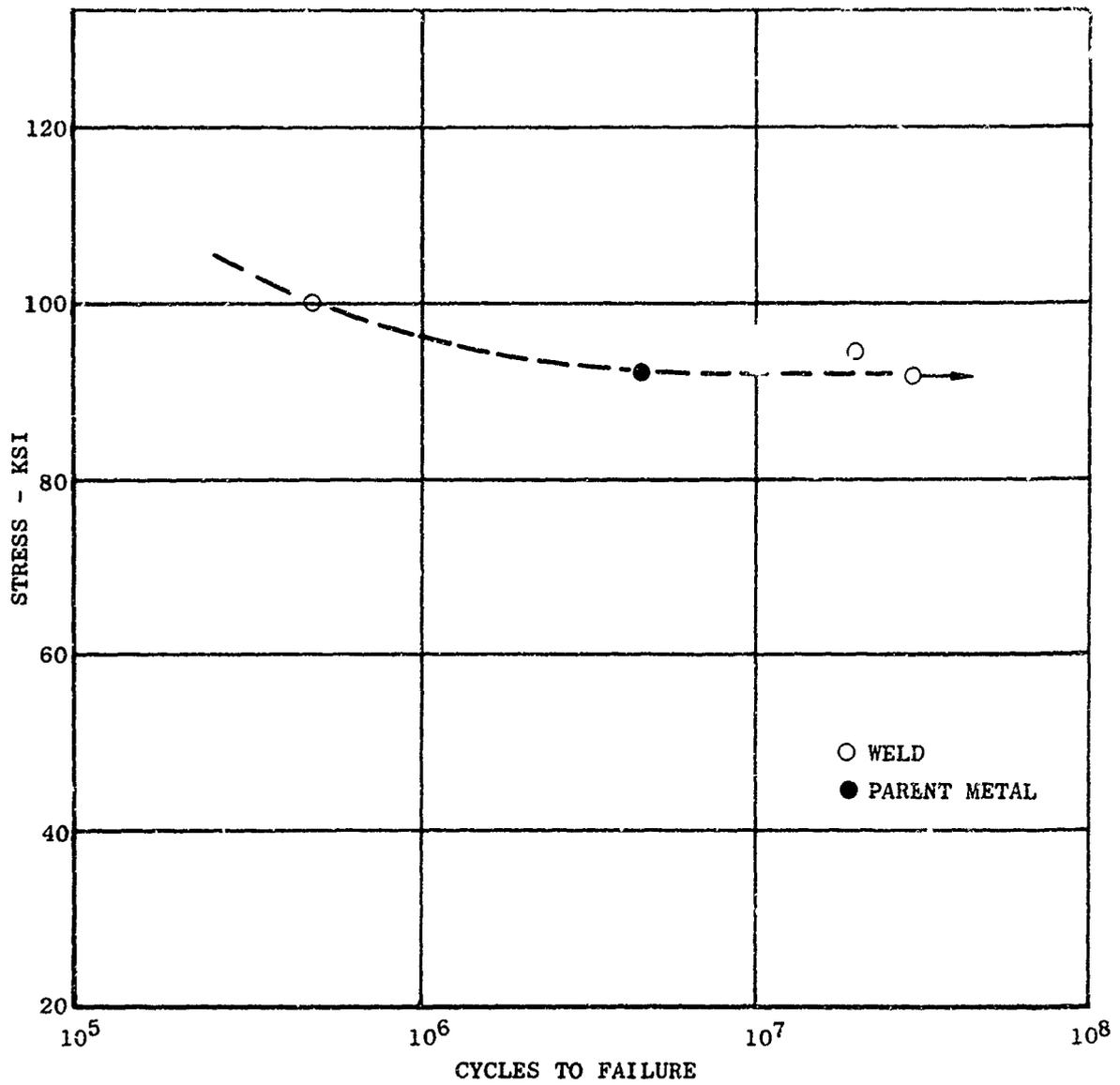
Figure 10 Rotating Beam Fatigue Properties - Inertia Welded
