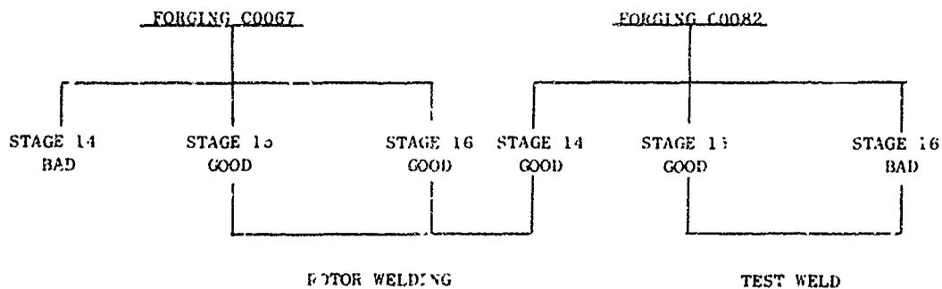
Also, as shown above, two discs were selected for test piece welding to insure that weld parameters previously used for cross rolled plate were applicable to this material.
