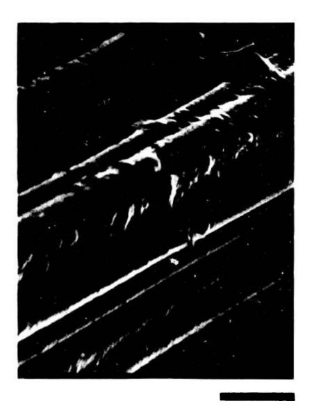
Figure 3. Scanning electron micrograph of exposed Thornel fiber on the tensile fracture surface of a sample molded at 275°C and then annealed at 245°C for three hours. Note the coating of matrix which almost completely covers the fiber. The scale bar represents 2 microns.
