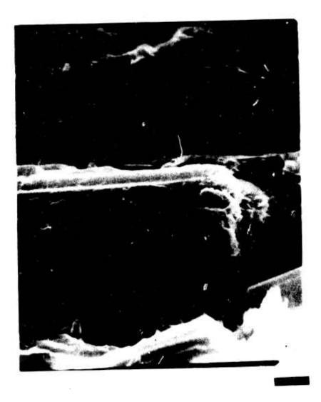
Figure 2. Scanning electron micrograph of exposed Thornel fiber on the tensile fracture surface of a sample molded at 275°C. Note the increase in adhering matrix on the fiber over that seen in Figure 1. The scale bar represents 2 microns.
