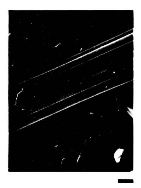
Figure 4. Scanning electron micrograph of an "as-received" Thornel fiber. The scale bar represents 2 microns.
