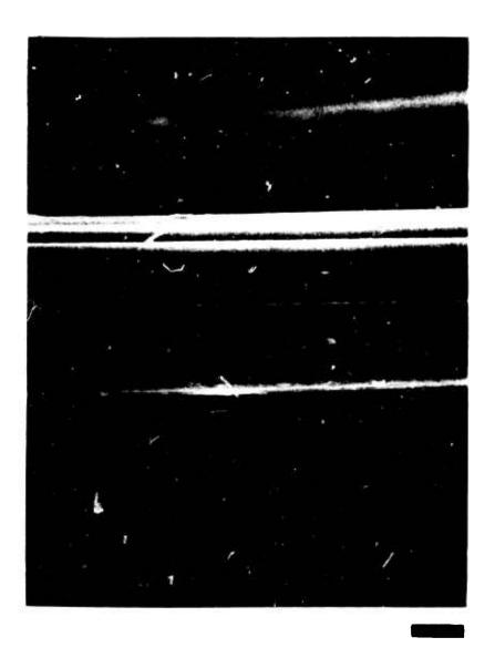
Figure 1. Scanning electron micrograph of exposed Thornel fiber on the tensile fracture surface of a sample molded at 190°C. Note the similarity of this fiber's surface to that of the "as-received" fiber in Figure 4. The scale bar representes 2 microns.
