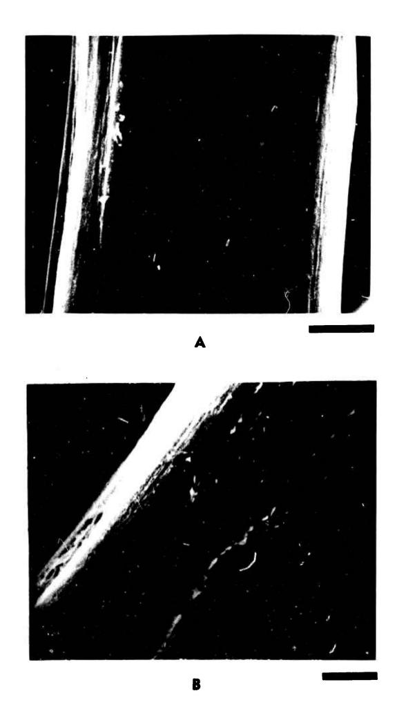
Figure 5. Scanning electron micrographs of exposed Hercules fibers on the tensile fracture surface of samples (A) molded at 190°C and (B) molded at 275°C and then annealed at 245°C for three hours. Note the increase in amount of adhering plastic from (A) to (B). The scale bar represents 2 microns.
