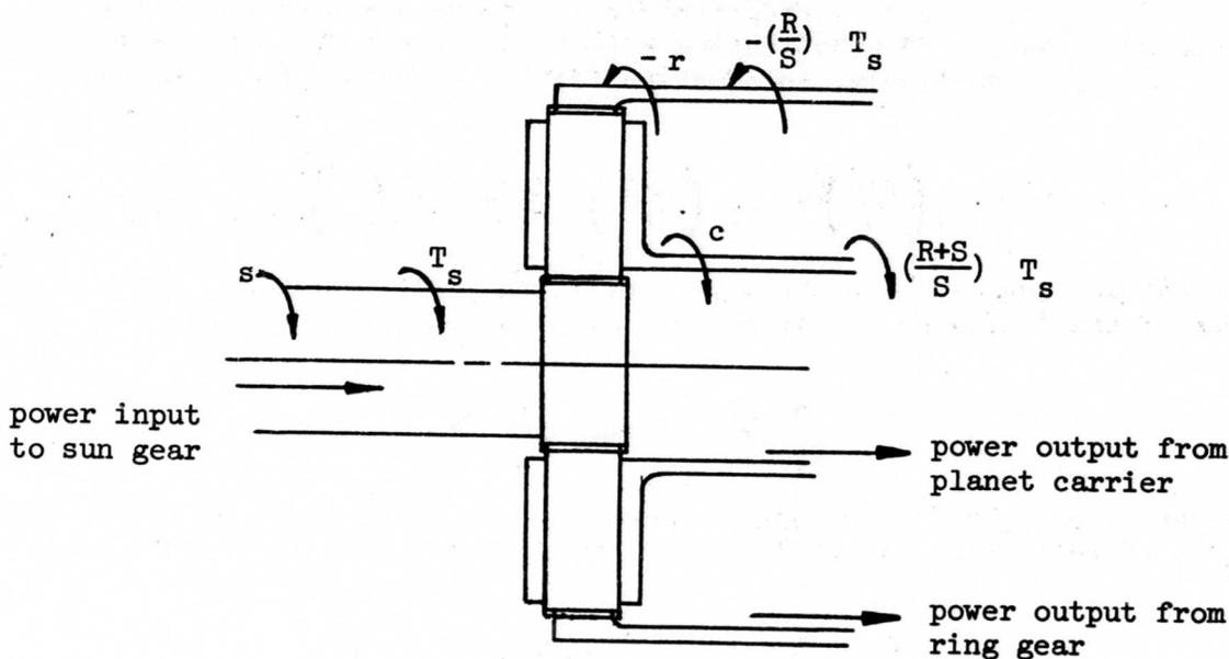
Figure 49. Directions of Rotation To Avoid Recirculation of Power.
