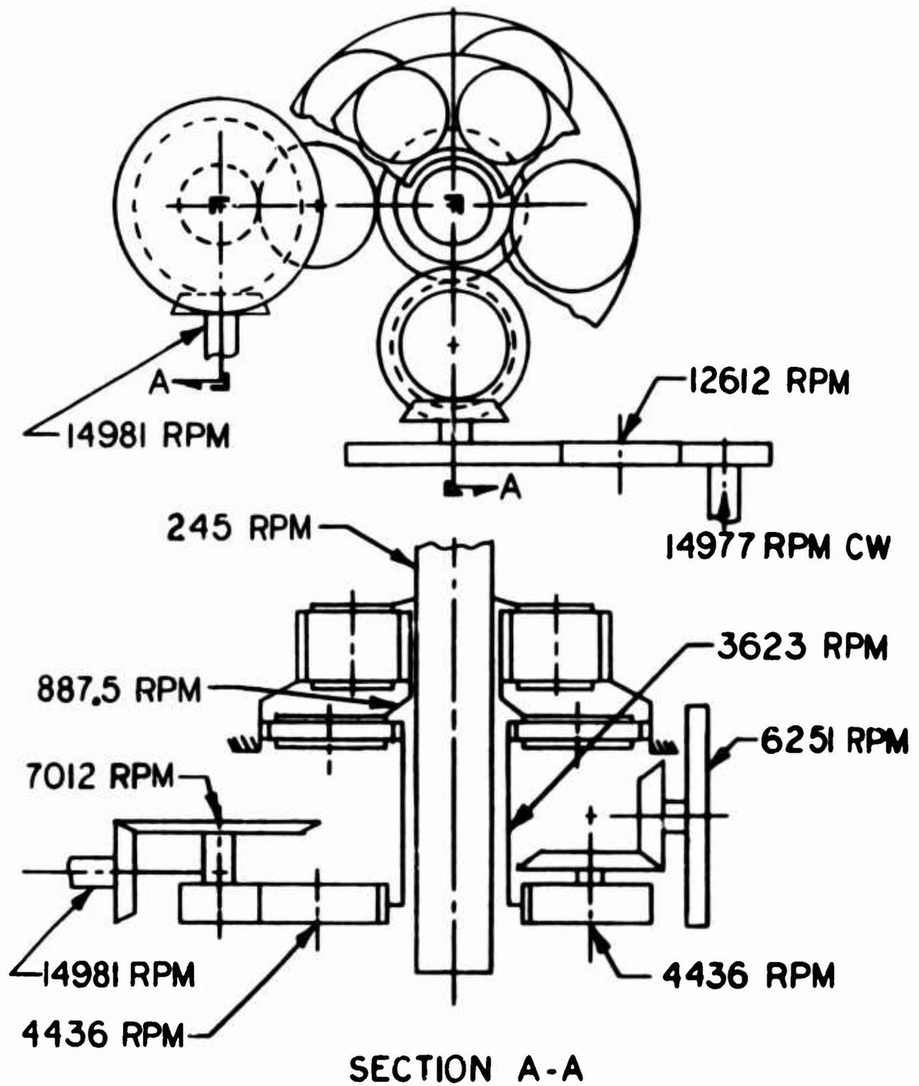
Figure 14. Gearing Schematic of Configuration Number 11.
