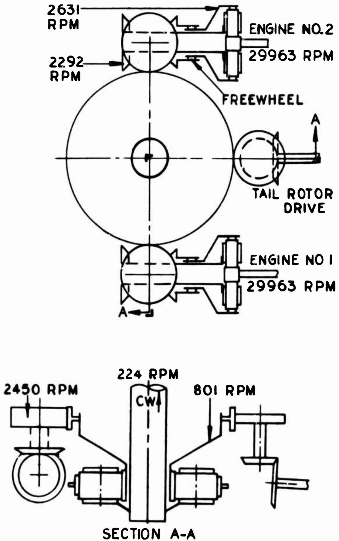
Figure 9. Gearing Schematic of Configuration Number 6.
