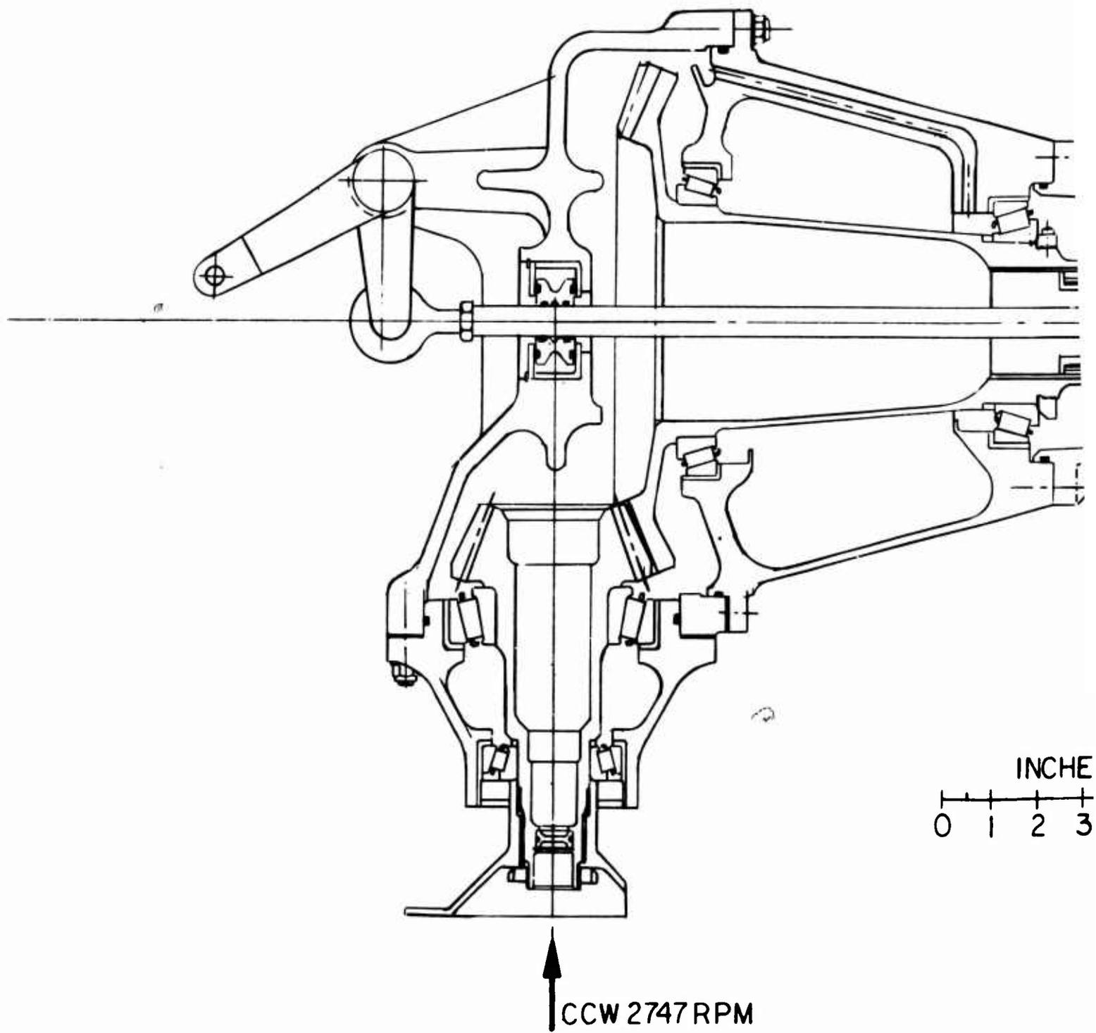
Figure 33. Tail Rotor Gearbox, Pure Helicopter.
