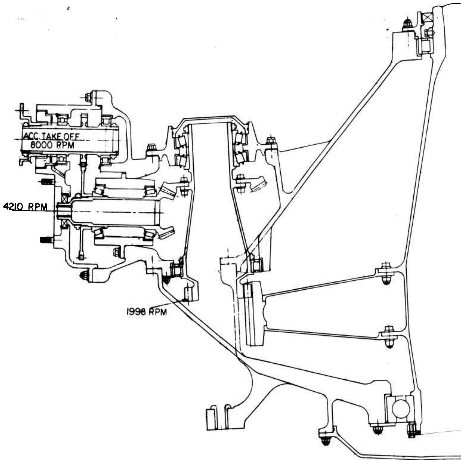
Figure 30. Section A-A, Main Gearbox, Pure Helicopter.
