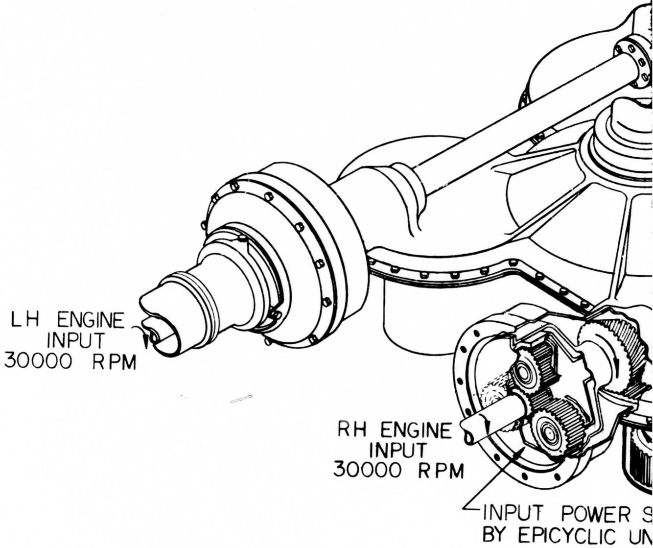
Figure 11. Main Transmission Arrangement, Pure Helicopter.
