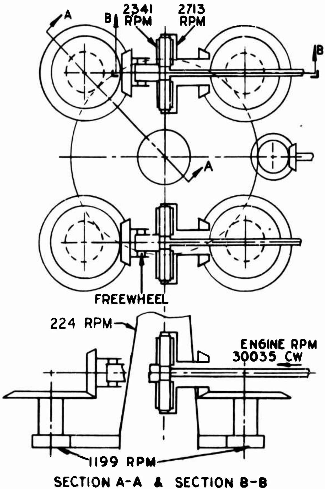
Figure 8. Gearing Schematic of Configuration Number 5.
