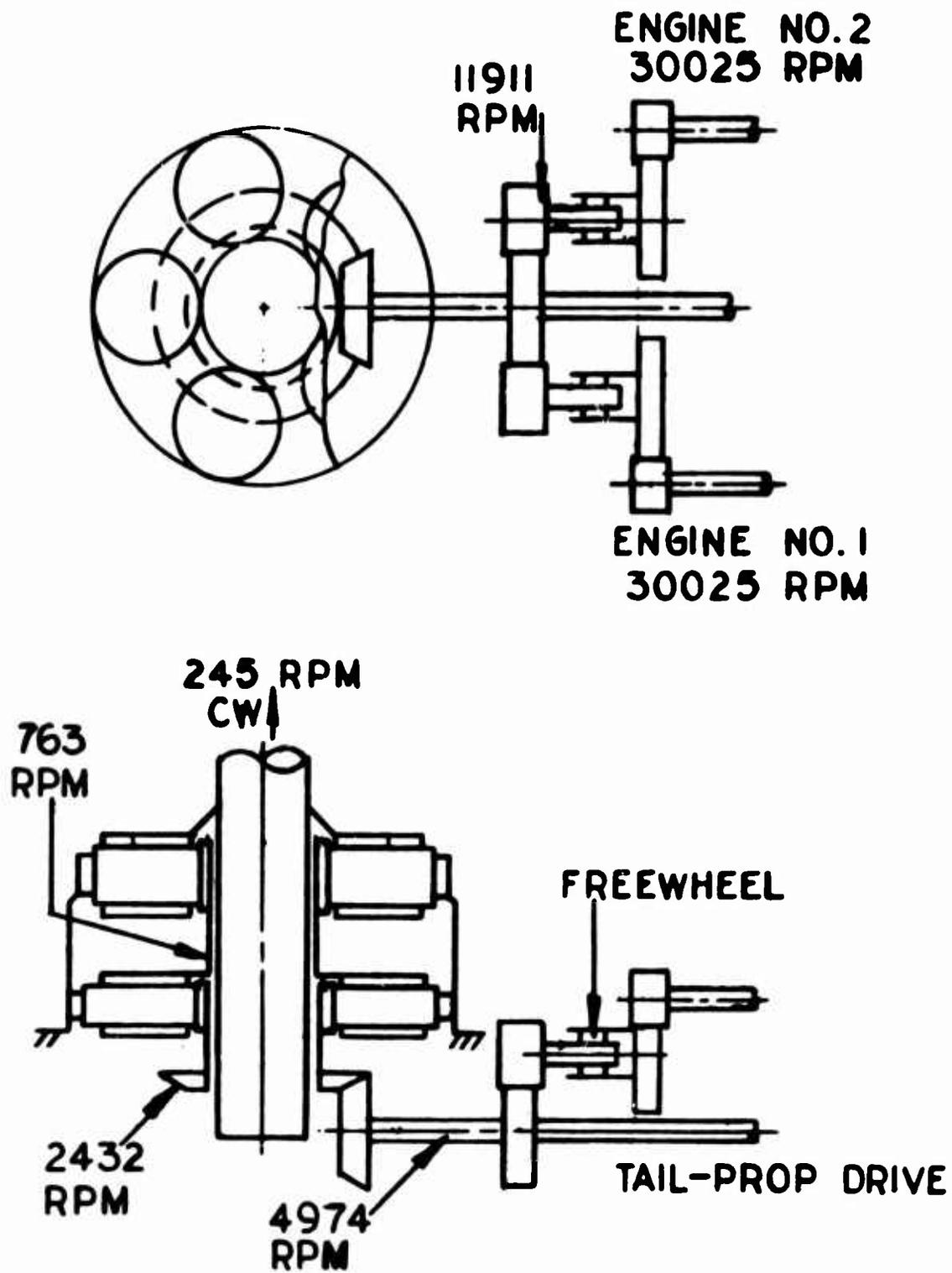
Figure 17. Gearing Schematic of Configuration Number 14.
