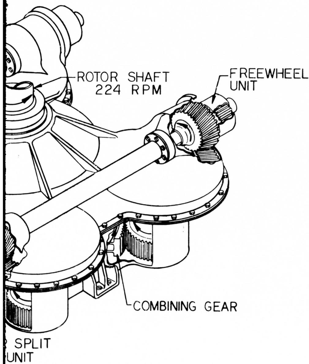
15,000 fpm. In this way the difficult bearing problems associated with bevel gears operating at high rotational speeds are avoided.
