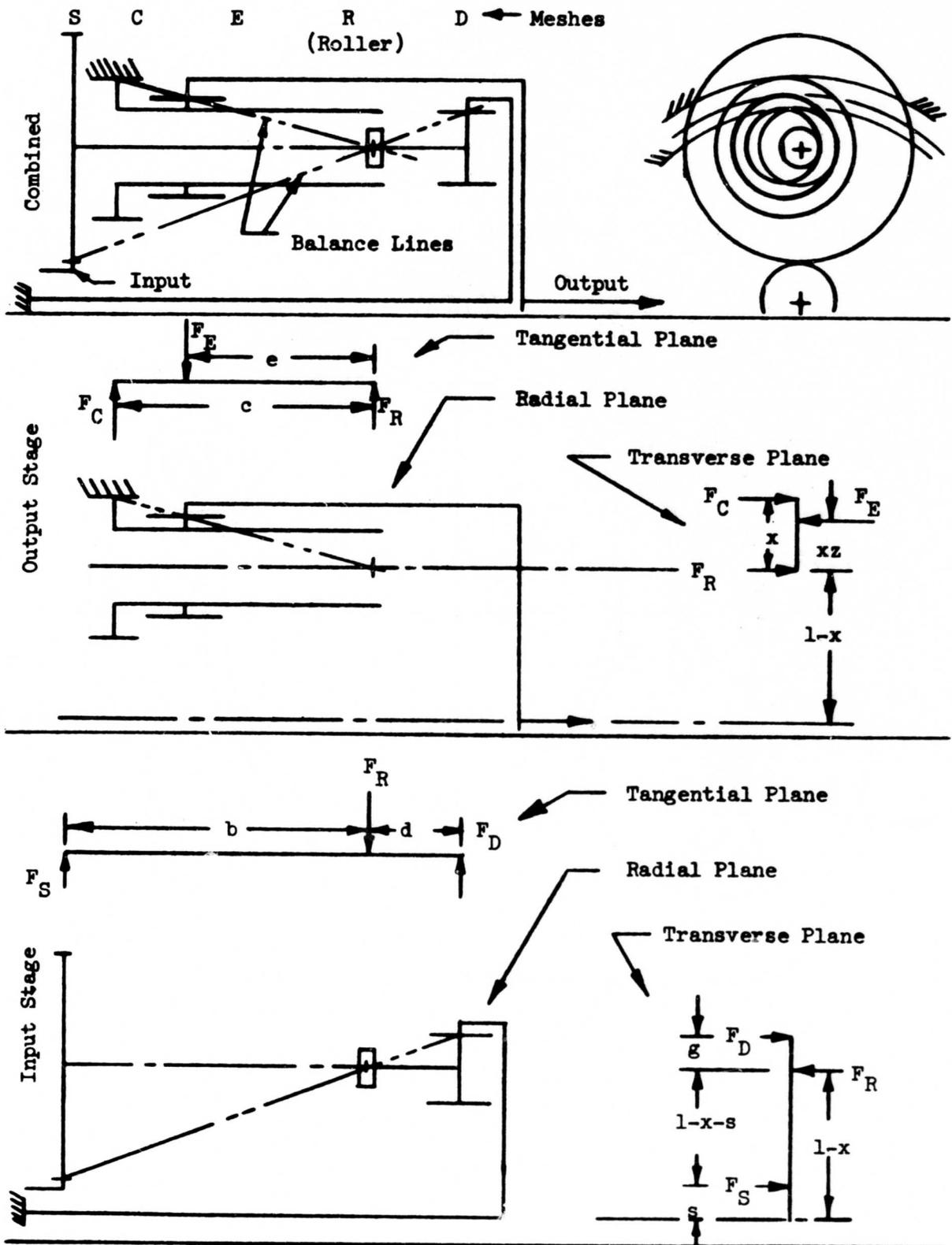
Figure 58. Schematic Diagram of Free-Planet Force Resolution.
