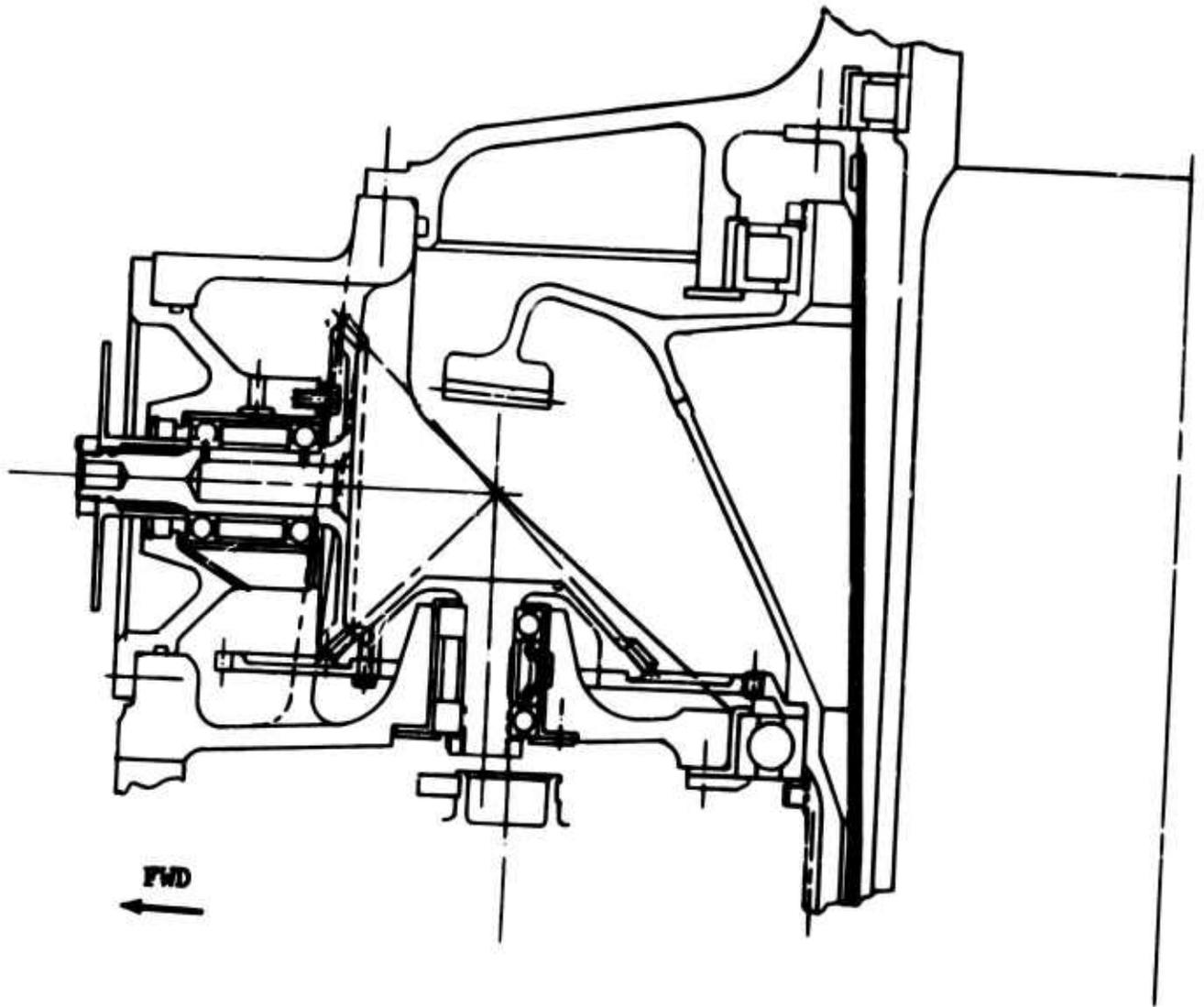
Figure 60. Accessory Drive Arrangement.
