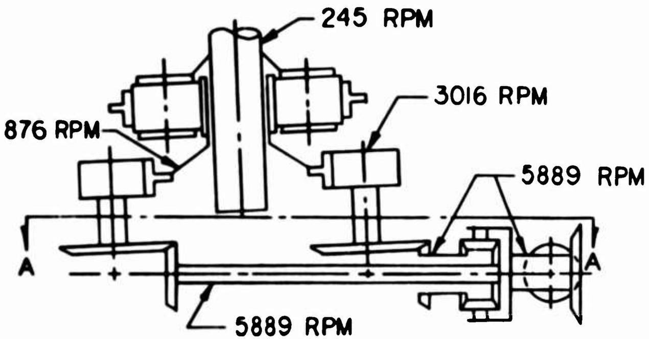
Figure 19. Gearing Schematic of Configuration Number 16.
