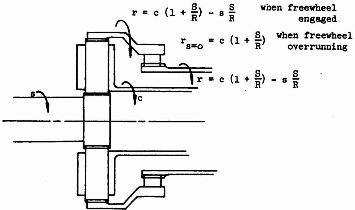
Figure 50. Speeds When Freewheel Is Driven by Ring Gear.
