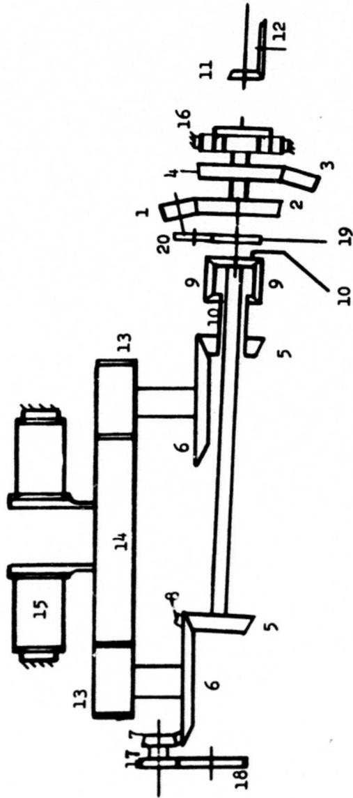
Figure 48. Gearing Schematic, Compound Helicopter Drive Train.
