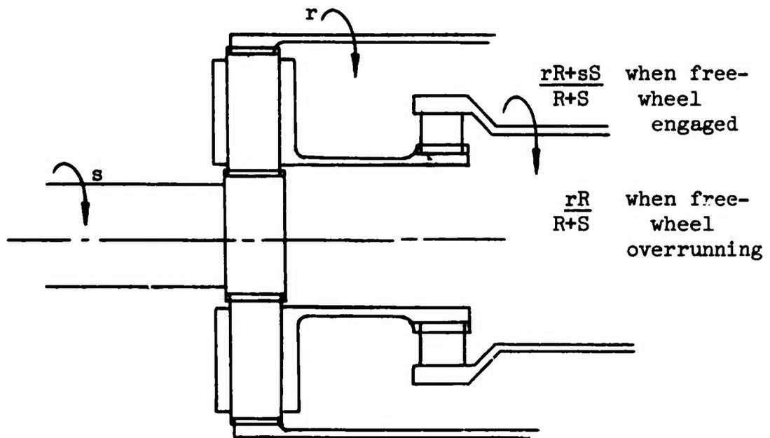
Figure 51. Speeds When Freewheel Is Driven by Planet Carrier.
