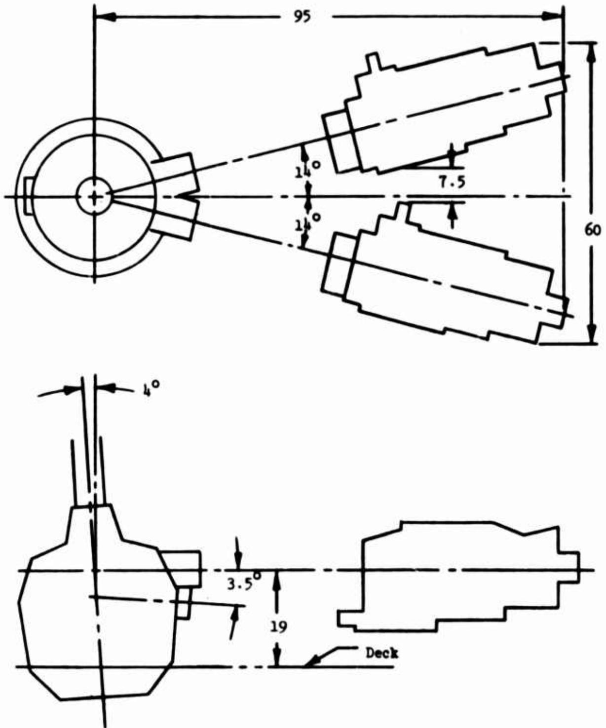
Figure 54. Engine - Gearbox Installation Arrangement.
