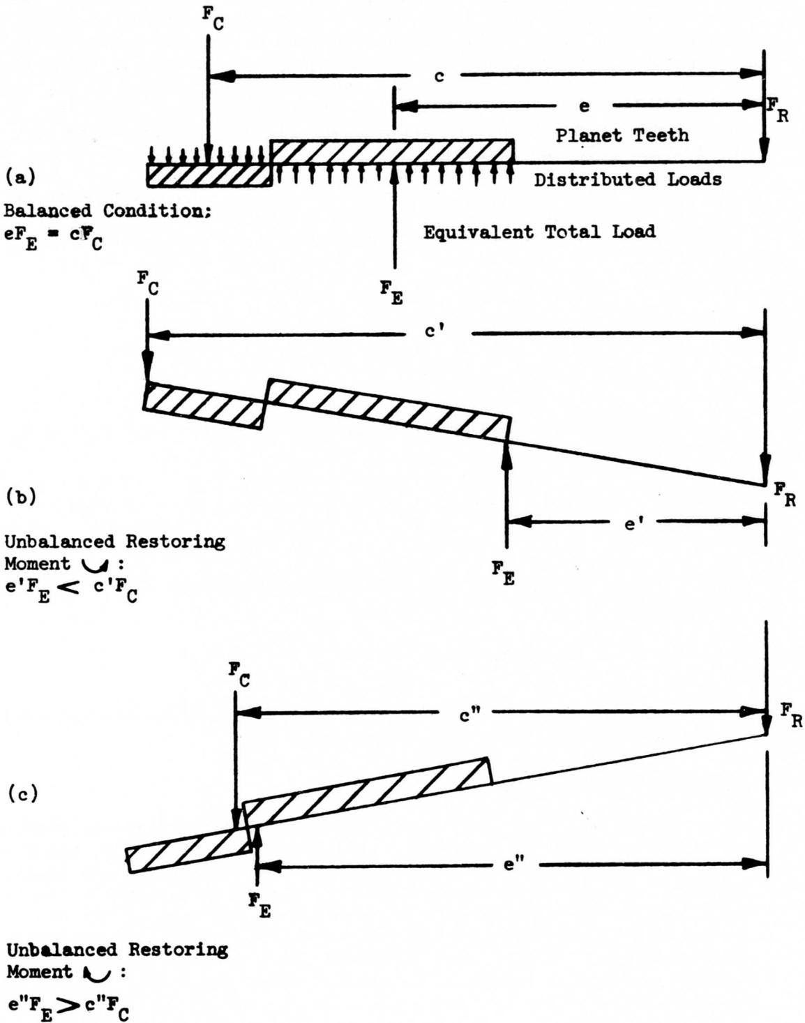
Figure 59. Schematic Diagram of Facewise Load Distribution.
