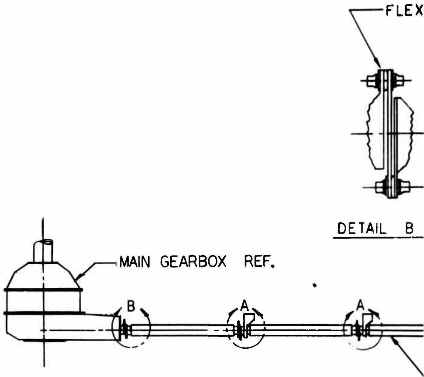
Figure 43. Propeller - Tail Rotor Drive System, Compound Helicopter.
