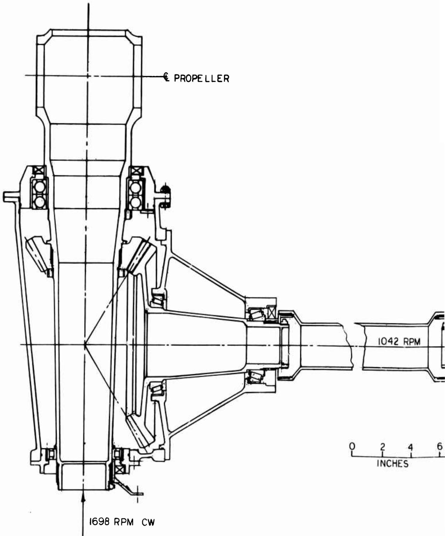
Figure 44. Propeller - Tail Rotor Gearbox Arrangement, Compound Helicopter.
