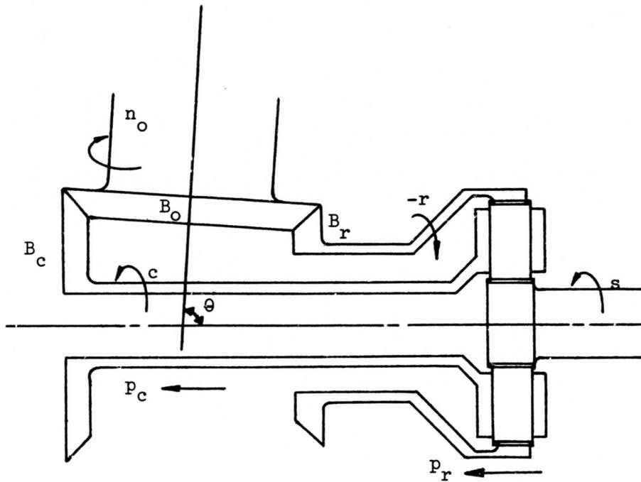
Figure 52. Arrangement of Epicyclic Unit and Bevel Gears in Configurations 6 and 12.
