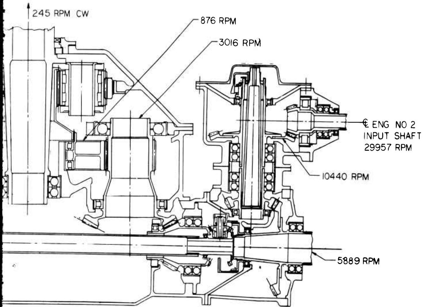
AND SECTION B-B. SECTION B-B ROTATED UP 90°
