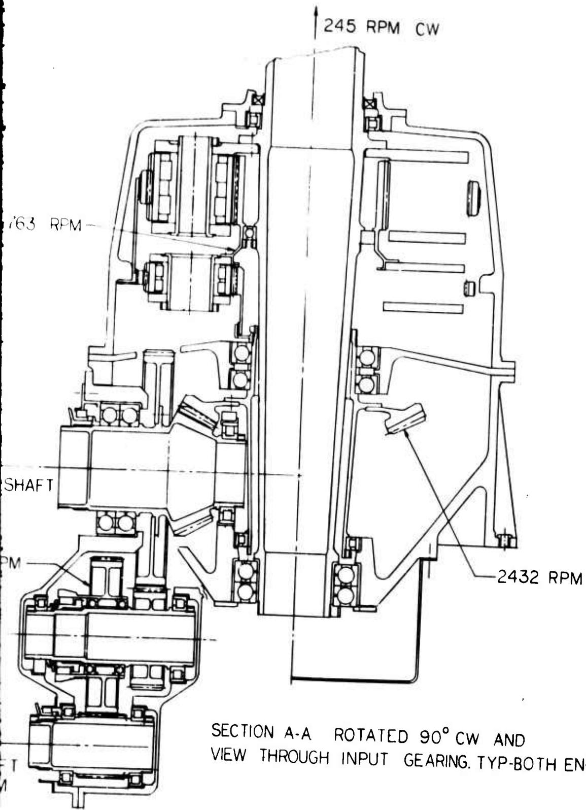
SECTION A-A ROTATED 90° CW AND
