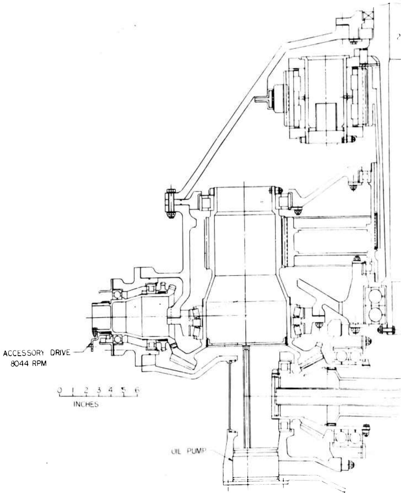
Figure 42. Section A-A, Main Gearbox, Compound Helicopter.
