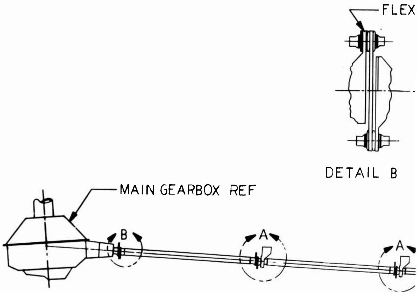
Figure 31. Tail Rotor Drive System, Pure Helicopter.
