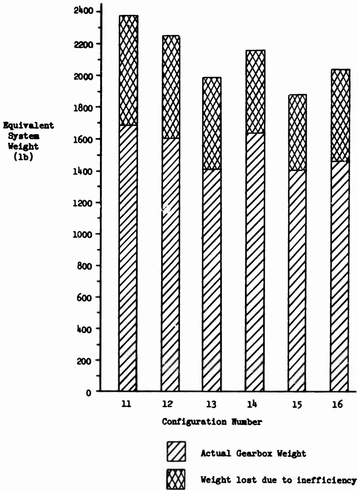
Figure 20. Weight Comparison, Equivalent System Weights.
