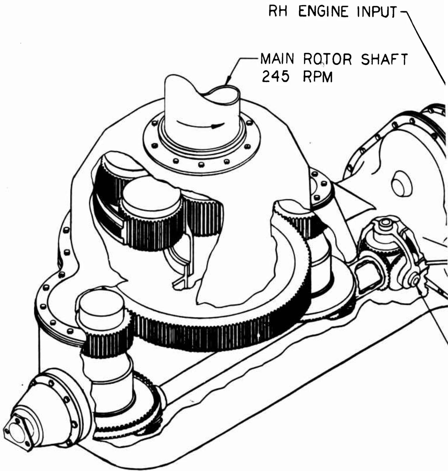
Figure 21. Main Transmission Arrangement, Compound Helicopter.
