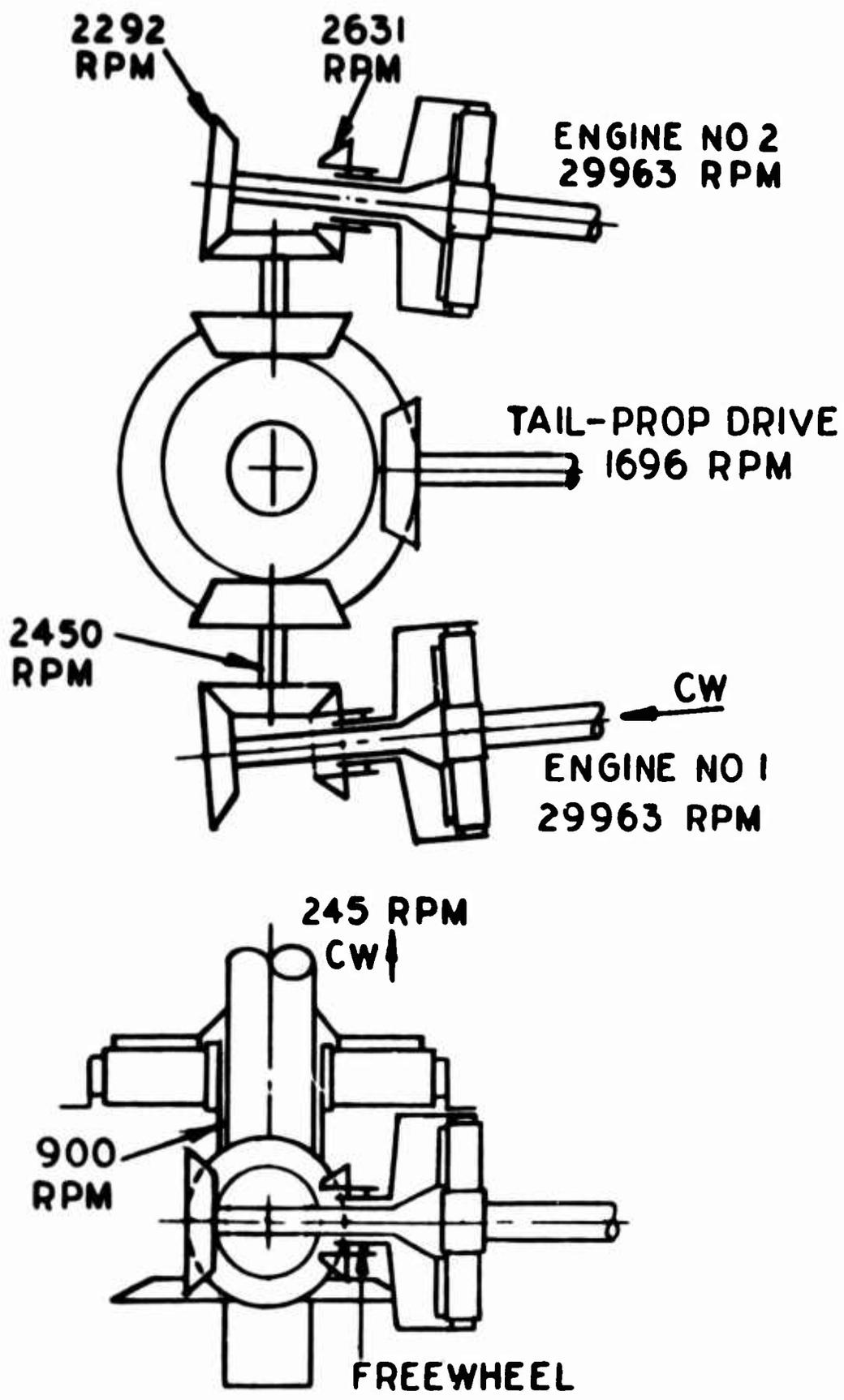
Figure 15. Gearing Schematic of Configuration Number 12.
