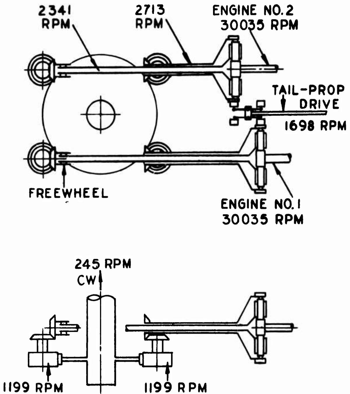
Figure 16. Gearing Schematic of Configuration Number 13.
