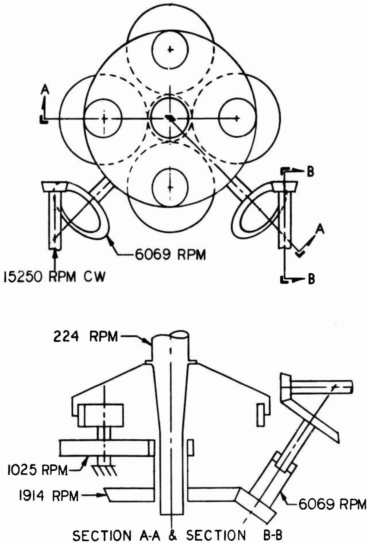
Figure 7. Gearing Schematic of Configuration Number 4.
