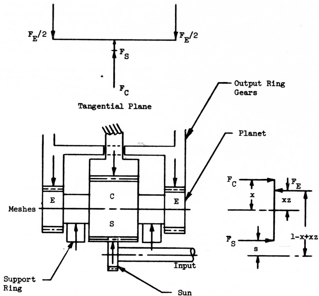
Figure 56. Power Hinge Schematic.
