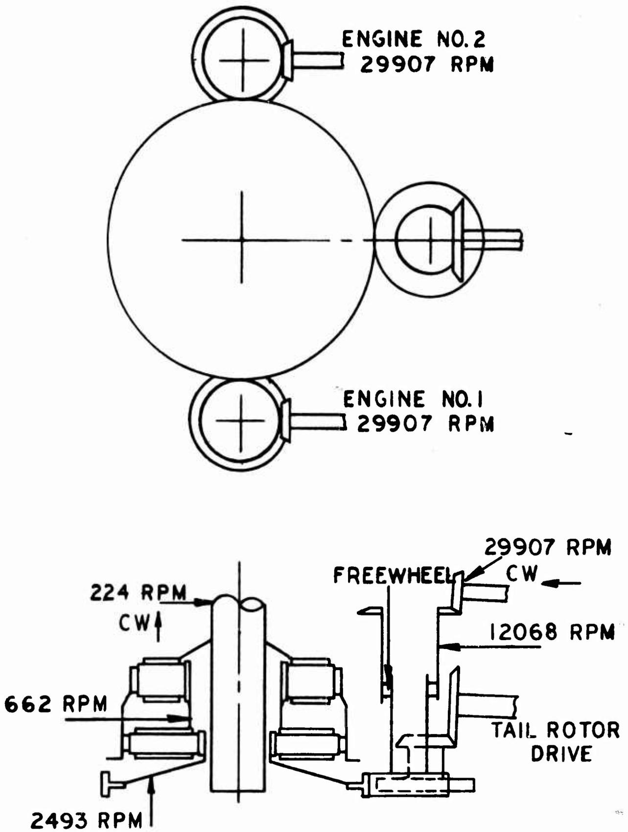
Figure 4. Gearing Schematic of Configuration Number 2.
