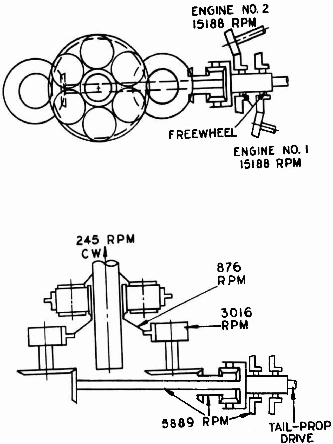
Figure 18. Gearing Schematic of Configuration Number 15.
