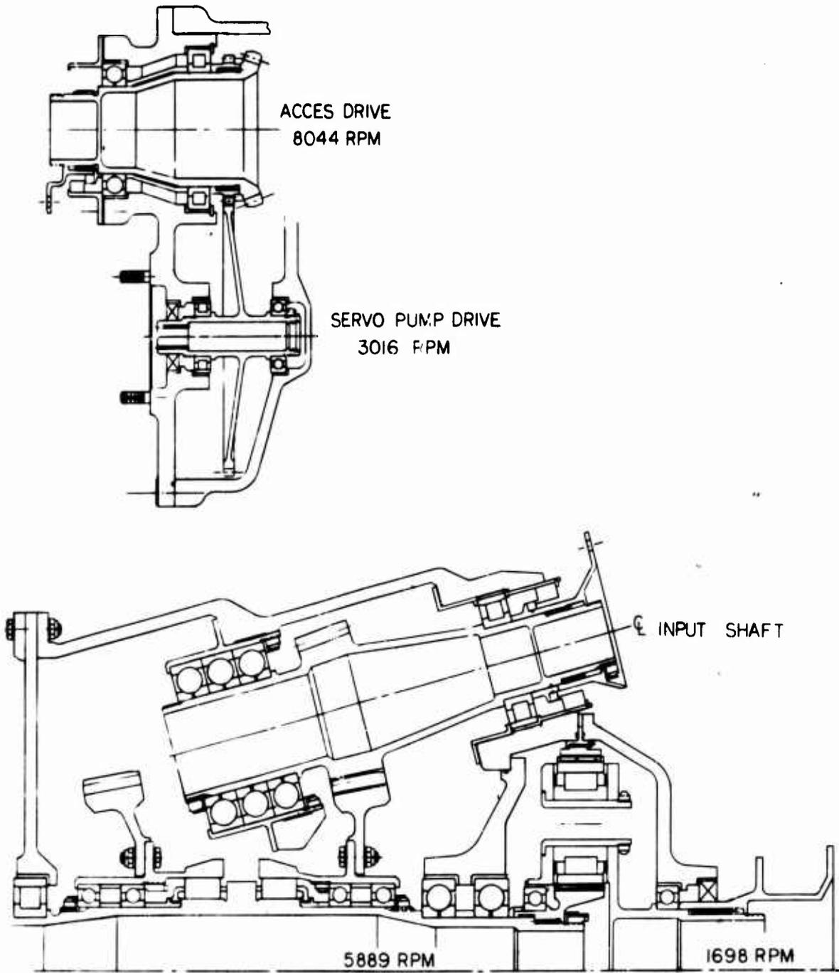
SECTION THROUGH NO 1 ENGINE INPUT GEARING
