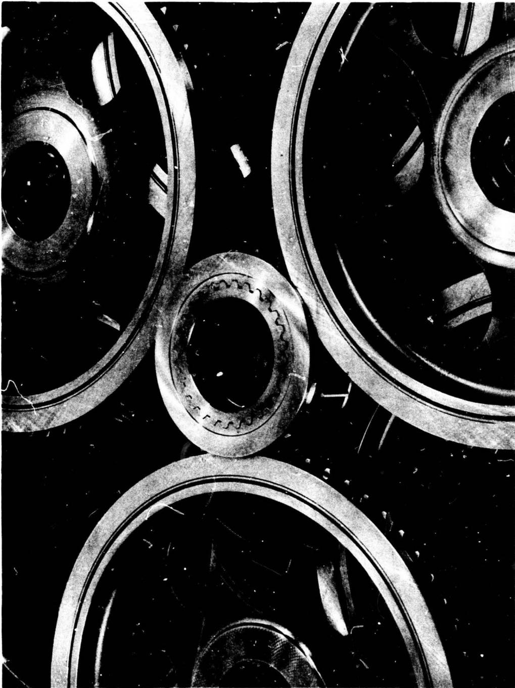
Figure 7. Sun Roller Gear Contact.
