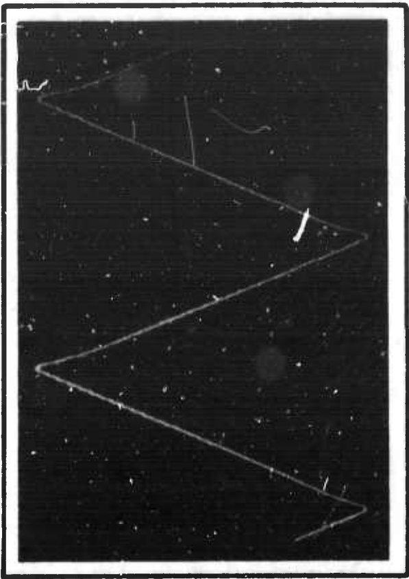
0.2 sec/cm 2 v/cm Figure 12. Triangle Scan, 1 Hz
