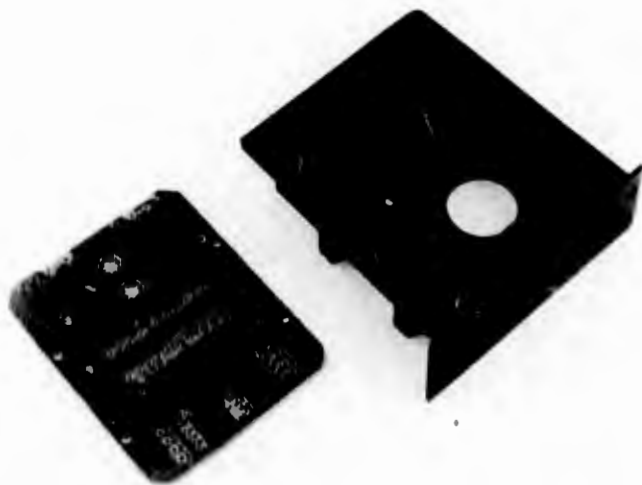
Figure 12. Instrumentation Conditioning Unit Housing and Circuit Card (Photo 4R14293)
