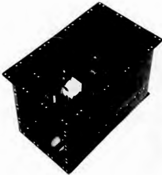
Figure 3. Electronics Unit Housing (Photo 4R14292)
