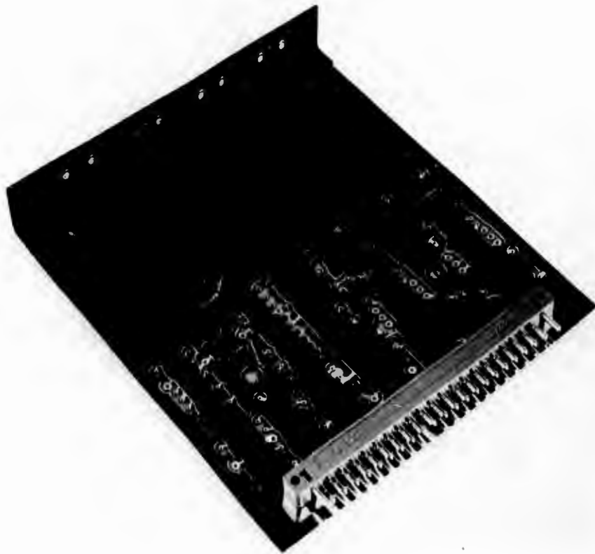
Figure 5. High-Power Circuit Card With Additional Heat Sink (Photo 4R14296)
