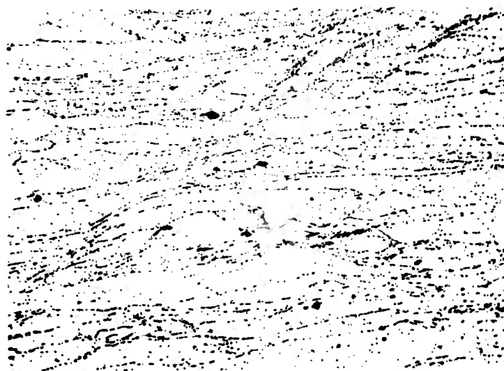
Fig. 18 - Microstructure of .063" MA09-F as-rolled sheet. Longitudinal section.
