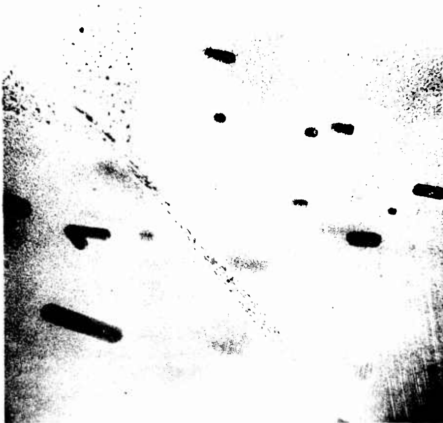
Fig. 22 - Electron micrograph of MA08. Solution heat treatment 1 hr at 910 F, precipitation treatment 36 hr at 275 F. Dispersoid particles within grains are \text{Al}_{20}\text{Cu}_2\text{Mn}_3 .
