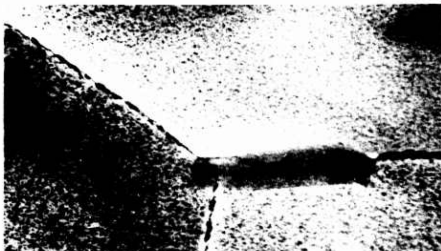
Fig. 26 - Electron micrographs of MA08. Solution heat treatment 1 hr at 910 F, precipitation treatment (a) 36 hr at 275 F, (b) 3 hr at 250 F plus 9 hr at 325 F.
