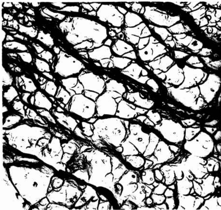
Fig. 31 - Transmission electron micrograph of oxide replica of fracture surface from MA07-T6 tear specimen of high U.P.E.
