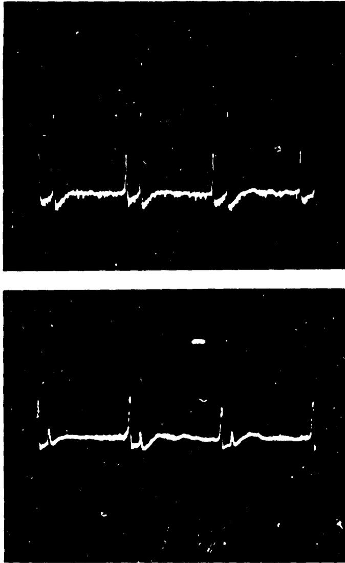
FIG. 2. Oscilloscope Traces of Yaw Sonde Signals.
