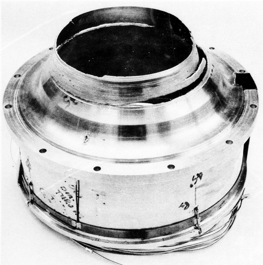
Figure 30. Bellmouth Liner and Fractured Ring Following Run 19 of Buildup A, Phase III Investigation.
