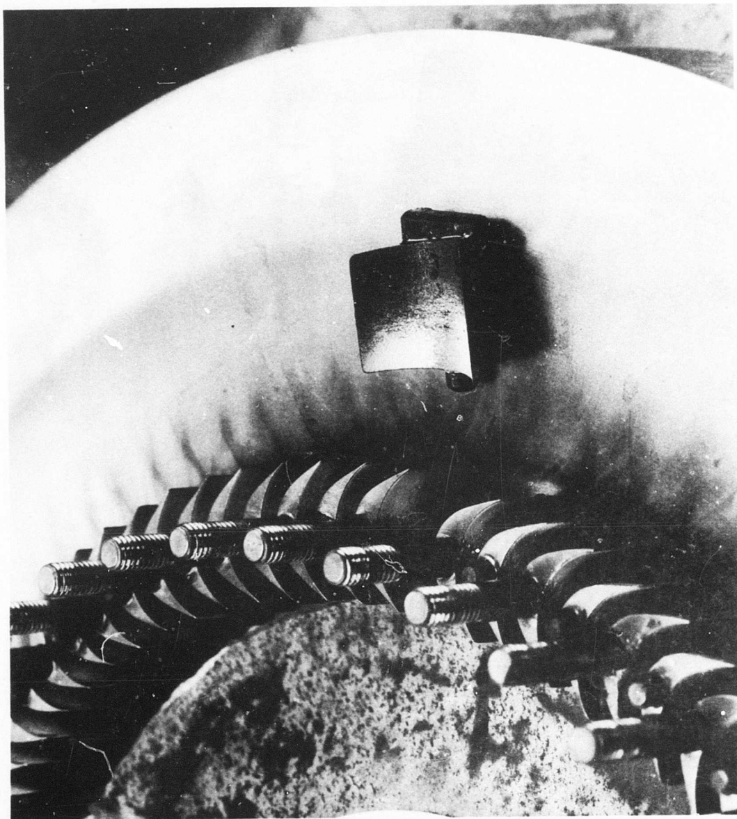
Figure 32. Soot Patterns on Rotor Blades and Disc Following Run Number 19 of Buildup A, Phase III Investigation.
