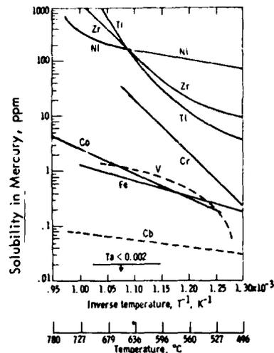
FIGURE 3. LIQUIDUS CURVES OF METALS IN HIGH-TEMPERATURE MERCURY(5)
