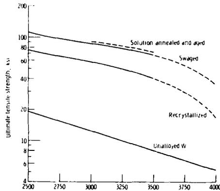
FIGURE 4. TENSILE STRENGTH OF OPTIMUM ALLOY COMPOSITION W-4Re-0.35Hf-0.35C COMPARED WITH STRENGTH OF UNALLOYED TUNGSTEN AT 2500 TO 4000 F<sup>(10)</sup>
