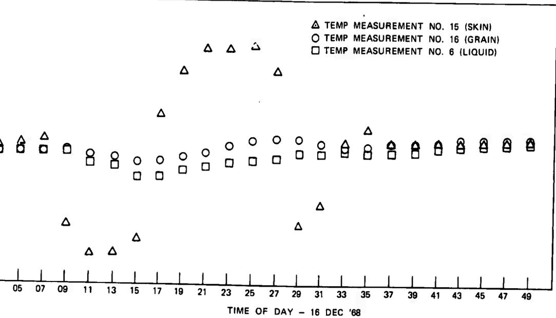
Aerodynamic Heating Profile for 12-Inch Diameter Liquid Propulsion Systems.
