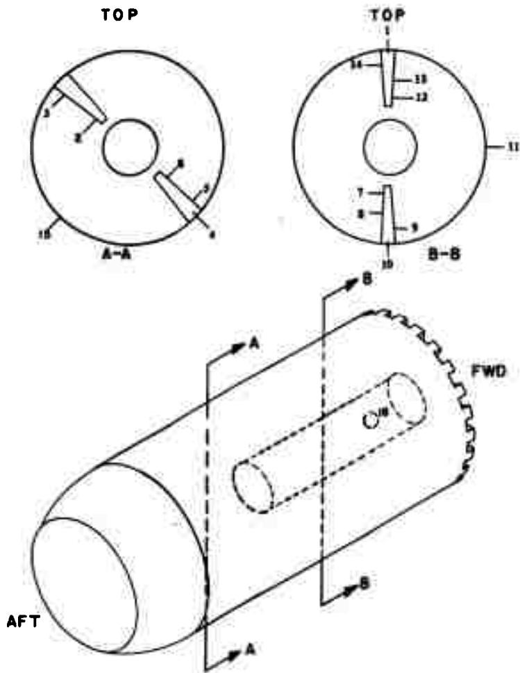
FIG. 3. Thermocouple Location in Bullpup Rocket Motor.
