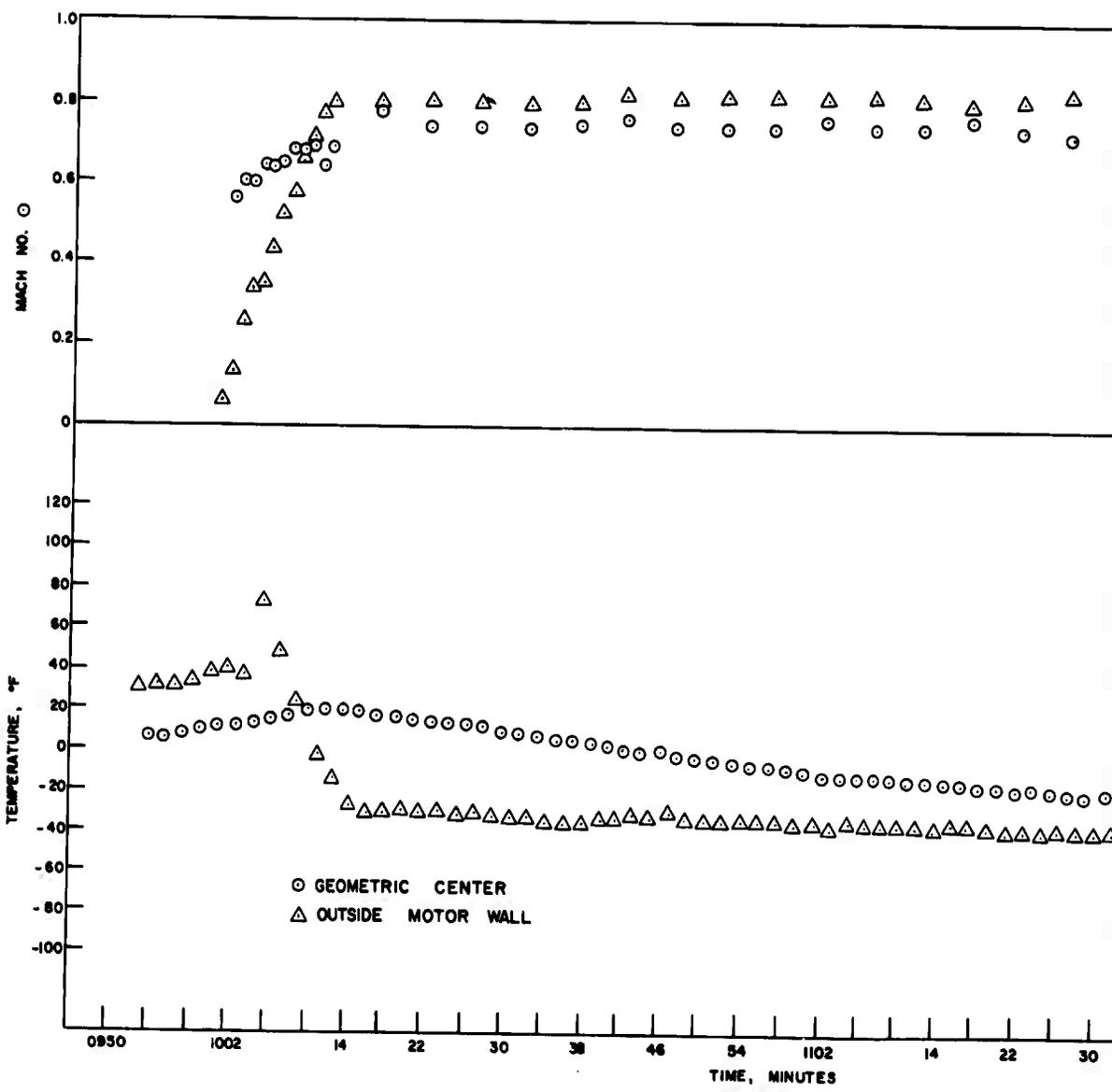
FIG. 10. Aerodynamic Cooling Profile for 12-Inch Diameter Liquid Propulsion
