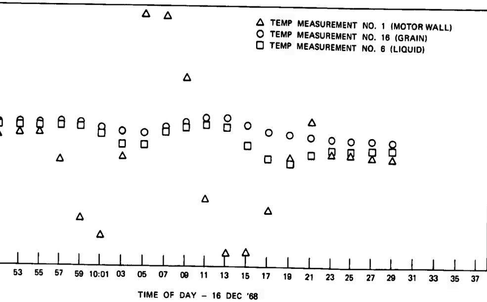
5. Aerodynamic Heating Profile for 12-Inch Diameter Liquid Propulsion Systems.
