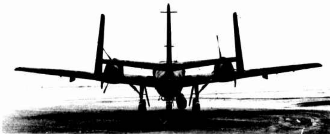
Photo 3. Rear View of IR Suppression Kit Installation.
