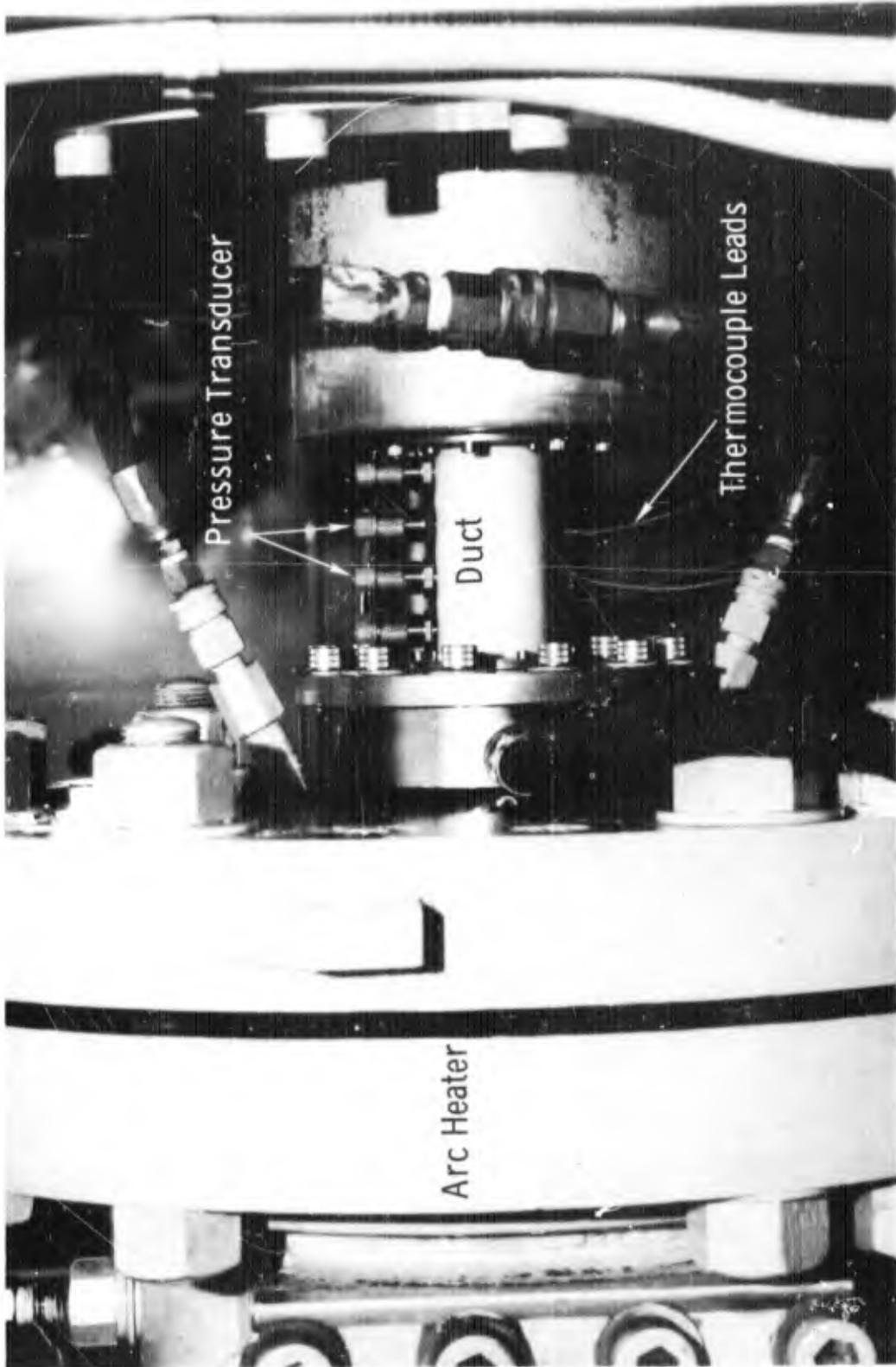
(U) FIG. 3 Experimental Set-up of Teflon Duct
