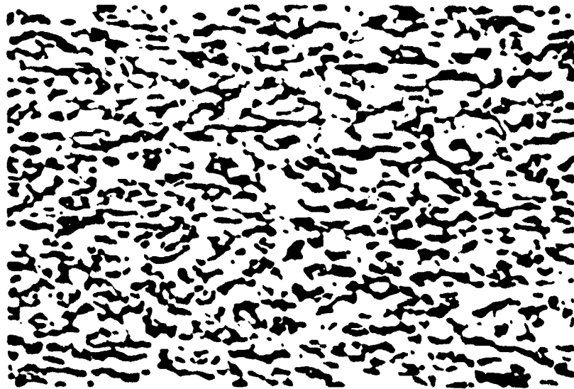
Ti-6Al-2Sn-4Zr-2Mo, Solution Treated and Aged Etchant: HF, HNO 3 , Glycerol Mag.: 500X
