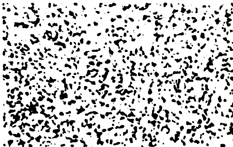
Titanium 679, Solution Treated and Aged
