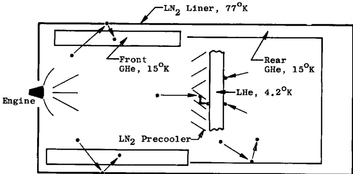
The front GHe cryosurfaces consist of fifty-two 8- by 1-ft panels positioned in a radial array about the axis of the chamber. The rear GHe cryosurface is 8 ft long and 6 ft in diameter. The supply of the gas to the front or rear GHe cryosurfaces could be distributed by externally operated valves.
