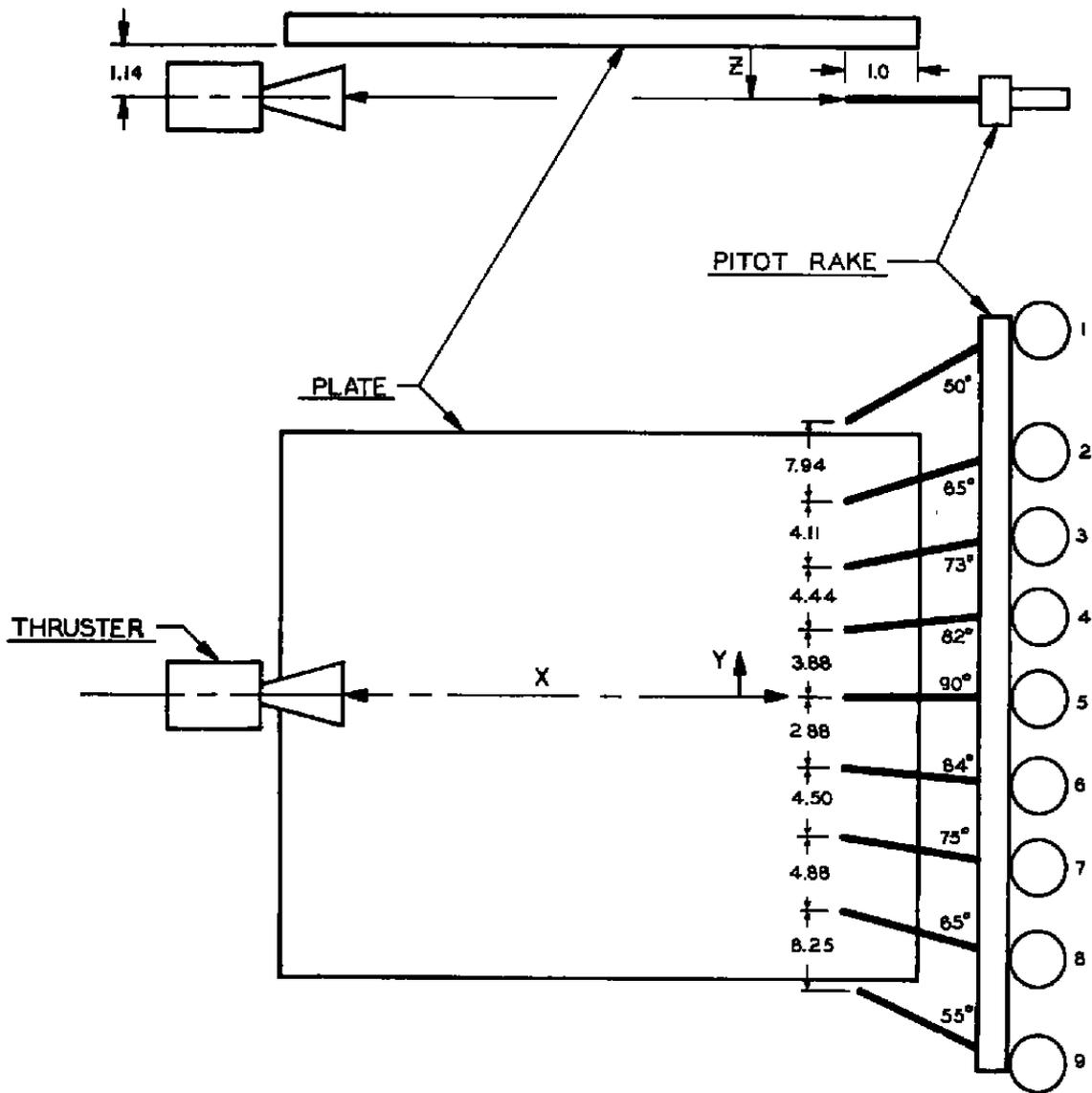
Fig. 5 Pitot Probe Rake with Plate
