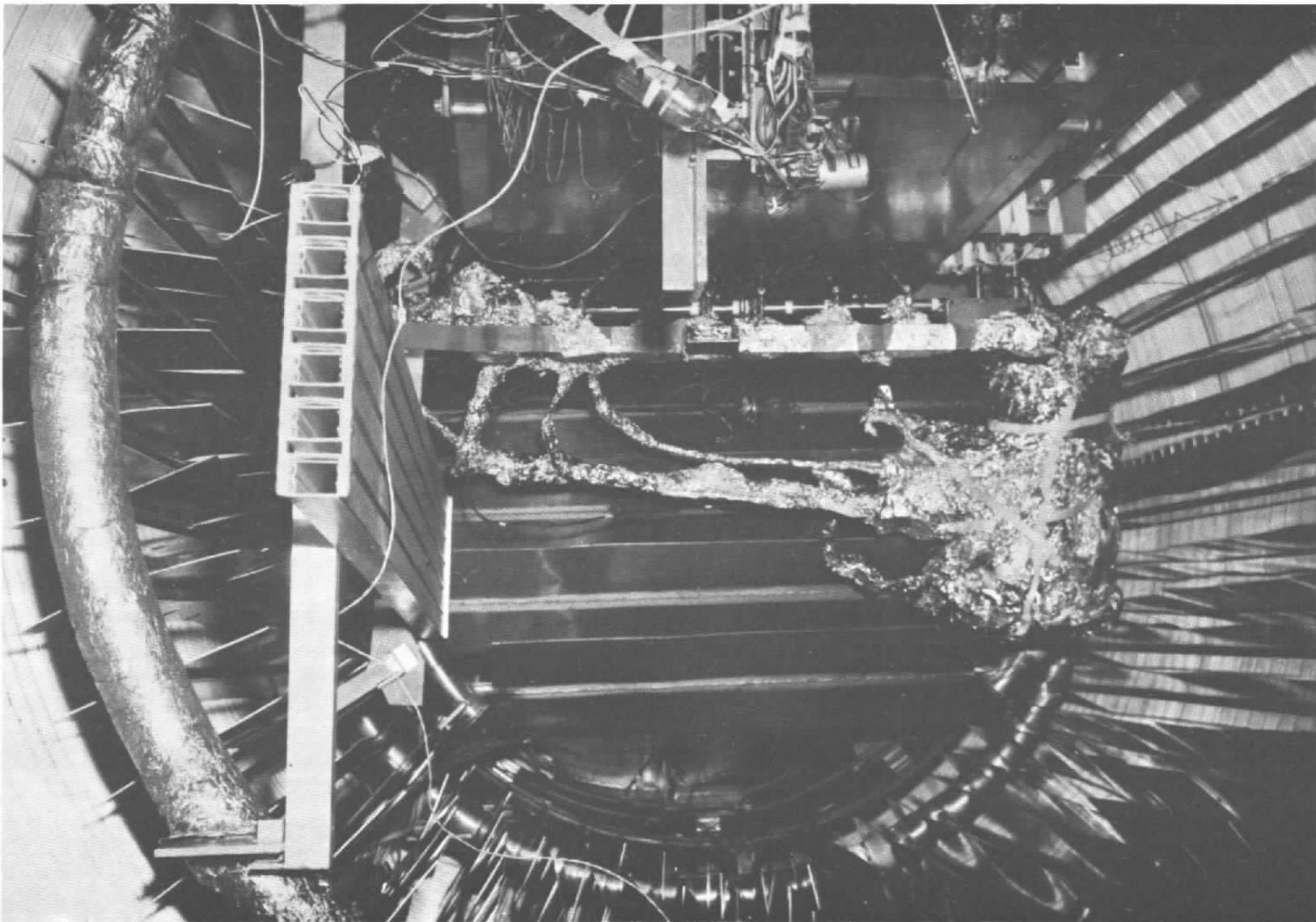
Fig. 6 Test Installation - Thruster, Plate, and Pitot Rake
