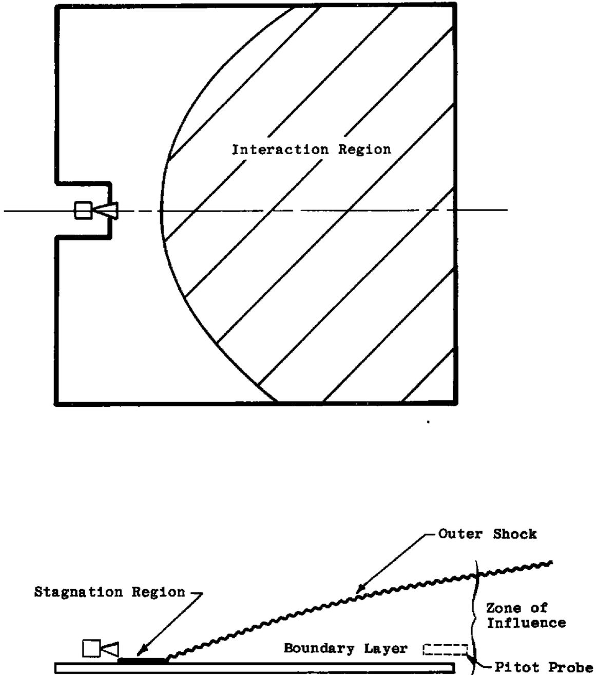
Fig. 16 Impingement Pattern on Plate
