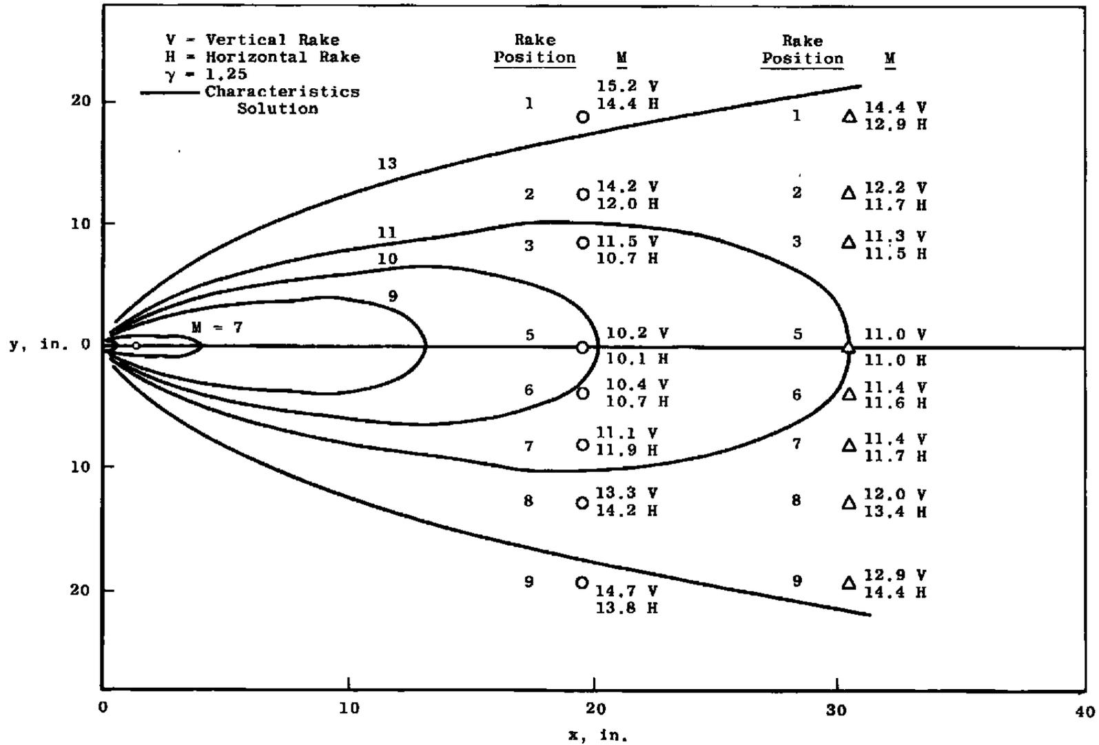
Fig. 13 Mach Number Contours for 1-lb-Thrust Engine
