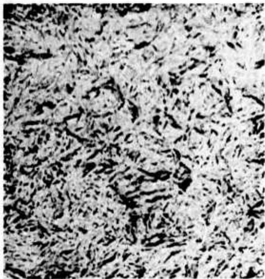
Figure 27. Typical Core Microstructure for the Four Gear Forging Processes.
