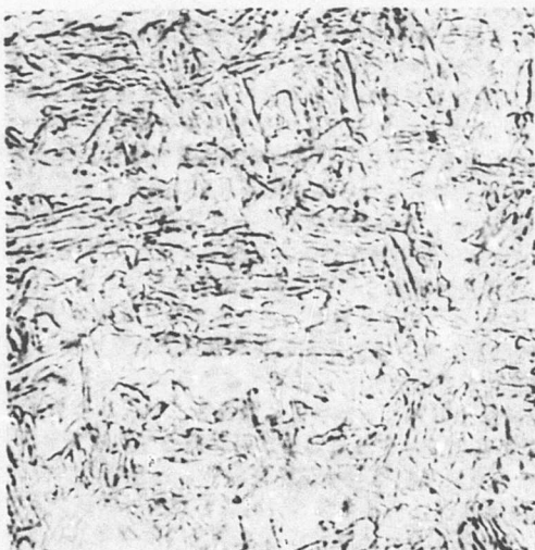
Figure 26. Typical Case Microstructure for the Four Gear Forging Processes.
