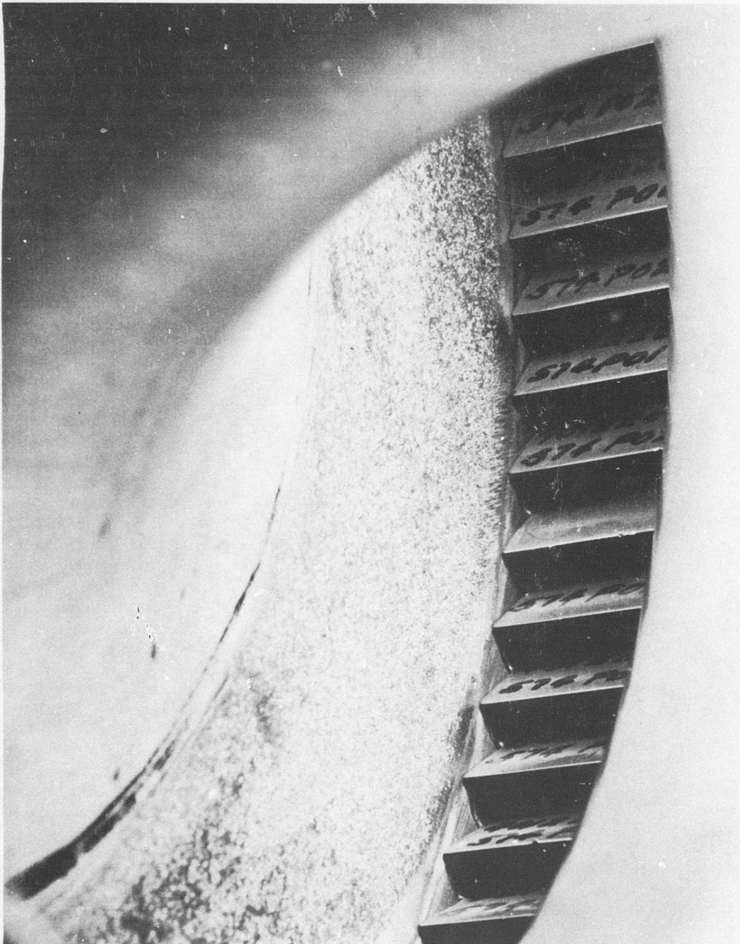
Figure 175. Rotor Blade Leading Edges Showing FOD Encountered During Tests of Buildup A - Sector 2.
