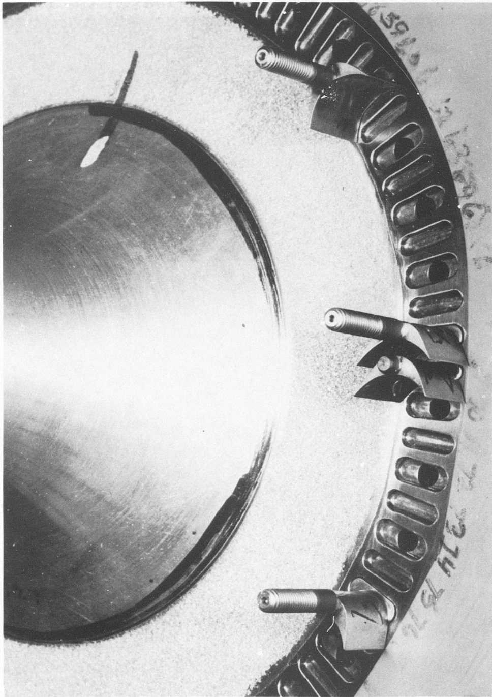
Figure 156. Trial Assembly of Alternate Long Shank and Short Pin Rotor Blades in Rotor Disc.
