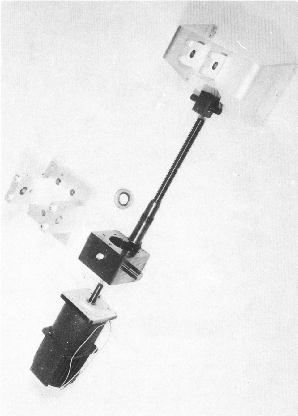
Figure 149. Motor, Reduction Gear, Pivotal Mounting, Drive Screw and Bracket for Actuating Supersonic Stator Blades.
