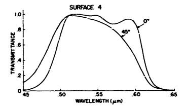
The first graph, beside the diagram, shows the computed transmittance for unpolarized light at normal incidence and at 45° for one of the wide-passband filters on a plane substrate. This would correspond to a 90° full field lens with a before-the-lens filter.
