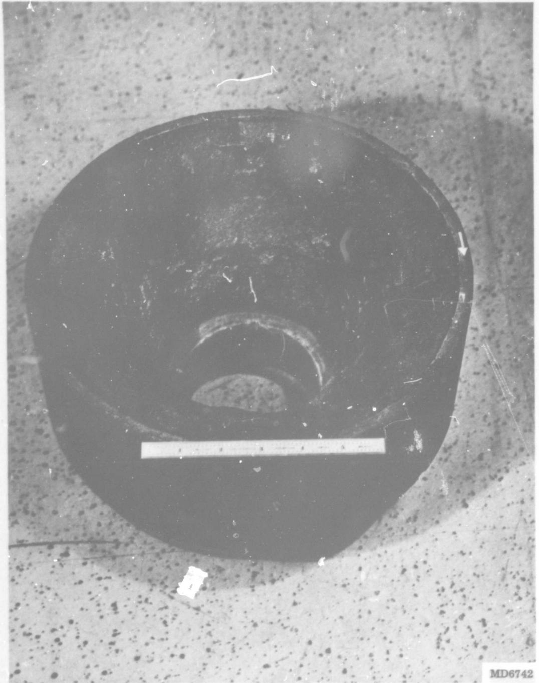
Figure 121. Nozzle No. 6 Postfired Inlet (View B)
