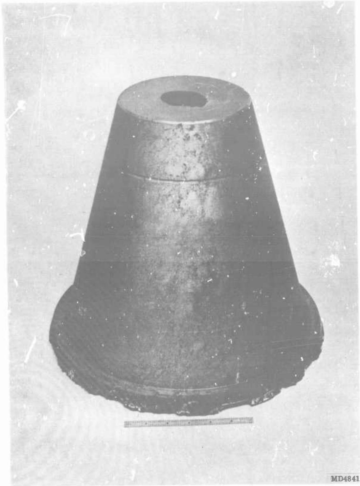
Figure 36. Nozzle No. 3 Exit Cone
