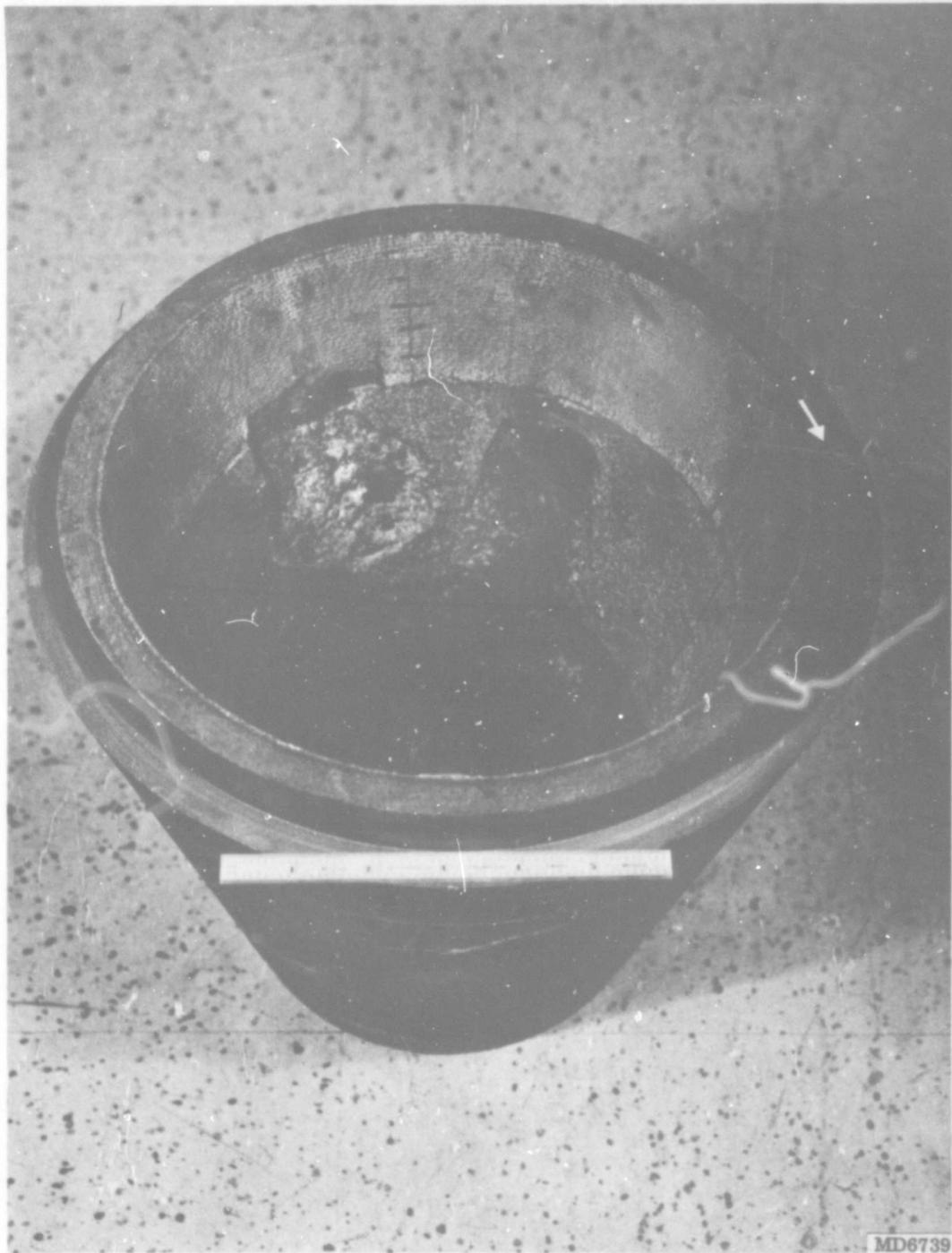
Figure 124. Nozzle No. 6 Postfired Throat Exit Ring
