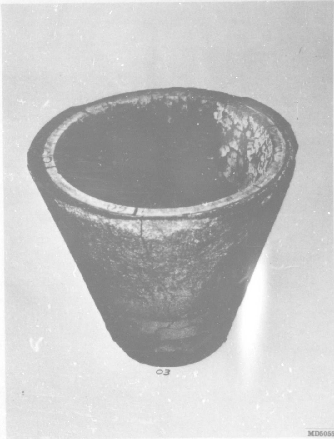
Figure 62. Nozzle No. 3 Postfired Condition, Exit Cone
