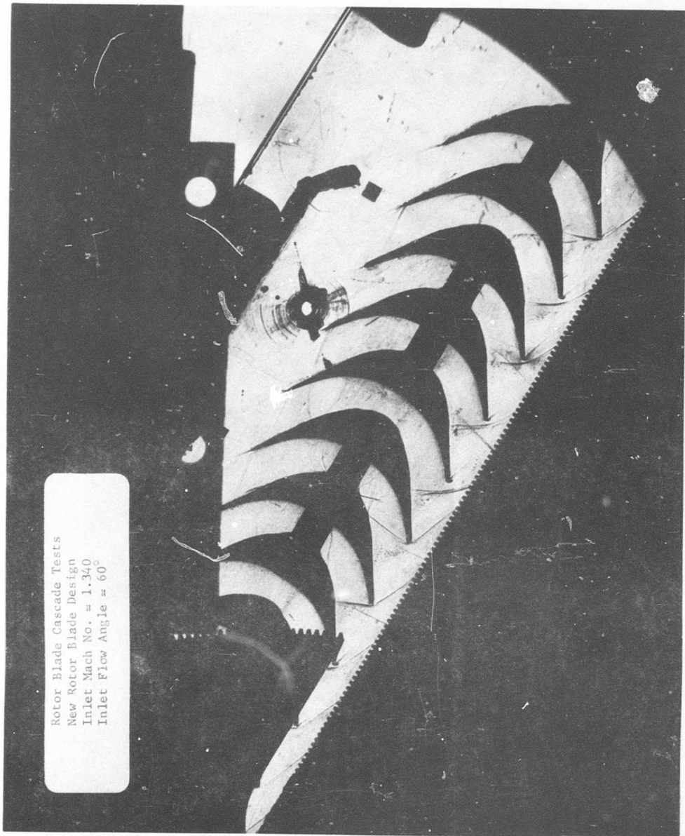
Figure 81. Schlieren Photograph, Rotor Blade Cascade Tests, Case Number 21984.
