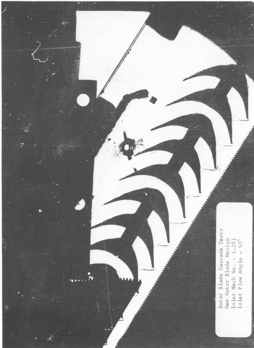
Figure 80. Schlieren Photograph, Rotor Blade Cascade Tests, Case Number 21983.
