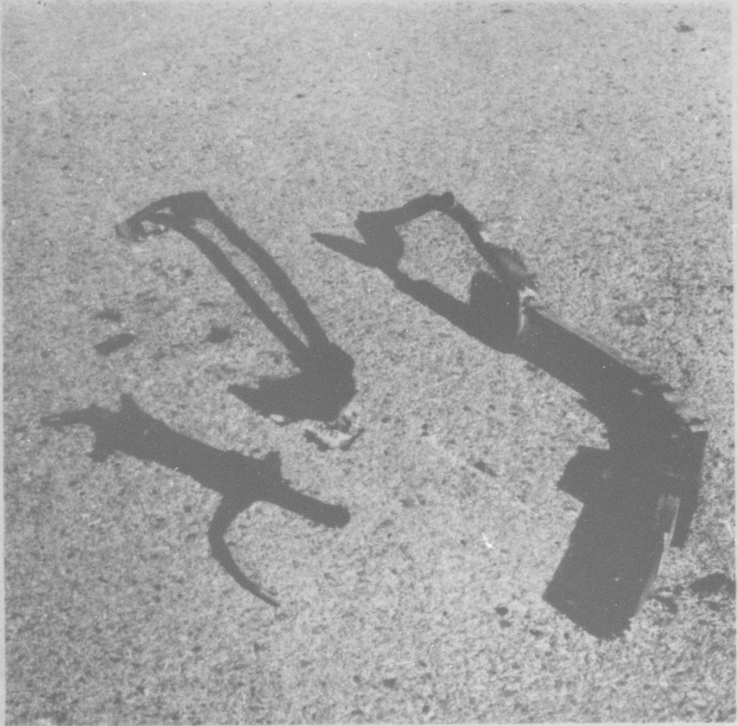
Figure 22. Remains of Materials Test Fixture
