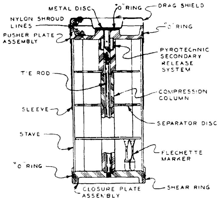
Figure 4. Cross Section of the Barrel Stave Canister
