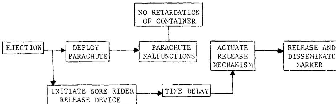
Figure II-2. Sequence of Operation of Concept A
