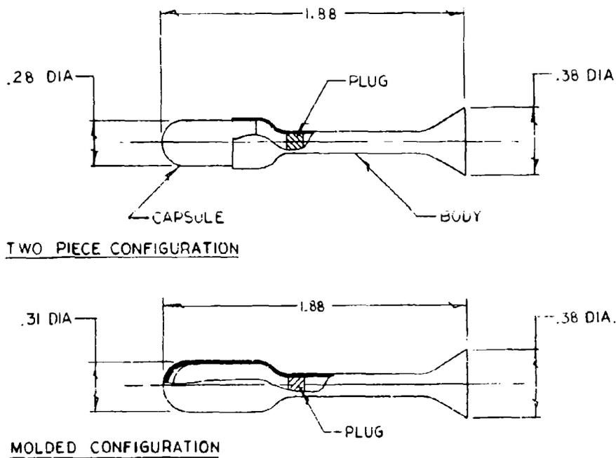
Figure I-6. Proposed Flechette Marker Configurations
