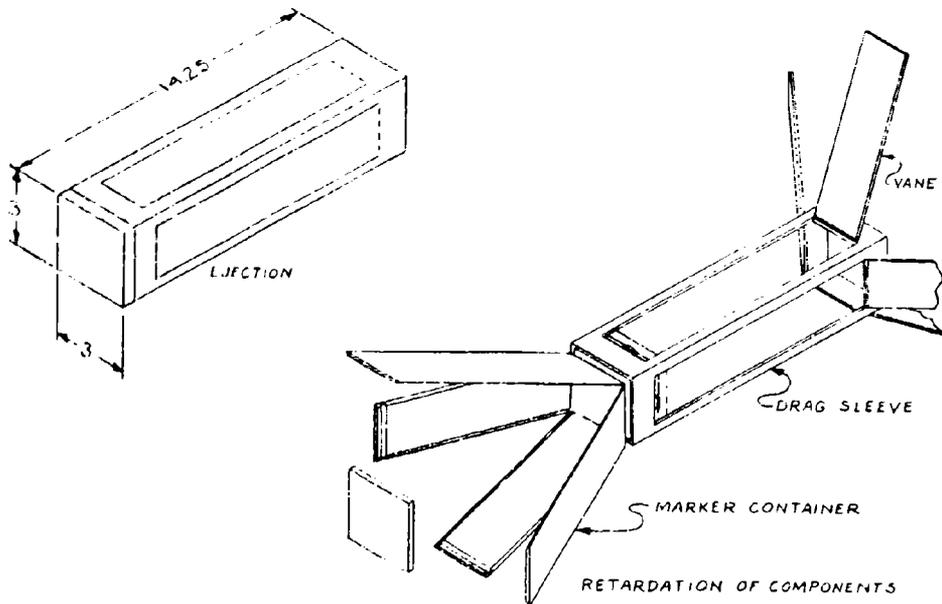
Figure IV-5. TFD Munition Autorotating Vane and Staves Concept
