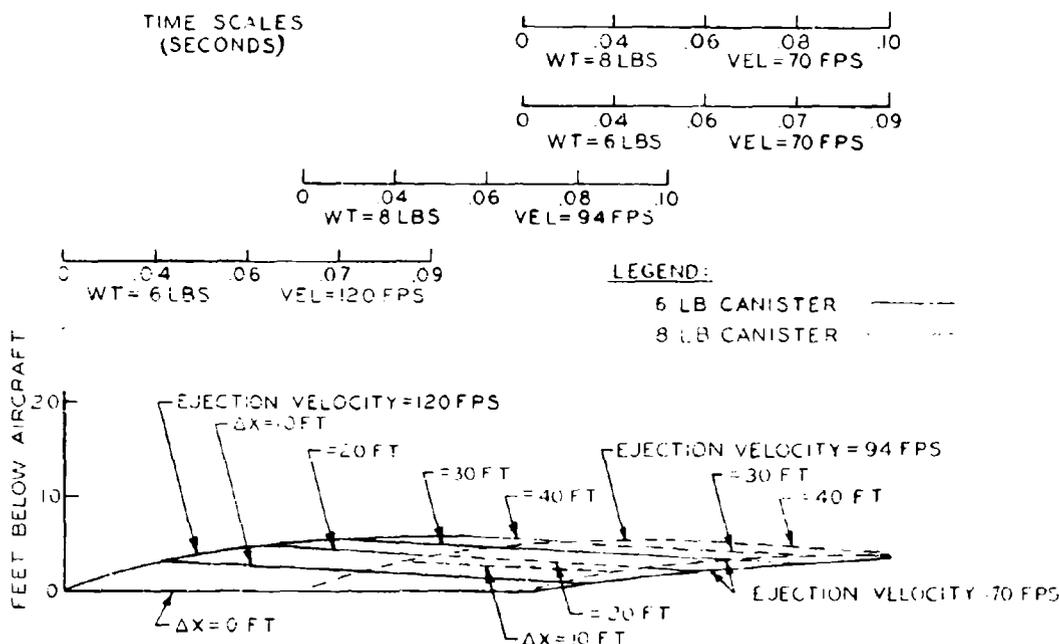
Figure II-9. Safe Separation Distance for a Parachute Munition
