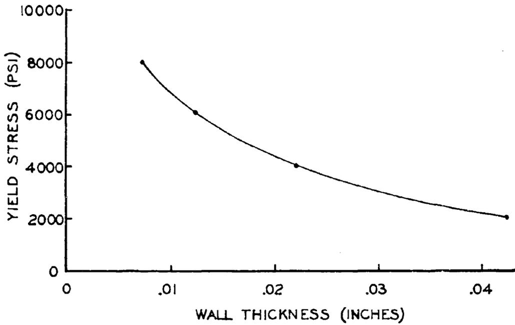
Figure III-1. Wall Thickness to Withstand Aerodynamic Force
