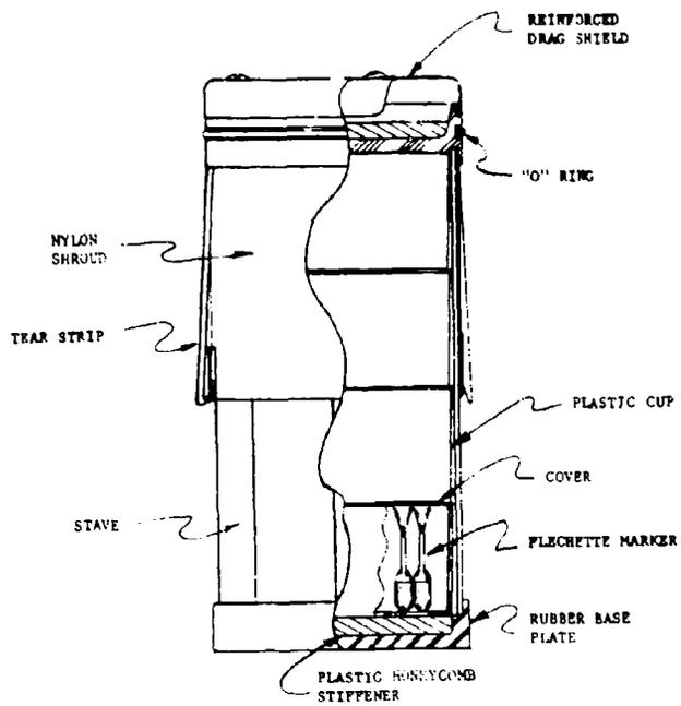
Figure 5. Barrel Stave Canister Rems II
