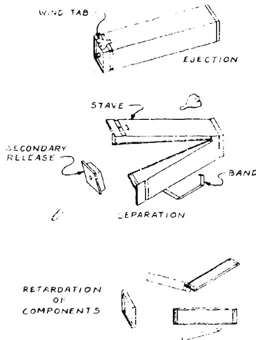
Figure IV-6. Operating Sequence of TFD Munition Stave Concept
