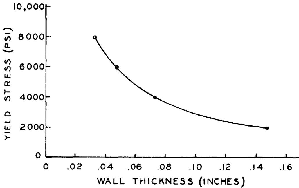
Figure III-2. Wall Thickness to Withstand Downward Ejection Force
