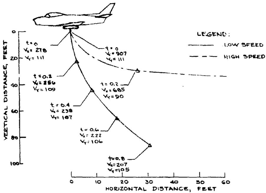
Figure VI-2. Safe Separation of Ejected Munition from Aircraft
