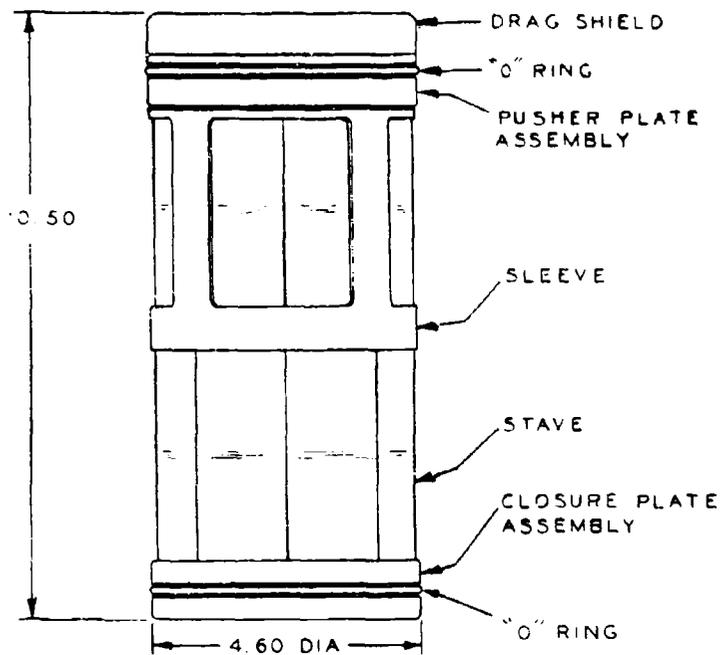
Figure 3. External Configuration of the Barrel Stave Canister
