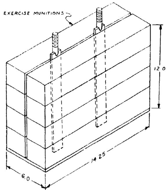
Figure IV-1. TFD Muniton per Bay Loading
