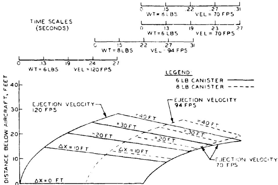
Figure II-7. Safe Separation Distance for a Non-Tumbling Munition
