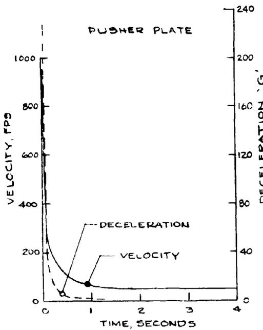
Figure II-14. Pusher Plate Deceleration
