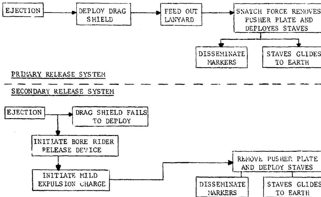
Figure II-6. Sequence of Operation of Concept C
