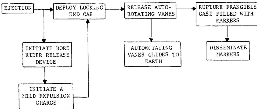
Figure II-4. Sequence of Operation of Concept B
