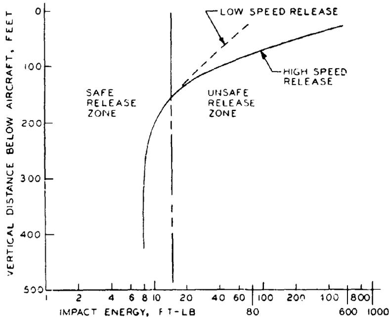
Figure II-12. Dynamic Characteristics for a Stave Munition System
