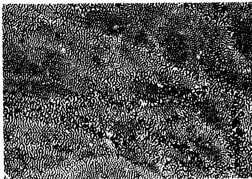
FIGURE 6. MICROSTRUCTURE IN CENTER OF SPECIMEN T50-27 ANNEALED 100 HOURS IN ARGON AT 1800 F
