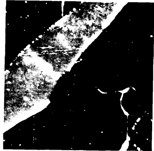
N6590 Dark Field Illumination X250 (a) Heat H-218 (71.5% Rh and 28.5% Mo)
