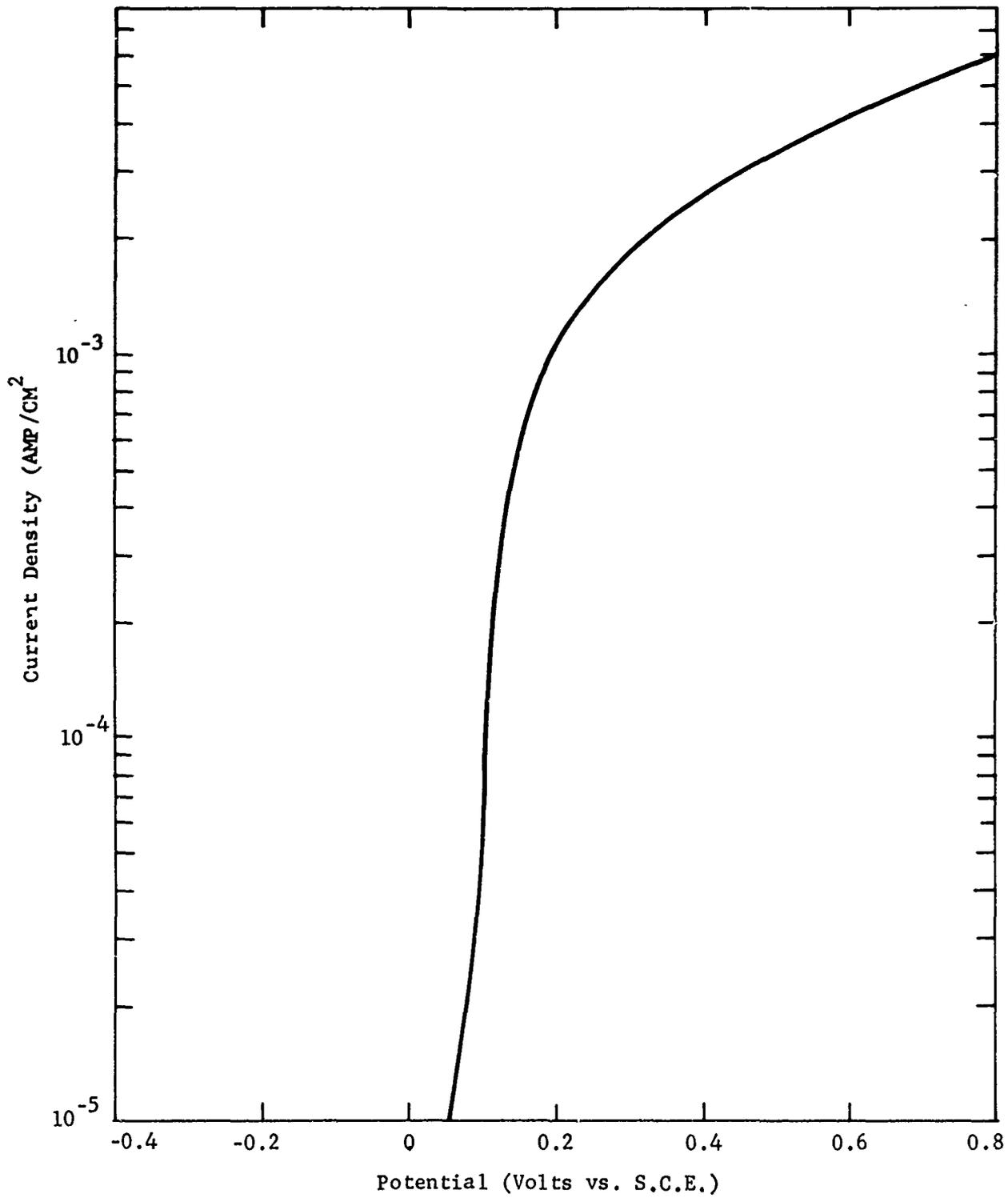
Figure 9. Anodic Polarization of ASTM B140 Alloy "A" in air-saturated tap water at 50C.
