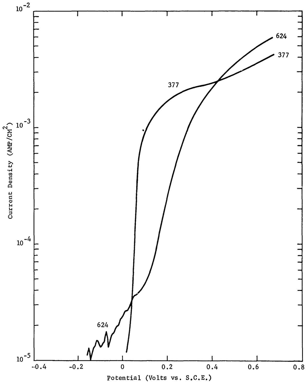
Figure 6. Anodic polarization of copper alloy 624 and copper alloy 377 in nitrogen-saturated tap water at 50C.
