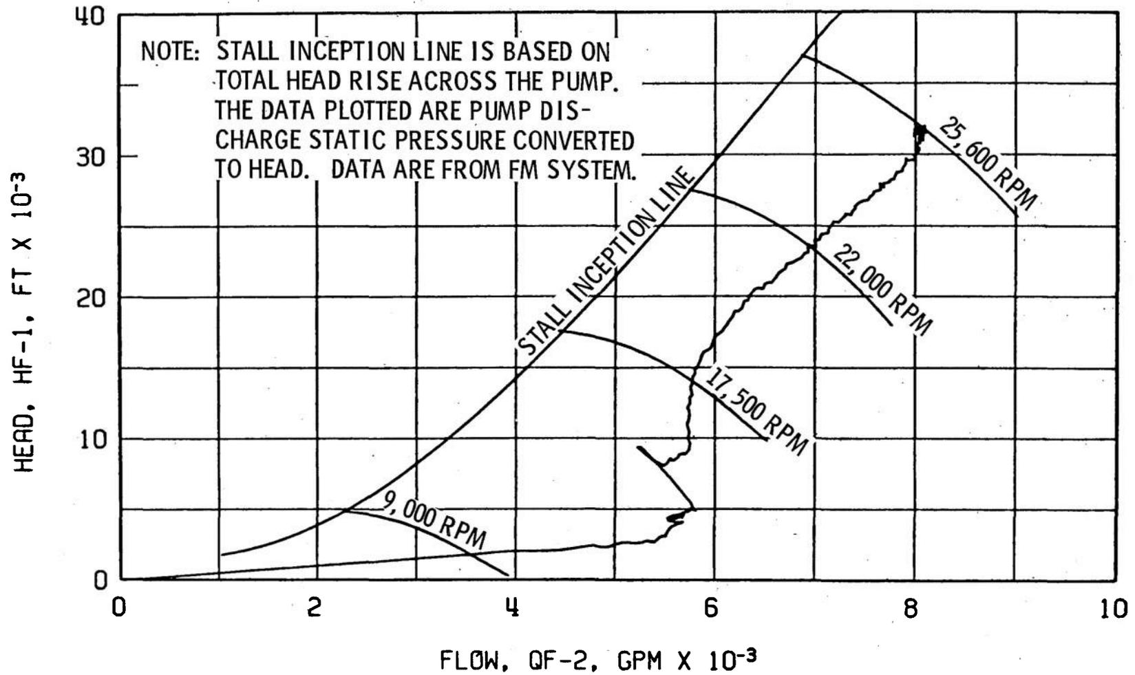
Fig. 18 Fuel Pump Start Transient Performance, Firing 39B
