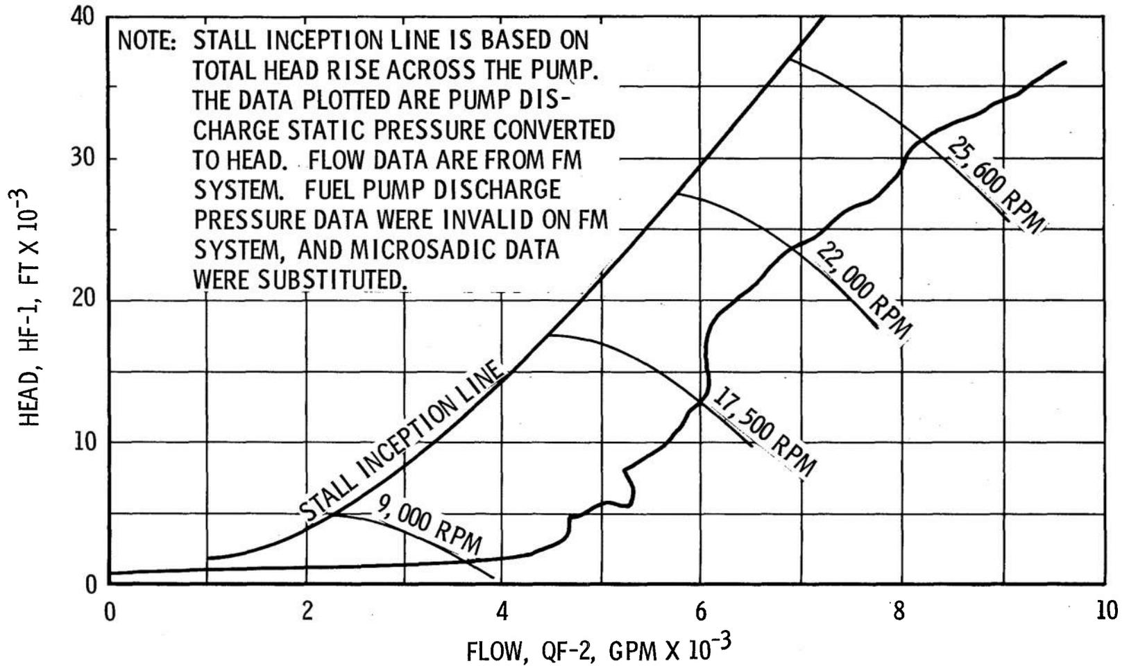
Fig. 35 Fuel Pump Start Transient Performance, Firing 40A
