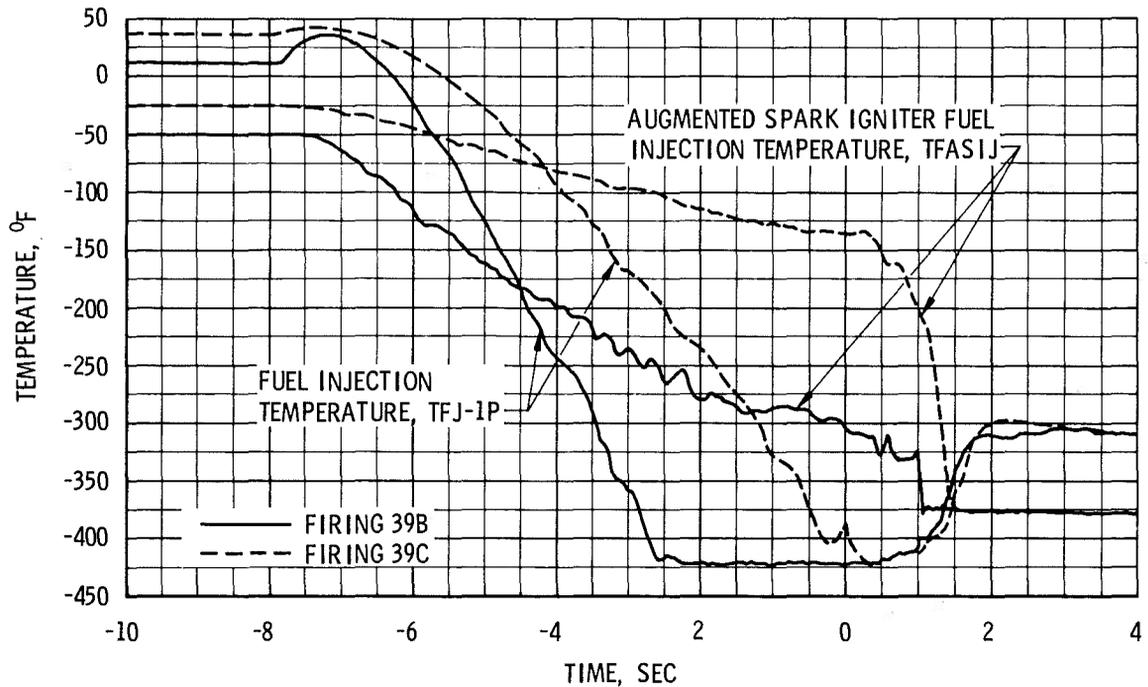
b. Augmented Spark Igniter Fuel Line Chilldown Rates
