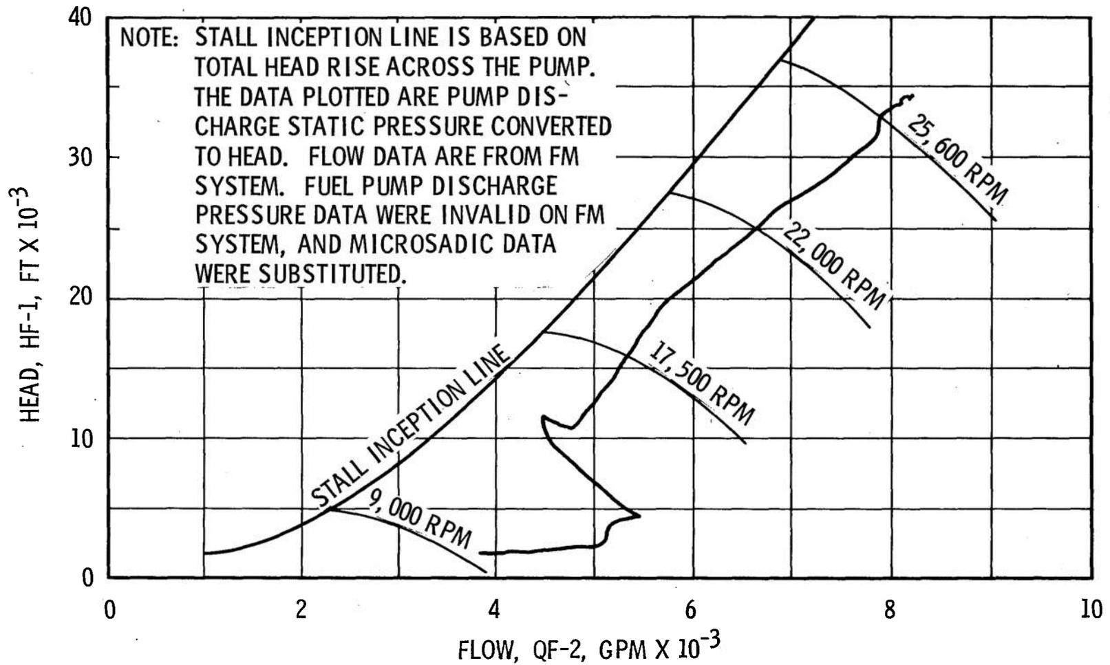
Fig. 55 Fuel Pump Start Transient Performance, Firing 41A
