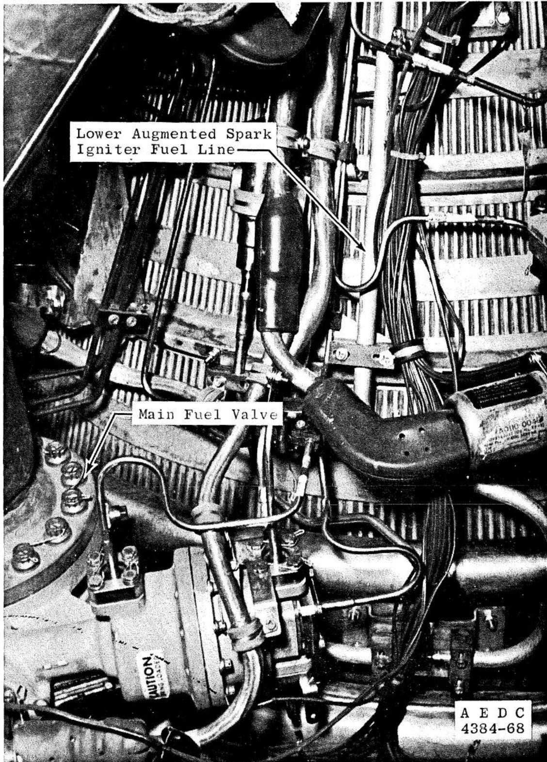
d. Lower Fuel Line Attachment Points to Thrust Chamber, Interim Configuration
