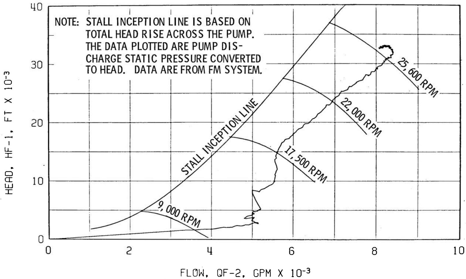
Fig. 43 Fuel Pump Start Transient Performance, Firing 40B
