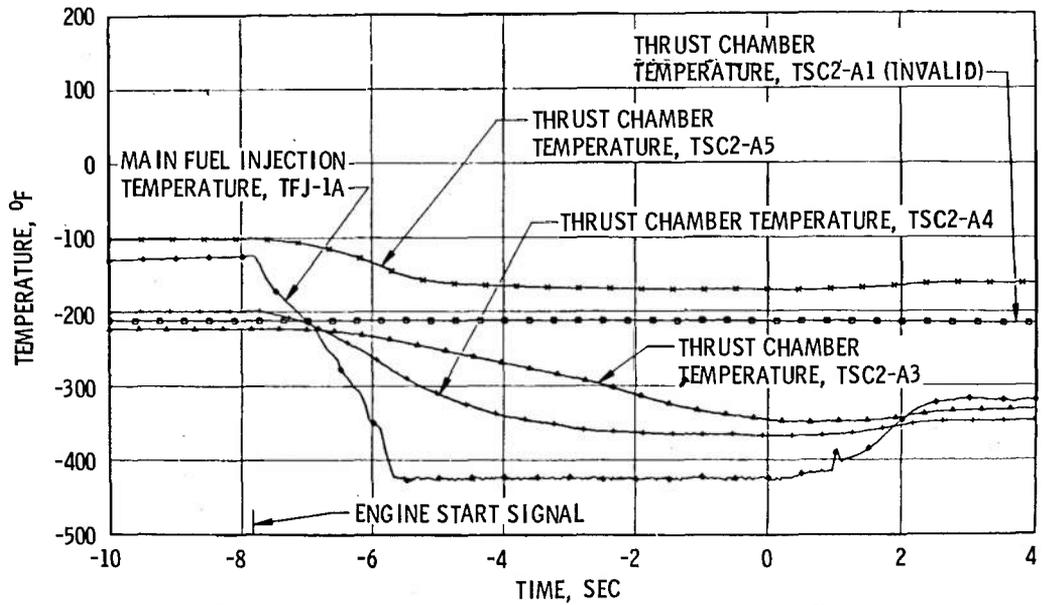
i. Thrust Chamber Temperature Transient, Start
