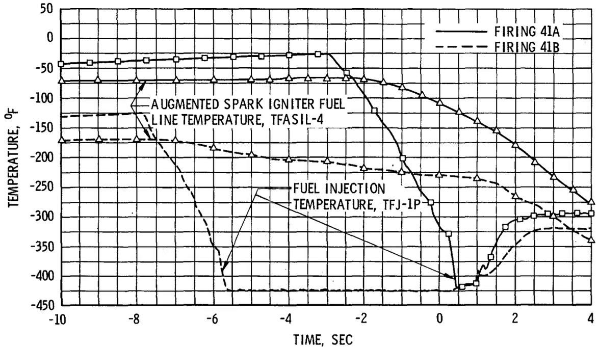
b. Augmented Spark Igniter Fuel Line Chilldown Rates, Firings 41A and 41B
