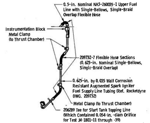
Original Augmented Spark Igniter Fuel Supply Line
