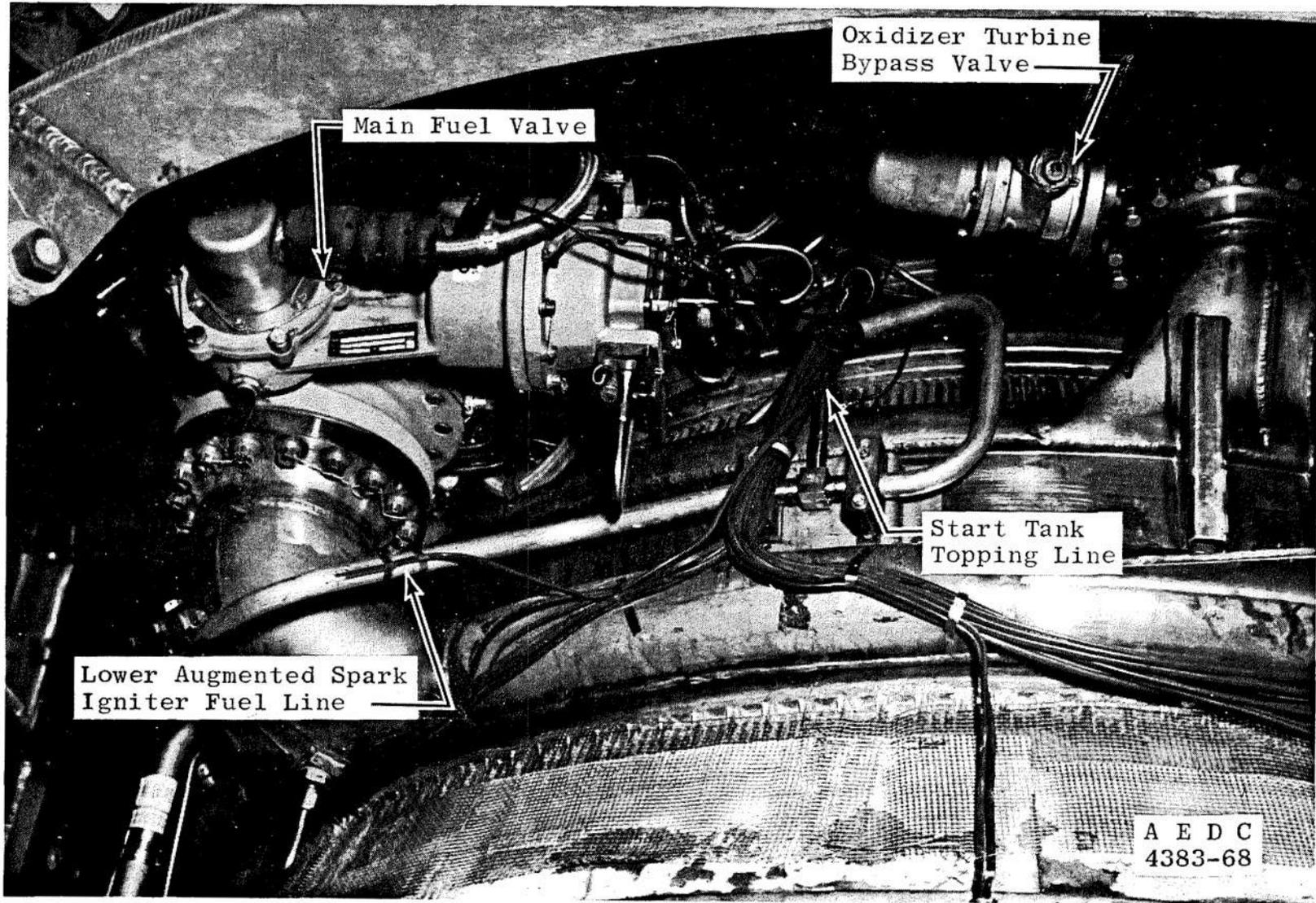
f. Lower Fuel Line and Start Tank Topping Line, Interim Configuration
