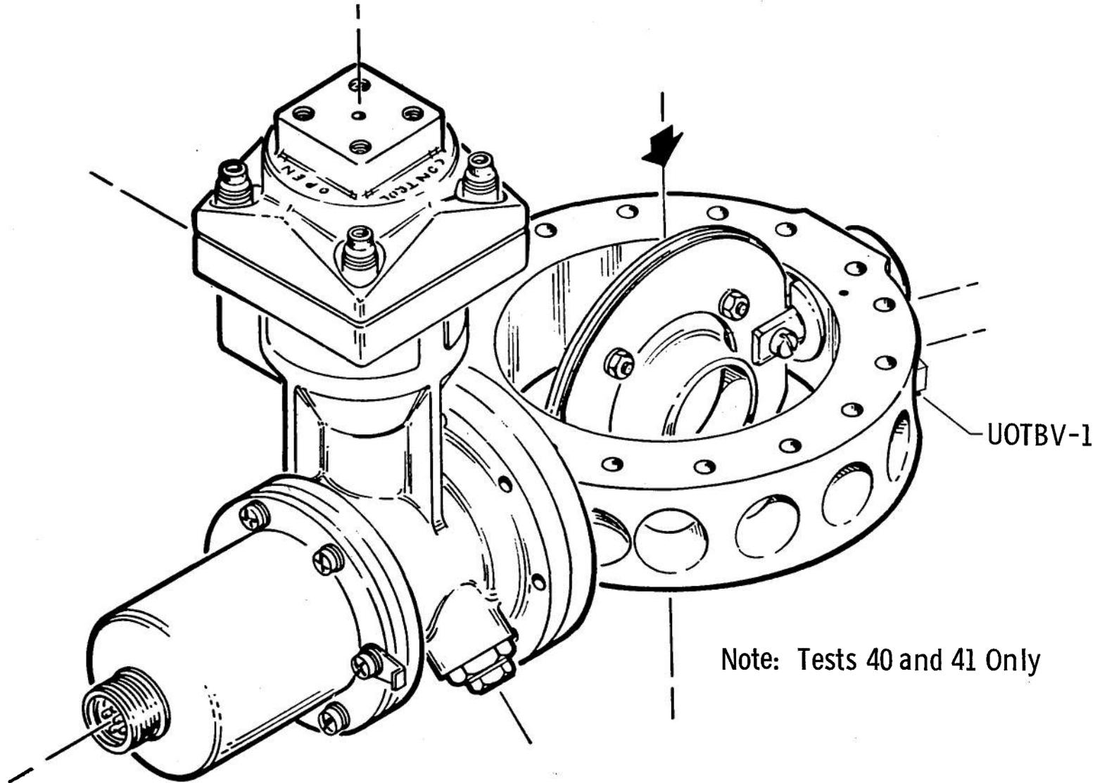
k. Oxidizer Turbine Bypass Valve Accelerometer
