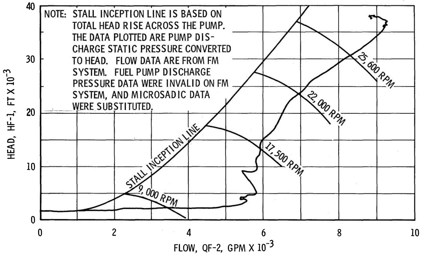
Fig. 39 Fuel Pump Start Transient Performance, Firing 40AA
