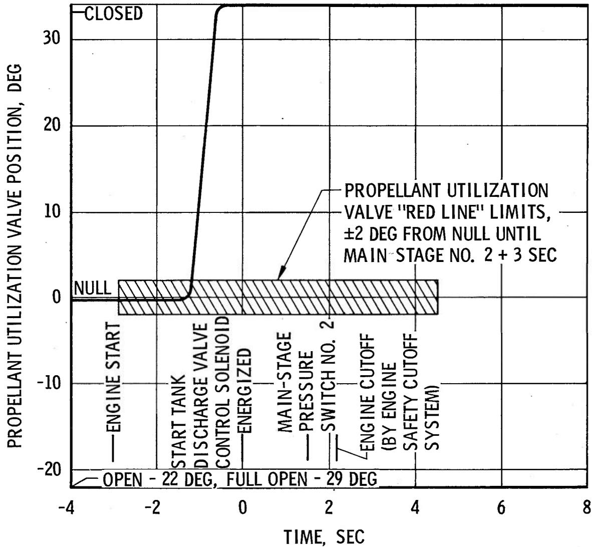
a. Propellant Utilization Valve Position History and "Red Line" Limits
