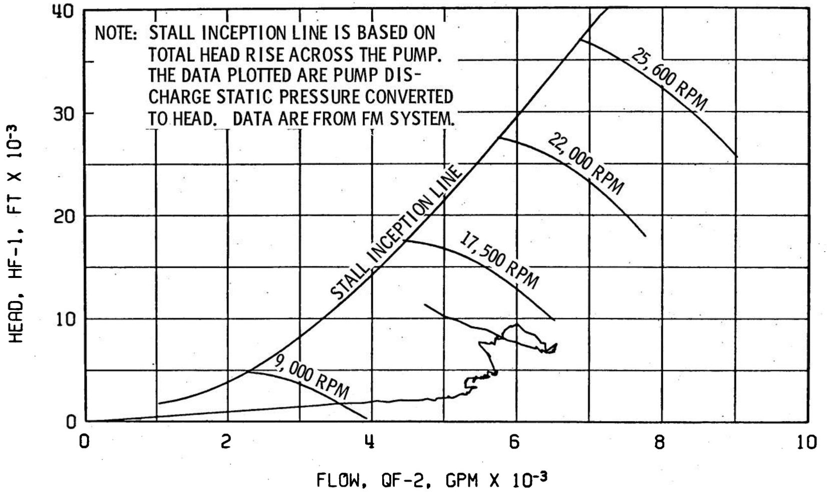
Fig. 30 Fuel Pump Start Transient Performance, Firing 39E
