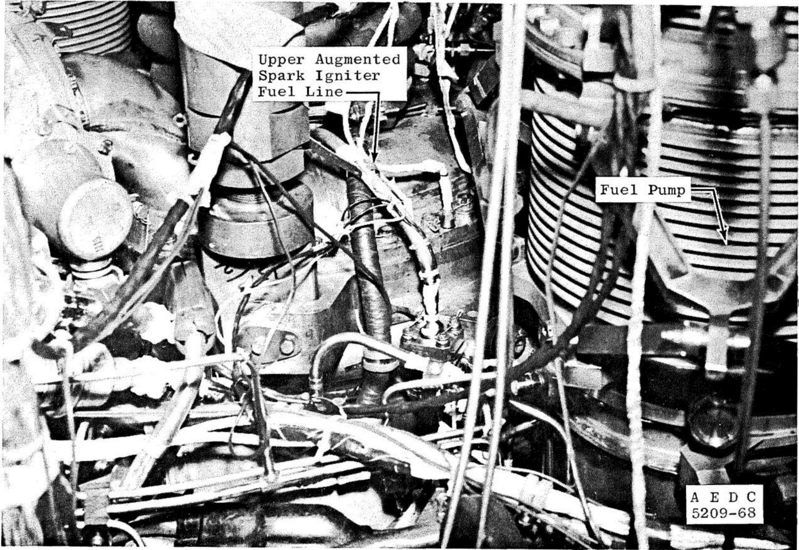
c. Upper Fuel Line Assembly, New Configuration
