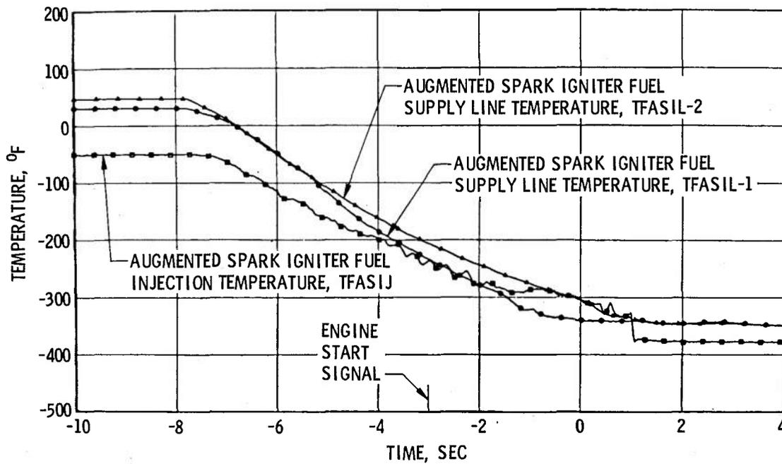
j. Augmented Spark Igniter Fuel Supply Line Temperature Transient, Start
