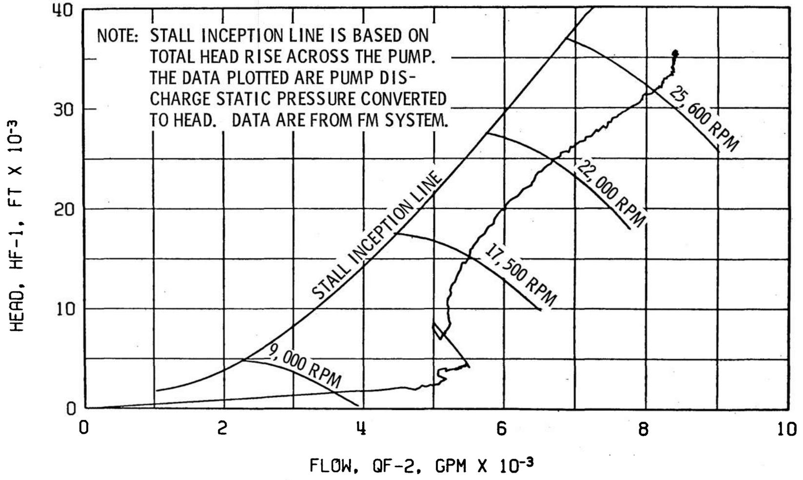
Fig. 14 Fuel Pump Start Transient Performance, Firing 39A
