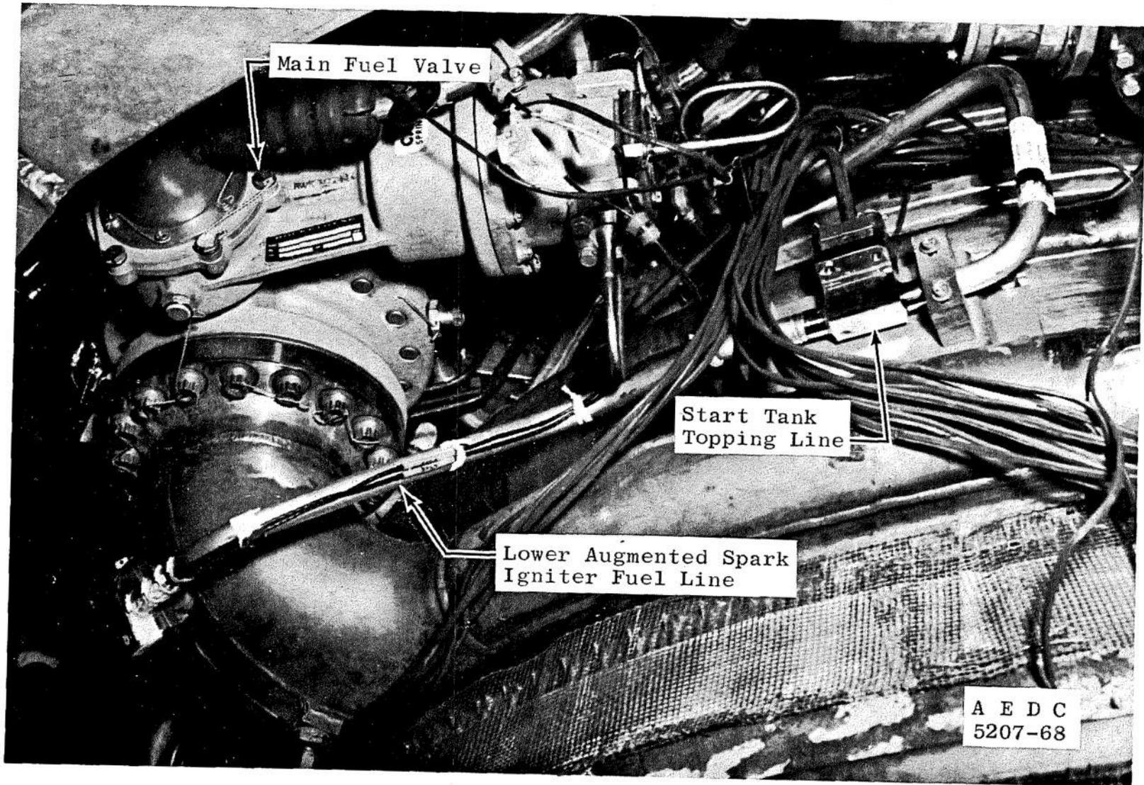
g. Lower Fuel Line and Start Tank Topping Line, New Configuration
