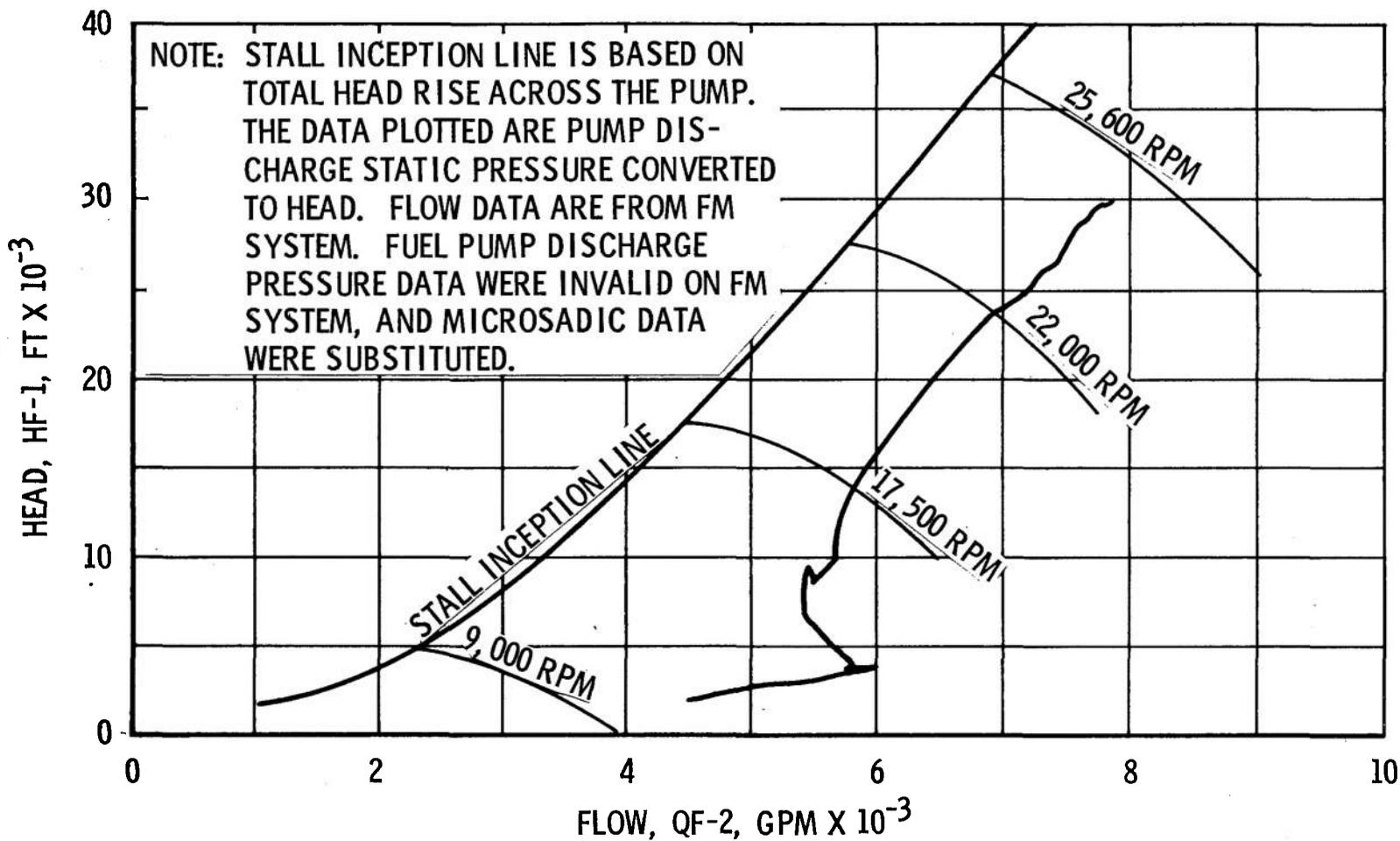
Fig. 59 Fuel Pump Start Transient Performance, Firing 41B
