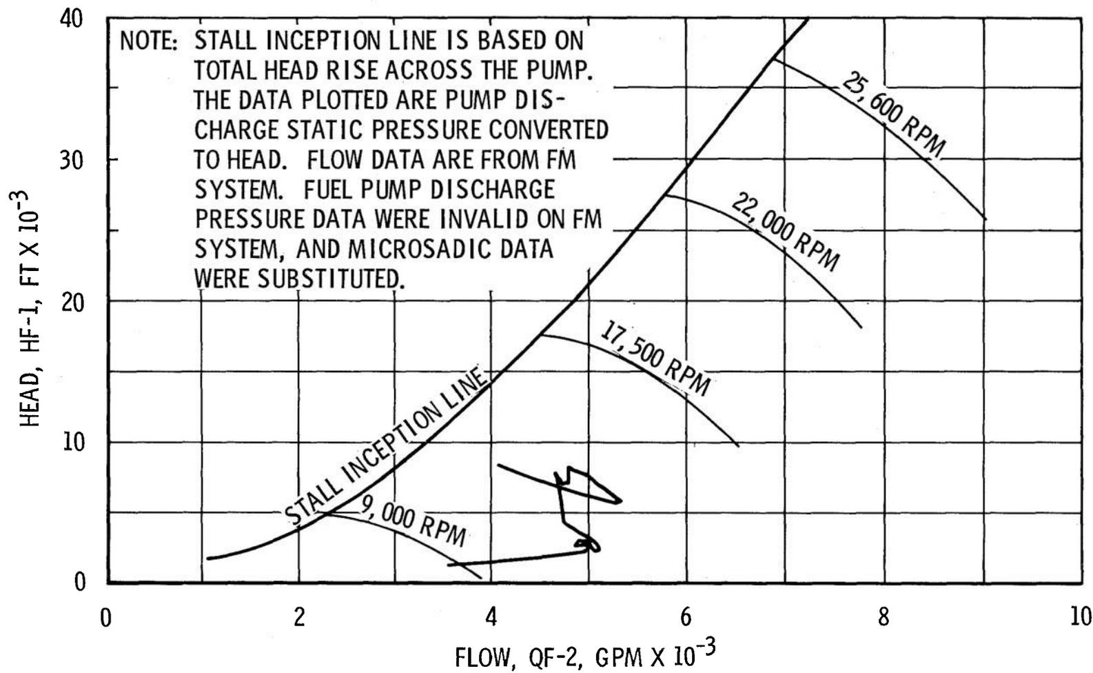
Fig. 67 Fuel Pump Start Transient Performance, Firing 41D
