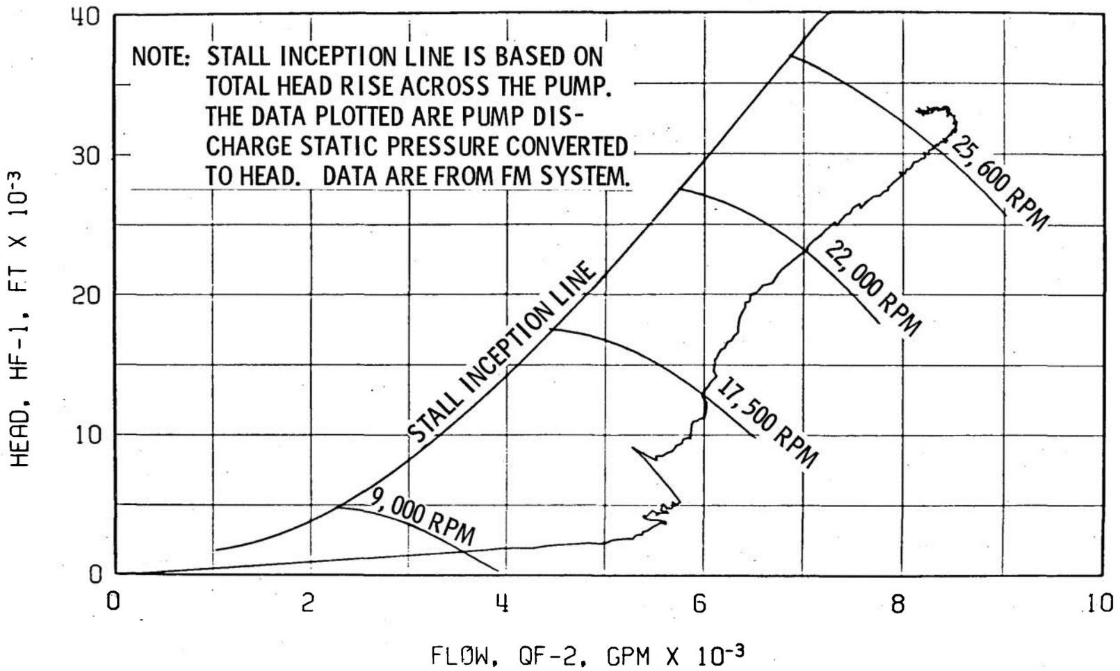
Fig. 51 Fuel Pump Start Transient Performance, Firing 40D
