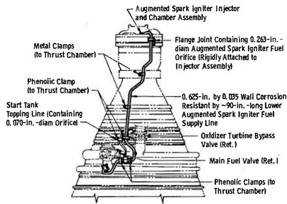
New Augmented Spark Igniter Fuel Supply Line
