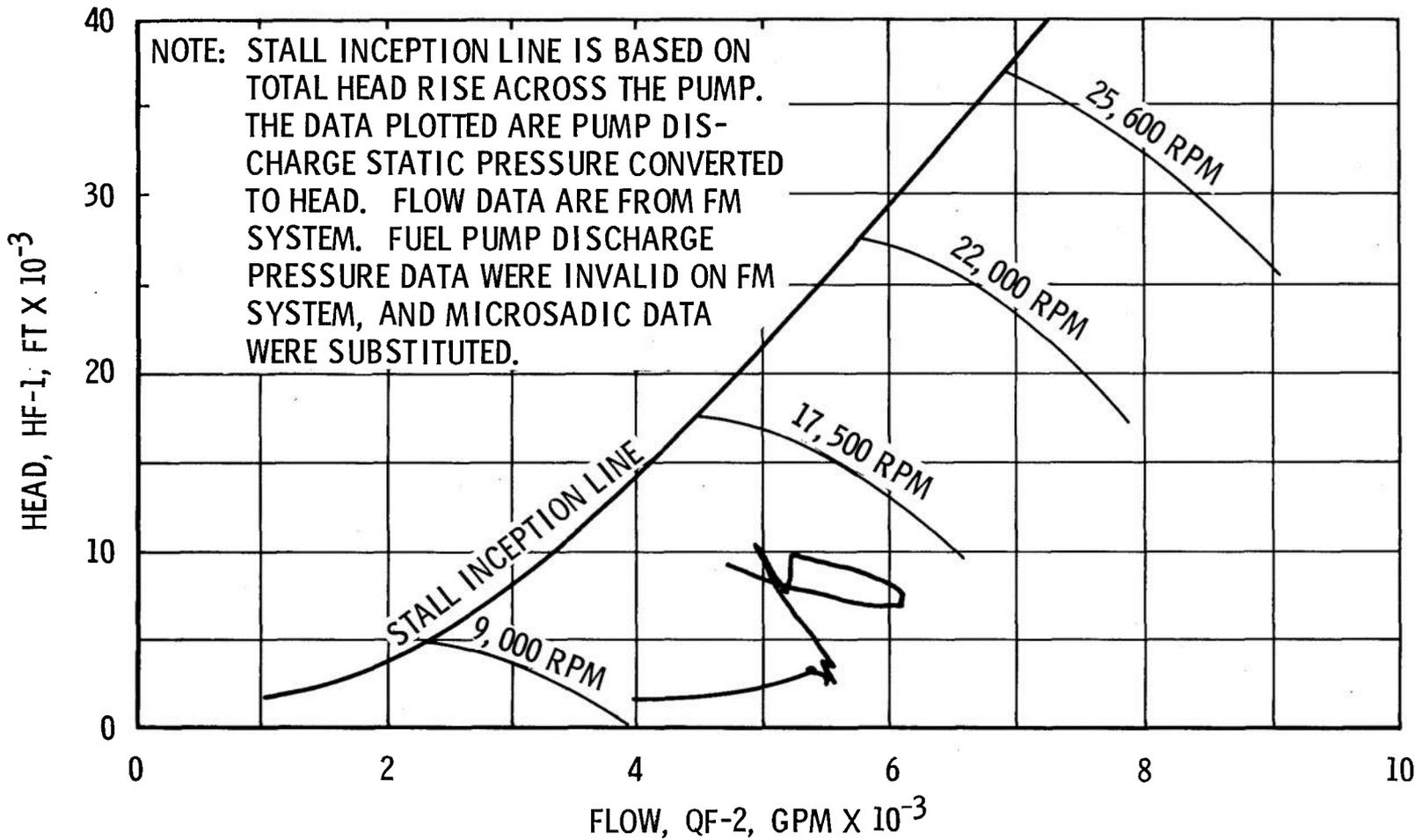
Fig. 63 Fuel Pump Start Transient Performance, Firing 41C
