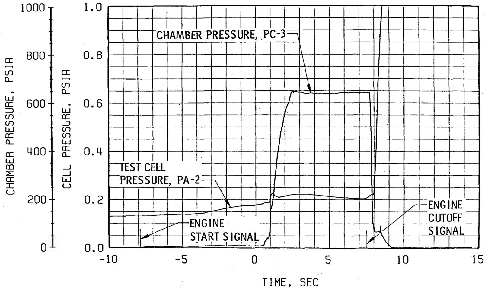
Fig. 50 Engine Ambient and Combustion Chamber Pressures, Firing 40D
