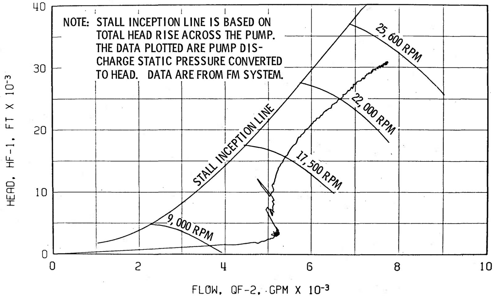
Fig. 47 Fuel Pump Start Transient Performance, Firing 40C
