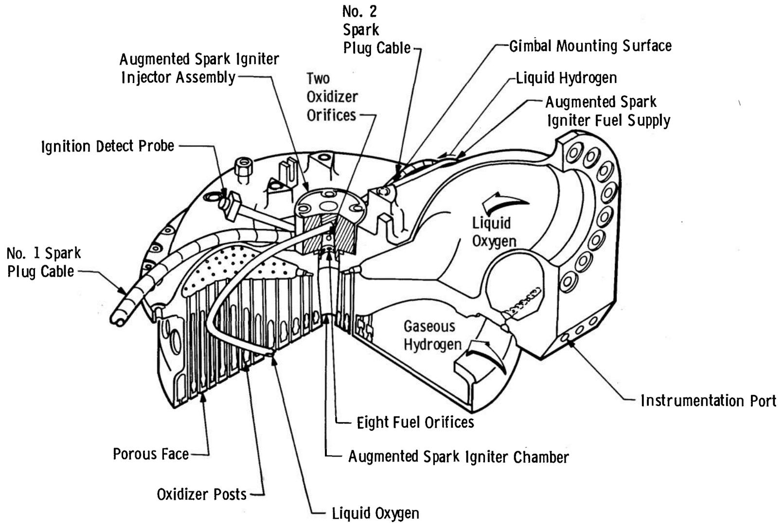
b. Details of the Augmented Spark Igniter Assembly and Main Chamber Injector
