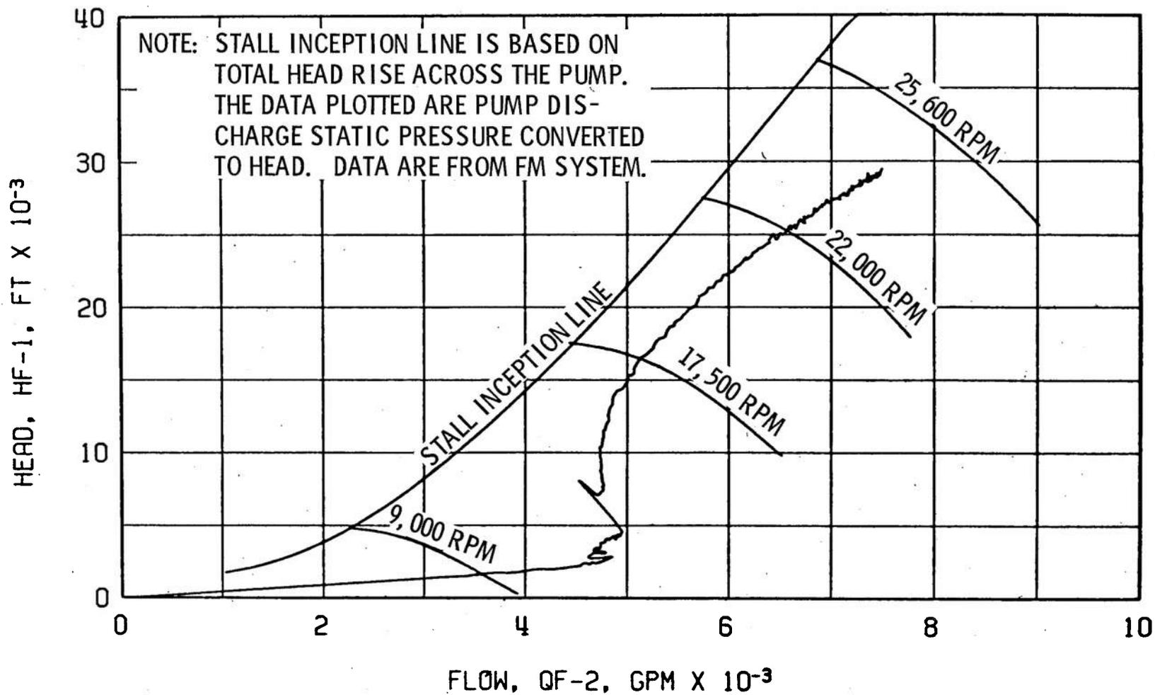
Fig. 22 Fuel Pump Start Transient Performance, Firing 39C
