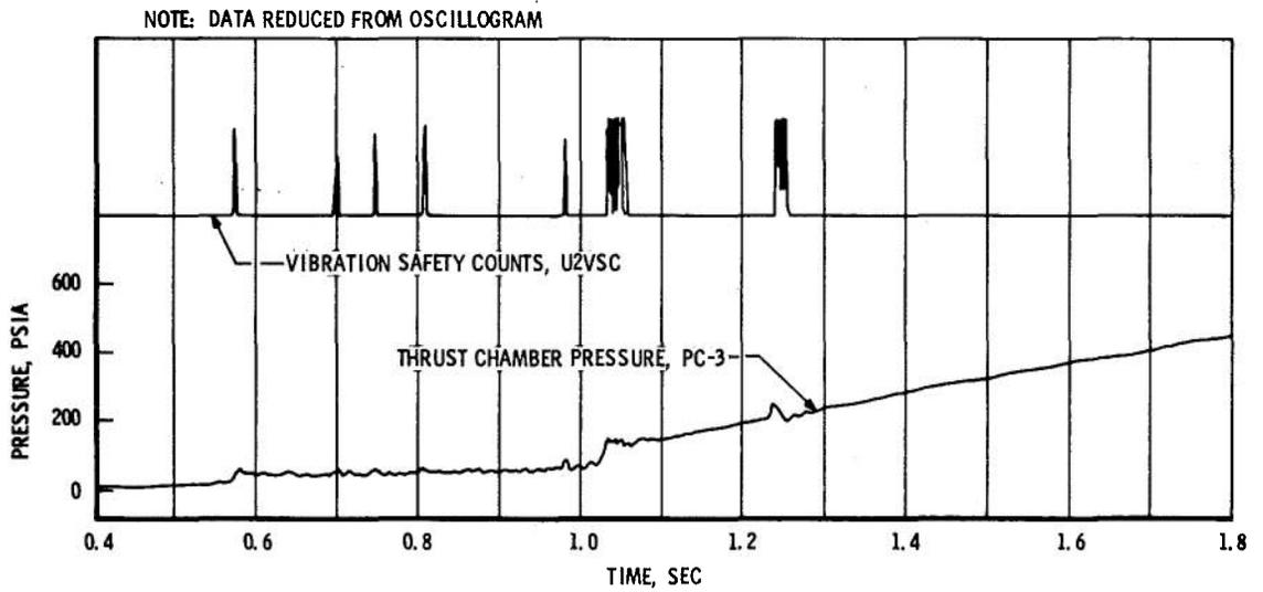
I. Augmented Spark Igniter Ignition Detect Probe Voltage and Thrust Chamber Ignition Transient
