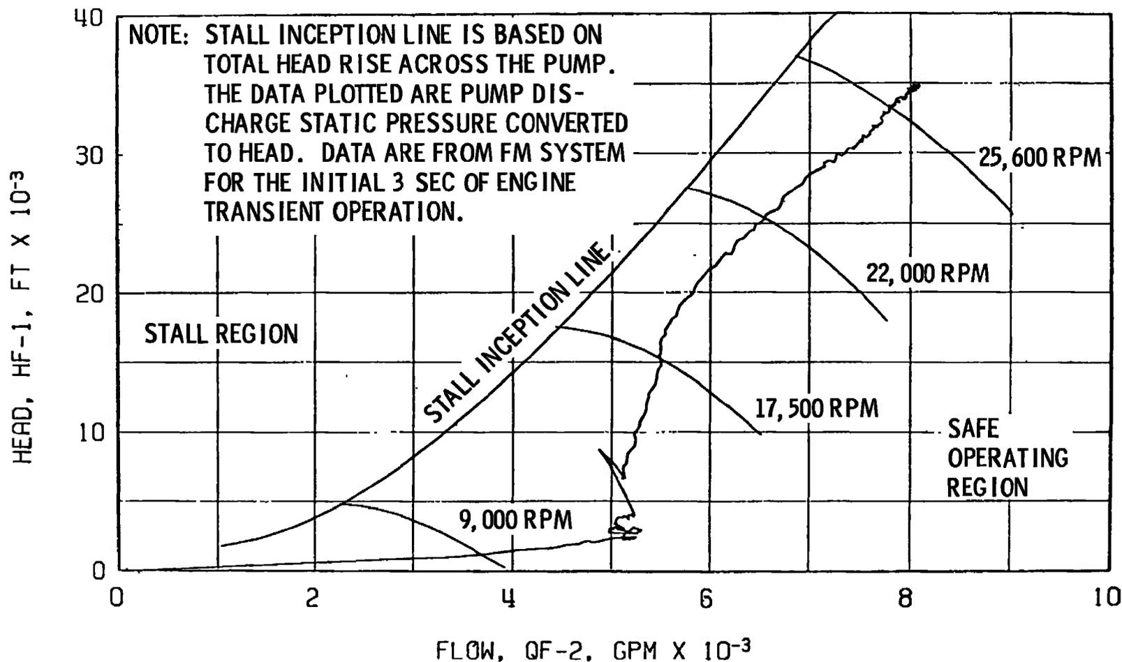
Fig. 18 Fuel Pump Start Transient Performance, Firing 42B
