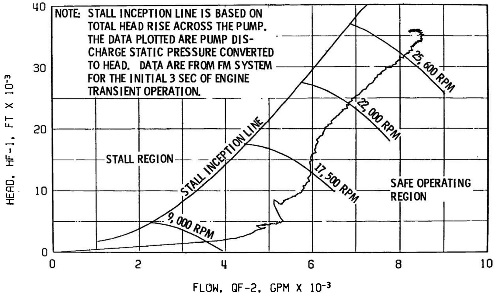
Fig. 48 Fuel Pump Start Transient Performance, Firing 01A
