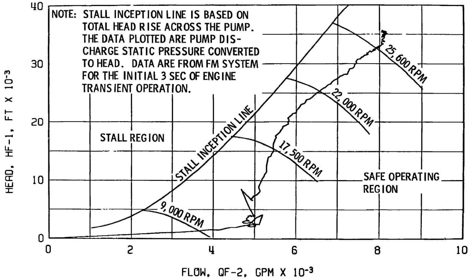
Fig. 38 Fuel Pump Start Transient Performance, Firing 43A
