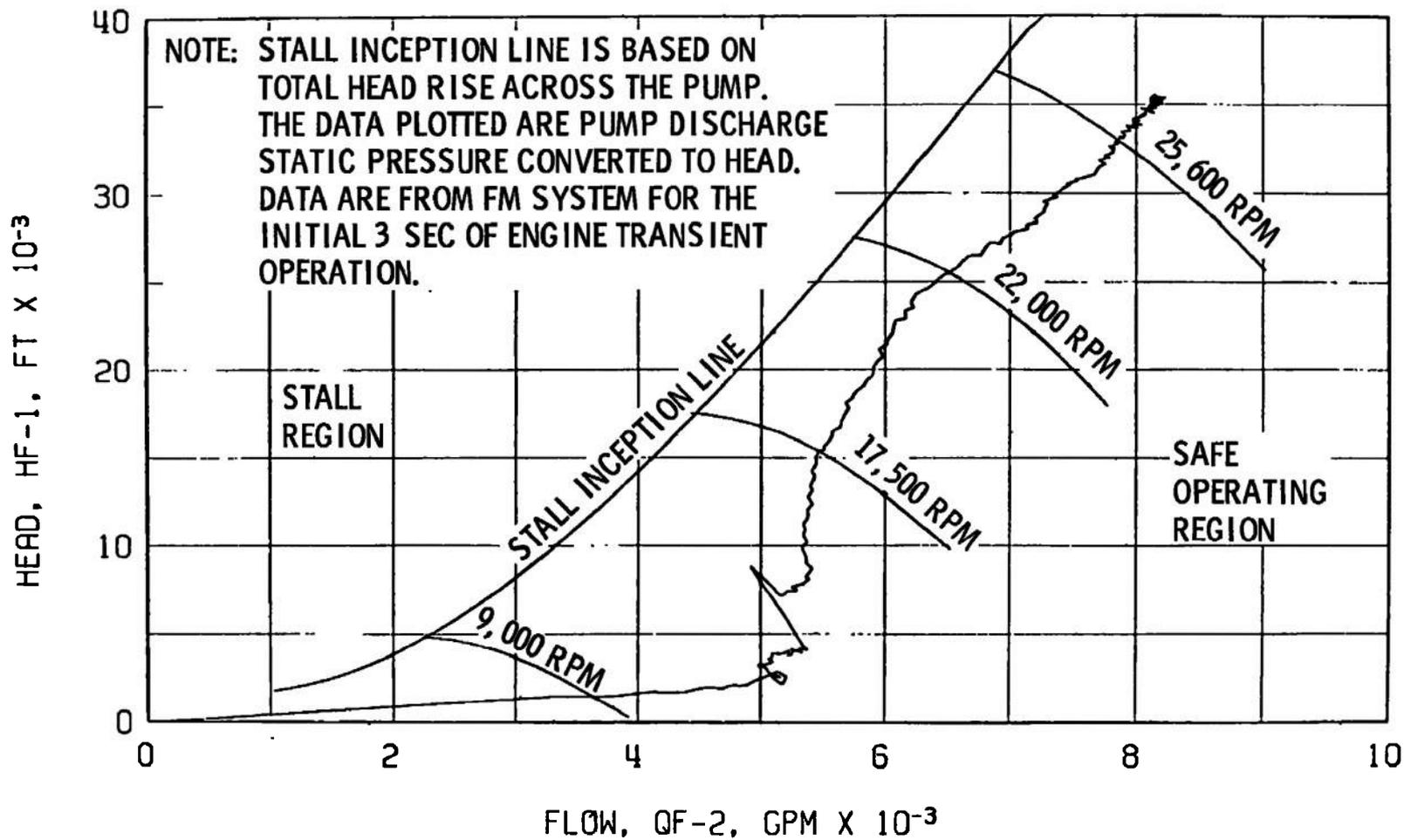
Fig. 13 Fuel Pump Start Transient Performance, Firing 42A
