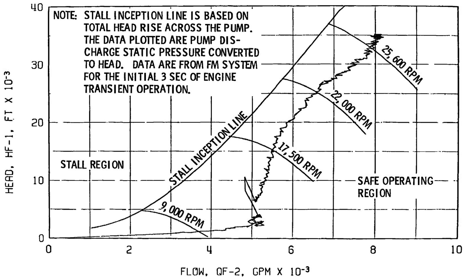
Fig. 58 Fuel Pump Start Transient Performance, Firing 01C
