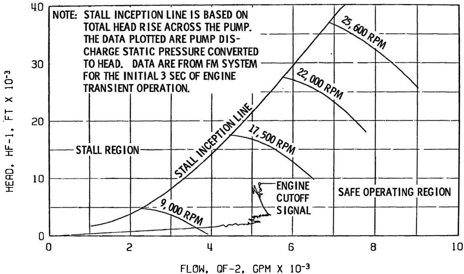
Fig. 33 Fuel Pump Start Transient Performance, Firing 42E
