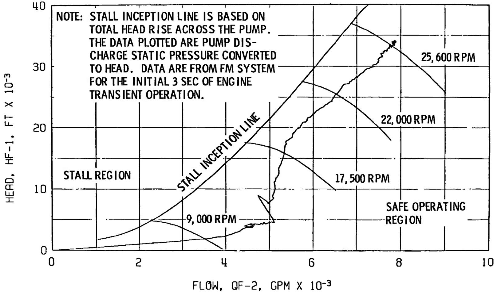
Fig. 28 Fuel Pump Start Transient Performance, Firing 42D
