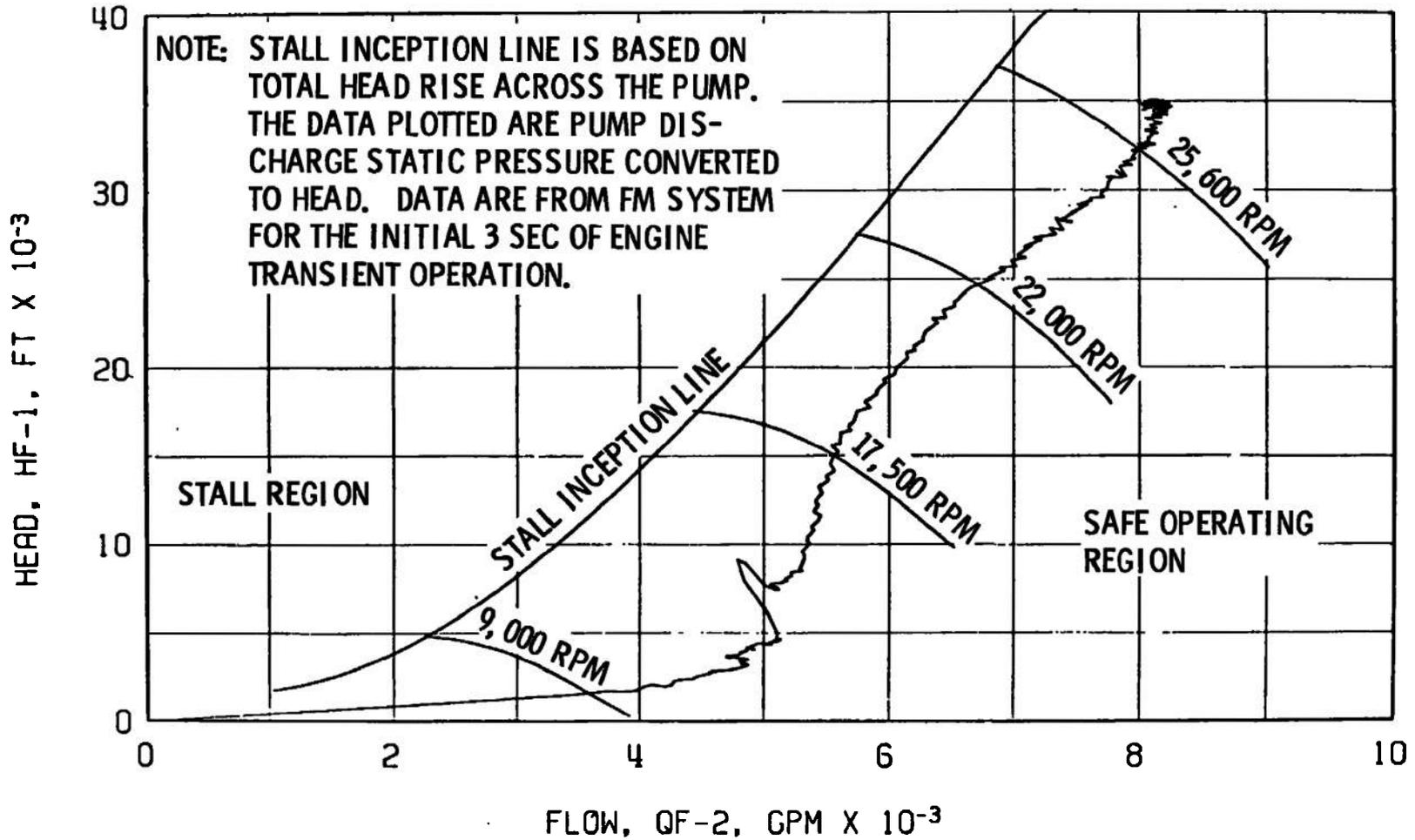
Fig. 53 Fuel Pump Start Transient Performance, Firing 01B
