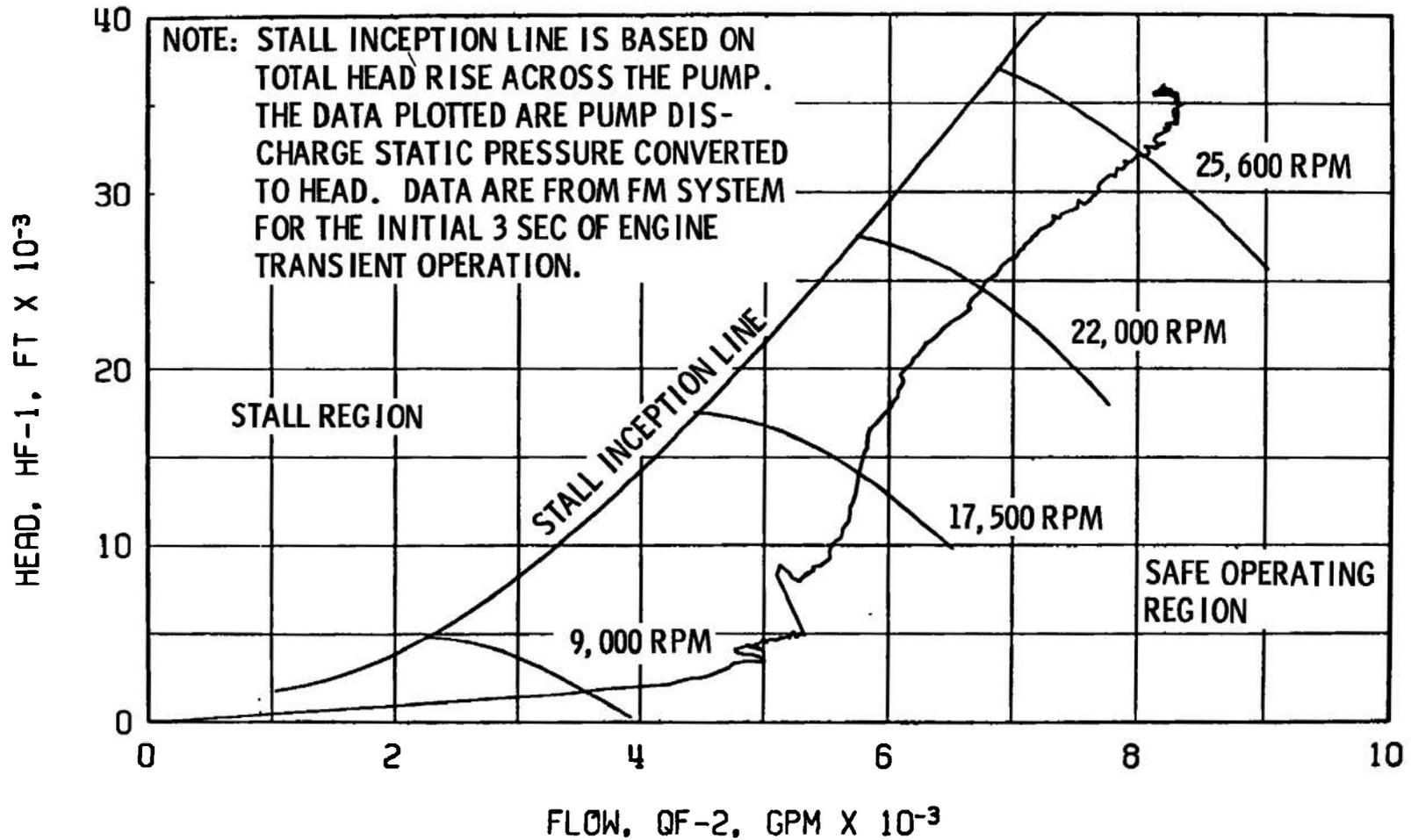
Fig. 43 Fuel Pump Start Transient Performance, Firing 43B
