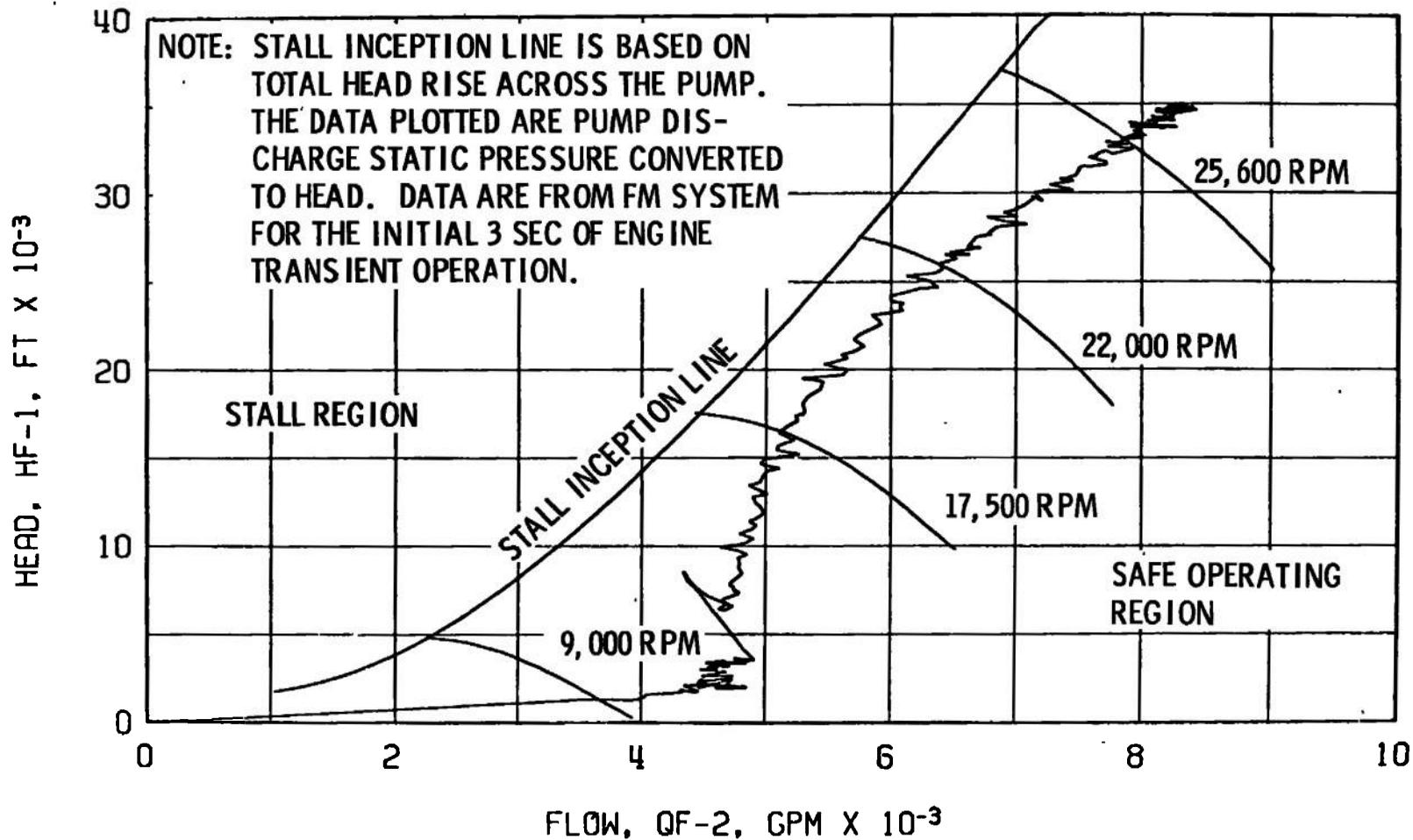
Fig. 73 Fuel Pump Start Transient Performance, Firing 02A
