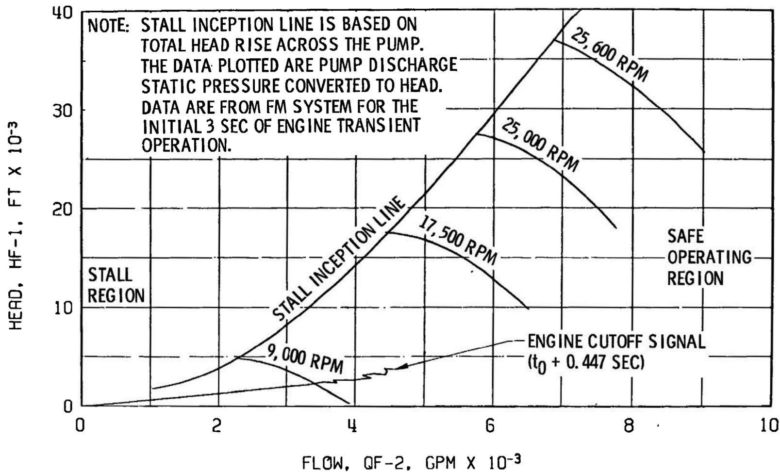
Fig. 88 Fuel Pump Start Transient Performance, Firing 02D
