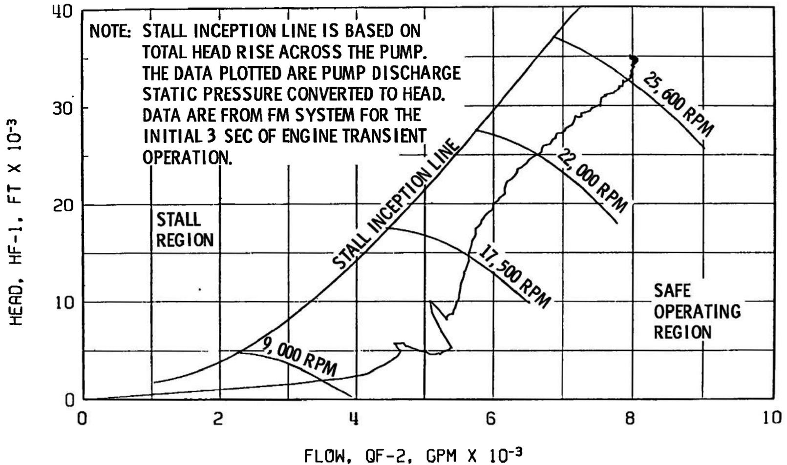
Fig. 23 Fuel Pump Start Transient Performance, Firing 42C
