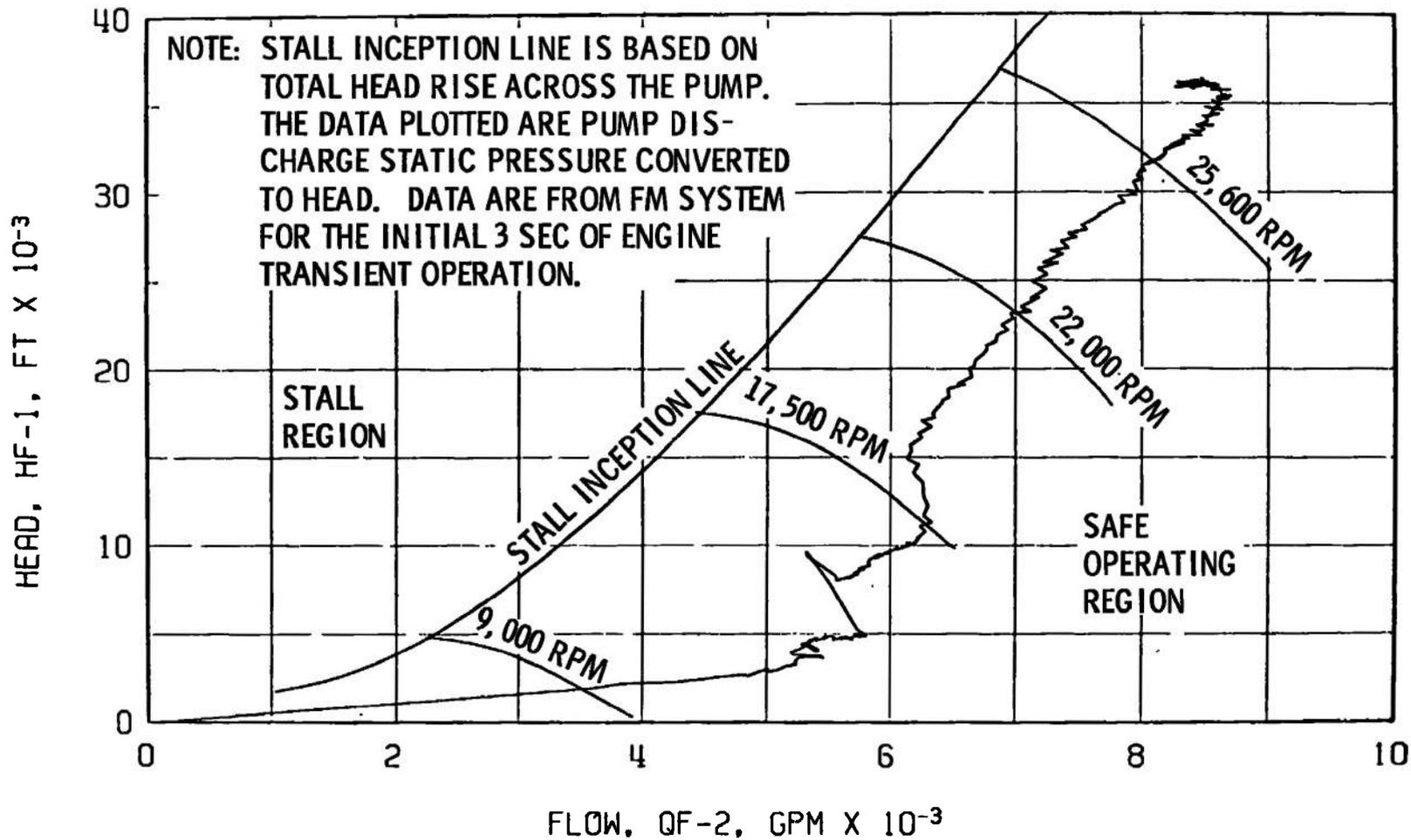
Fig. 63 Fuel Pump Start Transient Performance, Firing 01D
