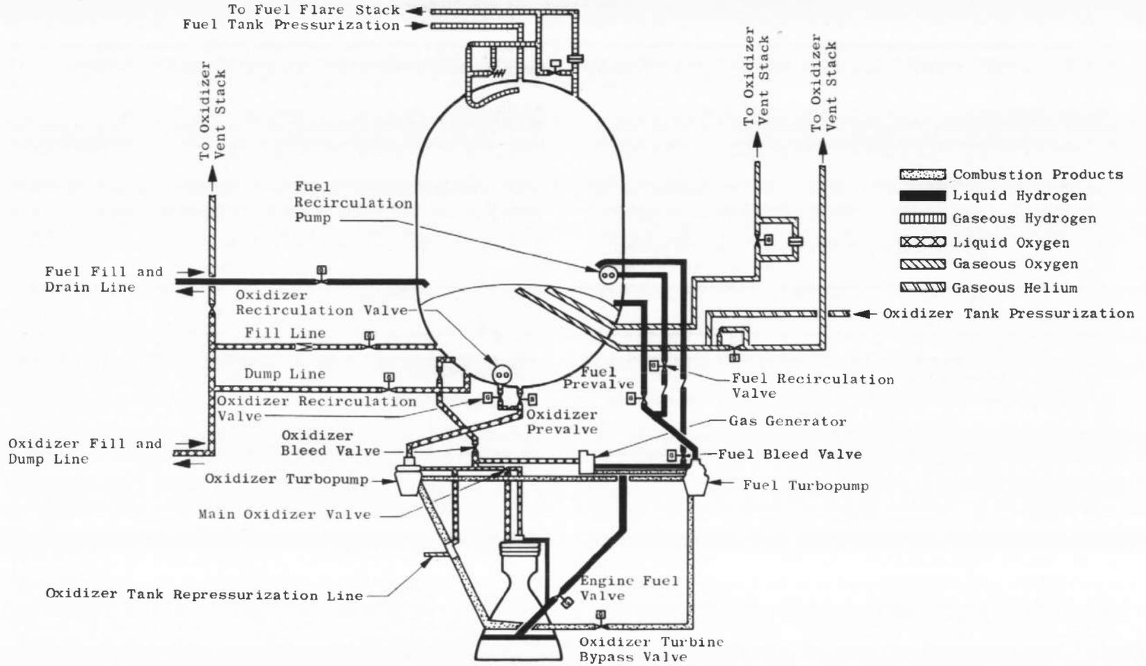
Fig. 5 S-IVB Battleship Stage/J-2 Engine Schematic
