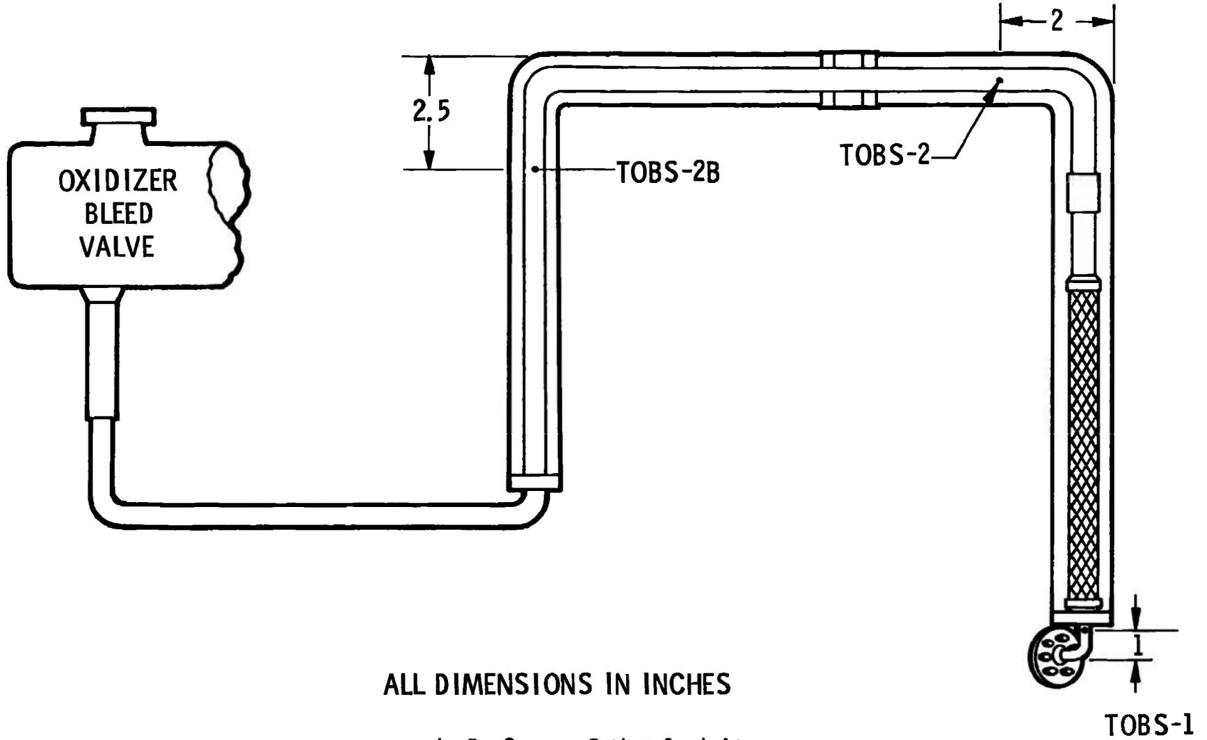
h. Gas Generator Oxidizer Supply Line
