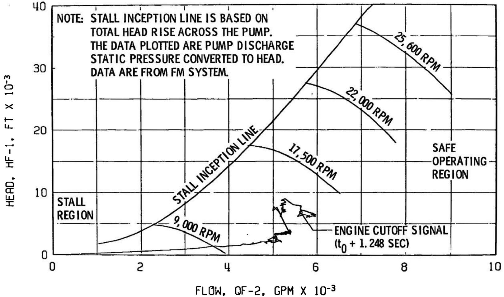
Fig. 68 Fuel Pump Start Transient Performance, Firing 01E
