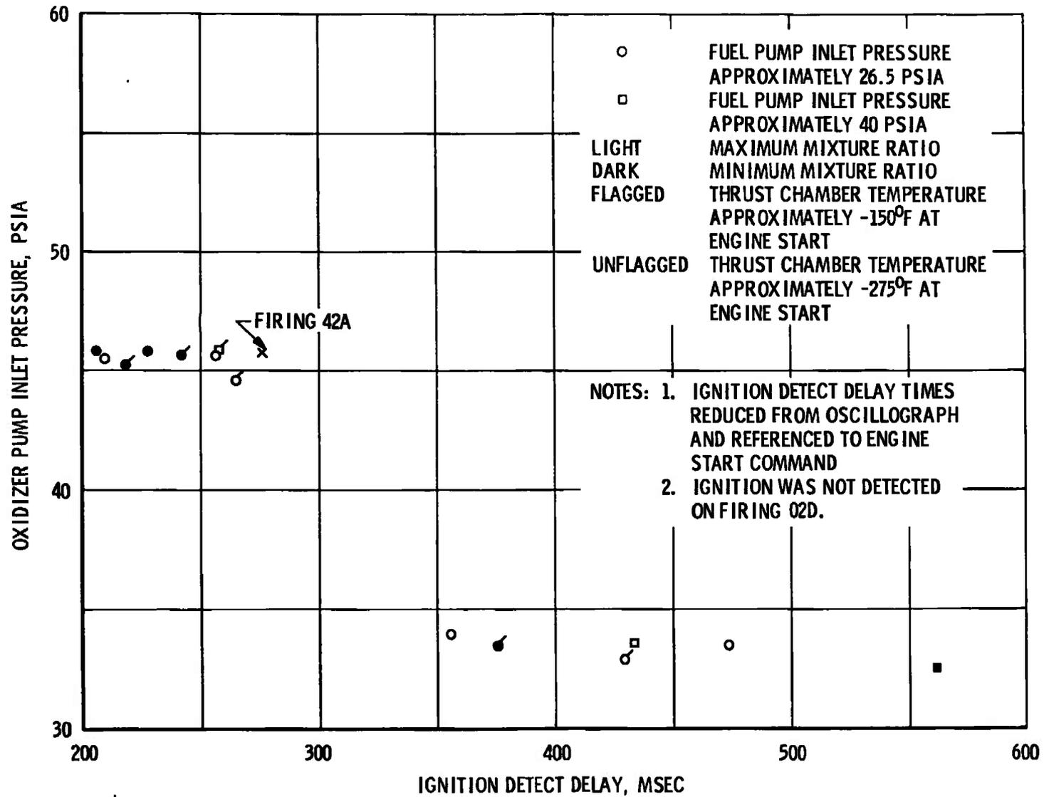
Fig. 91 Oxidizer Pump Inlet Pressure Effect on Augmented Spark
