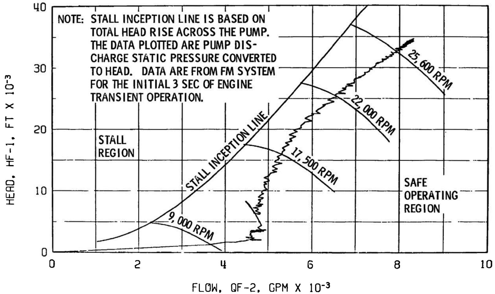
Fig. 78 Fuel Pump Start Transient Performance, Firing 02B
