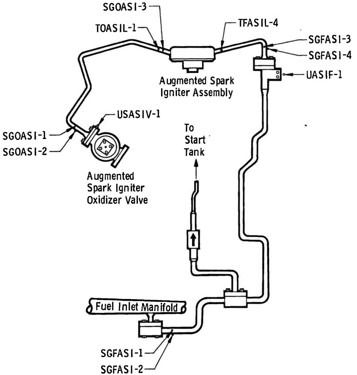
g. Augmented Spark Igniter Propellant Lines
