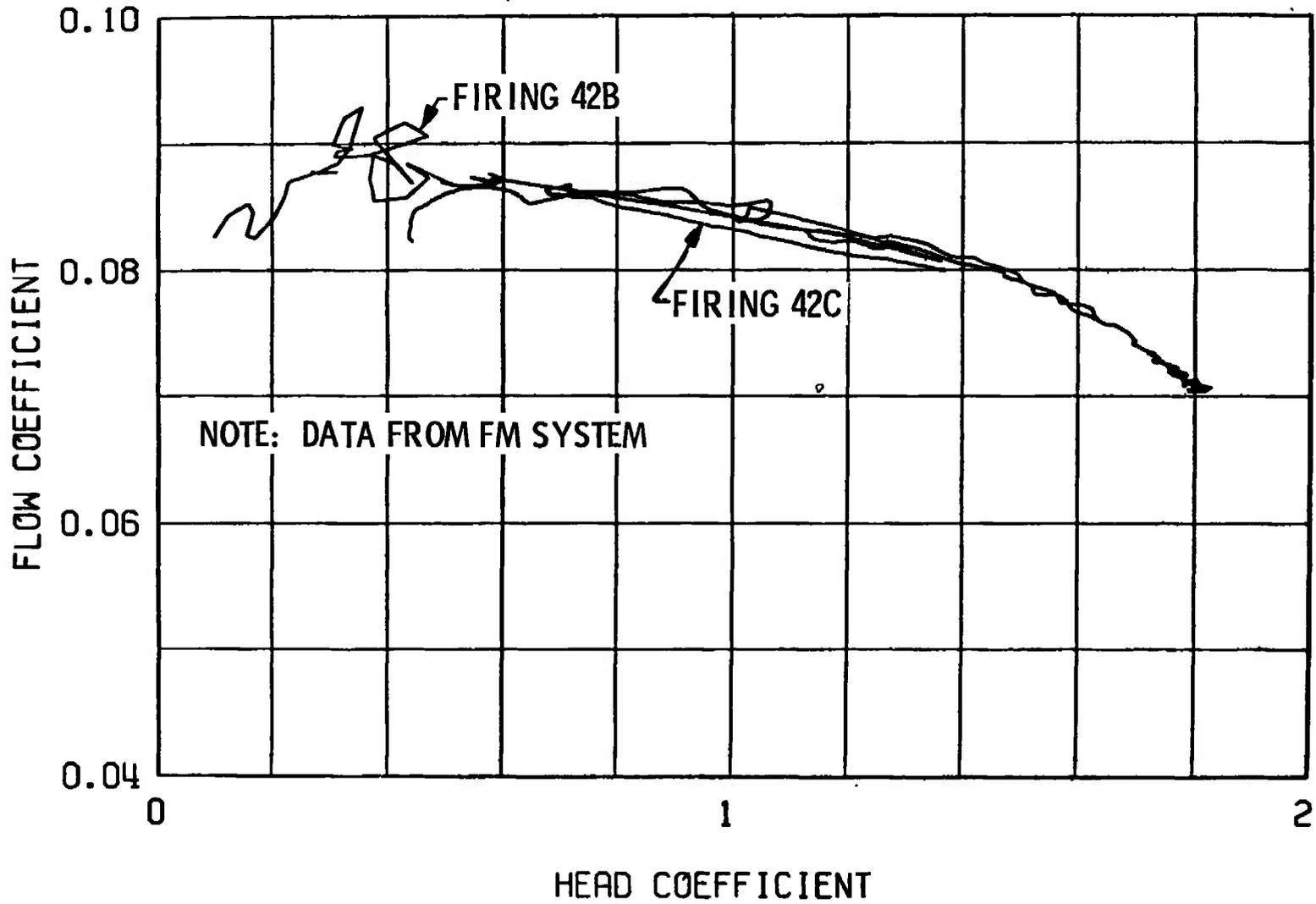
Fig. 94 Fuel Pump Operating Characteristics, Firings 42B and 42C
