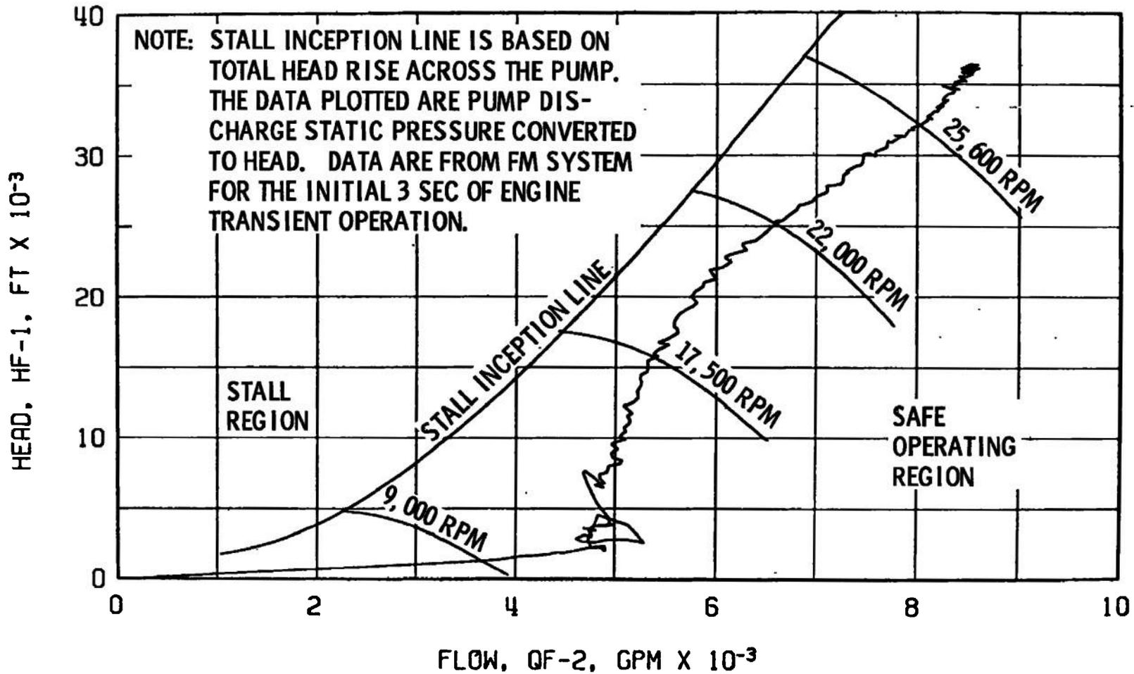
Fig. 83 Fuel Pump Start Transient Performance, Firing 02C
