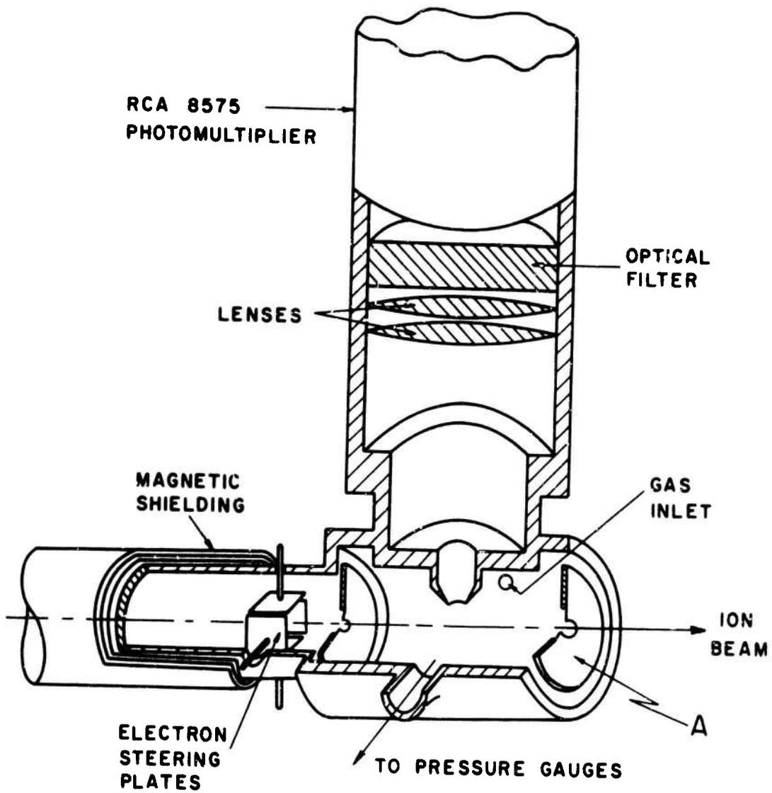
Figure 20. Details of the Collision Chamber and Optics in Studying Excitation of  $3914\text{\AA}$  Radiation
