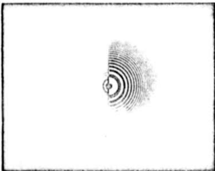
Fig. 2B. Interferograms of "synchronized" giant pulses, showing one supernumerary line in the slave laser spectrum.
