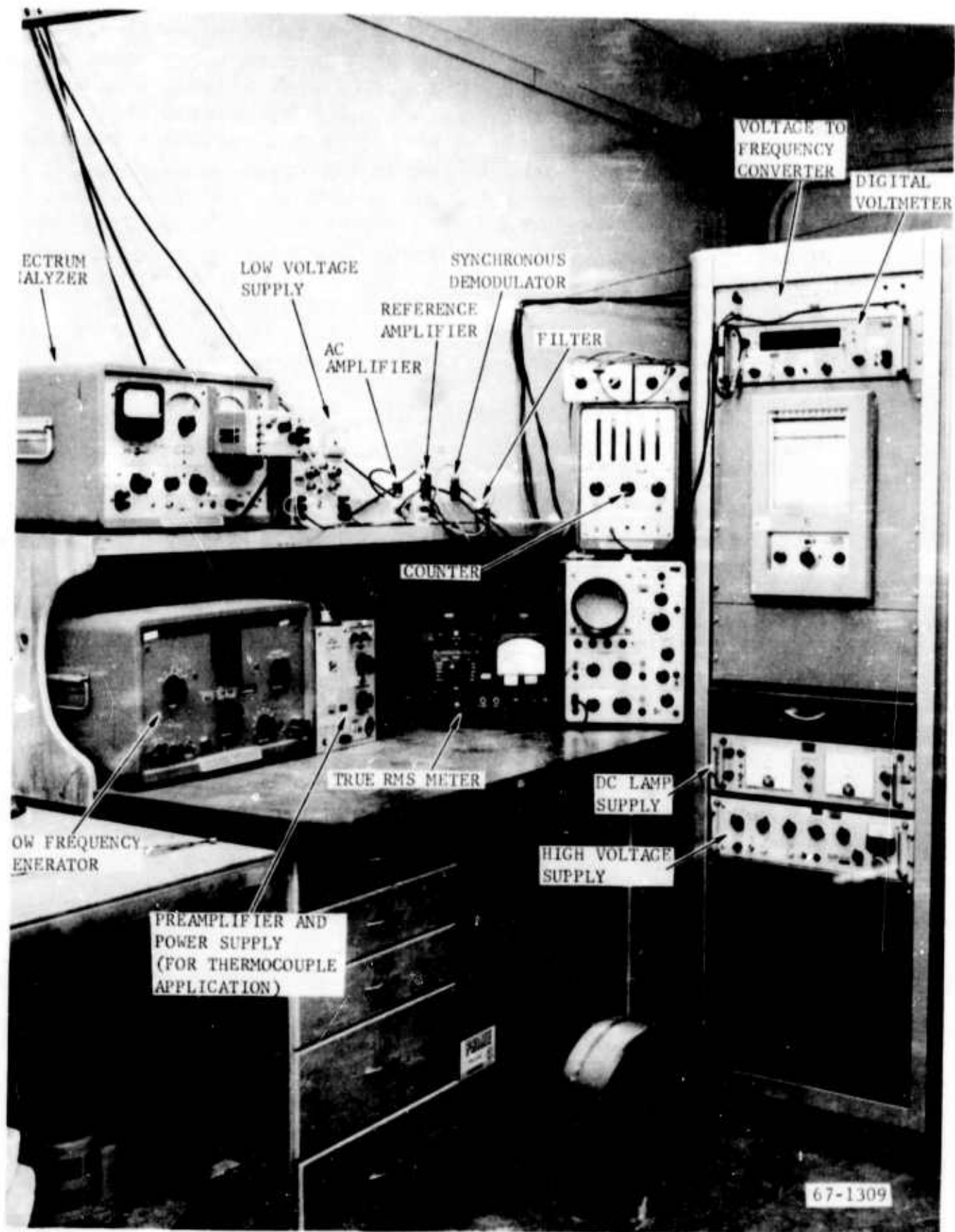
FIGURE 12. INSTRUMENTATION FOR THE OPTICAL PROBE SYSTEM AND FOR THE FAST RESPONSE THERMOCOUPLE PROBE
