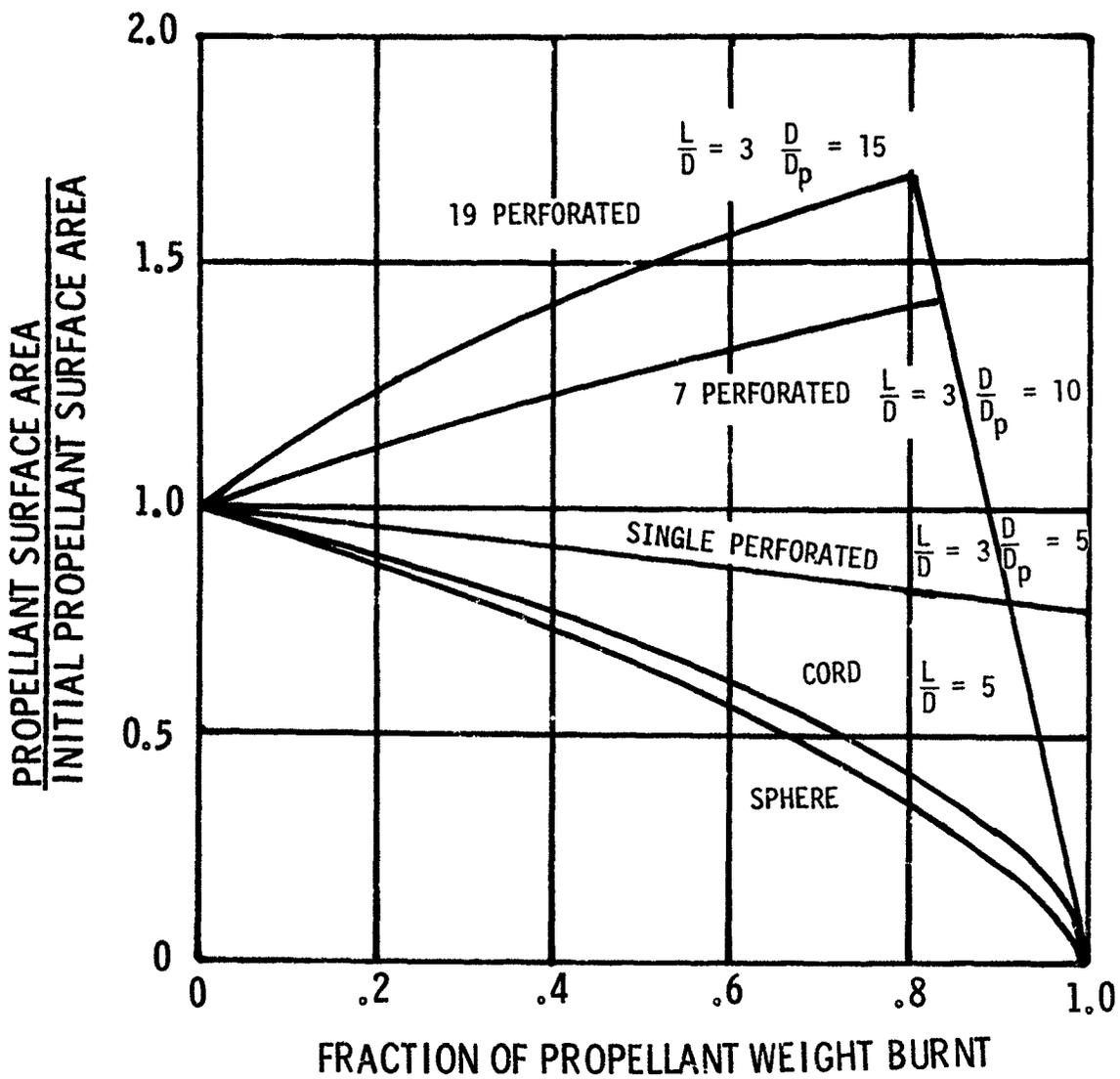
Figure 7. Variation of Propellant Burning Surface Ratio with Fraction Propellant Burnt for Various Grain Shapes.
